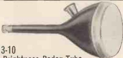
**MM13-10 High Brightness Radar Tube**
