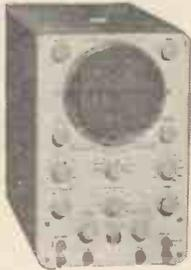
Laboratory quality at utility oscilloscope price and ease of assembly make this kit of outstanding value. Vertical frequency response 3 c/s to 5 Mc/s.,  $\pm 1.5$  dB. - 5 dB., sensitivity 10 mV. per cm. at 1 kc. Horizontal frequency 1 c/s. to over 400 kc/s. ( $\pm 1$  dB. up to 200 kc.). The Heath patented sweep circuit functions from 10 c/s to 500 kc. in five ranges giving five times the usual sweep of other 'scopes.
