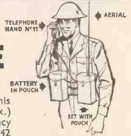
Mc/s., and operates from a Standard Dry Battery—HT/LT. 94/1. 3 v. (i.e. Ruben Mallory Type 1). 14 of the current series of B7G valves are employed: 1-3A4, 6-1L4, 4-1T4, 1-1S5, 2-1A3. Each set is fully tested and in good condition.
