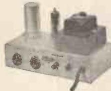
Compact, general purpose unit suitable for FM Tuners, Tape Recording Amplifiers and general Laboratory use. Input 100/120V, 200/250V, 40-60 c/s. Output 6.3 V 2.5A A.C.; 200, 250, 270V. 120 mA. max D.C. **£4.9.0**
