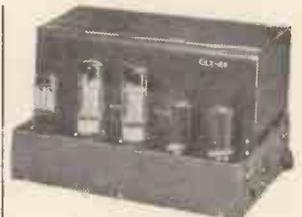
**DL7-35 Power Amplifier.** 54 watts peak output. Freq. response 5 c/s.-30 Kc/s ± 0dB. Two DL7-35 Amplifiers can be used in conjunction with SP21/2 Pre-Amplifier Control Unit for stereophonic reproduction. Size 14½in. long, 9in. wide, 8½in. high. List Price £31/10/-.
