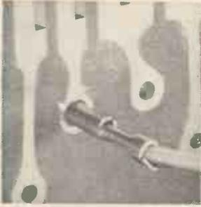
AMPin sel.-retaining pin for printed circuits.
