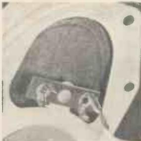
AMP Miniature Faslon Receptacles for loudspeaker and printed circuit tabs.
