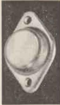
Here is the OC35—a new power transistor which supercedes the OC16 as a standard type for general use in industry. The OC35 is inexpensive and has a maximum current rating twice that of the OC16. It is well suited for use in a wide variety of industrial low frequency amplification and electro-mechanical applications, and in particular those equipments which are operated from a 12 volt supply.
