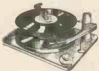
4-speed plays 10 records 12in., 10in., or 7in. at 16, 33, 45 or 78 r.p.m. Internazies 7in., 10in. and 12in. records of the same speed. Has manual play position; colour brown. Dimensions: 12in. x 10in. Space required above baseboard 4in., below baseboard 2in. Fitted with Ful-Fi turnover crystal head. £8/19/6. Plus 5/- P. & P.
