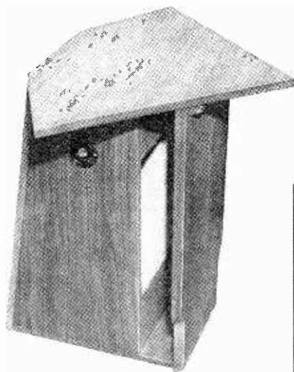
Goodman's hyperbolic-exponential law horn loudspeaker removed from the room corner and viewed from one side to show one of the two horn mouths.
