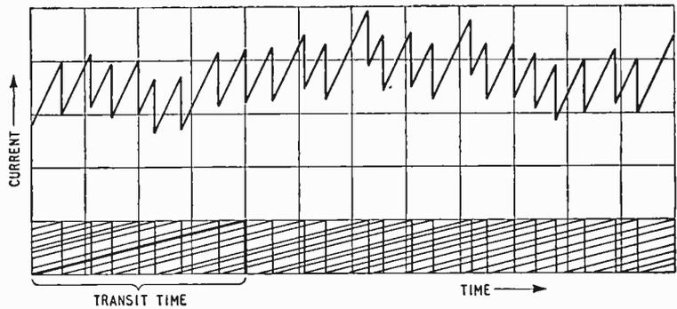
Fig. 3. Here there are, on the average, 8 electrons in flight all the time, but they start at irregular intervals. The resulting total current therefore has a slow irregular fluctuation as well as the fast saw-tooth ripple.
