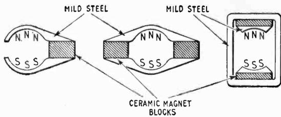
Fig. 3. Three typical methods of using anisotropic ceramic magnets as d.c. motor stators.
