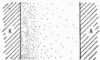
Fig. 4. The many electrons emerging from the cathode, on the left, form a negative space charge that neutralizes the distant positive charge on the anode and restricts further movement towards it. The surplus electrons are forced back to the cathode.
