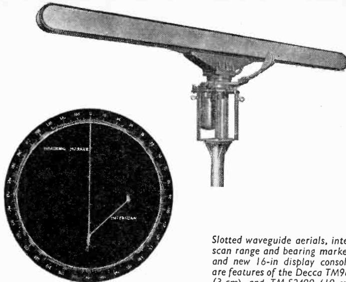
Slotted waveguide aeriels, inter-scan range and bearing markers and new 16-in display consoles are features of the Decca TM969 (3-cm) and TM-S2400 (10-cm) marine radars.
