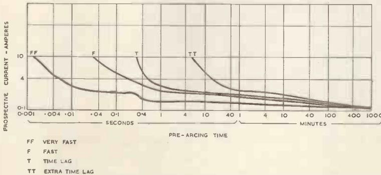
drawn through a minimum of six points plotted on Cartesian coordinates whose axes are prospective current, and pre-arcing time, shown on logarithmic scales. The current source which is used to obtain the results so plotted is usually D.C., since an alternating supply would give misleading results at very short pre-arcing times because they would depend on the instantaneous value of the current at the time of applying the overload; at fairly long pre-arcing times, of course an alternating
