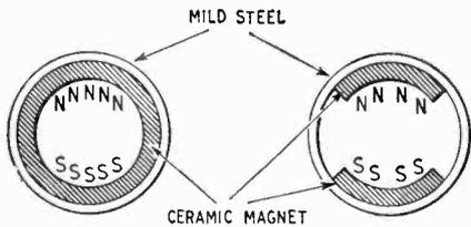
Fig. 2. Isotropic ceramic magnets for d.c. motor stators. Continuous cylinder (left) segments (right).
