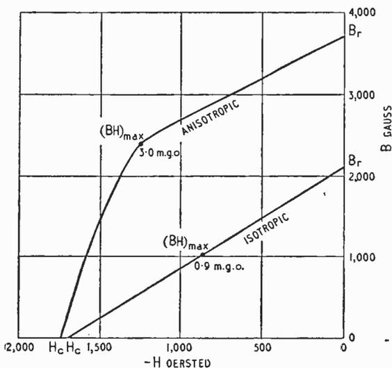
Fig. 1. Demagnetization curves for barium ferrite.
