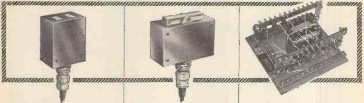
The Proximity Switch will provide a signal to operate a Basic Logic Unit, whenever a mass of ferrous material comes within 5mm of the operating face. Having no moving parts, it is an encapsulated wound component suitable for use in conditions of vibration, shock, dust, damp—in fact, in any environment where the epoxy potting compound and the cable gland will not be damaged.
