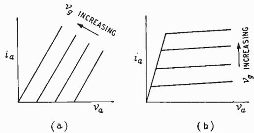
Fig. 1. Idealized triode (a) and pentode (b) characteristics.
