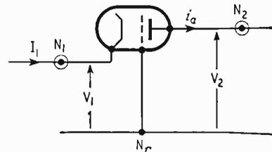
Fig. 9. Basic ideal grounded-grid valve.
