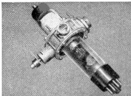
Fig. 4. Typical 3,000-Mc/s Klystron oscillator, the Type CV67.
