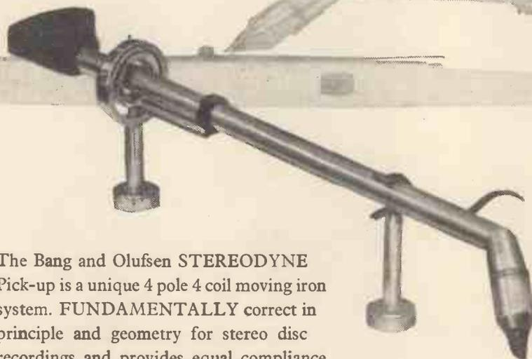
The Bang and Olufsen STEREO DYNE Pick-up is a unique 4 pole 4 coil moving iron system. FUNDAMENTALLY correct in principle and geometry for stereo disc recordings and provides equal compliance in all directions with high channel separation through the entire frequency range.
