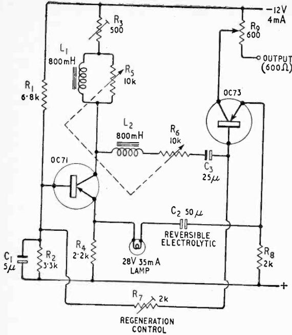
amplifier it is possible to maintain correct bias conditions very easily, merely by biasing the first stage directly and the last stage by means of negative feedback.
