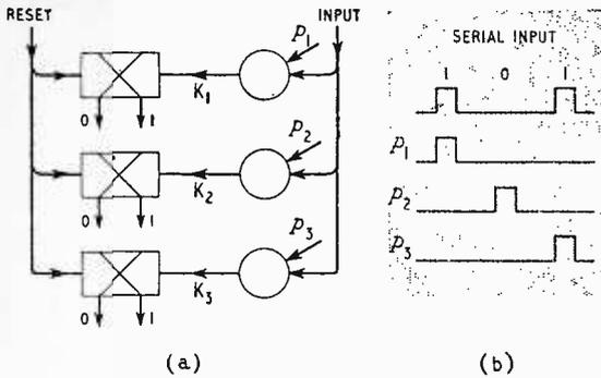
Fig. 10 (a) Staticisicor (store) for serial input train of three binary pulses. (b) Serial input train and clock pulses for storing 101 in the staticisicor of Fig. 10 (a).
