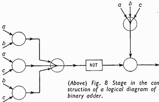
(Above) Fig. 8 Stage in the construction of a logical diagram of a binary adder.
