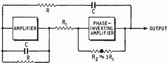
When this oscillator was subjected to temperature variation of 20°-80°C., it is stated that the frequency shifted by less than 0.1% and the output change was less than 1%.
