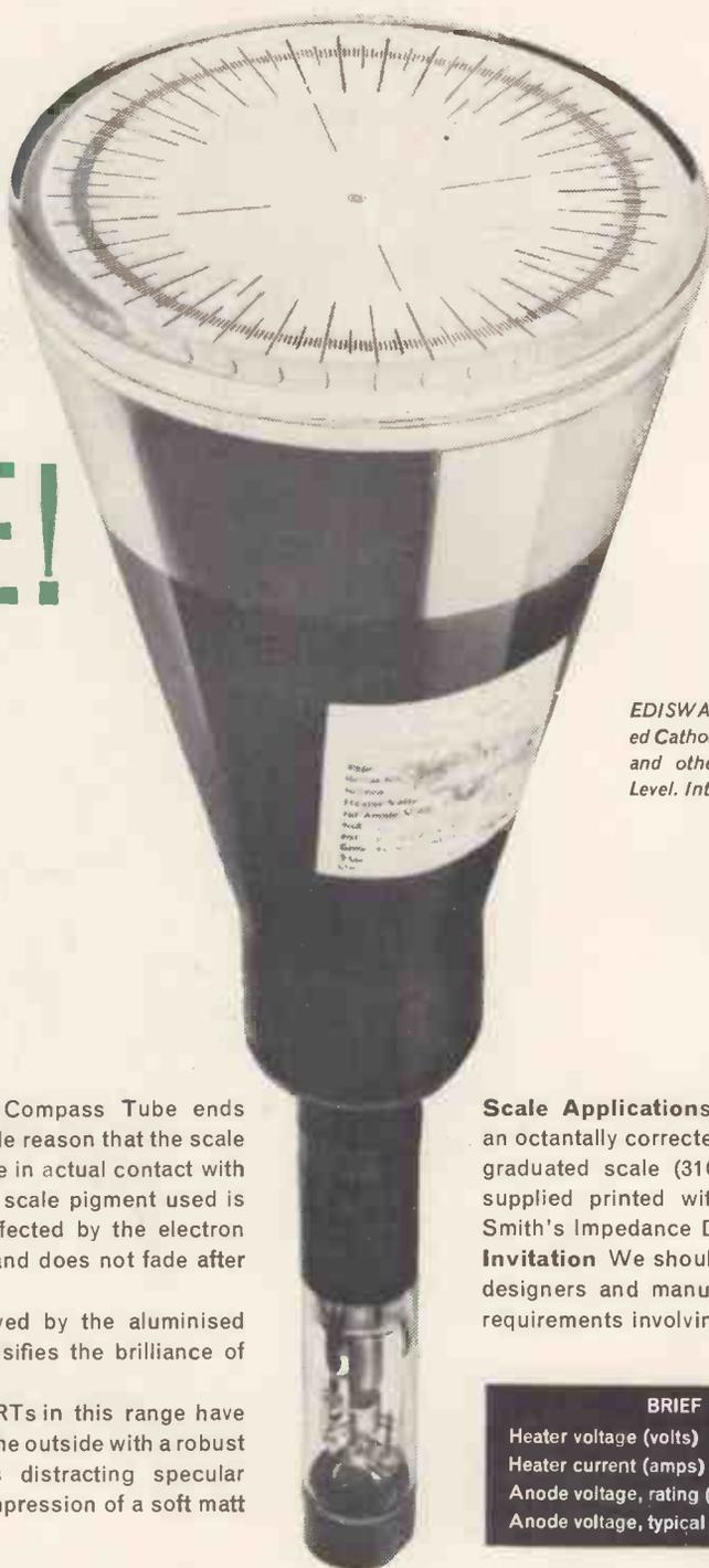
*EDISWAN 6-in. Aluminised Indirectly Heated Cathode Ray Tube for Radio DF Compass and other applications. High Brightness Level. Internal Scale.*
