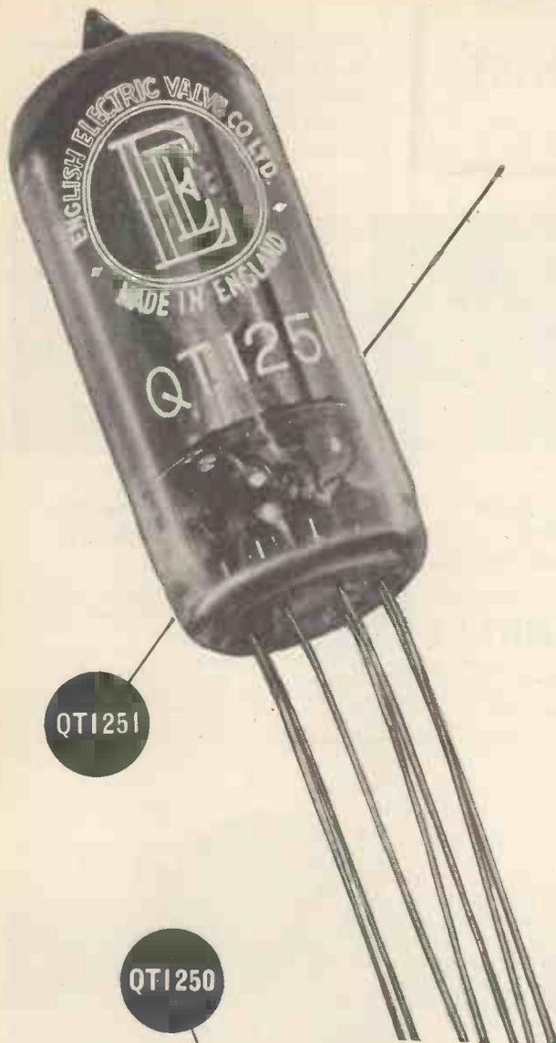
QT1251 was developed by the ENGLISH ELECTRIC VALVE COMPANY LTD. from the well known 5823 with the object of reducing the tolerance on trigger breakdown voltage. Flying leads have been incorporated for direct wiring-in. The improved characteristics find particular application in electronic telephone exchanges.
