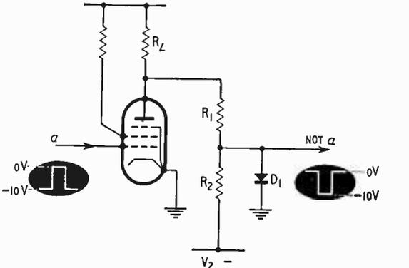
Fig. 6 Voltage inverter circuit of a NOT gate.
