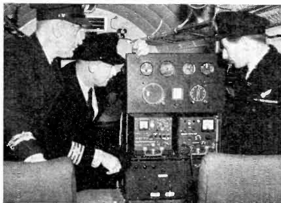
Doppler navigation equipment (Marconi) in a Viking aircraft.
