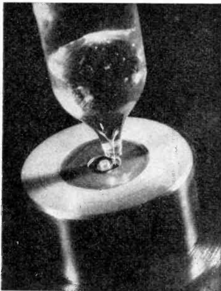
Electrolytic etching of grid groove of alcatron.
