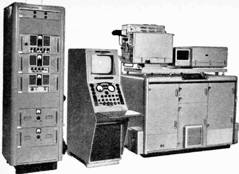
The B.B.C. standards converter. From left to right: the flicker correction bay, the camera and display control unit with monitor, and the display pedestal including the camera and display tube.
