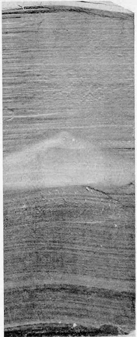
Fig. 10. Section across similar groove to Fig. 9 taken after 250 playings with a 1-mgm stylus at 2.7gm tracking weight. The path of the stylus is only perceptible as a smoother surface.
