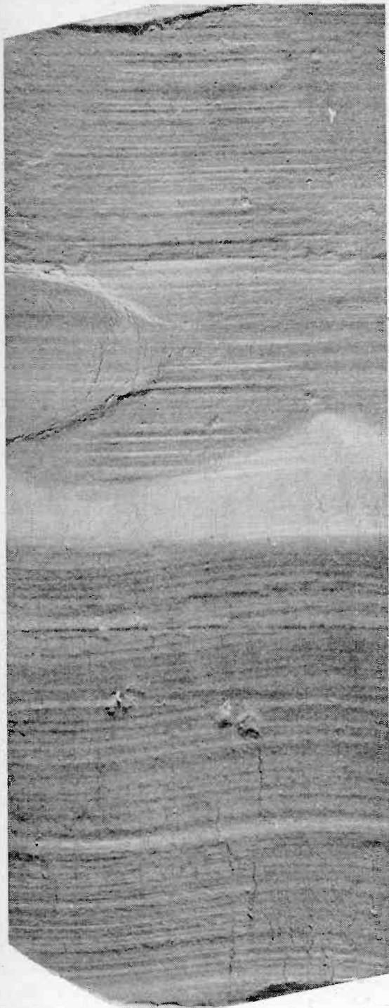
Fig. 9. Section of a flattened electron micrograph impression (X2400) of 5cm/sec r.m.s. 10kc/s stereo test record groove taken after one playing with a 3-mgm stylus at 2.7gm tracking weight. While the width of the indent shows a depth of permanent deformation equal to nearly half the amplitude of the modulation, the actual path of the stylus described on the unmodulated wall indicates that it penetrated to a depth nearly equal to that of the modulation.
