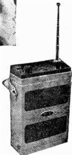
Right: B.C.C. Type 40 a.m. or f.m. packset, to work in the range 30-174 Mc/s.
