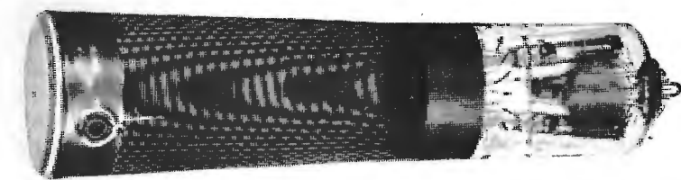
Above: Double-beam oscilloscope tube, Type E10-10GH ("La Radio-technique").
