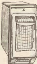
Range: 1 mA. direct-to-movement, D.C., and 1.1 mA. A.C. through internal rectifier. Curvilinear trace. 3/16 in. wide strip chart. Two-speed electric chart drive (230 v. A.C.) at 1 in. and 6 in. per hour. Two limit contacts provided for high and/or low current alarm.
