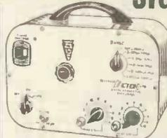
Covering 100 Kc/s-100 Mc/s. on fundamental and 100 Mc/s. to 200 Mc/s. on harmonics. Metal case 10in. x 6½in. x 5½in., grey hammer finish. Incorporating three miniature valves and metal rectifier. A.C. mains 200/250 v. Internal Modulation of 400 c.p.s. to a depth of 30%. Modulated or unmodulated R.F. output continuously variable 100 millivolts C.W. and mod. switch, variable A.F. output. Incorporating magic-eye as output indicator. Accuracy plus or minus 2%.
