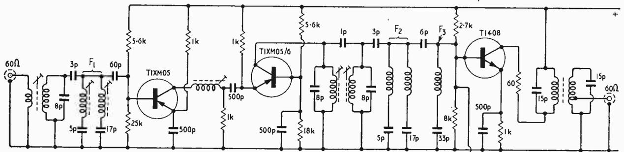
Fig. 3. Converter using germanium transistors. ( $F_1 = F_2$  = series resonance at 97 Mc/s and at 203 Mc/s with parallel resonance at 145 Mc/s.  $F_3$  = series resonance at 29 Mc/s with  $Q = 10$ ).
