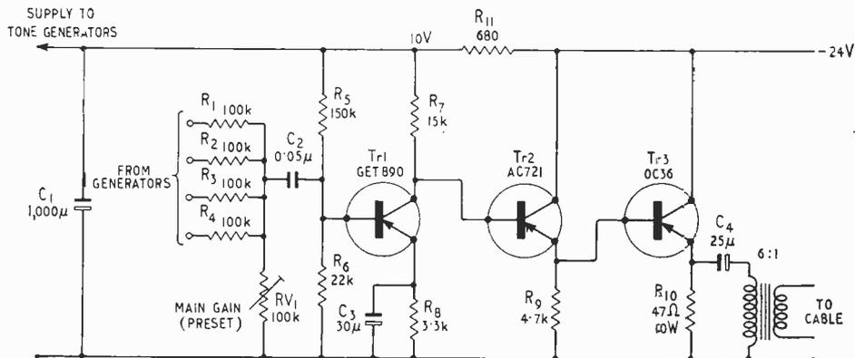
Fig. 3. Circuit of control amplifier (common to all tone generators) feeding the cable.
