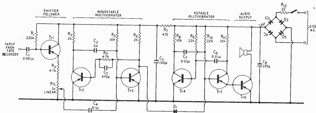
Fig. 1. Circuit diagram of the recording level indicator.
