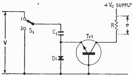
Fig. 4. A more refined version of the diode-transistor pump.
