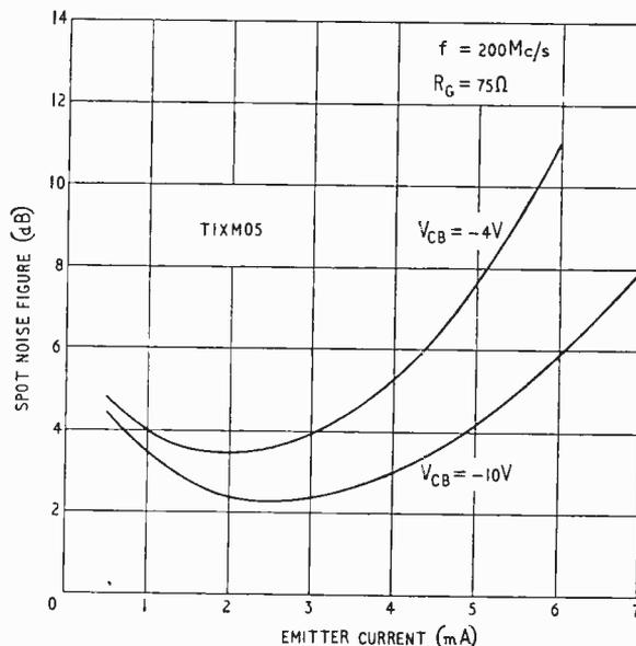
Fig. 4. Spot noise figure vs. collector current of TIXMOS transistor.
