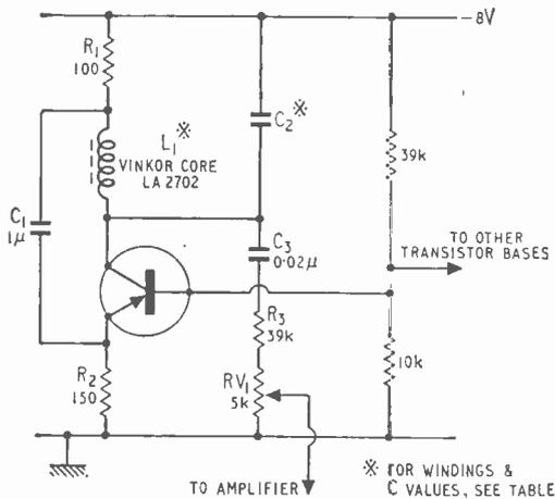
Fig. 8. Audio frequency control tone generator.
