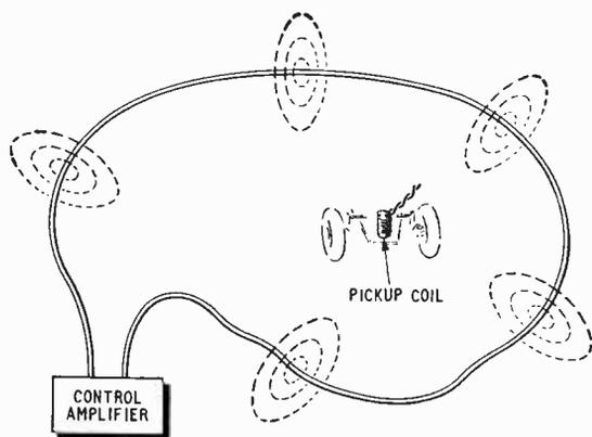
Fig. 1. Plan view of cable loop surrounding an area. The pick-up coil on the vehicle is mounted vertically.
