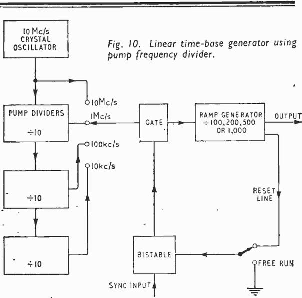
Fig. 10. Linear time-base generator using pump frequency divider.
