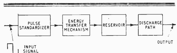
Fig. 1. Basic pump arrangement.
