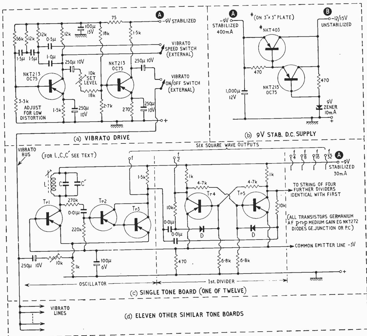
Fig. 2. Circuits grouped in tone generator assembly, including (a) vibrato oscillator and driver, (b) 9 V, 400 mA stabilized d.c. supply, each of which is ancillary to (c) and (d), the twelve tone boards, each with an oscillator and five dividers, together giving square wave outputs at six octave-related pitches.
