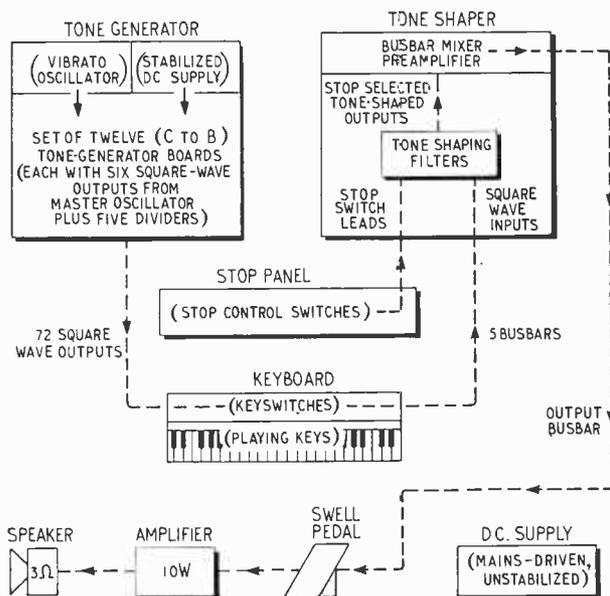
Fig. 1. System block diagram of home-constructed simple single-manual, bolyphonic, divider-type transistor electronic organ.
