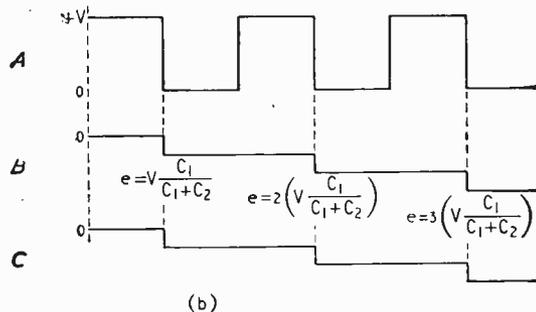
Fig. 3(a). Diode-transistor pump (original version). D<sub>1</sub> is replaced by the emitter follower Tr1 so that the voltage at B follows that at C. (b) Voltage waveforms at points A, B and C in (a).
