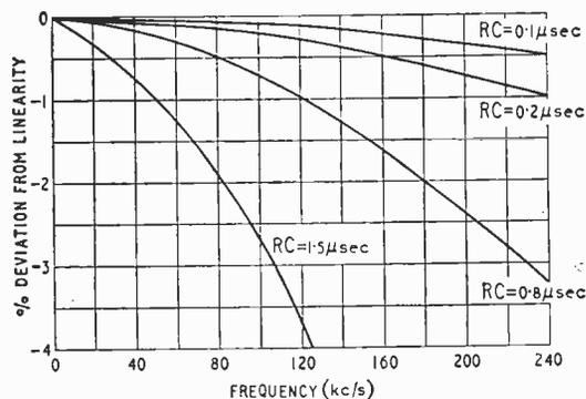
Fig. 6. Effect of charging time constant on linearity.
