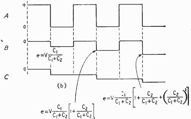
Fig. 2(a). Simple diode pump circuit. S<sub>1</sub> simulates a rectangular wave input. (b) Voltage waveforms at points A, B and C in (a).
