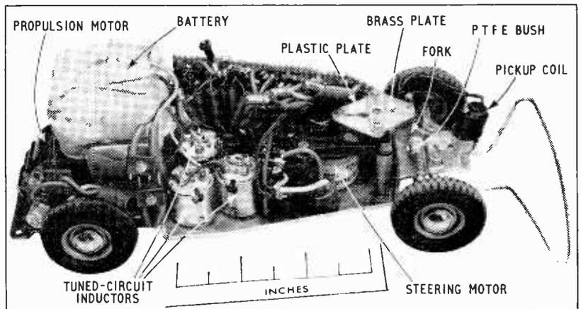
Fig. 7. Model with conventional steering by actuator. The pick-up coil is just ahead of the front wheels (right). The wire structure in front of them is a bumper. The large battery is mounted between the rear wheels.
