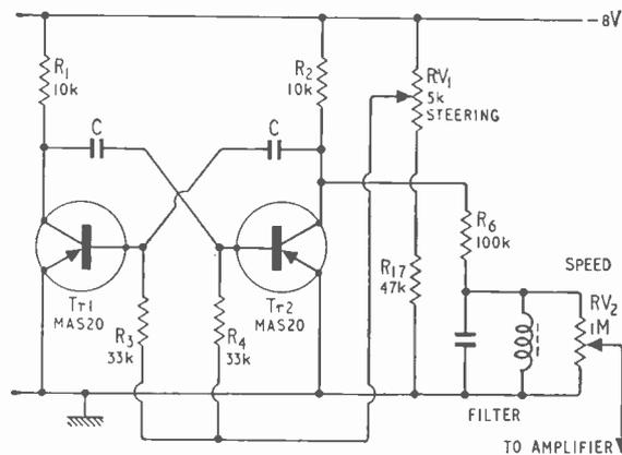
Fig. 11. Control tone generator for simplified model in Fig. 10. Capacitors  $C$  are about  $0.01\mu F$  and can be found by experiment, as can the  $L$  and  $C$  values of the filter (using a Vinkor core for the inductor).
