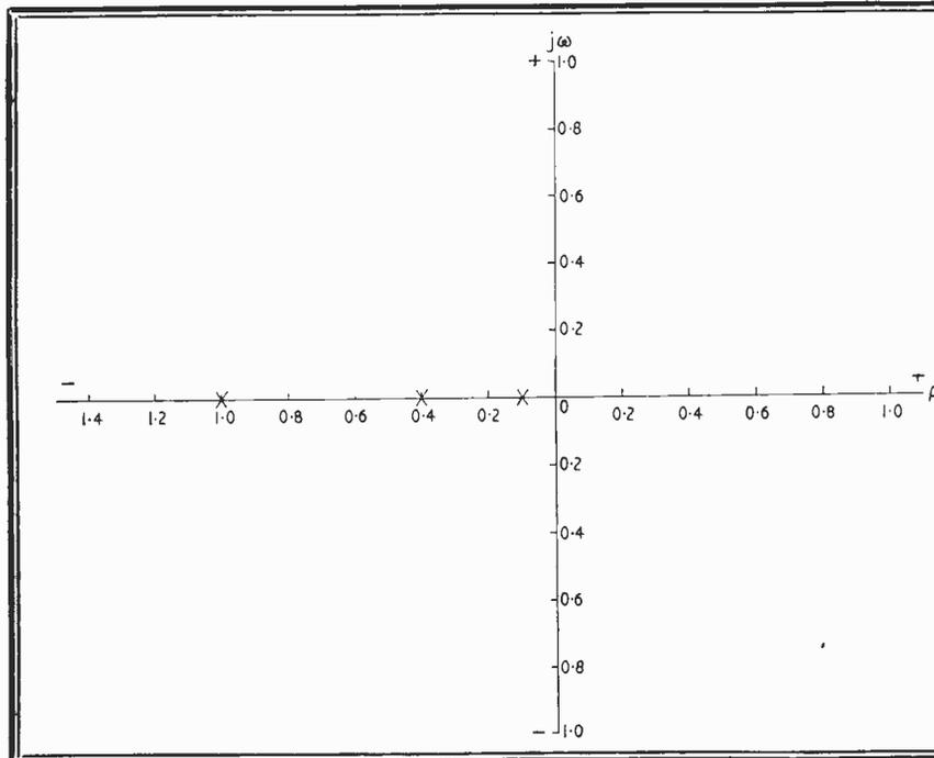
Fig. 1. For a root-locus plot the real and imaginary axes must be scaled the same. The first step is to plot the values of the poles and zeros. Here there are three real poles indicated by crosses.
