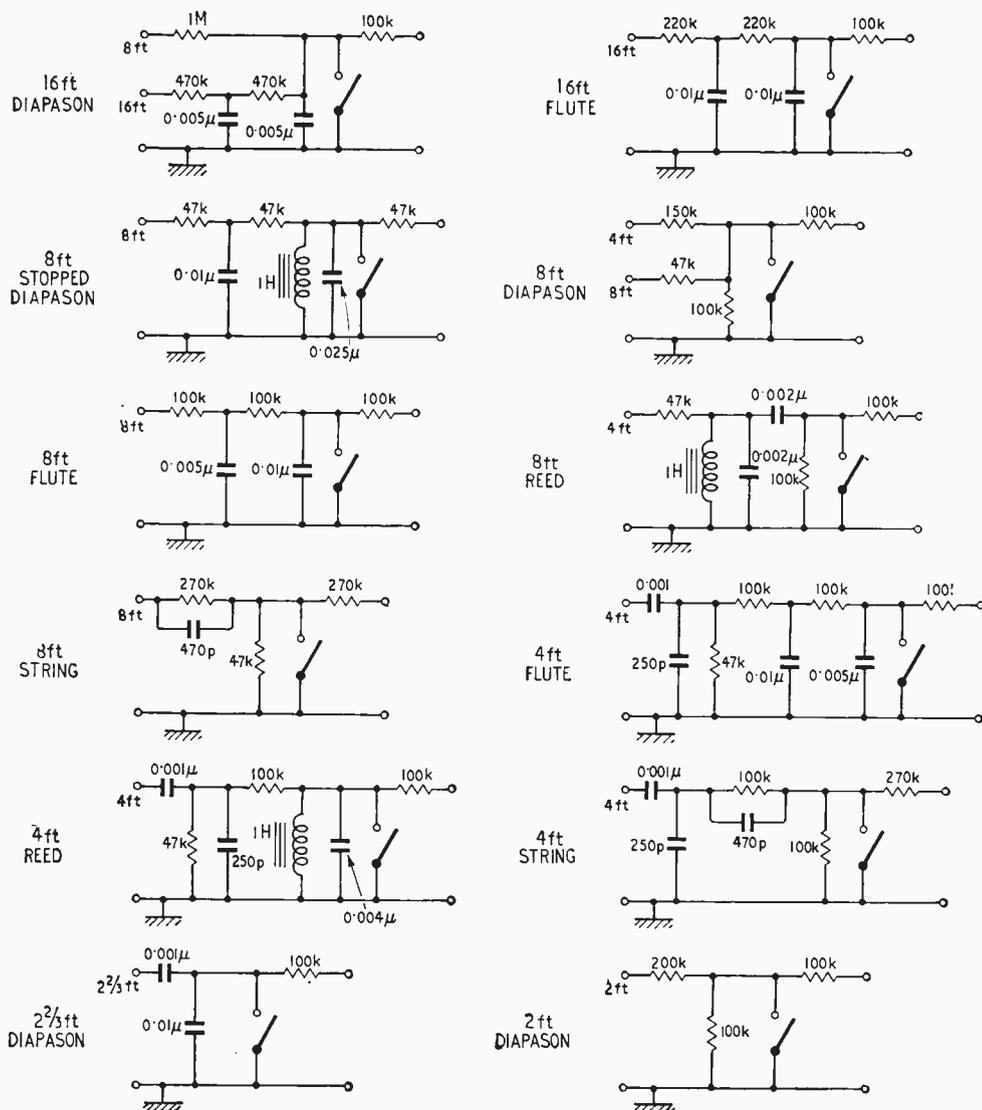
Fig. 6. Stop (tone filter) circuits; square wave input from left, out of corresponding bus pre-amplifier 5k output resistance; shaped outputs commoned to right into single bus mixer-amplifier input of approximately 10k resistance with same circuit as bus pre-amplifier, Fig. 5(b).
