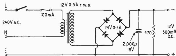
Fig. 8. 12 V, 500 mA d.c. unstabilized supply for oscillators, dividers and bus pre-amplifiers and mixer-amplifiers.
