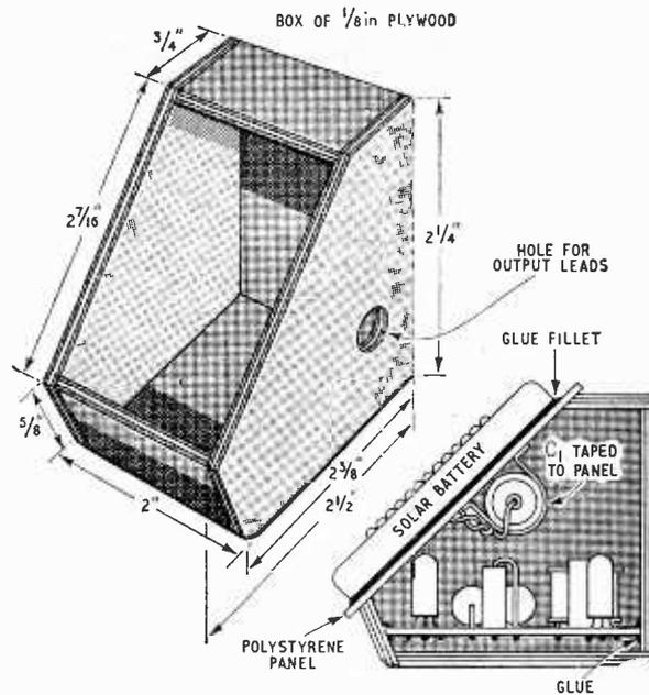
Fig. 5. Details of the housing of the charger. All joints are glued with epoxy resin and finished with polyurethane varnish.
