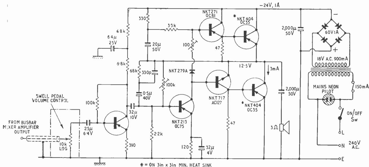
Fig. 7. 10 W power amplifier; mains driven; 3 ohm load, 100 mV input sensitivity; 10 k input resistance; swell pedal volume control at input
