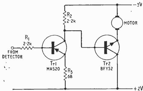
Fig. 5. Circuit of non-reversing drive for cars.
