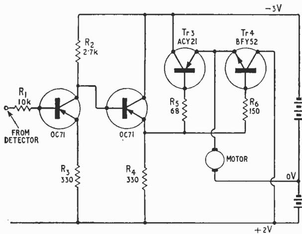
Fig. 6. Reversing drive circuit for cars.
