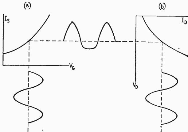
Fig. 2. Illustrating the "double deformation" process: (a) deformation caused by square-law characteristic of r.f. amplifier; (b) cancellation of distortion by "variable battery" effect.
