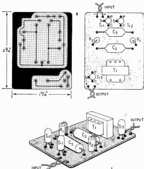
Fig. 4. Etched circuit and disposition of components.
