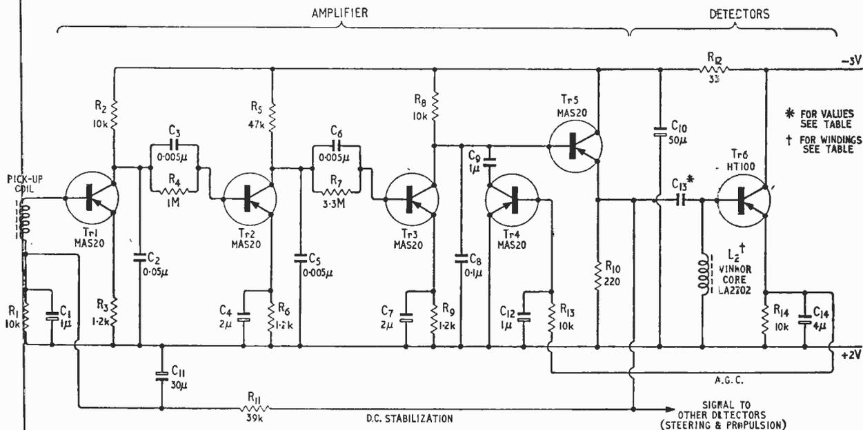
Fig. 4. Receiver circuit for the cars. D.C. control voltages are taken from the emitters of the steering and propulsion control detectors corresponding to Tr6.
