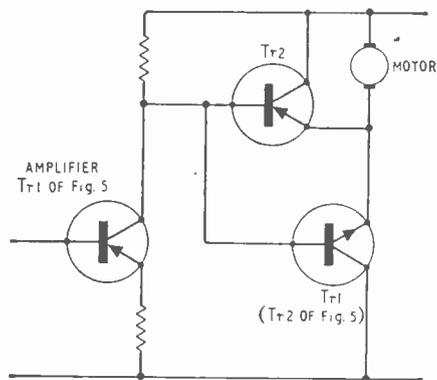
Fig. 9. Braking circuit.
