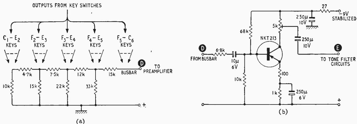
Fig. 5. Bus equalization and amplification provision; identical for each of five busbars (16 ft, 8 ft, 4 ft, 2½ ft, 2 ft); (a) attenuation network elements inserted between E and F in every octave except lowest; (b) bus pre-amplifier with output level setting provided by preset potentiometer in transistor collector circuit.
