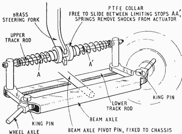
upper track rods, which are joined at their extremities to the firm lower track rod, supplied with the model. The whole front axle assembly is mounted on a single central pivot, so that it can accommodate itself to rough surfaces.
