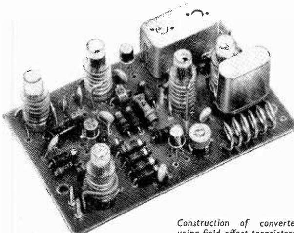
Construction of converter using field-effect transistors.
