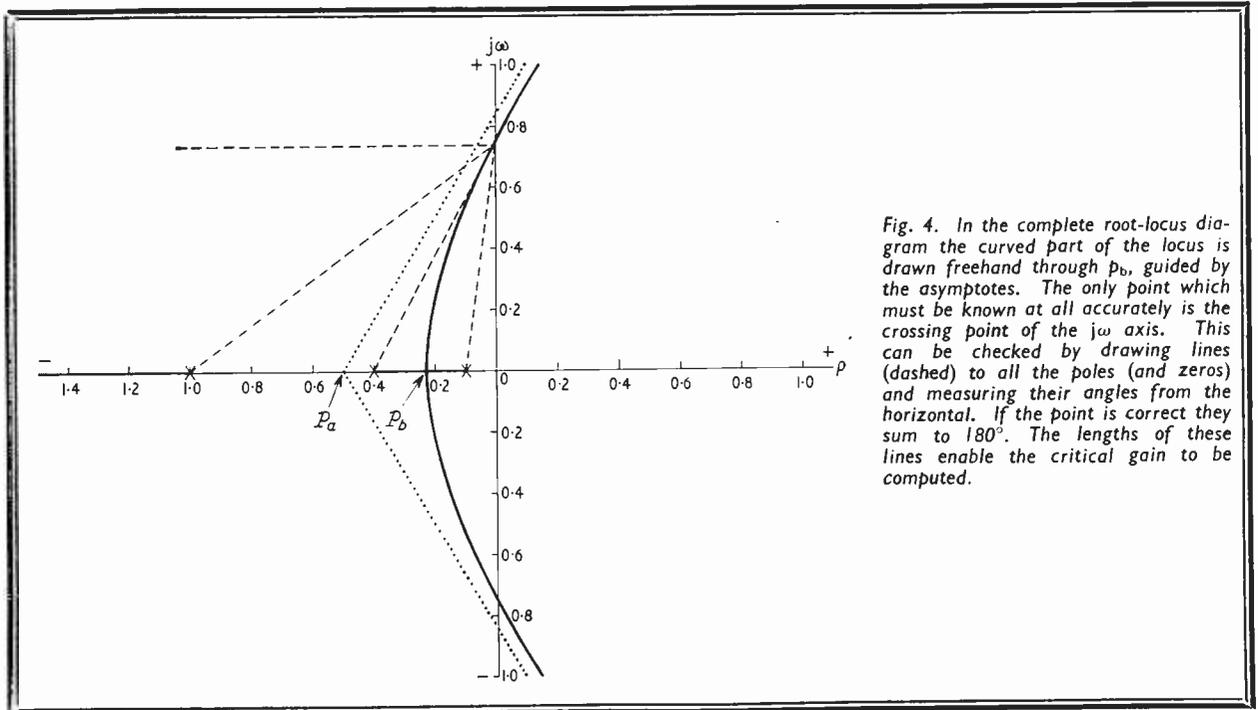
and a horizontal to the left through the point and assign negative signs to angles to zeros and positive to angles to poles. Add all the angles with due regard to sign. If the result is an odd multiple of  $180^\circ$ , the point is on the root-locus.
