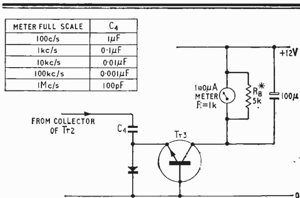
Fig. 7. Frequency meter modification. The value of the 5 kΩ resistor ( $R_B$ ) should be adjusted so that f.s.d. is obtained with 120 µA collector current through Tr3.
