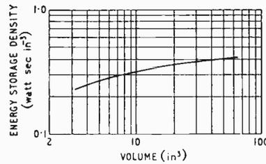
Fig. 3. Energy-storage density (watt sec/in<sup>3</sup>) as a function of volume at 15 V.
