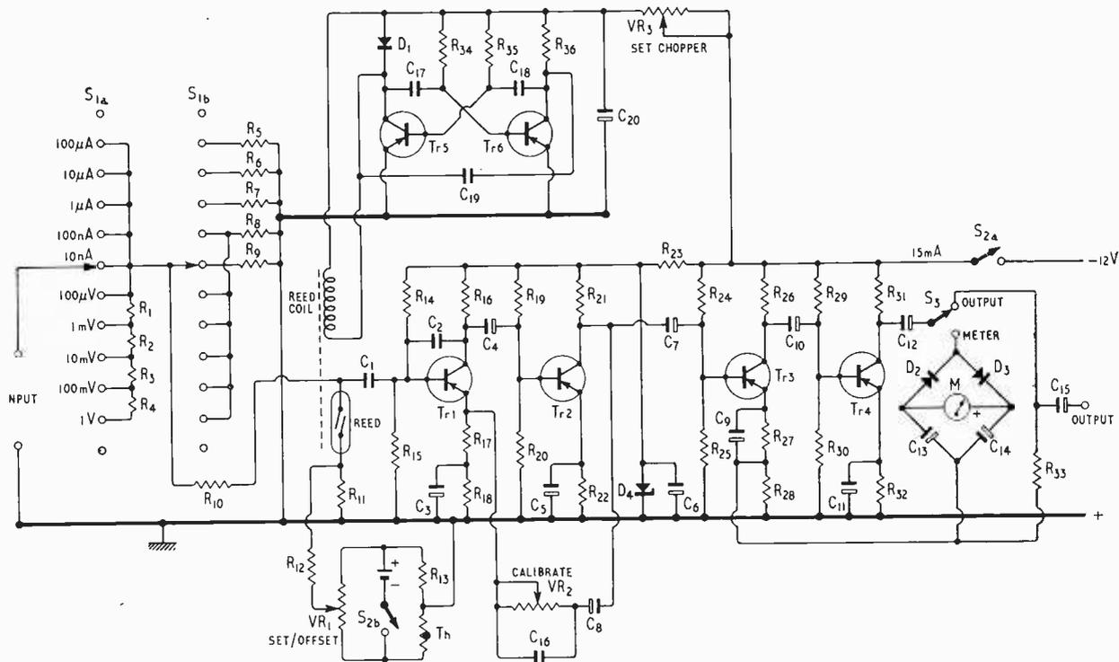
Fig. 4. Complete circuit of d.c. microvoltmeter/nanoammeter.
