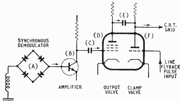
Fig. 6. Basic arrangement for preserving d.c. levels in colour-difference decoder channel.
