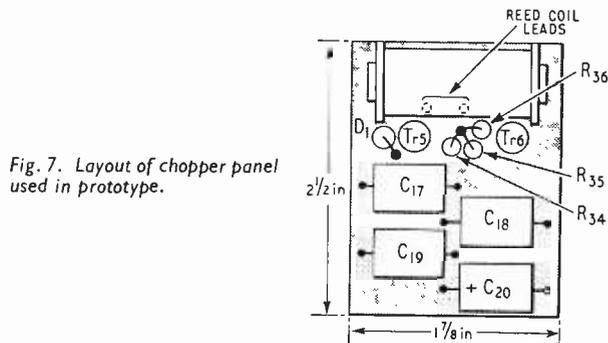
Fig. 7. Layout of chopper panel used in prototype.
