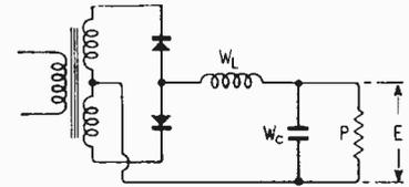
Fig. 4. Simple choke-input power supply with L, C and R in terms of energy storage and power.
