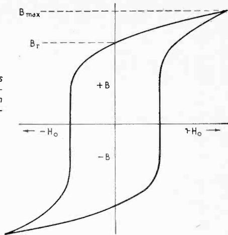
Fig. 3. Hysteresis loop for yttrium-iron-garnet with aluminium substitution.
