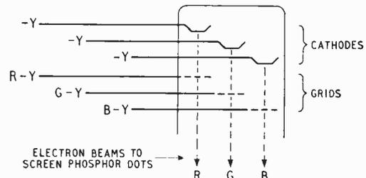
Fig. 2. Arrangement of voltage drives to cathodes and grids of three-gun, shadow-mask colour picture tube to ensure that grid-cathode on each gun sees only appropriate R, G, or B drive voltage on colour transmission and only luminance,  $Y$ , on monochrome transmission.
