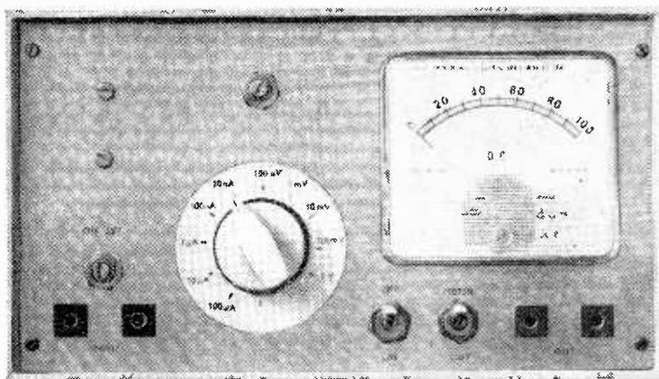
Low-drift chopper-type instrument measuring down to microvolt and nanoamp regions
