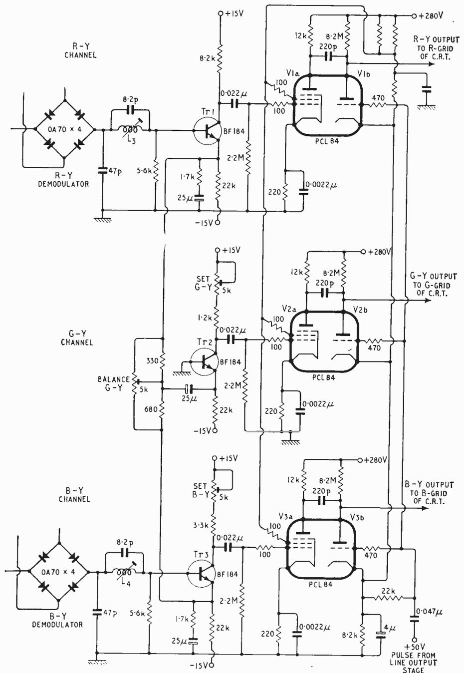
Fig. 8. Complete colour-difference matrix decoder section of commercial receiver (Mullard.)
