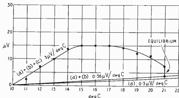
Fig. 3. Effect of substituting a thermistor for  $R_4$  in Fig. 1 and subjecting circuit to a 11 deg C rise ( $R_s = 1 \text{ k}\Omega$ ).
