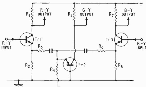
Fig. 5. Basic circuit of three-transistor, emitter-matrixing decoder circuit analogous to Fig. 4(c) valve version.
