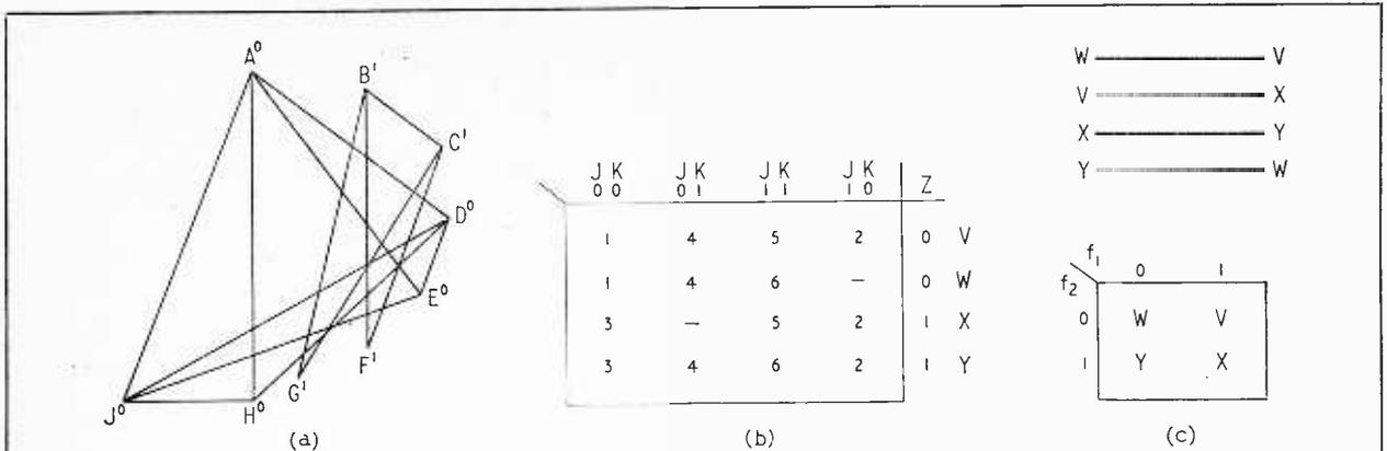
Fig. 13. (a) Merger diagram for Fig. 12, each line connecting two rows which could be merged. (b) Merged flow table. (c) Transitions and transition map.
