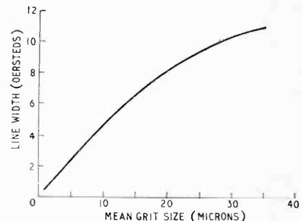
Fig. 5. Line width of a y.i.g. sphere as a function of polishing grit size.
