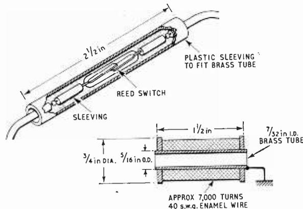
Fig. 6. Detail of reed and actuating solenoid.
