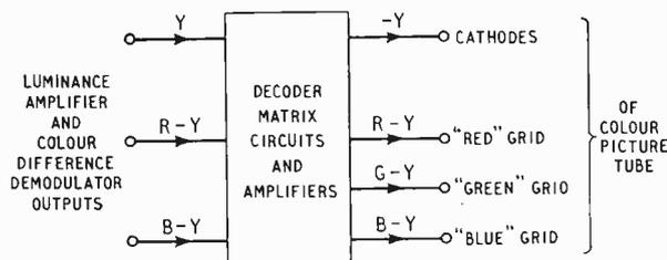
Fig. 3. Function of colour decoder section in converting three video signals  $Y$ ,  $R - Y$  and  $B - Y$  into four corresponding signals,  $Y$ ,  $R - Y$ ,  $G - Y$  and  $B - Y$  needed to drive colour tube.
