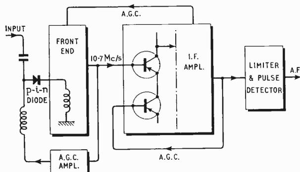
Fig. 3. Wide dynamic range of 120 dB of the Fisher TFM-1000 tuner is achieved by use of three a.g.c. loops, one using a p-i-n diode.
