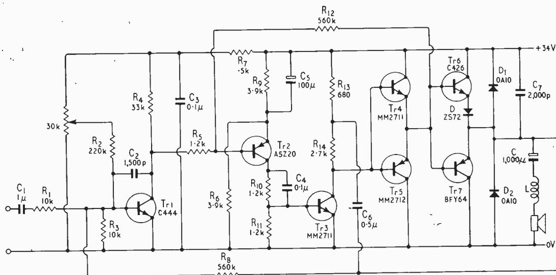
Fig. 12. Circuit of SW class D amplifier using configuration 2.
