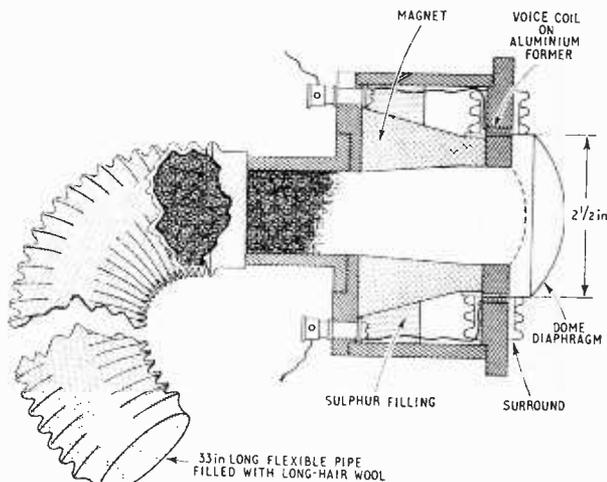
Fig. 1. KEF's new mid-range loudspeaker with absorbent load.
