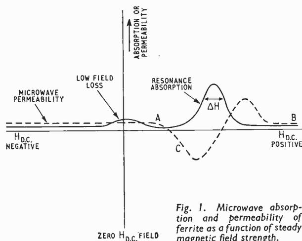
Fig. 1. Microwave absorption and permeability of ferrite as a function of steady magnetic field strength.
