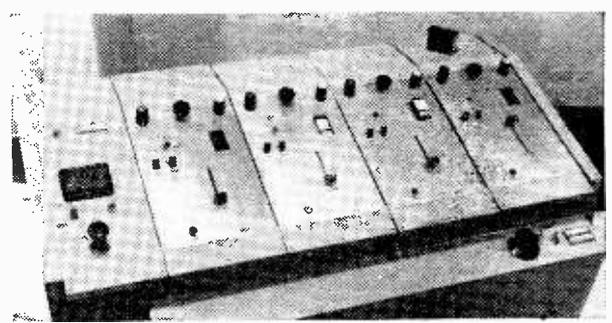
Insertion of sound effects into television and sound programmes is simplified by this "programme effects generator" just introduced by the B.B.C. The effects are recorded in specially developed matchbox-size tape cassettes, each giving 30 seconds playing time. Four reproducing channels are provided. Tape playing speed can be continuously varied, for example to alter the pace of footsteps.
