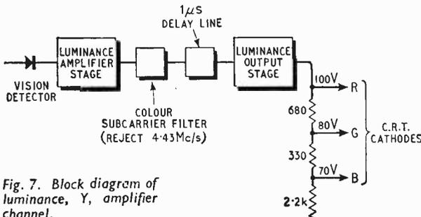
Fig. 7. Block diagram of luminance, Y, amplifier channel.
