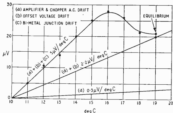
Fig. 2. Temperature characteristic of Fig. 1 circuit when subjected to a sudden rise of 9 deg C ( $R_s = 1 \text{ k}\Omega$ ).
