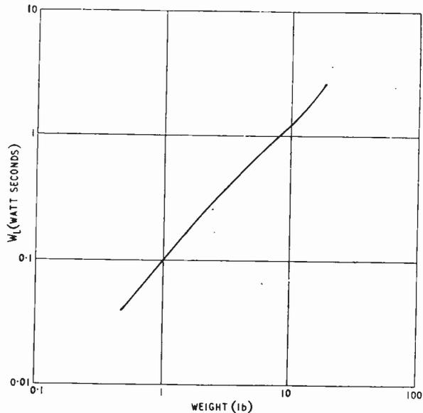
Fig. 5. Energy-storage capacity of an inductor (about 0.1 watt sec/lb)
