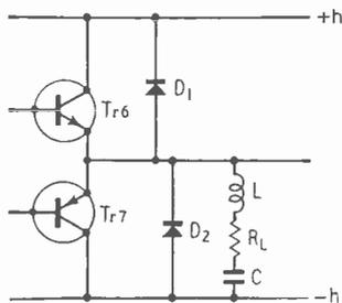
Fig. 9. Output stage configuration 2.
