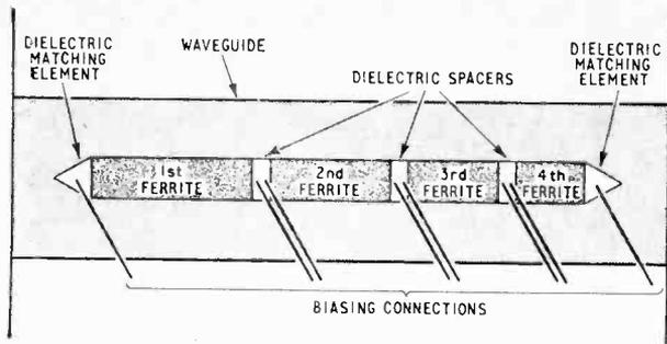
Fig. 2. Four-element latching digital phase shifter.
