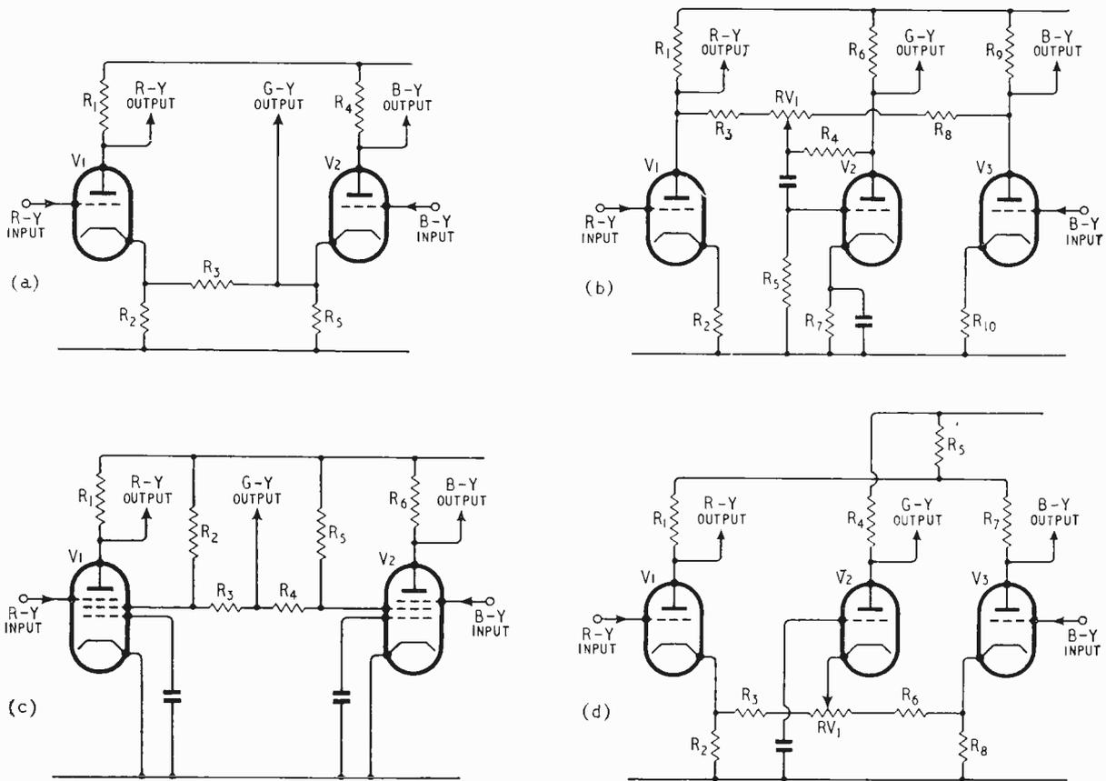
Fig. 4. Colour matrix basic decoder circuits that have been used in American commercial receivers: (a) double-triode, cathode-matrixing; (b) three-triode, anode-matrixing; (c) double-pentode, screen-matrixing; (d) three-triode, cathode-matrixing.
