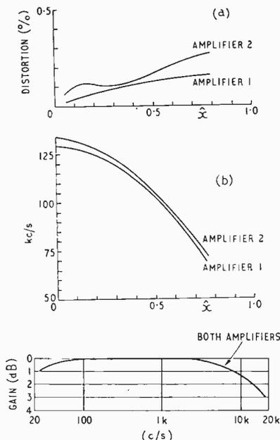
Fig. 14. Harmonic distortion, oscillation frequency and amplitude—frequency response of both amplifiers.
