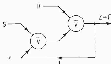
Fig. 6. Implementation of S-R bi-stable with NOR logic elements.
