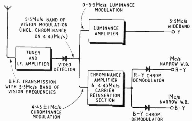
Fig. 1. How receiver accepts and amplifies colour transmission signals with three picture modulations ( $Y$  on main carrier and  $R - Y$ ,  $B - Y$  on colour subcarrier frequency) and extracts the modulations separately to provide signals for ultimately driving colour picture tube.
