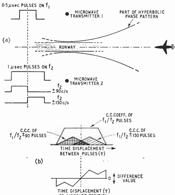
Fig. 1. Principle of R.A.E.'s correlation-protected I.L.S.: (a) localizer transmission; (b) cross-correlation in aircraft receiver.
