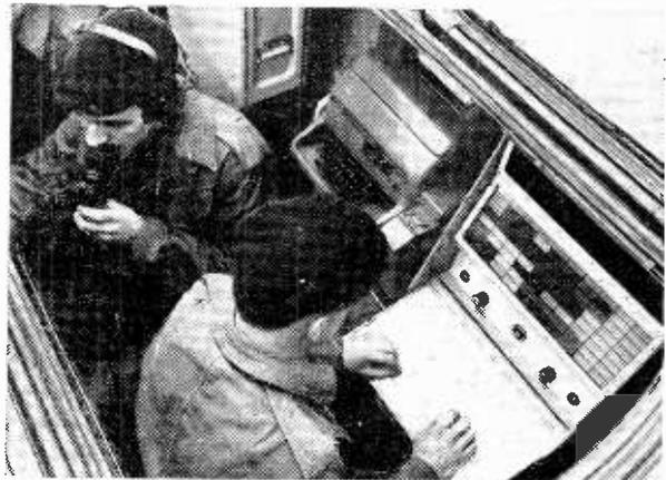
The operator's console for FACE, on the left of which is an automatic typewriter and on the far left part of the Elliott 920B computer.
