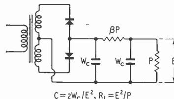
load power is dissipated in the filter resistor. Our first job is to get rid of  $C$ ,  $E$ ,  $R_F$ ,  $R_L$ , and to replace them by combinations of energy storage and power.
