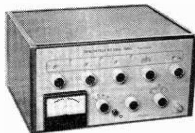
▲ RC oscillator with a frequency range of 1c/s to 1Mc/s shown by Alcatel.
