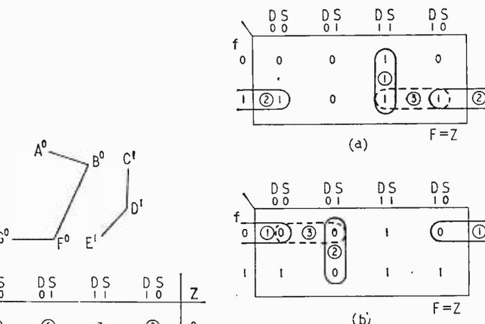
Fig. 10 (a) Excitation map with loops for NAND implementation of Fig. 7. (b) Alternative looping of zeros for implementation with NOR elements.
