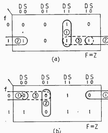
Fig. 10 (a) Excitation map with loops for NAND implementation of Fig. 7. (b) Alternative looping of zeros for implementation with NOR elements.
