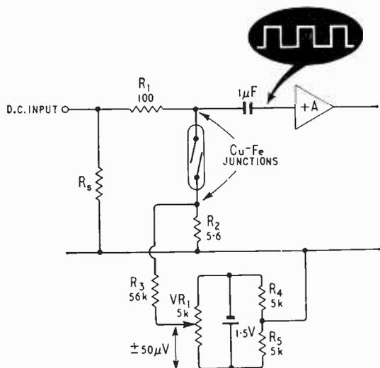
Fig. 1. Chosen method for neutralizing offset voltage.
