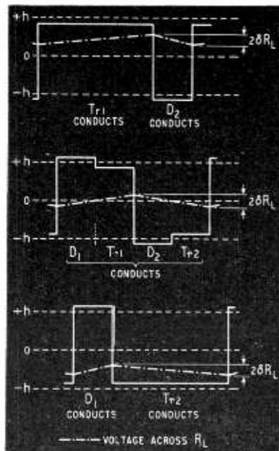
Fig. 10. Illustrating the operation of configuration 2.
