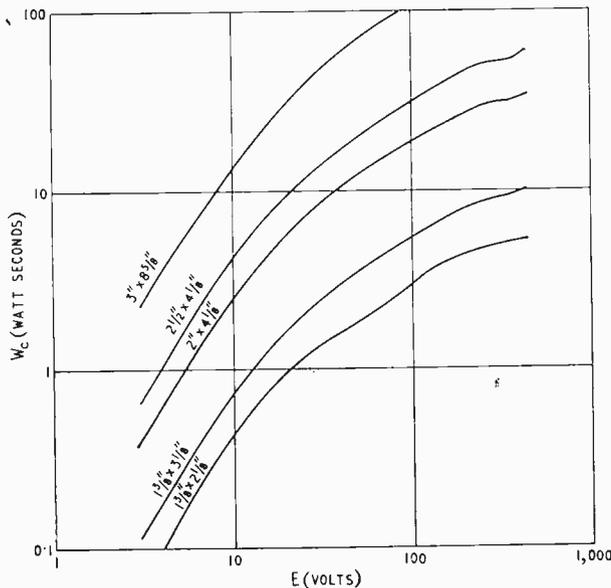
Fig. 2. Energy-storage capacity of currently available aluminium electrolytic capacitors.
