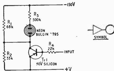
Fig. 12. Neon indicator stage and symbol. (Cost of stage: 4 resistors at 2d each, 1 transistor at 2s 0d and 1 neon at 2s 9d = 5s 5d)
