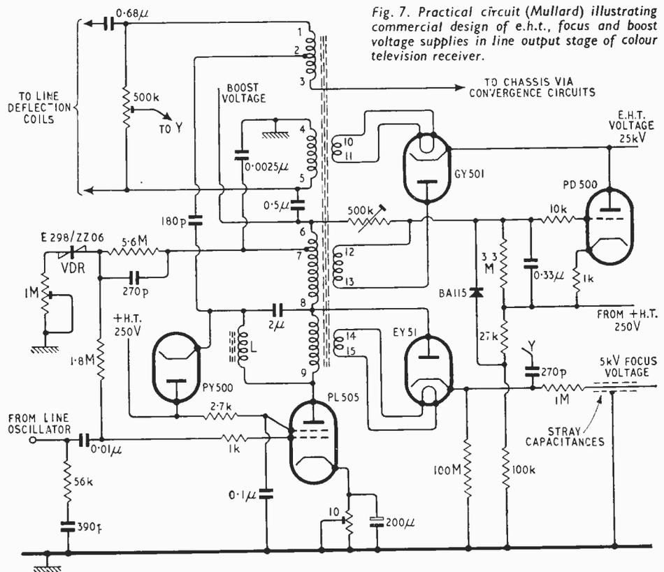
Fig. 7. Practical circuit (Mullard) illustrating commercial design of e.h.t., focus and boost voltage supplies in line output stage of colour television receiver.
