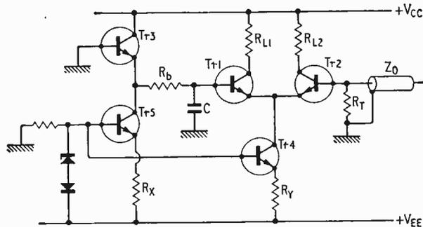
Fig. 7. Current switch for negative input pulses. Capacitor C is a decoupling component.
