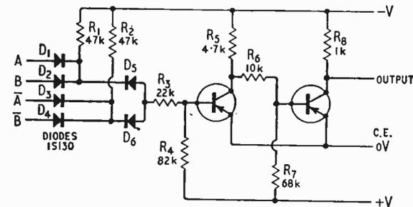
Fig. 9. Comparator circuit. (Cost per comparator: 8 resistors at  $2d$  each, 6 diodes at  $4\frac{1}{2}d$  each, 2 transistors at  $9d$  each =  $5s 1d$ )
