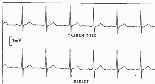
Left: The tracing shows a transmitted electrocardiogram compared with a simultaneous direct recording.
