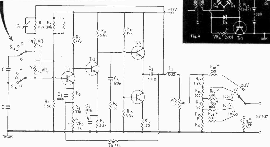
Fig. 3. Complete oscillator circuit with power supply circuit inset (Fig. 4). Note that Ni-Cd battery can be trickle charged by leaving connected to power supply when oscillator is switched off.  $R_6$  should be  $4.3\text{k}\Omega$ .
