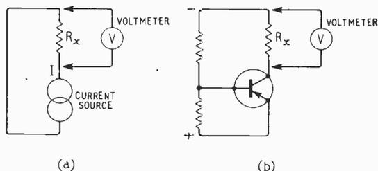
Fig. 1. (a) The measuring technique employed.
