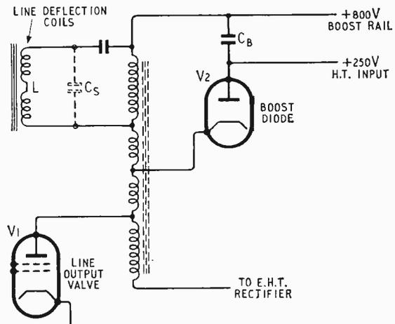
Fig. 4. How 800-V d.c. boost voltage rail is supplied by flyback current pulses through efficiency diode.
