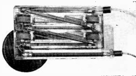
The e.h.t. Cockcroft-Walton voltage tripler is a separate sealed unit which is attached directly to the c.r.t. final anode by a clip connector (in the centre of a black circular insulating cover which can be seen underneath)
