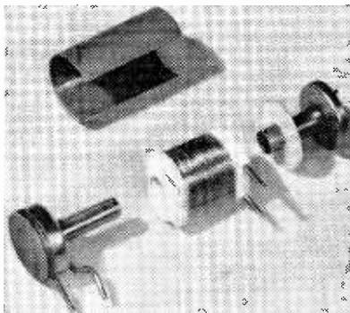
including contact bounce, and release time is of the order of 500  $\mu\text{s}$ . Mating surfaces are gold coated, and typical contact resistance is 30 m $\Omega$ . Operating life when switched 60 V d.c. at half an amp (resistive) is said to be at least one million operations, rising to five million at 60V 100 mA. The 1M can be produced in multiple forms. Overall dimensions are less than 1.5 cu. cm. STC Electro-Mechanical Division, West Road, Harlow, Essex.
