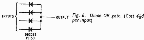
Fig. 6. Diode OR gate. (Cost  $4\frac{1}{2}d$  per input)
