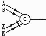
Fig. 8. Comparator symbol that will be used in system diagrams.
