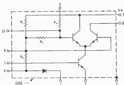
For this kind of operation pins 4, 8 and 10 should be by-passed to earth, the input signal applied to pin 1 ( $<100\Omega$  source resistance), a.g.c. input applied to pin 5, the output taken from pin 6 and pins 2, 3, 7 and 9 earthed.
