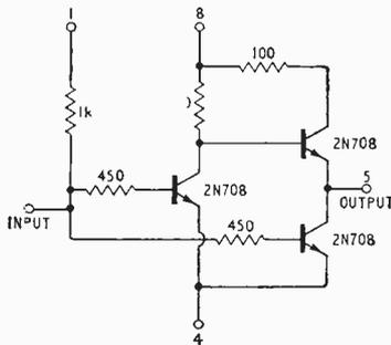
Fig. 1. Circuit of the Fairchild  $\mu$ L900 buffer.
