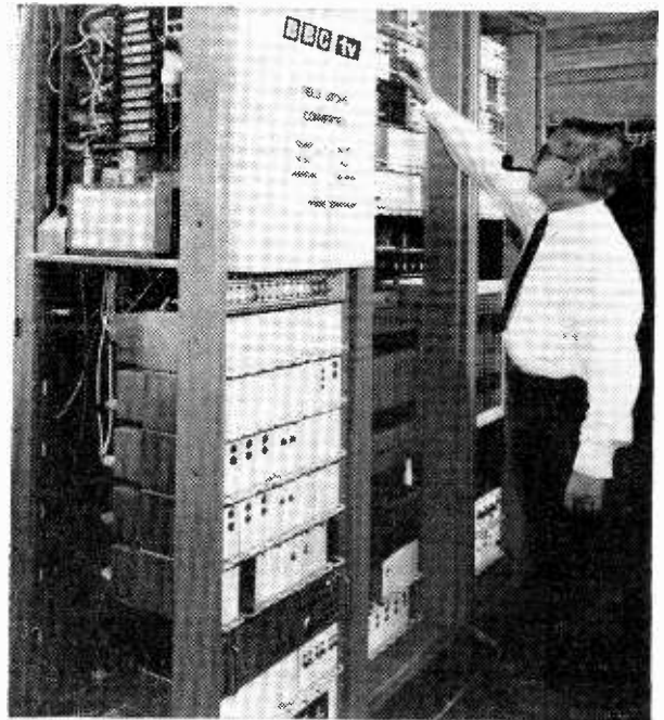
The complete conversion equipment in a B.B.C. laboratory near Broadcasting House, London
