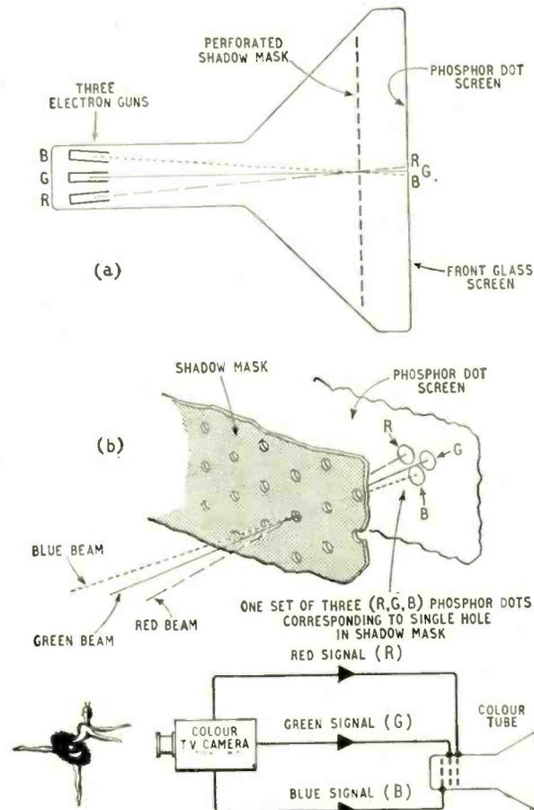
(Below) Fig. 2. Principle of shadow mask c.r.t.: (a) beams converging on mask and diverging on to screen; (b) close-up of mask and screen.
