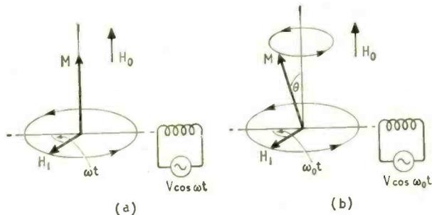
Fig. 2. Interaction of the macroscopic nuclear magnetic moment  $M$  with a steady magnetic field  $H_0$  and a rotating magnetic field  $H_1$ . (a) When the frequency of rotation  $\omega$  is different from the Larmor frequency  $\omega_0$ ,  $M$  remains aligned along  $H_0$  and is unaffected by  $H_1$ . (b) When  $H_1$  rotates at  $\omega_0$ ,  $M$  experiences a force which pulls it away from the  $H_0$  direction, about which it precesses.
