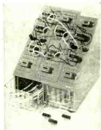
connections can be changed quickly to investigate a new design or evaluate an alternative supplier's product. The unit is ideal for prototype educational and feasibility studies. A logic handbook is provided for i.c. interconnection leads, and an i.c. extractor tool. The breadboard is  $6\frac{1}{2} \times 6\frac{1}{2}$  in and weighs 1 $\frac{1}{2}$  lb. Spectrum Electronics Ltd., Deneway House, Potters Bar, Herts.
