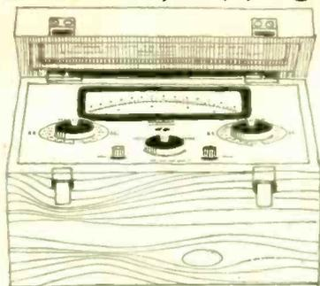
**a** PRECISION AVOMETER Measures d.c. voltage (1.5-1500V scales,  $\pm 0.3\%$  f.s.d.), d.c. current (1.5mA-15A scales,  $\pm 0.5\%$  f.s.d.), a.c. voltage (3V-1500V scales,  $\pm 0.75\%$  f.s.d.), a.c. current (3mA-15A,  $\pm 0.75\%$  f.s.d.). \*meets B.S.S. 89/1954 for precision-grade instruments.
