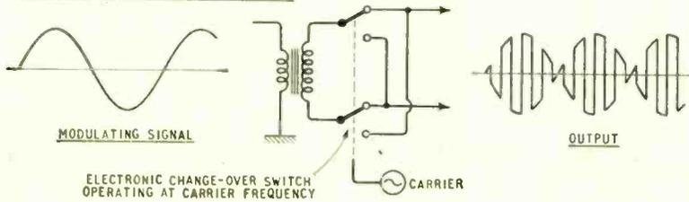
**NORMAL AMPLITUDE MODULATED SIGNAL**
