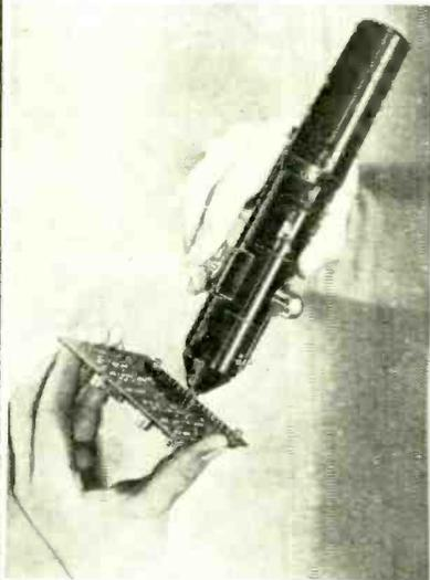
THE DIOTESTOR detects faulty diodes and transistors when still in circuit without need for unsoldering.
