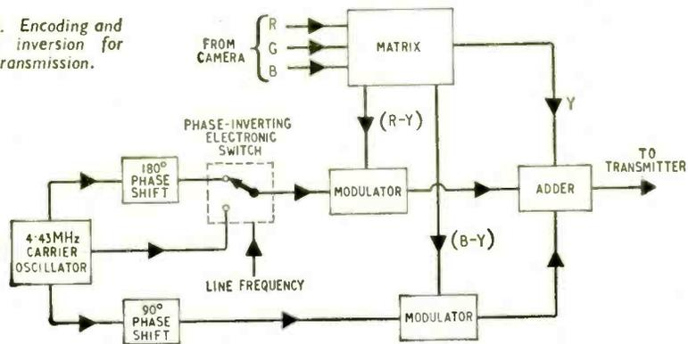
choosing a part of the transmitted waveform where video information is not present—i.e., during the sync pulse and fly-back period, and transmitting a short burst of carrier. A gate in the receiver separates this from the rest of the video wave-form, and feeds it to the local oscillator to synchronize it.
