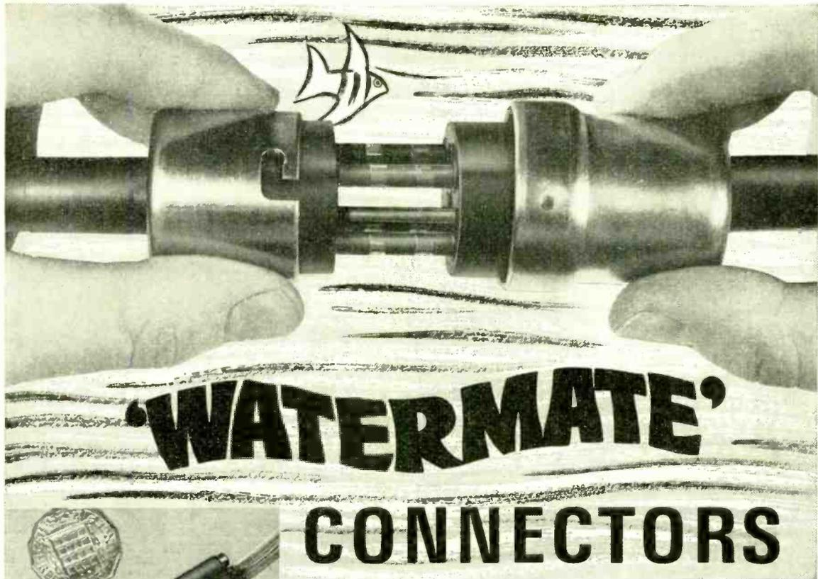
Depicted here are typical examples of a range of Water-proof Connectors of unique design enabling electrical circuits to be connected or disconnected even when under water. The range caters for electrical loads of 440 volts a.c. 175 amps. down to the signal current levels associated with instrumentation and similar arrangements.
