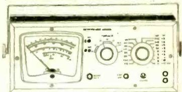
**b** MULTIMETER HI108 Battery-operated, fully-transistorised, measures a.c./d.c. voltage (100mV-1000V scales,  $\pm 4\% \pm 3\%$  f.s.d.), a.c./d.c. current (1 $\mu$ A-3A scales,  $\pm 4\% \pm 3\%$  f.s.d.), resistance (2k $\Omega$ -20M $\Omega$  scales), power (-20 to +60db, 9 scales), r.f. voltage (300mV-10V scales, up to 250MHz with external probe available separately).
