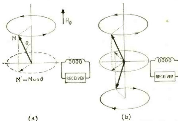
Fig. 3. (a) In the case of n.m.r., the component  $M'$  of  $M$  rotating in a plane perpendicular to the steady field direction induces an alternating voltage in the sample coil. (b) The case of n.q.r. in powdered samples is similar, except that  $H_0$  is not present and  $M$ , which is now the resultant of a large number of macroscopic moments each precessing about a different direction, is accompanied by an equal and opposite moment rotating in the opposite direction.
