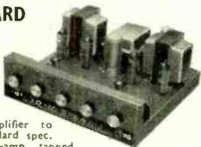
Valve amplifier to exact Mullard spec. With pre-amp, tapped o/p transformer 3 and 15Ω all controls, H.T. and L.T. outlet, mono, stereo and speaker phase switching. Complete with escutcheon, knobs, plugs, etc. Ready built (p. & p. 12/6) £20.0.0
