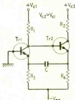
Fig. 3. (left) Basic emitter-coupled, emitter-timed, multi-vibrator.
