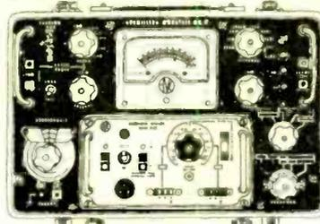
**f** TRANSISTOR ANALYSER MK2 Available in both mains-powered and battery-powered versions; provides accurate measurements in grounded-emitter configuration; accommodates high-power and switching types. Collector voltage: 0.05-12V (up to 150V external). Base current: 1-40mA scales. Collector current: to 1A in 5 ranges. Measures leakage current (from 2 $\mu$ A), hfe (25-250 scales), saturation voltage, turn-over voltage and noise factor.
