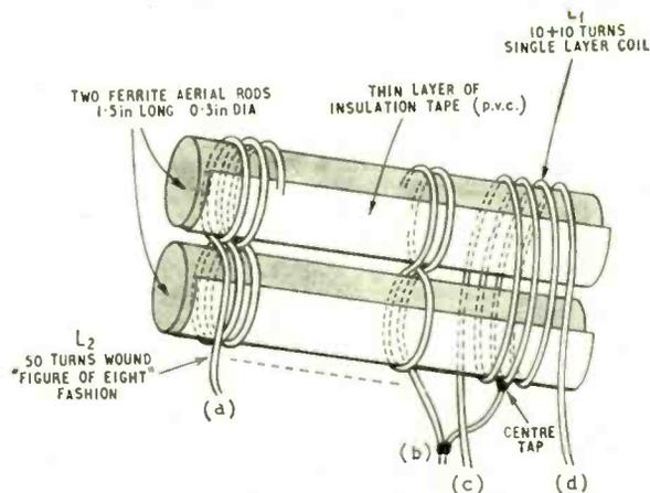
Fig. 5. Showing how to wind the inductors.
