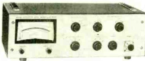
varies from 10 nV ( $\pm 50$  p.p.m.) at a gain setting of  $10^5$  to  $1 \mu\text{V}$  ( $\pm 5$  p.p.m.) at a gain setting of  $10^2$ . Input impedance is greater than  $50 \text{ M}\Omega$  and the output impedance is less than one ohm. Rise times are selectable at nominal settings of 0.05, 0.5, and 5 seconds.
