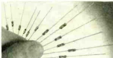
current limited to 50 mA maximum. Standard leads are tinned copper and dual purpose weldable/solderable leads of gold flashed dumet are available.
