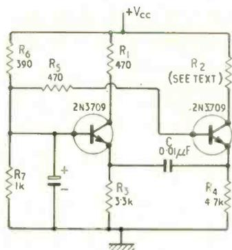
emitter of Tr1 to run down for a period  $t_2$ . Then Tr1 comes into conduction again and the cycle repeats.
