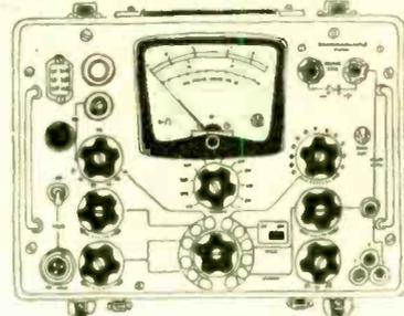
**e** TRANSISTOR & DIODE TESTER TT537 Measures both transistor and diode characteristics. Collector voltage: continuously variable 0-12V, stabilised. Collector current: 1 $\mu$ A-1A. Base current: 0.1 $\mu$ A-50mA. Measures hfe (50-1500 scales,  $\pm 3\%$ ), leakage current (50nA-1.5A scales), diode forward voltage drop (1.5-5V scales, 0-500mA forward current) and breakdown voltage (100-1000V scales, 3mA & 200 $\mu$ A currents limited on short circuit to 13mA & 1.3mA).
