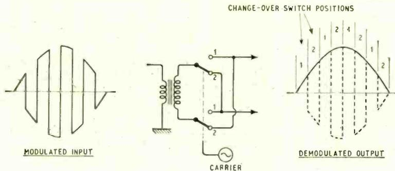
Fig. 6. Suppressed carrier demodulation in the receiver.
