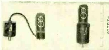
(ZM 1040) giving a 30 mm digit height; the power requirements are +6 V at 50 mA and +240 V at 5 mA. The input pulse requirements are amplitude +1.5 to 4 V, duration 150 ns minimum and the rise time must not exceed 1  $\mu$ s/V. The devices will operate in the temperature range 0-60°C. Darang Electronics Ltd., Restmor Way, Hackbridge Road, Hackbridge, Surrey.
