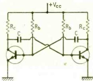
Fig. 1. (left) A conventional collector-base coupled astable multivibrator.
