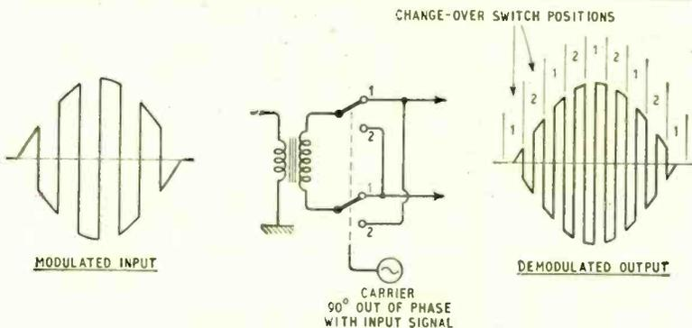
Fig. 7. Demodulator oscillator 90° out of phase.
