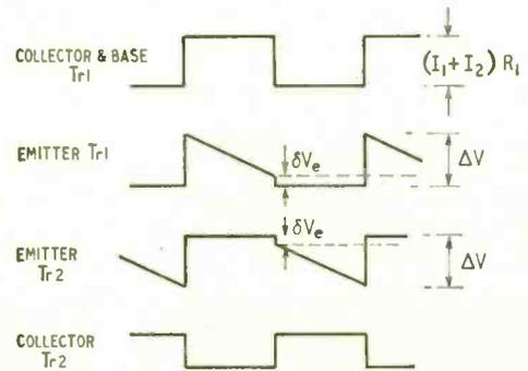
Fig. 4. Waveforms of an emitter-timed multivibrator.
