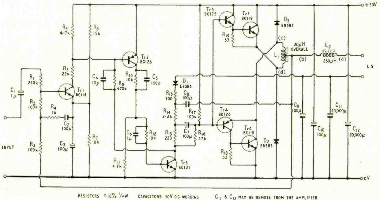
Fig. 4. The circuit diagram of the amplifier.
