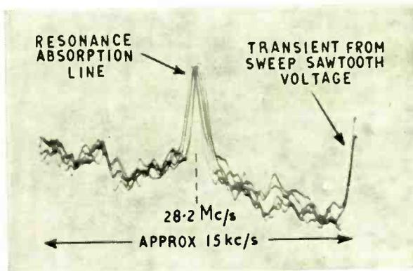
Fig. 6. Photographically recorded c.r.o. trace showing the <sup>35</sup>Cl n.q.r. line in potassium chlorate at room temperature, obtained with a circuit similar to that of Fig. 4. The position of the centre of the resonance line was slightly different on each of the five sweeps recorded because of jitter on the sawtooth generator used for the frequency sweep. Slightly higher signal-to-noise ratios can be expected for <sup>35</sup>Cl in para-dichlorobenzene.
