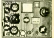
Frequency range 1.5-12 Mc/s. in 3 bands. Employ 7 valves. 2 or 1625 PA, 1625 Buffer, 1625 Mod., 3 x 12 A6 Osc. RT. or C.W. V.F.O. or provision for Xtals, incorporates plate and aerial-current metres. Require ext. P.S.U. Offered in excellent condition. £8/19/6, carr. 15/-.
