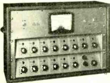
Assemblies, housing up to fourteen channels with combining amplifier etc., can be supplied for either Rack or Console mounting. Power supplies, v.u. meters can be incorporated to meet individual requirements.
