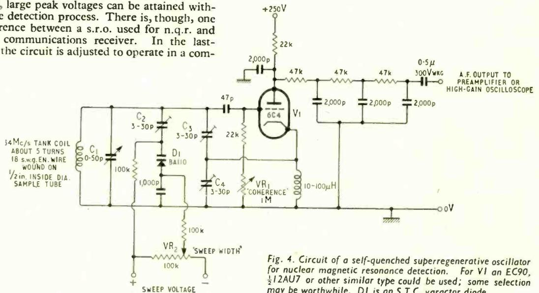
Fig. 4. Circuit of a self-quenched superregenerative oscillator for nuclear magnetic resonance detection. For V1 an EC90, 1/2 12AU7 or other similar type could be used; some selection may be worthwhile. D1 is an S.T.C. varactor diode.
