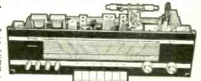
Long, medium and short wave bands coverage, plus VHF FM multiplex. Piano key wave change, separate fly wheel tuning on AM and FM, bass, treble and balance controls, and magic eye tuning indicator. Ferrite Rod aerial. The very latest printed circuitry. Output 6 watts per channel. Complete with multiplex decoder. 5 Valves, line-up: ECC85, ECH801, ECC83, ELL80, EAF801. Full vision tuning scale size: 21 x 6in. Overall dimensions: 21 x 6½ x 8in. Made to very highest standards.
