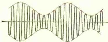
Fig. 5. Suppressed carrier modulation compared with a.m.
