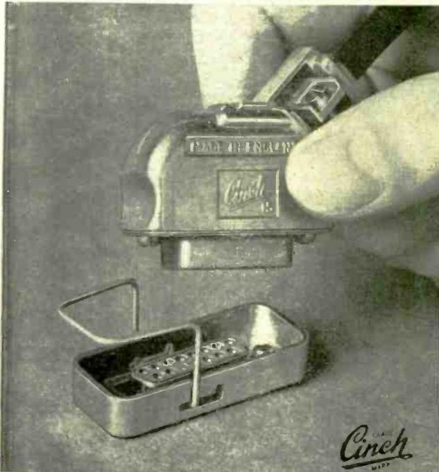
These connectors consist of one-piece Diallyl Phthalate moulding with hard gold plated plug pins, socket contacts, and beryllium copper contact clips. Closed entry contact design eliminates the risk of damage to the sockets by test probes. The shells are of passivated cadmium plated steel and the covers and cable clamps are of die-cast aluminium Grade LM6.
