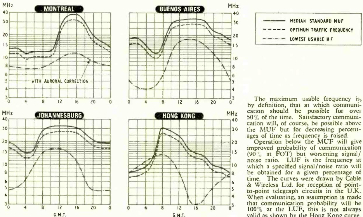
The maximum usable frequency is, by definition, that at which communication should be possible for over 50% of the time. Satisfactory communication will, of course, be possible above the MUF but for decreasing percentages of time as frequency is raised.
