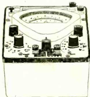
**c** MULTIMETER CT471A Battery-operated, fully-transistorised, sensitivity 100M $\Omega$ /V, measures a.c./d.c. voltage (12mV-1200V scales,  $\pm 3\% \pm 2\%$  f.s.d.), a.c./d.c. current (12 $\mu$ A-1.2A scales,  $\pm 3\% \pm 2\%$  f.s.d.), resistance (12 $\Omega$ -120M $\Omega$  scales,  $\pm 3\%$  m.s.d.), h.f./v.h.f./u.h.f. voltage with multiplier (4V-400V scales up to 50MHz; 40mV-4V up to 1000MHz).
