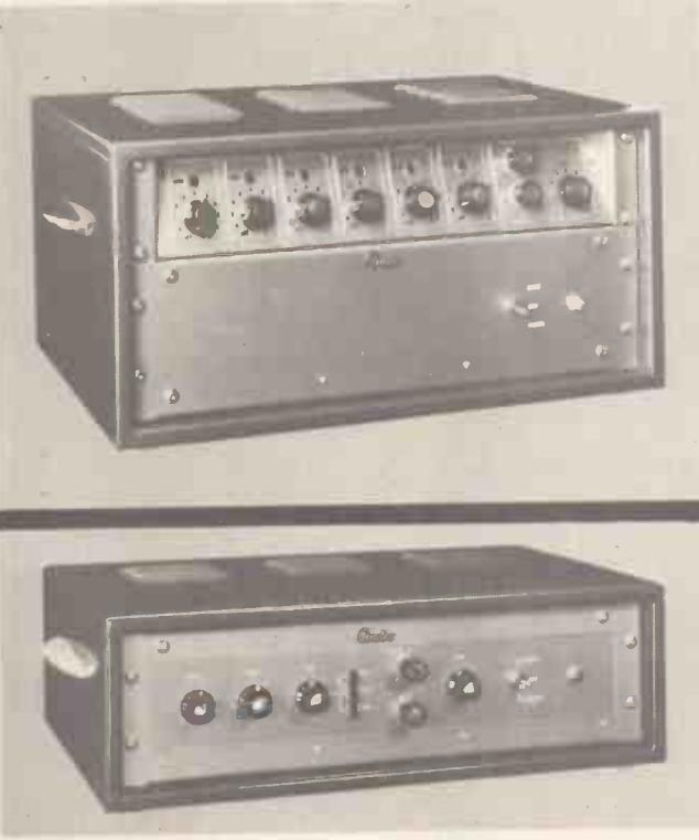
Integrated Mixer/Amplifiers Models A25-30 watts, and A80-60 watts, having inputs for two Microphone Channels balanced at 30 ohm. Auxiliary inputs for Microphone, Gramophone and Tape, each channel independently controlled. Overall Master Gain Control. Treble and Bass tone controls giving ± 12db lift and cut.
