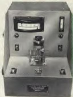
Incorporates many new features, including semi-automatic electrical timing, proportional temperature control, remote controlled specimen lowering system and a temperature meter calibrated to an accuracy of 0.25% full scale deflection at the test temperature.
