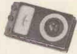
Battery powered Portable Resistance Bridge. Range 0.5 to 50 ohms with multiplier settings of 0.1-100-1000, providing a measuring range of 0.05 to 50,000 ohms. Accuracy in the middle 3 ranges—0.5% approx. PRICE ..... £15 15
