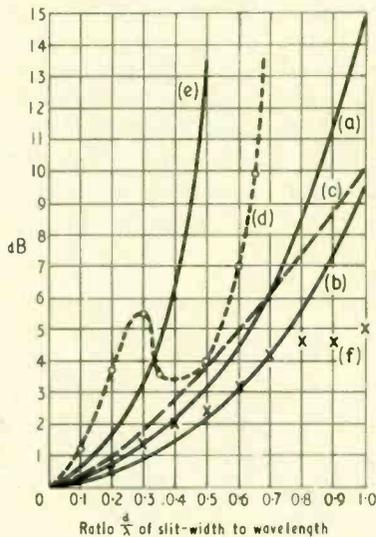
Fig. 16 Deviation of 60° characteristics from axial characteristics for differing types of source: (a) line source (calculated); (b) piston source in infinite plane (calculated); (c) piston source at end of pipe (calculated); (d) measured values obtained with slit on low-frequency unit; (e) sound pressure concentrated at edges of slit (calculated); (f) measured values taking  $d$  as front of cabinet.
