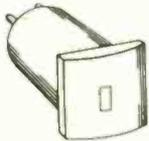
Size is  $\frac{7}{16}$  in. square at the front with body  $\frac{3}{8}$  in. dia. by  $\frac{5}{8}$  in. long. Curved front  $1\frac{1}{4}$  in. radius. This head is available in a wide range of Record/Playback impedances. Also available as Erase. This novel design possesses many advantages over comparable types — higher output — lower losses—extremely good H.F. response—very low noise pick up—has internal mumetal screen. Round body aids mounting arrangements—easy azimuth alignment.
