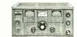
4 band receiver covering 550 Kcs to 30 Mc/s. continuous and electrical band spread on 10, 15, 20, 40 and 80 metres. 8 valve plus 7 diode circuit. 4.8 ohm output and phone jack. SSB-CW. ● ANL ● Variable IF ● 8 meter. ● Step band spread dial ● IF 455 Kcs ● audio output 1.5 W. ● Variable RF and AF gain controls. 115 250 v. A.C. Mains. Beautifully designed. Size: 7.15 x 10in. With instruction manual and service data. £37 10/0. Carriage 12/6.
