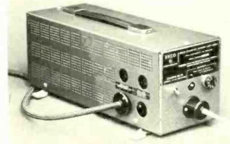
manual selection of the charge rate. Type E239 operates from a 24-V battery and has a power output of 200 W. Current drawn from the batteries is switched by power transistors and fed to the mains output at any load up to full rating. The inverter circuit is protected against damage if the output is short-circuited.
