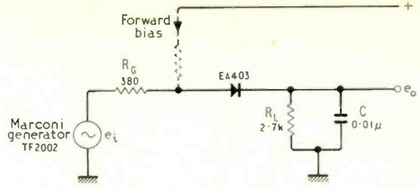
Fig. 2. Conventional diode envelope detector.
