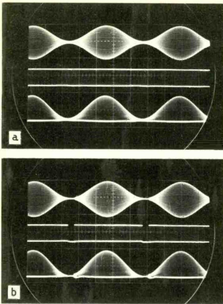
Fig. 7. Waveforms associated with a system such as Fig. 6, using a Schmitt trigger: (a) modulation depth 90%; (b) modulation depth 100%. In each picture the top waveform is the input carrier, the middle one the Schmitt waveform and the bottom waveform the demodulated output.
