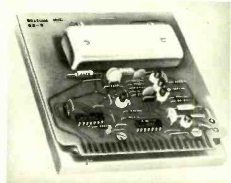
continuously. An address counter is not required for sequential write-in and readout of data, making the module suitable for c.r.t. display and offer memory applications. The memory has a maximum storage of capacity of 10,000 bits at a delay of 10 ms and a clock rate of 1 MHz.
