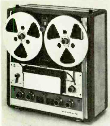
One of the new Series 7 Ferrograph tape recorders. F.E.T. input stages are employed in the all-transistor amplifier. Separate motors are provided for each of three speeds.
