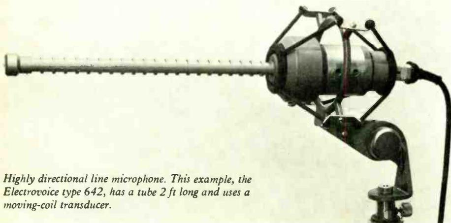
Highly directional line microphone. This example, the Electrovoice type 642, has a tube 2 ft long and uses a moving-coil transducer.
