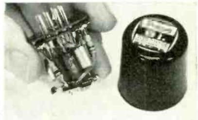
**BI** (Bistable) module shows B9A base for ease of connection. Pins 7, 8, 9 are always power connections.
