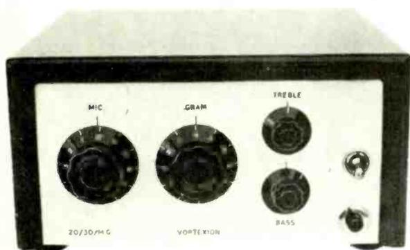
**20 30 WATT MIXER AMPLIFIER.** High fidelity all silicon model with F.E.T. input stages to reduce intermodulation distortion to a fraction of normal transistor input circuits. The response is level 20 to 20,000 cps within 2db and over 30 times damping factor. At 20 watts output there is less than 0.2% intermodulation even over the microphone stage at full gain with the treble and bass controls set level. Standard model 1-low mic. balanced input and HiZ gram. Price £35 0 0.
