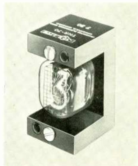
nd +1.5 V to +4 V for an 0; the neon indicator requires a power supply of +180 V d.c.  $\pm 10$  V t 2 to 3 mA. Small quantity price is in the region of £11 per unit.
