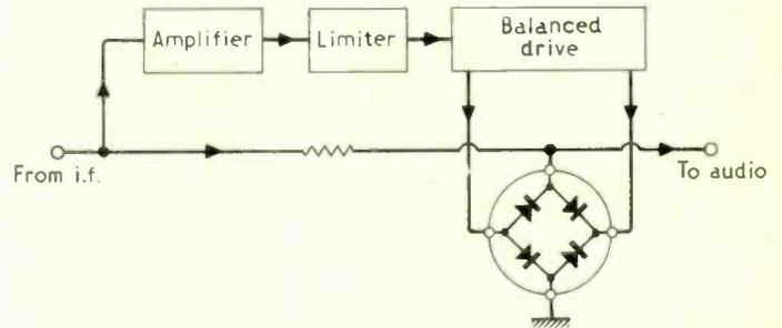
Fig. 6. Zero-crossing detection system.
