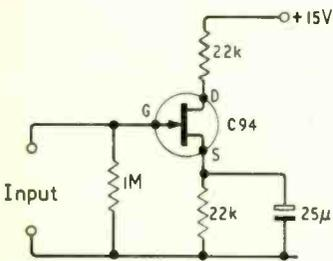
Fig. 1. The basic f.e.t. amplifier. All resistors of 10% tolerance.
