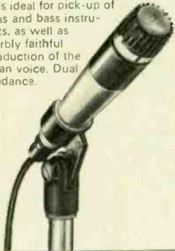
Model **585 SAV** Unisphere A. A high impedance unidirectional dynamic microphone with built-in filter to protect against 'pop' and wind noise. Suppression of boom and feedback, combined with a smooth pure sound, makes this the ideal microphone for use with orchestras, small combos, groups and vocalists. A built-in volume control on the microphone enables user to change the loudness of the P.A. system at the microphone location.
