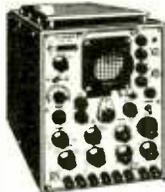
An extremely high quality oscilloscope originally costing £400. Switched beam. Identical Y1, Y2 Amplifiers D.C. to 9 Mc/s. Sensitivity 5mV/cm. Time 10 to 100 V/cm. Time base 10u/sec. to 10 Mc/s. Calibrator. X amplifier D.C. to 2.5 Mc/s. Z Modulation. 110/200/250 v. A.C. Supplied in good working order. £65. carriage £2. or available as received from Ministry untested £50. carriage £2. (Handbook £2 extra).
