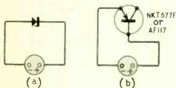
Fig. 2 Reverse-biased "breakdown" diode meter shunt protection.—(a) low-voltage Zener diode; and (b) emitter-base diode of diffused transistor.
