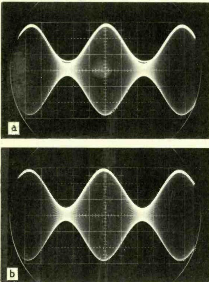
Fig. 4. Observed waveforms: (a) response of Fig. 2 circuit; (b) response of Fig. 3 circuit. In each case the 1kHz detected envelope is superimposed on the 470kHz, 80% modulated input carrier, adjusted so that waveforms have equal amplitude. The carrier level was 1 volt peak-to-peak.
