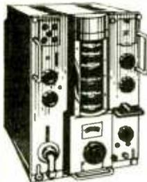
Just released by the Ministry. High quality 10 valve receiver manufactured by Murphy. Coverage in 2 bands 650 Kcs-30 Mc/s. I.F. 300 Kcs. Incorporates 2 R.F. and 3 I.F. stages, bandpass filter, noise limiter, crystal controlled B.F.O. calibrator, I.F. output, etc. Built-in speaker, output for phones. Operation 150/230 volt A.C. Size 19 1/2" x 12 1/2" x 16in.
