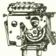
Numerous applications. Electro-magnet and brass tooth wheel. A switch wiper and contacts are employed to this and arranged to be set on for 10 pulses and off for 45. An auxiliary contact is normally on but off 1 in every 25.
