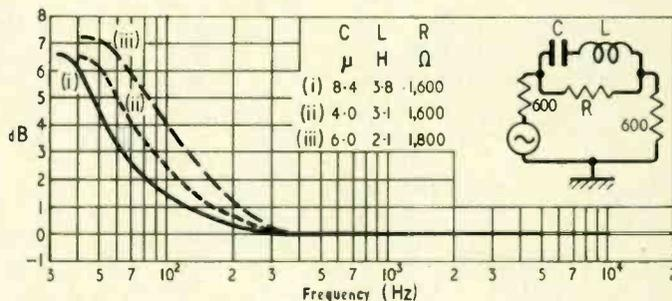
Fig. 13. Response/frequency characteristics of bass-lift circuits.
