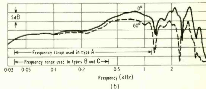
Fig. 15. (a) Response/frequency characteristic of unequalized low-frequency unit without slit at 0° and 60° to the axis. (b) Response/frequency characteristic of unequalized low-frequency unit with 100 mm slit at 0° and 60° to the axis.
