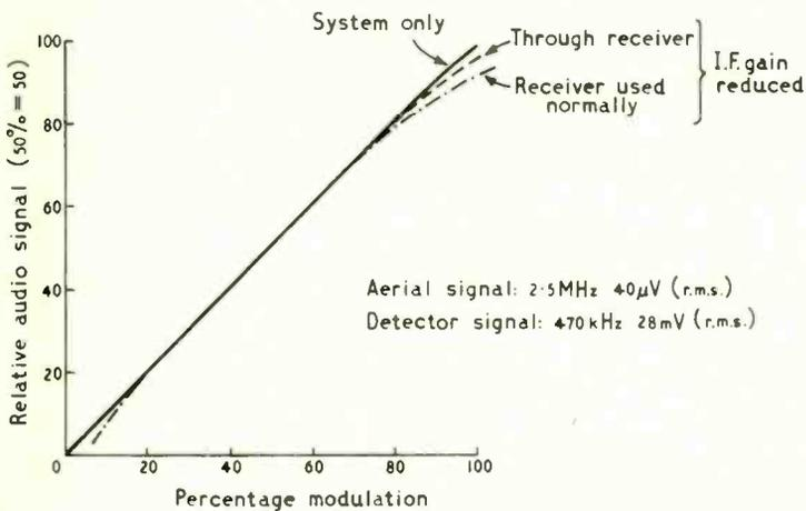
Fig. 10. Modulation depth curves.
