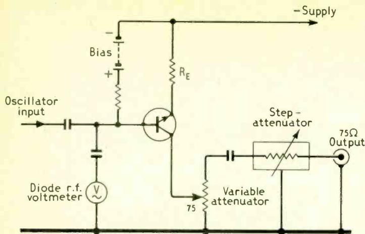
Fig. 2. Oscillator output amplifier and attenuator arrangement.
