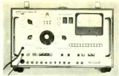
error. These are totalized and the stored count displayed up to a maximum of 2,047 counts. The error counter may be switched to display element counts or 511-bit pseudo random blocks in error. Trend Electronics Ltd, St. John's Works, Tylers Green, Nr. High Wycombe, Bucks.
