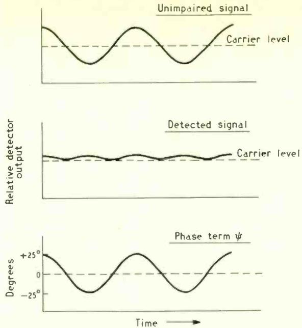
Fig. 5. Calculated waveforms for 50% modulated a.m. signal. (Carrier phase rotated 90° during transmission.)
