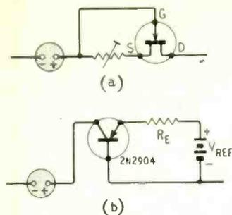
Fig. 4 Multiple series element protection circuits:—(a) f.e.t. with preset  $I_{ds}$ ; and (b) fixed-bias transistor.
