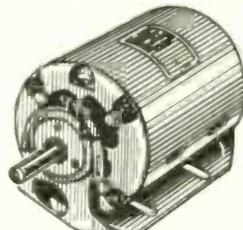
Made by Crompton Parkinson. Single phase 1/4 H.P. motor, 220/230v., 30 cycles, 1.3 amp., 1,425 r.p.m. Continuous rating. Sphd. 1 1/2" dia. Overall dia. less sphd. approx. 3 1/2" dia.
