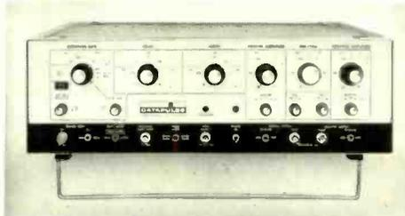
trigger output is supplied for all modes of operation. Pulse delay is variable from 15 ns advance to 50 ms delay, pulse width is variable from 10 ns to 5ms. Repetition rate, delay and width jitter errors are less than 0.05%, while overshoot, undershoot, ringing and top slope aberrations are less than  $\pm 3\%$  at amplitudes of 300 mV and higher. Output stages cannot be damaged by any combination of panel-control settings, open or short circuits or back voltages of up to 10 V.
