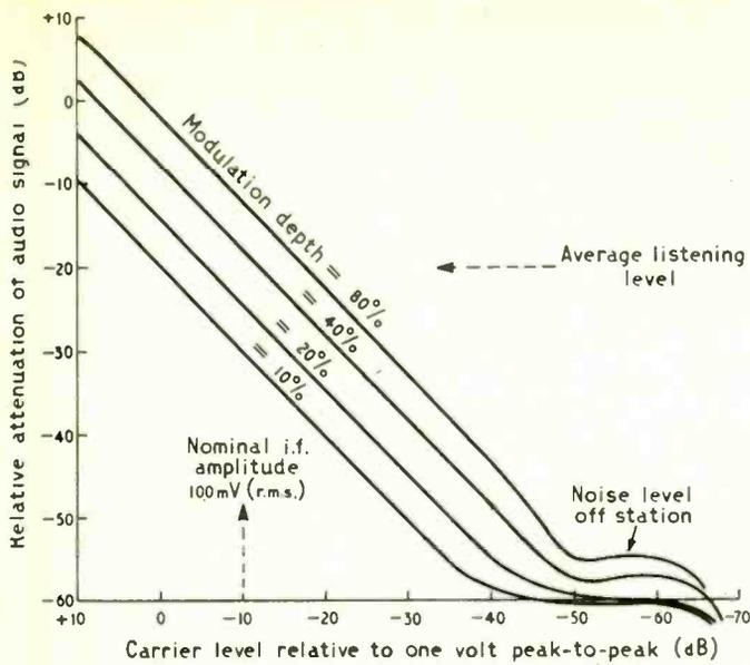
Fig. 9. Dynamic performance of Fig. 8 circuit (i.f. = 470kHz. a.f. = 1kHz).
