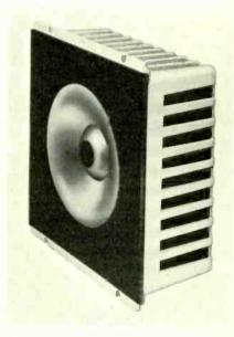
The module (Mk II) used in the Jordan-Watts loudspeakers to be shown by Boosey & Hawkes. The aluminium diaphragm, with plastic surround, is mounted in a 6-in. square frame.
