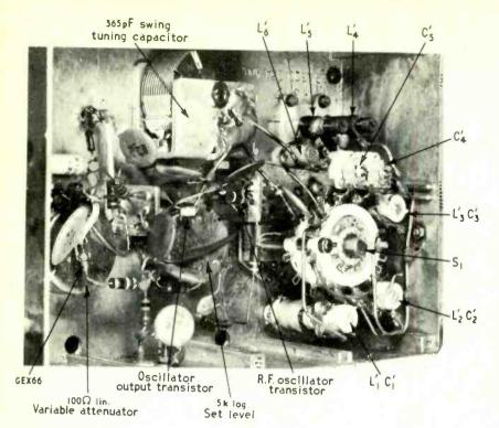
Fig. 6. Internal view of the r.f. oscillator enclosure.
