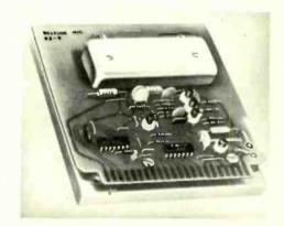
ontinuously. An address counter is not required or sequential write-in and readout of data, making the module suitable for c.r.t. display and uffer memory applications. The memory has a naximum storage of capacity of 10,000 bits at a elay of 10 ms and a clock rate of 1 MHz.
