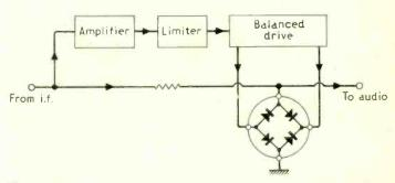
Fig. 6. Zero-crossing detection system.
