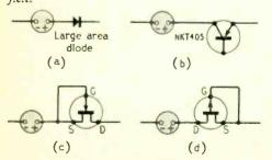
ular BC108 used as a substitute for the diode of Fig. 1(a). In Fig. 1(d) the emitter-base junction is used. These substitutes are useful when you have some reject transistors to hand.
