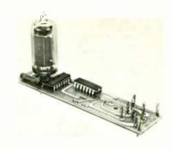
numeral while the decade is still counting. The binary information in n.b.c.d. is brought out to solder-pin connections as are the reset line, hold and sample line and all power supplies (+4 V and +250 V). Units may be cascaded indefinitely. A.S.R. Designs Ltd, 1 Vineyards, Bath, Somerset.
