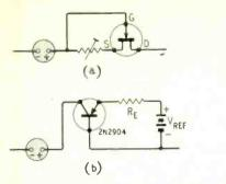
Fig. 4 Multiple series element protection circuits:—(a) f.e.t. with preset I<sub>DS</sub>; and (b) fixed-bias transistor.
