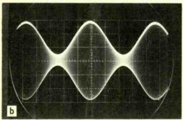
Fig. 4. Observed waveforms: (a) response of Fig. 2 circuit; (b) response of Fig. 3 circuit. In each case the 1kHz detected envelope is superimposed on the 470kHź, 80% modulated input carrier, adjusted so that waveforms have equal amplitude. The carrier level was 1 volt peak-to-peak.
