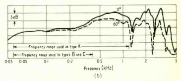
Fig. 15. (a) Response/frequency characteristic of unequalized low-frequency unit without slit at 0° and 60° to the axis. (b) Response/frequency characteristic of unequalized low-frequency unit with 100 mm slit at 0° and 60° to the axis.
