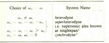
The homodyne does not have a separate oscillator and is described below. Autodyne refers to a self-oscillating mixer and so does not constitute a complete receiver system.
