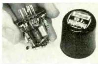
£20/19/6 (normally BI (Bistable) module shows B9A base for ease of connection. Pins 7, 8, 9 are always power connections.
