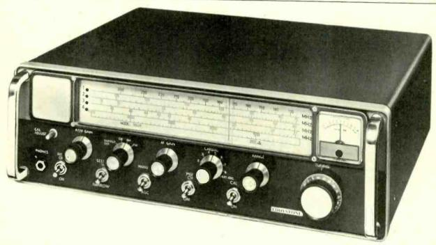
The '990R' when used in conjunction with the matching '990S' provides continuous AM/FM coverage from 27 to 870MHz. A common Panoramic Display Unit is available for use with hoth receivers.
