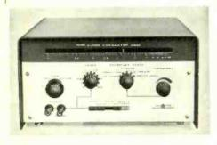
outputs at up to 2.5 V r.m.s.—the square-wave rise time is typically 50 ns. The output level is selected by a four-position push-button attenuator and a variable control, the output frequency being read on a horizontal "easy-to-read" scale. Two internal PP9 batteries provide the power and these can be checked by means of a front-panel push button. If mains operation is required a battery eliminator is available for £7 10s.
