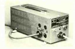
manual selection of the charge rate. Type E239 operates from a 24-V battery and has a power output of 200 W. Current drawn from the batteries is switched by power transistors and fed to the mains output at any load up to full rating. The inverter circuit is protected against damage if the output is short-circuited.
