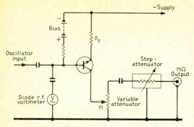
Fig. 2. Oscillator output amplifier and attenuator arrangement.
