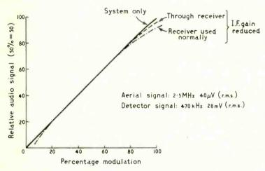
Fig. 10. Modulation depth curves.
