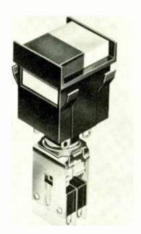
suitable for horizontal or vertical matrix mounting requiring individual rectangular holes 1.00 in. by 1.14 in. for single units and additional 1.250 in. per switch for matrix mounting. One- to four-pole momentary or maintained snap-on switch modules are available as standard, each pole being s.p.d.t. or two circuit. The basic two-circuit microswitches are rated at 10 A., 125/250 V a.c., 30 V d.c.
