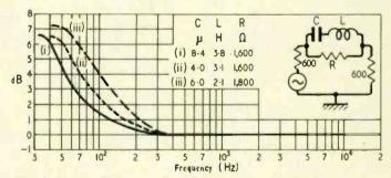
Fig. 13. Response/frequency characteristics of bass-lift circuits.
