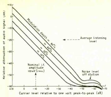
Fig. 9. Dynamic performance of Fig. 8 circuit (i.f. = 470kHz, a.f. = 1kHz).
