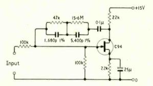
Fig. 4. Alternative equalization circuit using 100 k $\Omega$  gate resistor. All resistors are of 10% tolerance.
