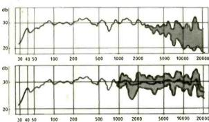
The new Monitor Gold now incorporates a Treble Roll Off Control and Treble Energy Control enabling precise adjustments to be made for room acoustics and programme material.
