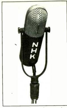
Ribbon microphone incorporating an acoustic labyrinth, type NHK RV1-A, developed by the Japanese broadcasting authority's research laboratories.
