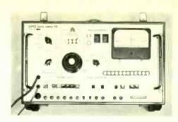
error. These are totalized and the stored count displayed up to a maximum of 2,047 counts. The error counter may be switched to display element counts or 511-bit pseudo random blocks in error. Trend Electronics Ltd, St. John's Works, Tylers Green, Nr. High Wycombe, Bucks.
