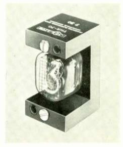
nd + 1.5 V to + 4 V for an 0; the neon indicator equires a power supply of + 180 V d.c. ± 10 V t 2 to 3 mA. Small quantity price is in the region f f.11 per unit.
