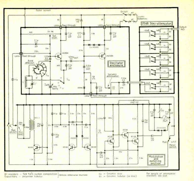
Fig. 5. Overall circuit diagram of the generator. Some reduction in cost may be realized by using the transistors marked with an asterisk in the components comments section.
