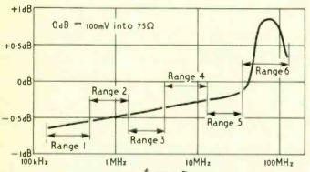
Fig. 3. Graph showing output versus frequency for a constant setting of the r.f. level indicator.
