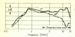
Fig. 20. Response/ frequency characteristics of high flux density 58 mm high-frequency unit at 0° and 60° to the axis.
