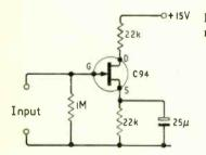
Fig. 1. The basic f.e.t. amplier. All resistors of 10% tolerance.
