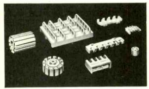
Refractories for high-temperature insulation.
