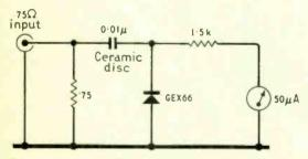
Fig. 4. Circuit used to obtain the graph of Fig. 3.
