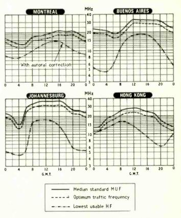
Predictions are based on an ionospheric index (IF2) of 132 and sunspot number 115. April/May is forecast as maximum of the current sunspot cycle. Seasonal changes are evident on the two northern hemisphere routes, MUF
