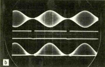
Fig. 7. Waveforms associated with a system such as Fig. 6, using a Schmitt trigger: (a) modulation depth 90%; (b) modulation depth 100%. In each picture the top waveform is the input carrier, the middle one the Schmitt waveform and the bottom waveform the demodulated output.
