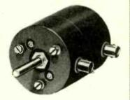
Despite its low cost, this new Hatfield Attenuator will operate efficiently from DC to 100 MHz. The design features individual resistive sections, each selected in turn by a rotary switch mechanism. Careful attention to screening and the elimination of earth loops results in good accuracy being maintained throughout the frequency range.
