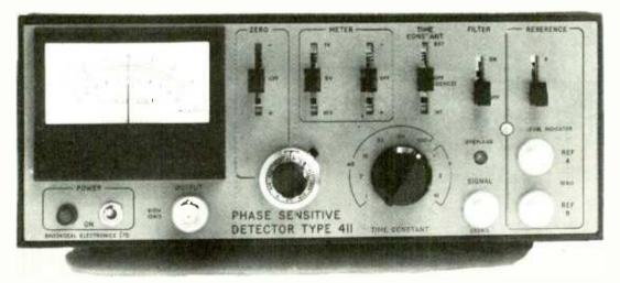
Frequency Range 1.0 Hz to 1.0 MHz Non linearity < 0.05% of f.s.d. Zero Drift < 0.005% of f.s.d. Recovers signals 70dB below noise
