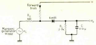
Fig. 2. Conventional diode envelope detector.
