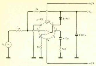
Fig. 3. Amplifier/diode envelope detector.
