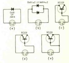
Fig. 1 Forward-biased diode shunt protection of moving-coil meter movements:—(a) single-diode for forward overload; (b) double-diode (for forward or reverse overload); (c) transistor collector-base junction as diode; (d) transistor emitter-base as diode; and (e) transistor with collector and base strapped together.
