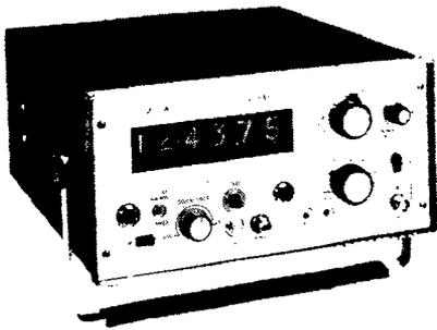
gated counting. Display time is variable from 0.5 to 5 seconds or infinite, and accuracy is  $\pm 1$  count  $\pm$  crystal stability ( $\pm 1 \times 10^{-6}$ ). Venner Electronics Ltd., Kingston By-Pass, New Malden, Surrey.
