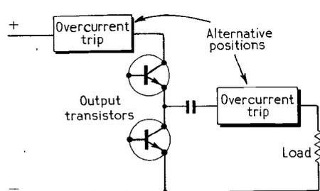
Fig. 1. Normal positions for mean overcurrent protection devices.
