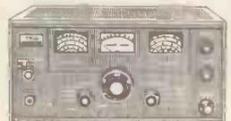
4 band receiver covering 560 Kc/s to 30 Mc/s. continuous and electrical band spread on 10, 15, 20, 40 and 80 metres. 8 valve plus 7 diode circuit. 4/8 ohm output and phone jack. 8SB-CW • ANL • Variable BFO • 8 meter. • Sep. band spread dial • IF 455 Kc/s • audio output 1.5 W. • Variable RF and AF gain controls. 115/250 V. A.C. Mains. Beautifully designed. Size 7 x 15 x 10in. With instruction manual and service data. £37/10/- Carriage 12/6.
