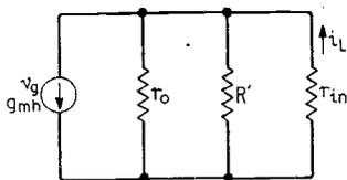
becomes that of Fig. 8, where the voltage source  $v_g$  and the impedance  $z_k$  form the Thévenin equivalent of the cathode follower. Note that  $v_g$  also is the input voltage on the grid of the valve. In the derivation of the mutual conductance  $g_{mh}$  of the combination, the load resistance is regarded as zero, which means that the influence of  $h_{re}$  is omitted.
