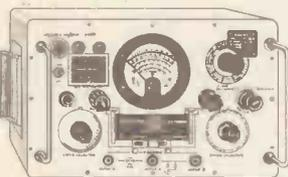
High quality 97 range instrument which measures A.C. and D.C. Voltage, Current, Resistance and Power output. Ranges D.C. volts 250mV-10,000 v. (10 megΩ-110megΩ input). D.C. current 10µA 25 amps. Ohms: 0-1,000 megΩ. A.C. volt 100 mV-250 v. (with R.F. measuring head up to 250 Mc/s). A.C. current 10µA-25 amps. Power output 50 micro-watts-5 watts. Operation 0/110/200/250 v. A.C. Supplied in perfect condition, complete with circuit lead and R.F. probe, £25. Carr. 15/-.
