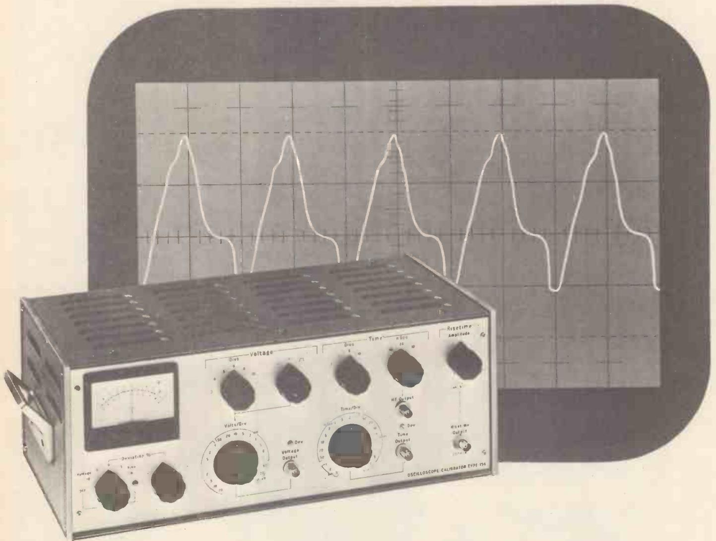
A new instrument, the BRADLEY Oscilloscope Calibrator 156 provides all the facilities required for the calibration of modern precision oscilloscopes. Simple to use, it is designed to calibrate vertical amplitude and sweep speeds, and to check risetime. A unique feature is the direct reading of percentage deviation from true values.
