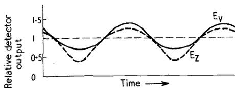
Fig. 1. Relative output for envelope and zero-crossing detector for a 50% modulated a.m. signal when the phase of the upper sideband is advanced by  $90^\circ$  relative to the carrier and the lower sideband.
