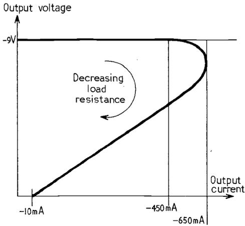
Fig. 7 The current cut-off characteristic of the circuit of Fig. 6.
