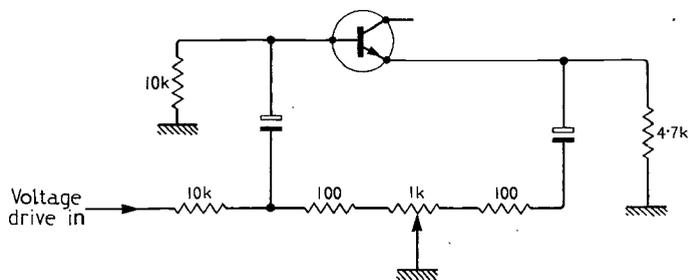
Fig. 3. Schematic diagram of the gain control circuit.
