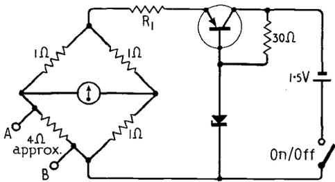
shunt of app. 4Ω was fitted between A & B to obtain a -f.s.d. The voltage and current at A & B are app. 0.2V and 100mA.
