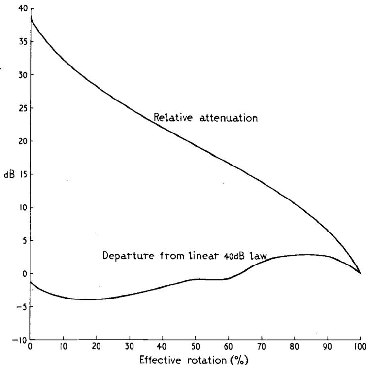
Fig. 4. Curves showing the overall gain/attenuator characteristic.
