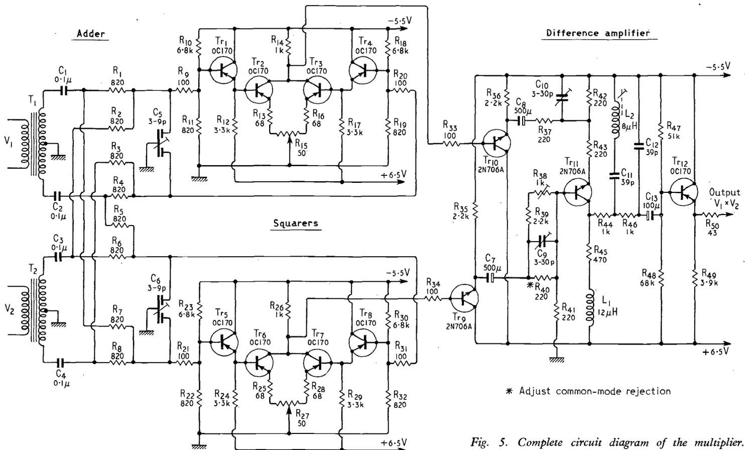
Fig. 5. Complete circuit diagram of the multiplier.
