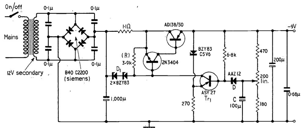
decoupling their interconnection with a capacitor or a Zener diode. The second disadvantage is often overcome with an extra circuit for current limiting or current cut-off.
