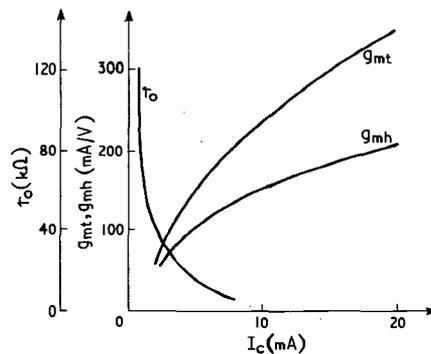
Fig. 3. Showing transistor output impedance  $r_o$  and mutual conductance  $g_{mi}$ , also the mutual conductance of a transistor and valve combination  $g_{mh}$  as functions of collector current.
