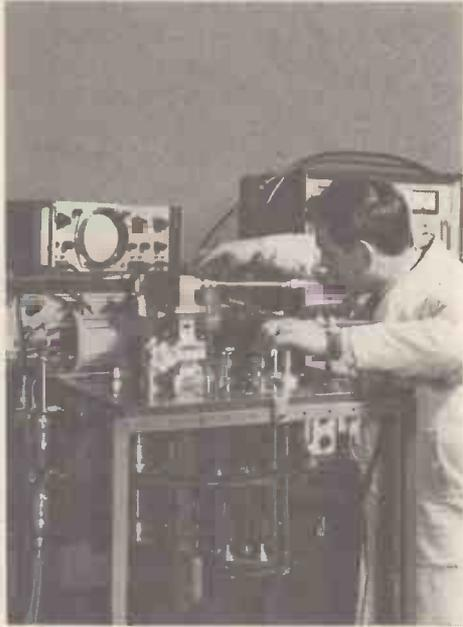
**This month's cover.** A development engineer at Mullard's Mitcham works adjusts a cooled two-stage parametric amplifier designed for use as a low-noise r.f. input stage in communications satellite earth stations. The amplifier operates at 4GHz with a bandwidth of 500MHz, and has a gain of 40dB and an overall noise temperature of 20°K.
