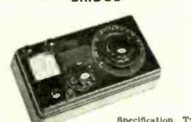
Specification. Type: Moving Coil Galvanometer. Ranges: 1, 0.05 to 5 ohms, 2, 0.5 to 50 ohms, 3, 5 to 500 ohms, 4, 50 to 5,000 ohms, 5, 500 to 50,000 ohms. Scales: Switched. Slidewire: 0.5 to 50. Galvanometer Scale: 10-0-10. Case: Moulded plastic. Internal Source: 4V. Dry battery. Operating Temperature: +10 to +35 deg. C. Operating Humidity: Up to 80% R.H. Dimensions: 200 x 110 x 45mm. Weight: 0.9 kg. List price **£25**. Our price **£9/19/6**.
