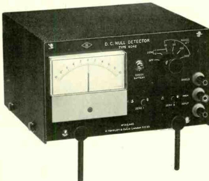
TYPE 6042 uses an F.E.T. Chopper followed by a solid state a.c. amplifier with large open scale output meter.
