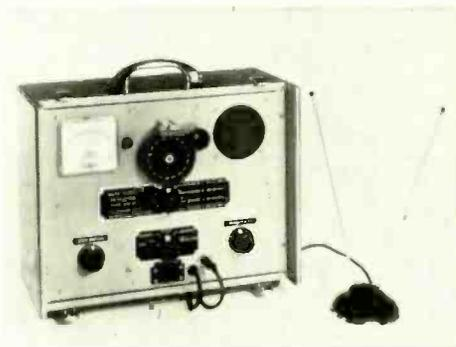
is heard the instrument locks on to the signal which, say the makers, enables the operator to determine if the signal is from a legitimate local transmitter or from a clandestine unit. Having established that the room contains hidden illegal equipment, a probe enables the offending equipment to be located. Leonard Wadsworth & Co. Ltd., Broadway House, Broadway, London S.W.19.
