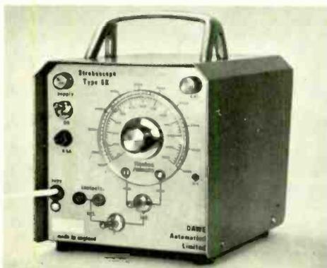
is by means of an internal oscillator or contact closure and accuracy is 2%. A high-intensity flash tube with an output of 10W is incorporated. The instrument measures 165 × 215 × 165mm and weighs 3kg. Price: £45. Dawe Automation Ltd., South Hill Lodge, South Hill Avenue, Harrow, Middx.
