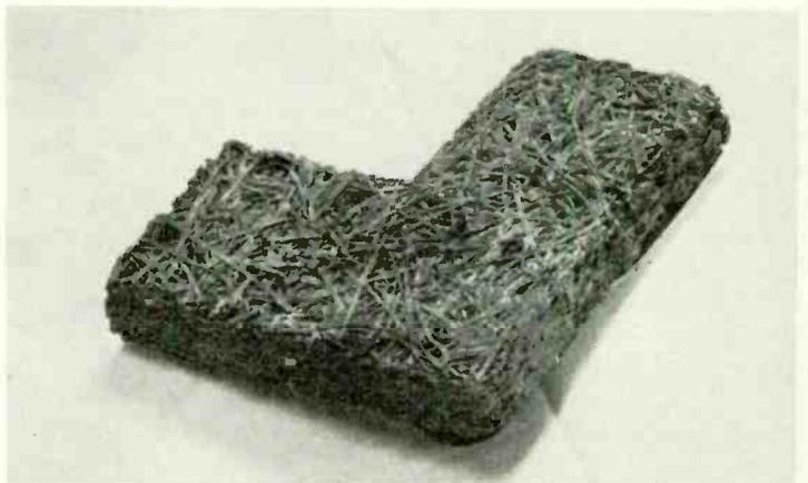
(e) Gypklith. Building slabs of wood/wool material. Provides both thermal and sound insulation. In many sizes and thicknesses. Density 28lb per cubic foot.
