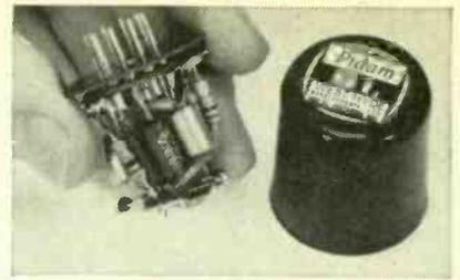
**PIDAM** (Plug-in Digital and Analogue Modules) perform all the usual logic functions, but, unlike other units, can be plugged in, using their B9A bases and can be quickly connected to the required configuration. To help learning, the module covers are easily removable for circuit examination and sets of components are available.
