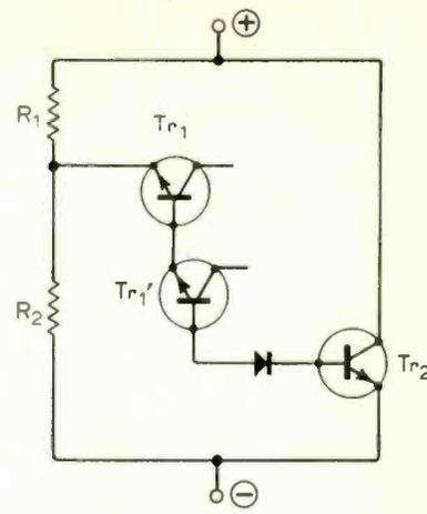
Fig. 4(a and b). Possible alternatives for current boosting without an undue increase in stand-by current.
