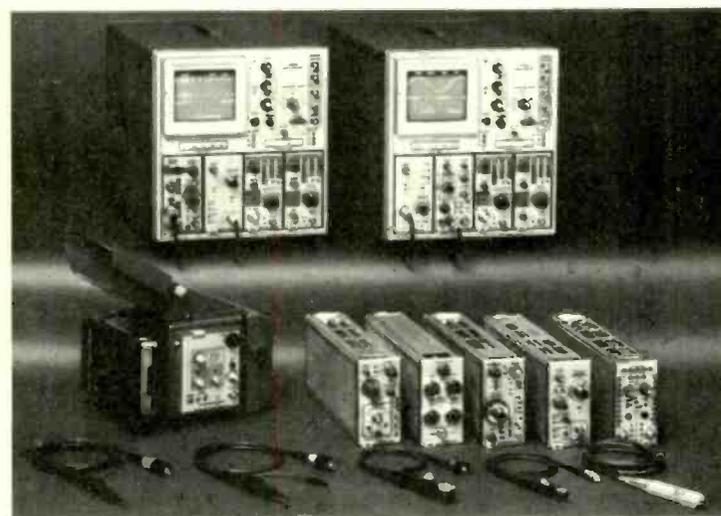
Fig. 3. Tektronix's new generation of plug-in oscilloscopes (the 7000-series) consisting of two mainframes and thirteen plug-in units, including six amplifiers, four timebase units, and three sampling units.
