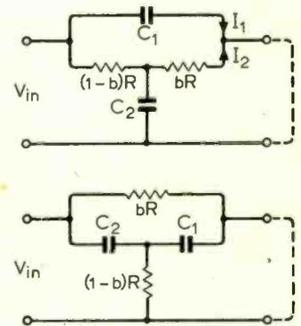
Fig. 11. Network of Figs. 9 (a) and (b) redrawn to show the two paths between input and output.
