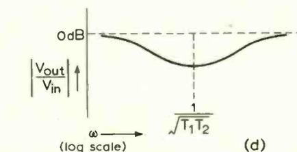
Fig. 9. Three connections of the basic 2nd-order CR network which give attenuation at middle frequencies,  $T_1 = C_1R$ ,  $T_2 = C_2R$ .
