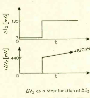
Performance characteristics of a 1W "active zener" (top) and its ordinary zener counterpart (bottom). In both cases  $\Delta V_z$  has been allowed sufficient time to settle down to a steady state.
