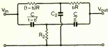
Fig. 16. For a null  $T_2' = \frac{CT_2}{b'(1 - b')}$
