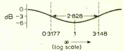
Fig. 10. Inverted Wien-bridge network showing relative component values for minimum bandwidth when maximum attenuation is 6dB.
