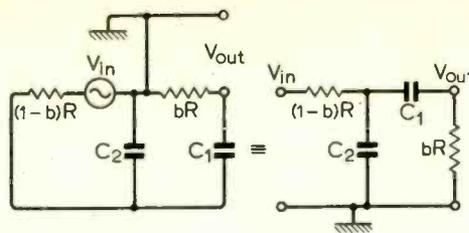
Fig. 5. Alternative connection for band-pass response.
