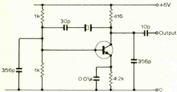
Fig. 4. 2.5-MHz oscillator incorporating calculated values.
