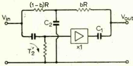
Fig. 14. For a null  $T_2' = T_2 = b(1 - b)C_2R$ .
