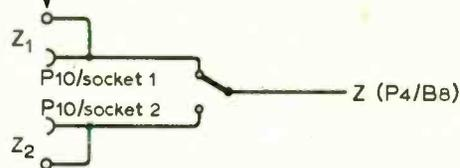
Left Fig. 78. Switching between more than one external logic circuit.
