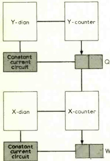
Fig. 80. Block diagram showing the additions required to produce four display areas
