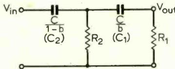
Fig. 8. The same connection as in Fig. 7 with the elements remarked to conform with the idea of a single capacitive reactance C divided into two parts.
