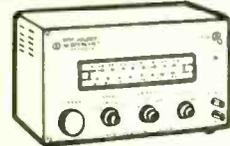
Weinbridge RC Audio oscillator featuring four overlapping scales covering 18c/s to 200 Kc/s. Output waveforms are sine, square and complex. Mirror scale with smooth geared tuning control. Output 5 volts RMS or 10 volts P-P. Sine wave response ±0.5dB. Distortion under 1% at 1Kc/s. Stability ±1%. Accuracy ±2%. O/P impedance under 3k ohms. Variable Attenuator. Mains operated. With Handbook.
