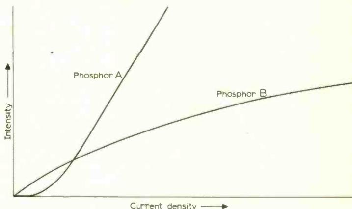
Fig. 5. Current density versus intensity plot of a single gun, dual-phosphor c.r.t. for producing multicoloured displays.
