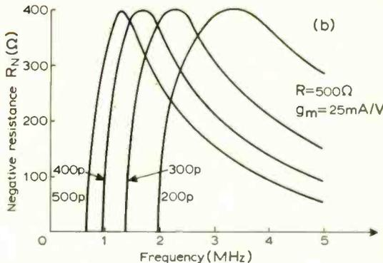
Fig. 3. Negative resistance  $R_N$  as a function of frequency (a) for  $R = 700 \Omega$  and (b) for  $R = 500 \Omega$ .
