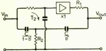
Fig. 15. For a null  $T_2' = b'(1 - b')$   $R_2 = T_2$ . Then, if  $T_1 = CR_1$   $\omega_\infty = 1/\sqrt{(T_1 T_2)}$ .
