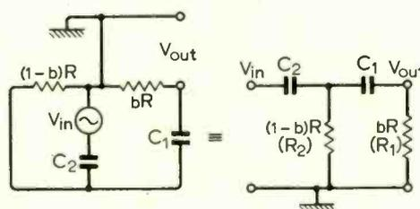
Fig. 7. Here the basic 2nd-order CR network is connected to give high-pass response.
