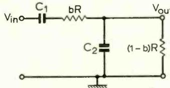
Fig. 6. Another band-pass connection—the Wien-bridge network (i.e. a Wien bridge less the ratio arms).
