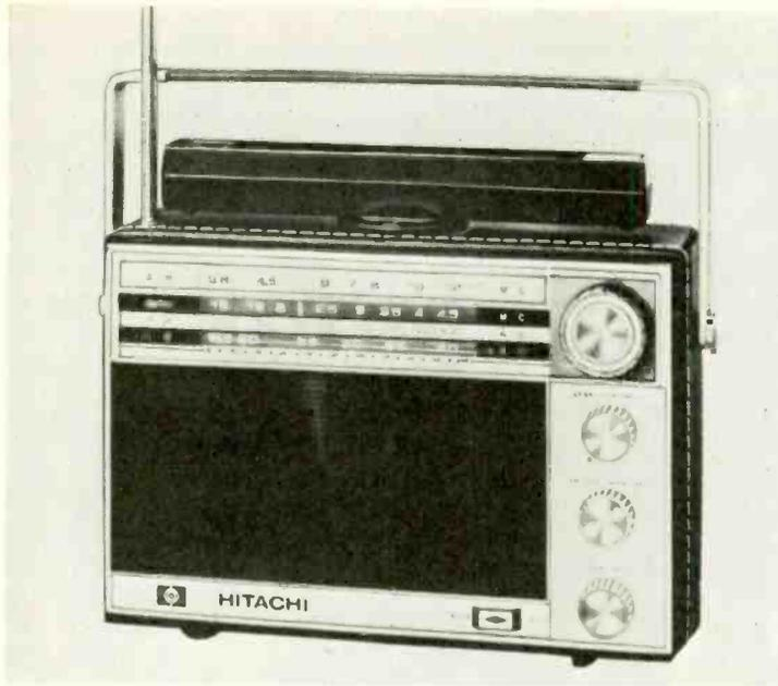
*Hitachi portable, which covers the marine band (67-188 metres) and l.w., m.w. and s.w. bands, embodies a rotatable aerial.*
