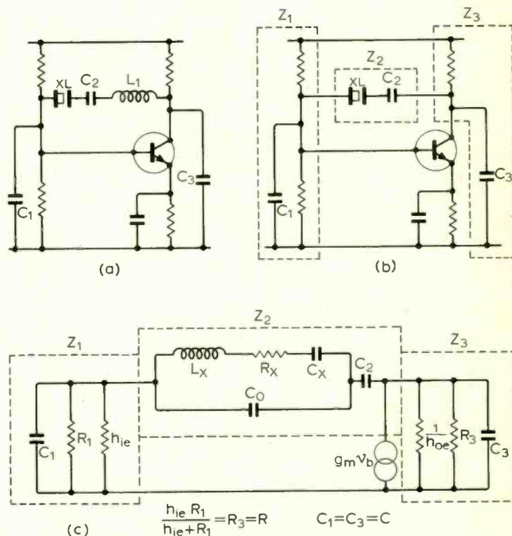
Fig. 1. Common crystal oscillator circuit (a) and with  $L_1$  removed (b). The equivalent circuit of (b) is given at (c).
