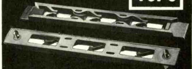
Investigations into the problems of accommodating circuit boards in conditions of extreme vibration has resulted in the exclusive features of the UNITRACK Card Guide. Moulded fingers act as pressure pads to hold boards from 0.050" to 0.125" thickness, five lengths and two styles available. Send for literature and complete details to:
