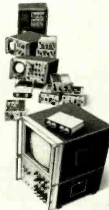
With such features as 12.4 GHz sampling, 50 µV/cm sensitivity with no drift, and variable persistence and storage, the excellence of the hp 140/141A scope system is obvious.
