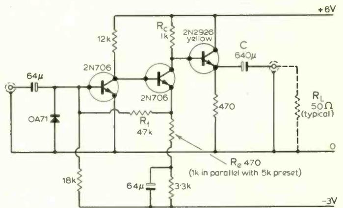
Circuit diagram of direct-coupled wideband amplifier
