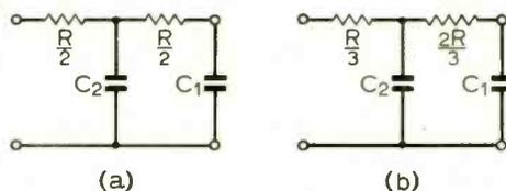
Fig. 3. Two-lag CR networks in which: (a) the two resistances are equal; (b) are in the ratio 1:2.
