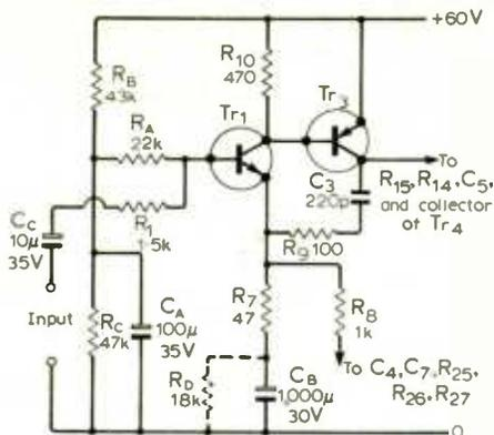
flow through the feedback resistor  $R_8$ , and thus the output stage unbalance, is only 1.5-2mA. Even this can be reduced by the addition of  $R_D$ , (shown dotted). In my own amplifiers, this has reduced the d.c. in  $R_8$  to 50µA. The values of  $C_A$  and  $C_B$  may seem excessively large, but this has been done deliberately to maintain the amplitude and phase of the a.c. feedback at the extreme low-frequency end of the audio spectrum.
