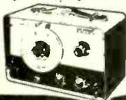
Provides audio output on 4 bands. Sine wave 20c/s to 200kc/s, output up to 7V; square wave 60c/s to 200kc/s, 7V p-p. Distortion under 2%. Output impedance 1kΩ. Variable output amplitude control. Supplied with leads and instructions. A.C. mains operated.
