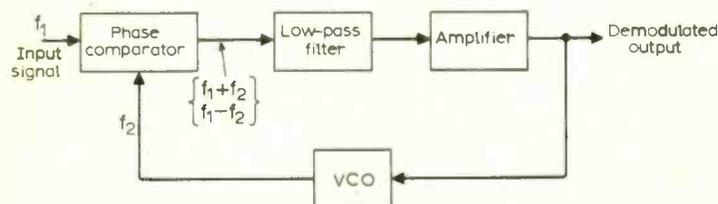
Fig. 2. An integrated circuit phase-locked loop can be employed in f.m. receivers to eliminate L-C networks and conventional detector circuitry.
