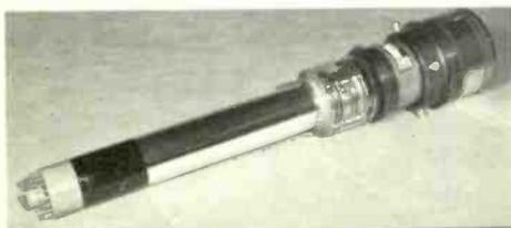
refractive optical system. The intensifier output screen and the 3-in image isocon (type P887) photocathode are both fitted with fused fibre optic faceplates, which coupled together provide an efficient transfer of the intensifier output image on to the photocathode of the isocon. Both the P899B and P887 can be supplied separately if required. English Electric Valve Co. Ltd, Chelmsford, Essex.
