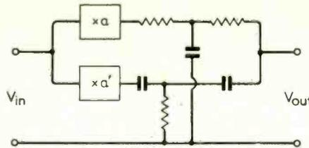
Fig. 18. Network for unsymmetrical notches: low-pass if  $a > a'$ ; high-pass if  $a' > a$ .
