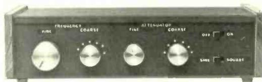
an indispensable accessory for audio enthusiasts. Neat modern styling makes this unit a most suitable companion for the Hi-fi equipment in the lounge, or an impressive addition to the workshop test gear. It is a self-contained battery-operated instrument covering frequencies from 15Hz to 200kHz, with low distortion sine or square wave output through a calibrated attenuator.
