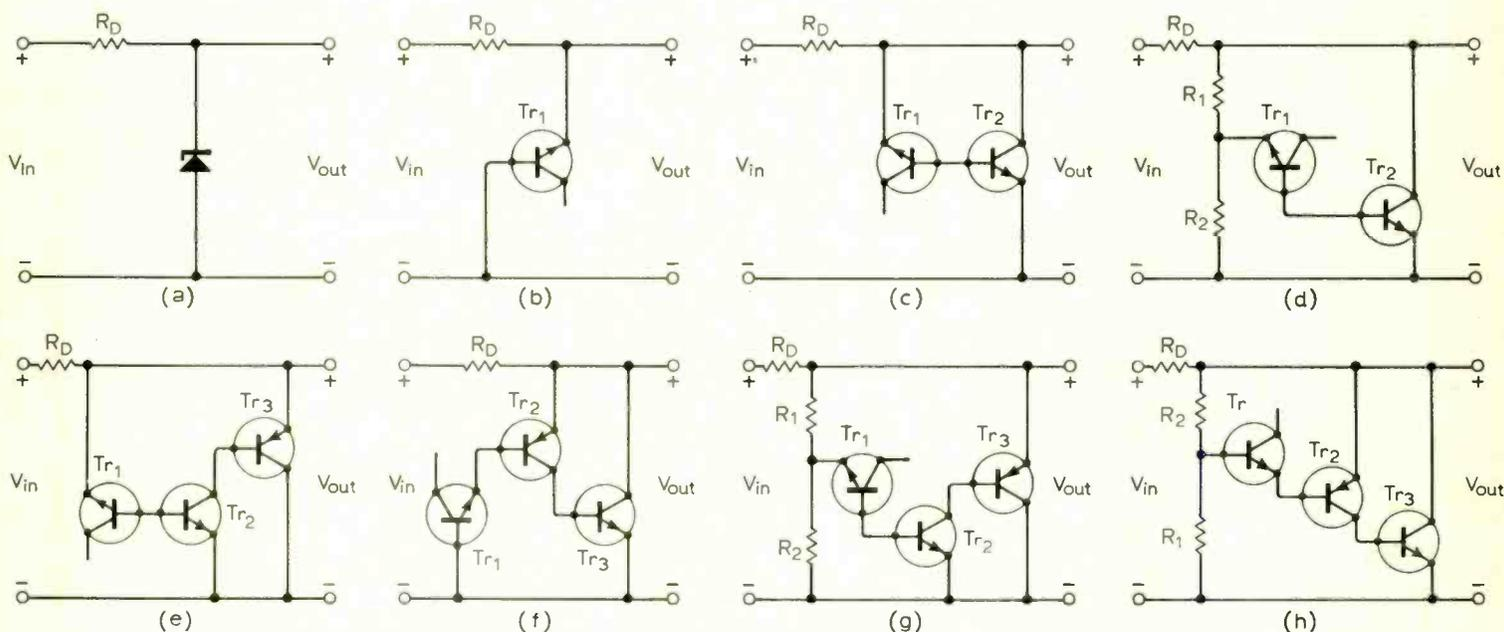
Fig. 6. (a) Zener diode shunt regulator, (b) "zener transistor" shunt regulator, (c) "active zener" shunt regulator, (d) "active variable zener" shunt regulator, (e and f) alternative "active zener" shunt regulators with boosted output current, (g and h) "active variable zener" shunt regulators with boosted output current.
