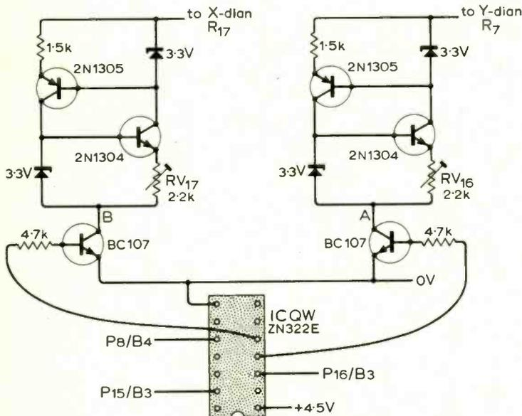
Fig. 81. Details of the circuitry needed to provide four display areas
