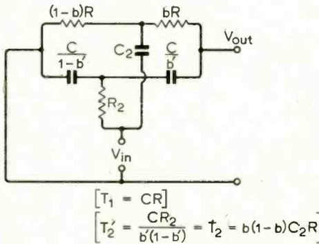
Fig. 20. Balanced parallel-tee network with output taken for "tuned-circuit" or band-pass response with  $|V_{out}/V_{in}|$  (max) = 1.
