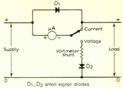
In situ current and voltage metering circuit.
