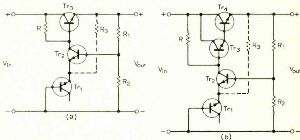
Fig. 7. (a) A simple "zener transistor" ( $Tr_1$ ) series regulator, and (b) with boosted output current.
