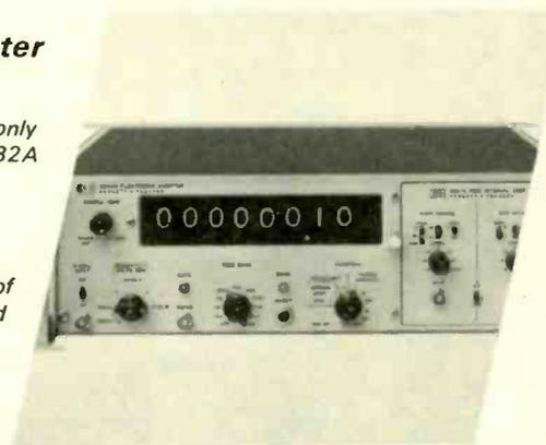
The 100 MHz time base of the 5248L has an aging rate of less than  $3 \times 10^{-9}$ /day. A second version (5248M) is equipped with an ultra-stable 100 MHz time base whose aging rate is less than  $5 \times 10^{-10}$ /day. Your hp office has the complete story.
