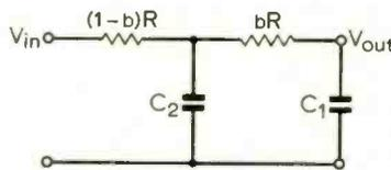
Fig. 2. Low-pass network of the two-lag type without buffer amplifier. The resistances are marked with values according with the idea of a single resistance *R* divided into two parts.
