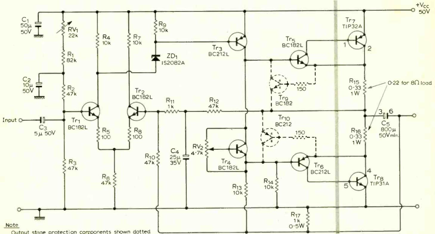
Fig.1 Amplifier circuit for driving resistive and inductive loads of 15Ω or 8Ω
