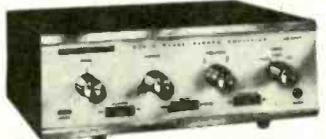
19 transistors, 8 diodes, 1HF music power 30 watts at 8 ohms. Res. 30-20,000 ±2 dB at 1 w. Distortion 1% or less. Inputs 3 mV and 250 mV. Output 3-16 ohms. Separate L and R volume controls. Treble and bass controls. Stereo phono jack. Brushed aluminium, gold anodised extruded front panel with metal case. Size 10 1/2 in. x 3 1/2 in. x 7 1/2 in. Operation 115/230 volt A.C. £28. Carr. 7/6.
