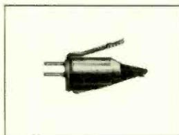
**S.P.6.** Response 20 – 20,000 Hz  $\pm$  2.5 dB. Compliance 15 x 10<sup>-6</sup> cm/dyne. Pressure 1.5 – 2.0 g. Stylus: 15  $\mu$  diamond. Output: 7 mV. 47K ohms. Price \*£7.19.6d. Replacement styli available: 15 $\mu$ , 75 $\mu$ , and 5 x 17 $\mu$  elliptical.
