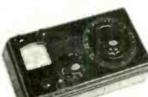
Specification. Type: Moving Coil Galvanometer. Ranges: 1. 0.05 to 5 ohms. 2. 0.5 to 50 ohms. 3. 5 to 500 ohms. 4. 50 to 5,000 ohms. 5. 500 to 50,000 ohms. Scales: Switched. Slidewire: 0.5 to 50. Galvanometer Scale: 10-10. Case: Moulded plastic. Internal source: 4V. Dry battery. Operating Temperature: +10 to +35 deg. C. Operating Humidity: Yp to 80% R.H. Dimensions: 200 x 110 x 65mm. Weight: 0.9 kg. List price £25. Our price £9/19/6.
