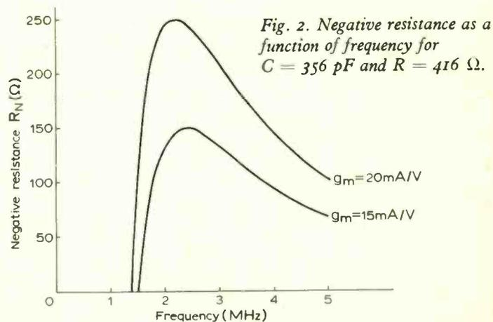
Fig. 2. Negative resistance as a function of frequency for  $C = 356$  pF and  $R = 416 \Omega$ .
