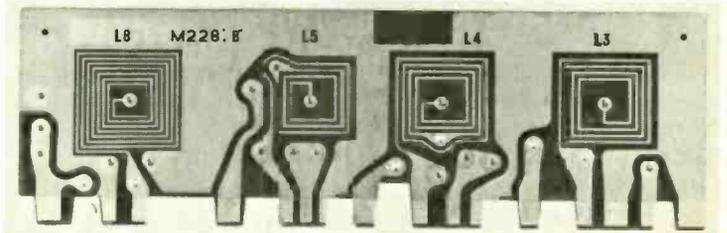
*Printed-circuit coils used in the i.f. section of the type 1500 B.R.C. single-standard monochrome receiver.*
