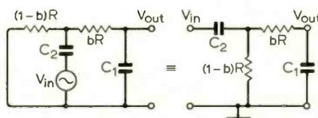
Fig. 4. Showing source ( $V_{in}$ ) and output terminals connected to give band-pass response.
