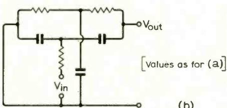
Fig. 22. Parallel-T networks connected to give "tuned-circuit" or band-pass response with peak gain  $< 1$ .
