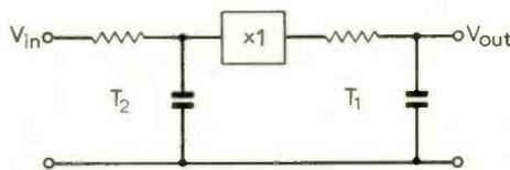
Fig. 1. 2nd-order CR network (low-pass connection) consisting of two simple lags separated by a buffer amplifier.
