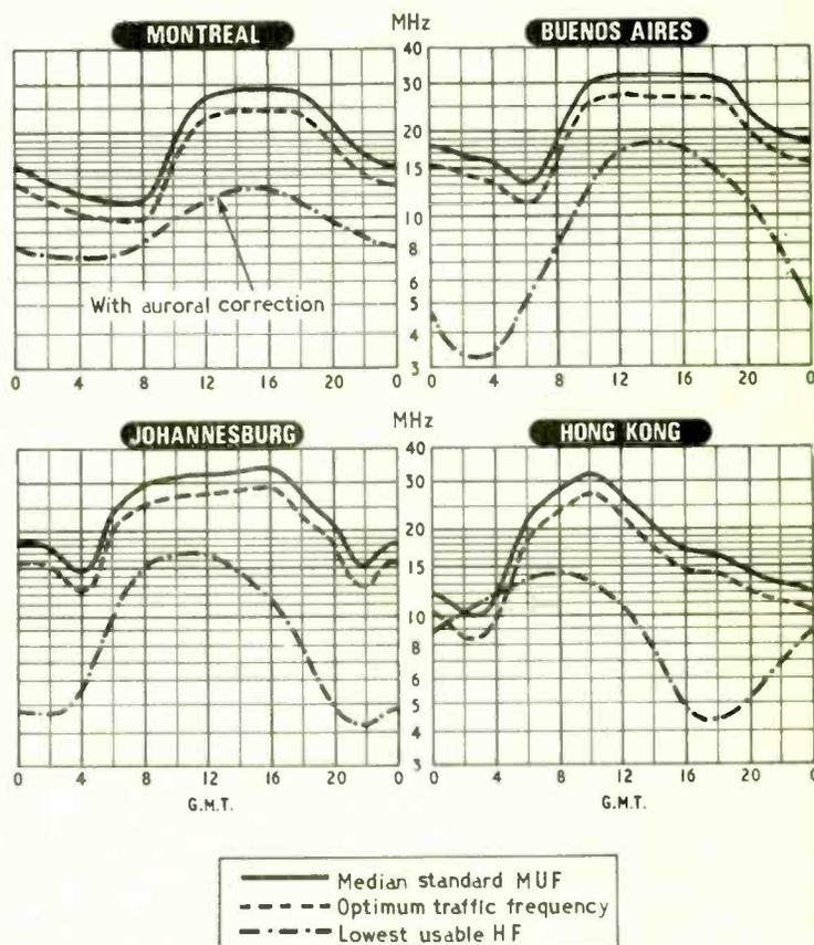
The prediction curves show the median standard MUF, optimum traffic frequency and lowest usable frequency (LUF) for reception in this country. Unlike the standard MUF, the LUF is closely dependent upon such factors as transmitter power, aerials, and type of modulation. The LUF curves shown are those drawn by Cable & Wireless Ltd, for commercial telegraphy and assume the use of transmitter power of several kilowatts and rhombic aerials.
