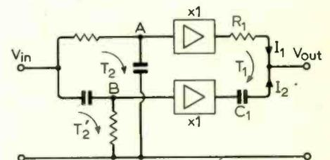
Fig. 12. Two-path network which gives a null (zero transmission) when  $T_2' = T_2$ .
