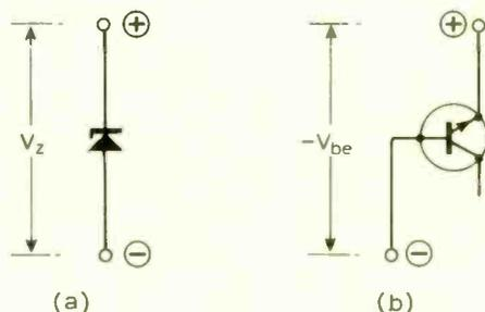
Fig. 1. (a) Ordinary zener diode, and (b) a "zener transistor".
