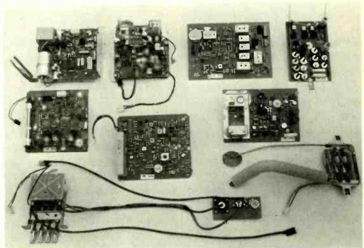
Replaceable modules constituting the circuitry of the British Radio Corporation's new single-standard colour television receiver (chassis type 3000).
