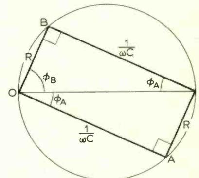
Fig. 13. Showing the 90° phase difference between the voltages at A and B when  $T_2' = T_2 = CR$ .
