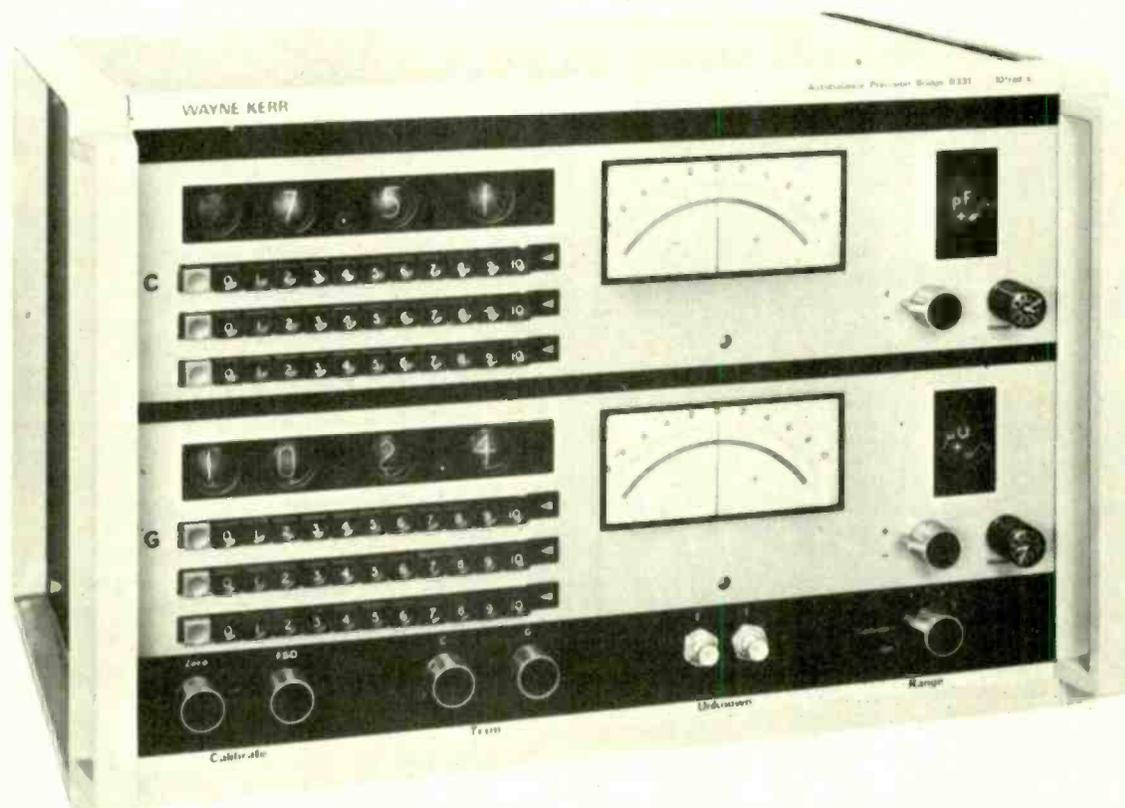
WIDE RANGE a.f. bridge for precise measurements of single components or any LCR combination – including negative resistance.
