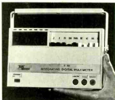
Input impedance varies from 10M $\Omega$  to 1kM $\Omega$  on d.c. volts and is 10M $\Omega$  on all a.c. voltage ranges. The display includes 3 digits and over-range indication, polarity and decimal points. Readings are given at 0.2s intervals and there are optional facilities for b.c.d. and print command outputs. Power requirements are 115 or 230V, 50 to 60Hz. A battery version is available. Price £198. Guest International Ltd, Nicholas House, Briggstock Road, Thornton Heath, Surrey, CR4 7JA.
