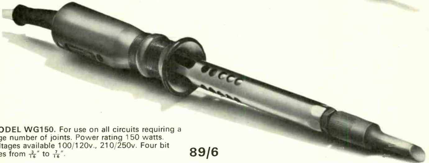
**MODEL WG150.** For use on all circuits requiring a large number of joints. Power rating 150 watts. Voltages available 100/120v., 210/250v. Four bit sizes from  $\frac{3}{16}$ " to  $\frac{7}{16}$ ".
