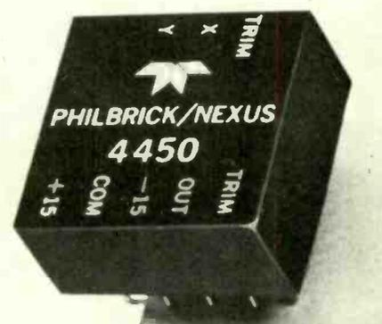
trim is required for setting up. An optional scale factor trim may be used to improve accuracy to  $\pm 0.6\%$  typical ( $\pm 1\%$  maximum) referred to 10V full-scale output. When scale-factor trim is not used, accuracy is  $\pm 1\%$  typical and  $\pm 2\%$  maximum. The price of the model 4450 in quantities of 1-9 is £41 10s each. Philbrick/Nexus Research, 81a North Street, Chichester, Sussex.
