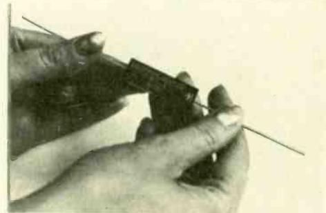
devices can be applied in all standard, single and polyphase rectifier circuits. The units are corona free and said to meet stringent electrical, mechanical and environmental specifications. Soliton Devices, Inc, 256 Oak Tree Road, Tappan, N.Y.10983, U.S.A.
