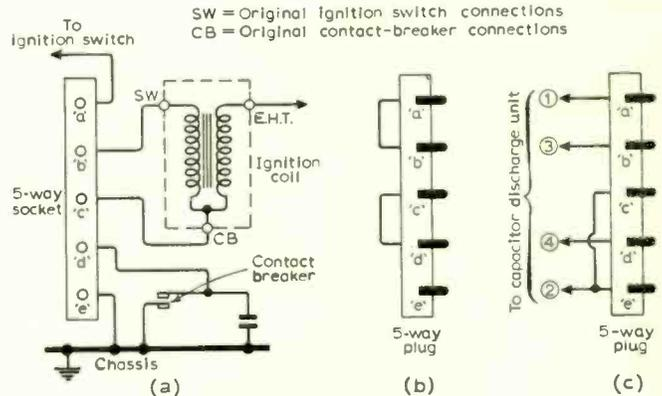
Fig. 7. Plug and socket connections required for fitting the unit to a vehicle. Unplugging the plug (c) and inserting the plug (b) into socket (a) changes from conventional to capacitive discharge ignition system.
