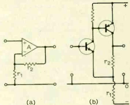
Fig. 5. Feedback less than 100%.
