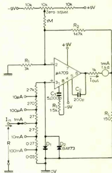
of accuracy with temperature is given as  $0.2\% ^\circ C$ . Extracted from: "The Application of Linear Microcircuits", Vol.1, SGS Ltd.
