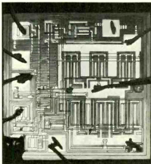
*A 13 transistor circuit measuring only one twentieth of an inch square by one hundredth of an inch thick!*
