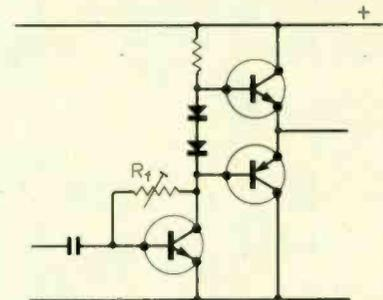
Fig. 2. Typical low-to-medium power output stage.
