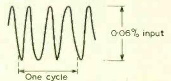
Fig. 8. Residual waveform at the base winding after passing through the twin-T filter.
