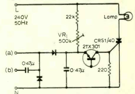
n-p-n silicon planar transistors, but by few p-n-p types. The relaxation oscillator in Fig. 1 can be used as a test circuit.
