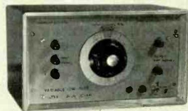
9th order Butterworth or Chebychev configuration and can realize 80dB/decade attenuation at cut off. The filters will accept an input voltage of  $\pm$ 10V peak and may be loaded with a minimum of 2,000  $\Omega$ . Lionmount & Co. Ltd, Bellevue Road, New Southgate, London N.11.
