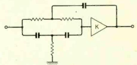
Fig. 12. Notch filter without buffer.
