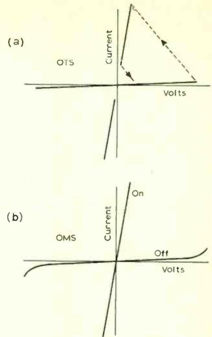
Fig. 5. Ovonic switches (a) the ovonic threshold switch: O.T.S. (b) the ovonic memory switch: O.M.S.
