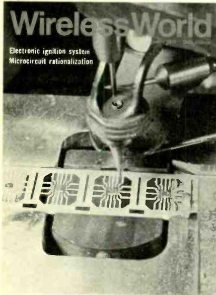
The macrophotograph on this month's cover shows wires being bonded on to integrated circuits at the Mullard Southampton works. On page 6 the future of linear i.c.s is discussed.
