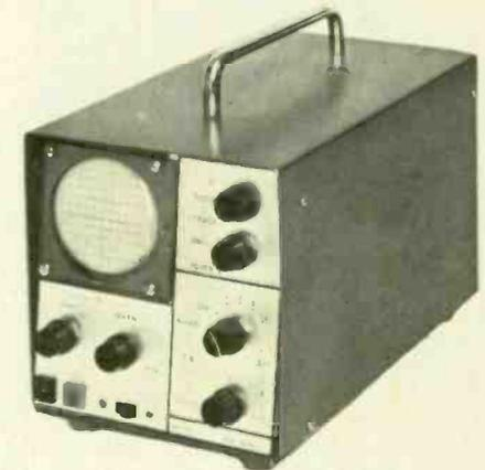
to  $100\text{kHz}$ . The instrument costs  $\pounds 24.10\text{s}$ . (discount for schools) and features a Y sensitivity of approximately  $100\text{mV/cm}$  at maximum gain with full Y shift. The timebase range covers approximately  $100\text{ms/cm}$  to  $10\ \mu\text{s/cm}$  and is automatically synchronized. The X input required is  $1\text{V/cm}$  with full X shift when the timebase is switched off. Flyback suppression and access to Y plates
