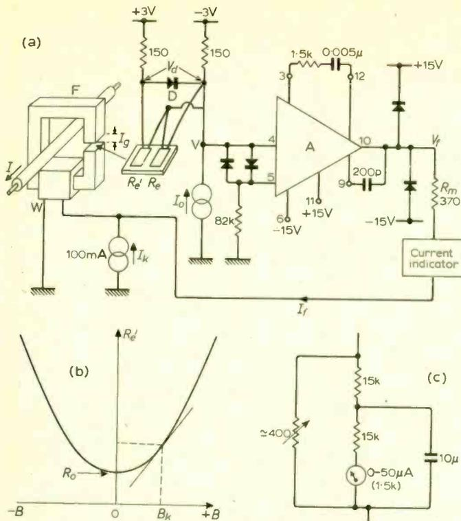
Fig. 4. Direct-current transformer. The basic circuit diagram (a) has  $R_{e'}$ ,  $R_e$  = type FP17L100 magnetoresistances (see Fig. 1 and Table 1). All diodes = silicon, type ZS72 (Ferranti).  $F$  = manganese-zinc ferrite, grade A5 ( $l_g = 0.89$  mm,  $l_l = 18.7$  cm,  $\mu = 1,000$  (Ferroxcube U-cores FX1795)).  $W = 500$  turn (N) winding of 24 s.w.g.  $A = 45,000 \pm 50\%$  (MC1709CP integrated amplifier, Motorola).
