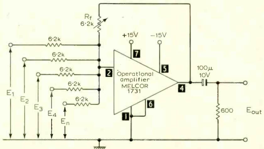
Fig. 2. Mixer using operational amplifier.
