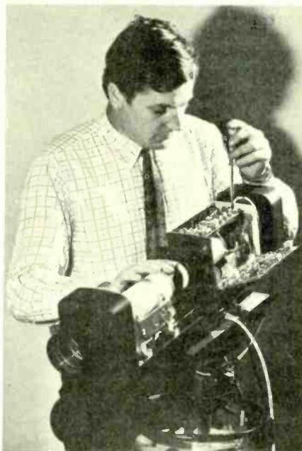
The STC low-light television camera with cover removed
