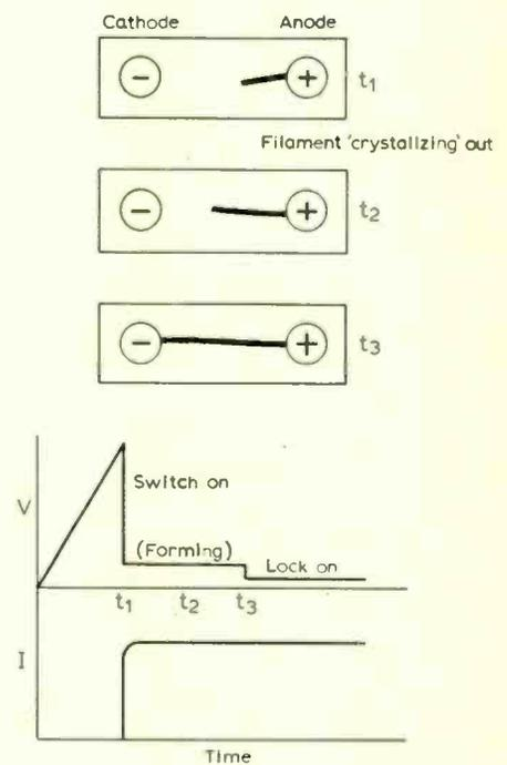
Fig. 6. Schematic of filament formation in memory device. When the voltage exceeds the threshold the current increases (switches on) but the filament takes time to form travelling from the anode. When fully formed the device resistance is lowest. This is termed locked on.
