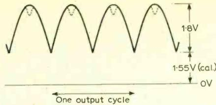
Fig. 5. Waveform across tail resistor. 'Dents' in the peaks indicate that the collectors are bottoming.
