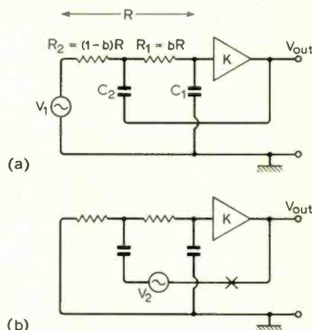
Fig. 1. (a) Sallen-and-Key low-pass filter; (b) the same with  $V_1$  short-circuited and a new source  $V_2$  introduced to facilitate analysis as a lead-lag loop with positive gain.
