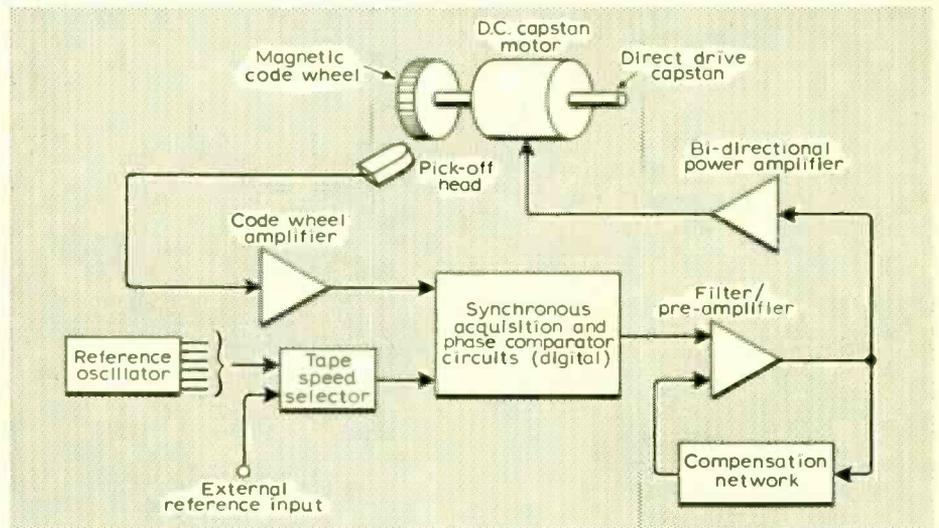
Fig. 1. Speed control system employing magnetic tachometer.
