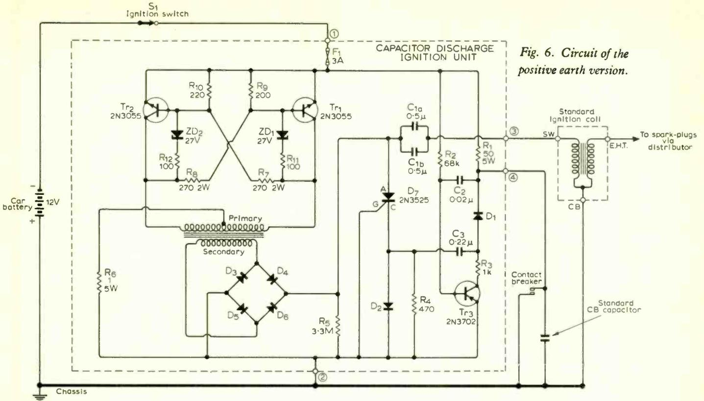
Fig. 6. Circuit of the positive earth version.
