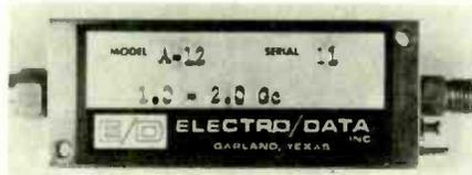
amplifier's noise figure is 6dB typical with a maximum value of 8dB. It has miniature 50  $\Omega$  input and output connectors and a shielded d.c. bias input. A single, negative 12V, 14mA source is required for biasing. Two or more units can be cascaded to provide increased gain, with minor changes in passband ripple and bandwidth. The amplifier has linear gain for output signals up to  $-10$ dBm. Electro/Data Inc., 1621 Jupiter Road, Garland, Texas 75040, U.S.A.
