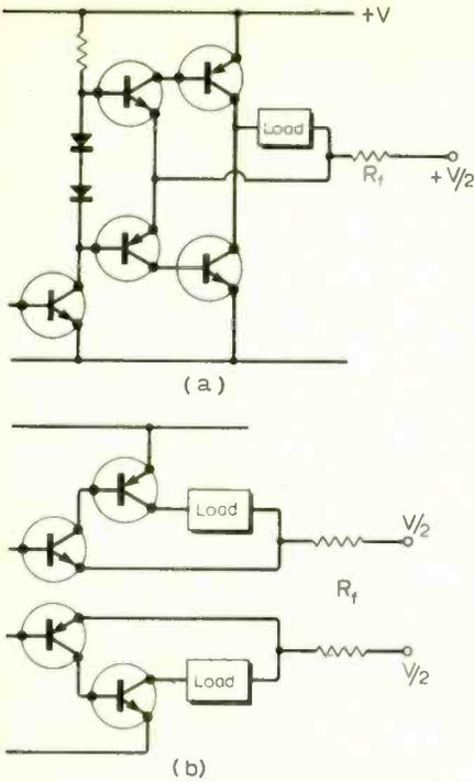
Fig. 5. High output impedance power stage. (a) Actual configuration, (b) Convenient bisection for analysis.
