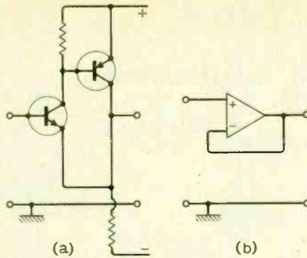
Fig. 3. Possible amplifier configurations for  $K \rightarrow 1$ .
