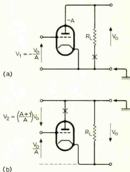
Fig. 2. Example of an active device—a valve: (a) in common-cathode connection, i.e. as a high-gain amplifier,  $V_o/V_1 = -A$ ; (b) in common-anode (cathode-follower) connection, i.e. with 100% series negative feedback,  $V_o/V_2 = A/(A + 1)$ .
