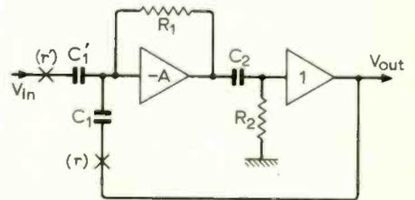
Fig. 9. Practical difficulty in high-pass circuit obtained by direct transformation of low-pass circuit (Part 5, Fig. 13).
