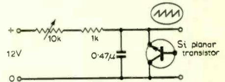
Fig. 1. Test circuit giving ramp waveform.
