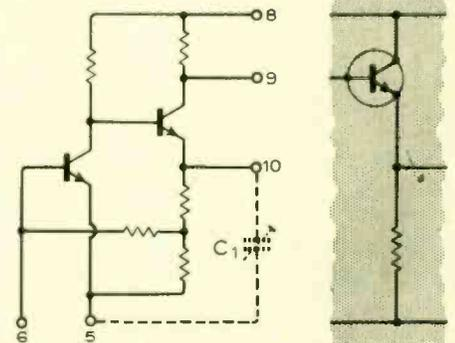
Fig. 1. The Mullard F104A/B is shown on the left which can fulfil nearly all the industrial manufacturers needs for l.f. and h.f. amplification. The shaded area contains an emitter-follower circuit which can be added so that the circuit can be made to drive long coaxial lines.
