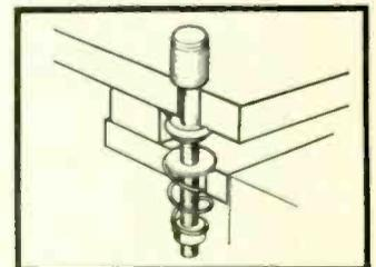
*Four-point spring suspension adjustable for height and damping protects the motor board from acoustic feedback and external vibration.*
