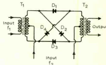
Fig. 3. Basic ring modulator circuit.
