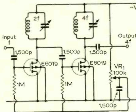
for maximum efficiency. Since  $C_{iss}$  is not highly dependent on the applied gate voltage, adjustment of  $VR_1$  does not detune the preceding circuit. Doublers are not prone to feedback and interaction problems so that dual m.o.s. devices such as the Marconi-Elliott E6029 could be used. The circuit will operate up to 150MHz with the high  $g_m$  devices of the E6019, E6029 series.
