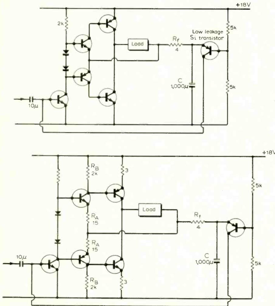
Fig. 7. Modification of the previous circuit to limit standing current in the output stage.
