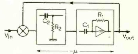
$$T_2' = C_2 R_2 = \frac{1}{q}, \quad T_1' = C_1 R_1 = qT$$
