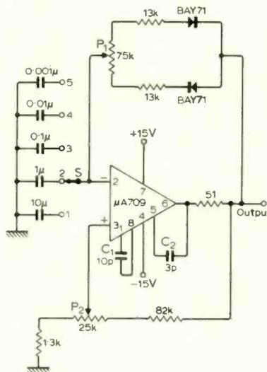
which operates by varying the hysteresis cycle. Extracted from "The Application of Linear Microcircuits", Vol.1, SGS Ltd.
