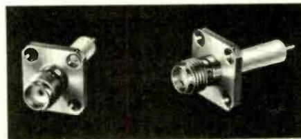
50-645-4520-31, the receptacle is constructed of gold plated stainless steel, Teflon, and gold-plated beryllium copper. It meets all requirements of MIL-C-39012 regarding contact and dielectric torque and captivation. R. F. Components Division, Sealectro Ltd, Walton Road, Farlington, Portsmouth, PO6 1TB.
