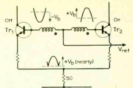
Fig. 6. How base-winding voltages add to build up reverse emitter-base voltage.
