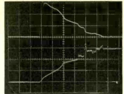
**Simultaneous Single-shot Displays.** Current versus voltage display of a 0.75 ampere, fast-blow fuse during destructive overload. Both beams are driven by B Time-Base at 50  $\mu\text{s}/\text{cm}$  which is delayed by pre-triggered A Time-Base to provide base reference lines before and after the event. The upper beam shows the current waveform at 30A/cm while the lower beam shows the corresponding voltage across the fuse at 100V/cm.
