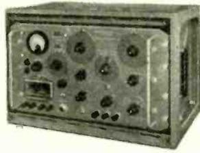
**VALVE VOLTMETER TYPE TF 958.** Measures AC 100mV; 20 c/s to 100 Mc/s, DC 50mV to 100V, multiplier extends ac range to 1.5kV. Balanced input and centre-zero scale for DC. AC up to 100MHz. £32.10.0.
