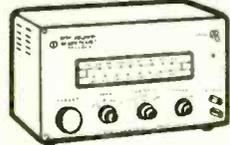
Weinbridge RC Audio oscillator featuring four overlapping scales covering 180c/s to 200 Kc/s. Output waveforms are sine, square and complex. Mirrored scale with smooth geared tuning control. Output 5 volts RMS or 10 volts P.P. Sinewave response ±0.5dB. Distortion under 1% at 1Kc/s. Stability ±1%. Accuracy ±2%. 0/P impedance under 3kΩ. Variable Attenuator. Mains operated. With Handbook.
