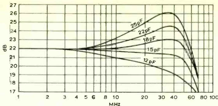
Fig. 2. Frequency response of the F 104 B with different values for  $C_1$ .
