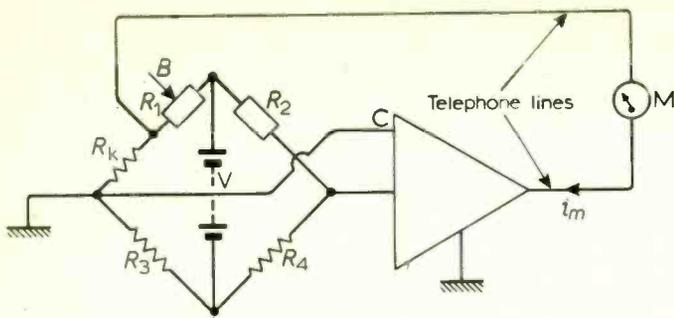
Fig. 2. Mean-square ammeter circuit.  $F_1$  = type A<sub>1</sub> manganese zinc ferrite (Ferroxcube toroid FX 1322) ( $i.d.$  = 6.35 mm,  $l_i$  = 2.76 cm,  $l_g$  = 0.59 mm,  $\mu_{min}$  = 100).  $T_{r1}$ ,  $T_{r2}$  = type C444 transistors (SGS Fairchild).  $R_1$ ,  $R_2$  = type FP28D470 magnetoresistances (see Fig. 1 and Table 1).
