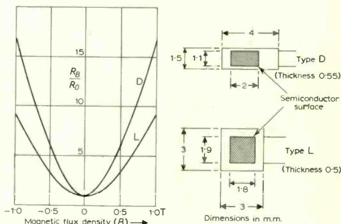
Fig. 1. Magnetoresistance relation  $R_B/R_0$  as a function of the magnetic flux density  $B$  for two commercial devices.
