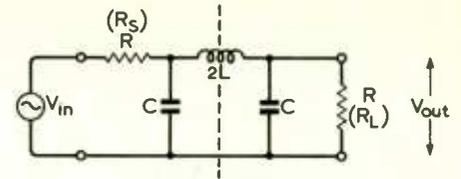
Fig. 11. Structure of simple (all-pole) passive 3rd-order low-pass filter.
