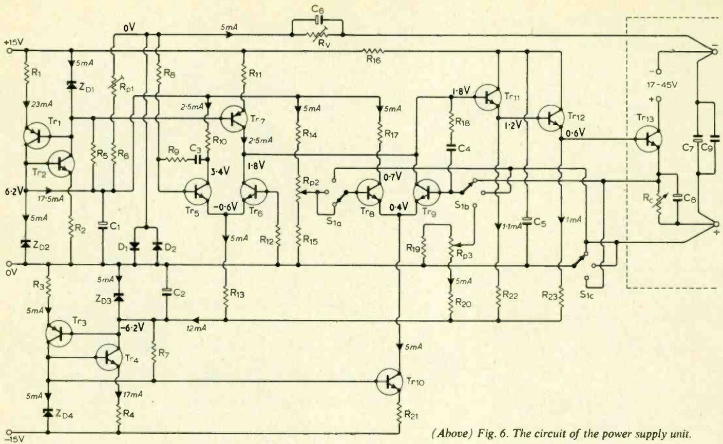
(Above) Fig. 6. The circuit of the power supply unit.
