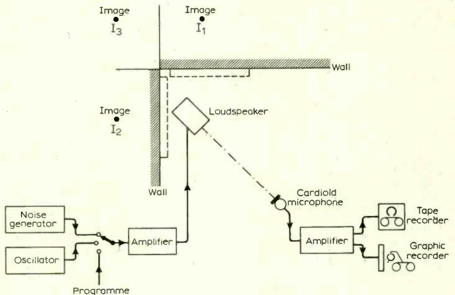
Fig. 1. Experimental set up used for investigating effects of corner placing.
