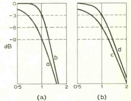
Fig. 17. Amplitude responses of Butterworth and approximately linear-phase filters.
