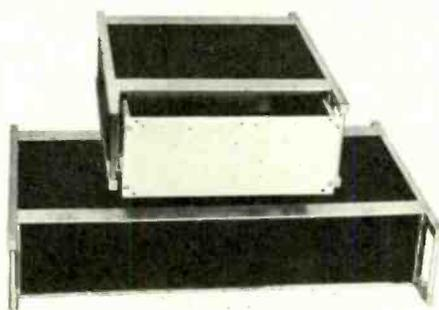
downwards or accidentally dropped. The protrusions at the rear which allow the case to stand face upwards, also protect rear connectors and components. The standard case, CS1 which is bench mounting can be converted to 19-in rack mounting simply by fitting brackets to each side. The CS1 will accept one module M1 or two modules M2. The CS2 or "half rack" case accepts one module M2 only. Case Systems, 20 Hunt Lane, Chadderton, Lancs.
