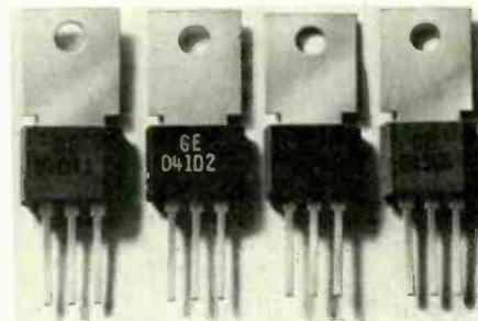
pairs: D40 brown, 1A 6W, n-p-n; D41 black, 1A 6W, p-n-p; D42 red, 3A 12W, n-p-n; D43 green, 3A 12W, p-n-p. Each type is available with 30, 45 or 60V continuous rating, with a wide range of gains up to 30. The flat pins are easily formed to TO5 or TO66 configurations. 100 up prices range from 7s 8d to 21s. Jermyn Industries, Vestry Estate, Sevenoaks, Kent.
