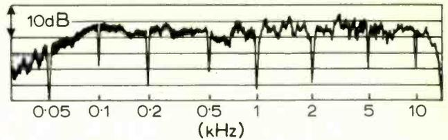
Fig. 4. Calculated response/frequency characteristics from loudspeaker in corner of room: curve A, calculated from direct and strongest three images; curve B, smoothed from measured characteristic in Fig. 2.
