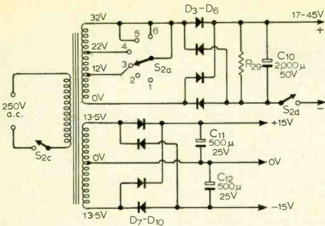
Fig. 8. The d.c. supply circuits.
