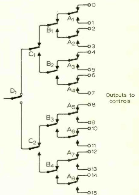
Fig. 2. (Above) Showing how the decoding can be performed with relays.
