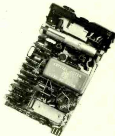
(Right) Chassis of the fireman's pocket receiver which has an operating range of between 5 and 8 km from the base station according to terrain.
