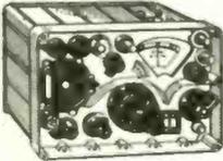
11 valve high grade communication receiver suitable for tropical use. 120 Mc/s. on 4 bands. AM/CW/PM operation. Incorporates precision variable drive. B.F.O. Aerial trimmer, internal speaker and 12v. D.C. internal power supply. Supplied in excellent condition. fully £15.00 Carr. tested and checked. 20/-.
