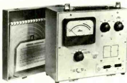
1MHz. The instrument is protected against overloads of up to +25dBm on all inputs and the measurement range of -1 to +1dBm is displayed over the full 4-in scale of the meter. The accuracy of the standard version is ±0.05dB on all inputs. However, it is now available as option 1 with special calibration charts guaranteeing an accuracy of 0.02dB on all three inputs. Hatfield Instruments Ltd, Burrington Way, Plymouth PL5 3LZ, Devon.
