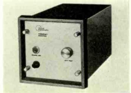
speed and overspeed modules can be housed in a single instrument to provide bandpass or high- and low-limit facilities. Thirteen overlapping ranges cover the frequency spectrum 1Hz to 30kHz. Alarm operation is within 0.1% of the set point and reset is automatically carried out without hunting. Output can be in the form of a relay changeover or of a logic level change. Construction is of i.c.s mounted on plug-in p.c. modules. Orbit Controls Ltd, Alstone Lane Industrial Estate, Cheltenham, Glos.
