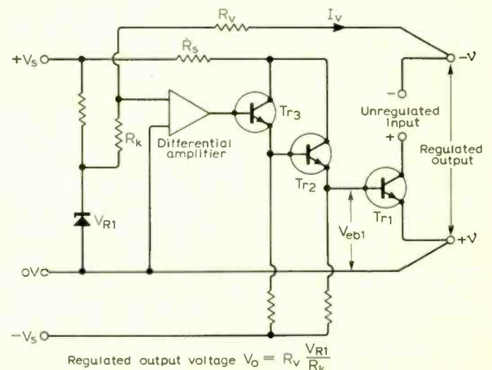
Fig. 2. Using a separate supply line for the stabilizer circuitry.
