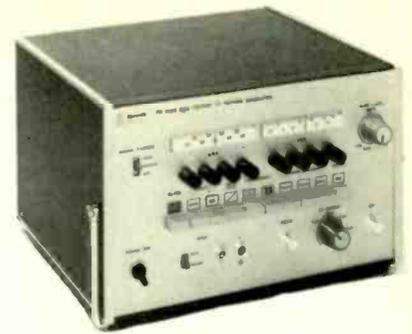
ranges covered are bands I, III, IV and V, which are selected by push-buttons and continuous tuning is provided. Outputs are 15–20mV at r.f. (continuously variable) and 1V at video, both into 75 $\Omega$ . Burst amplitude is variable for checking colour killer and a.g.c. The sound carrier can be modulated internally, unmodulated or switched off. The generator measures approximately 270 × 290 × 190mm and weighs approx. 5.6kg. Pye Unicam Ltd, York Street, Cambridge.
