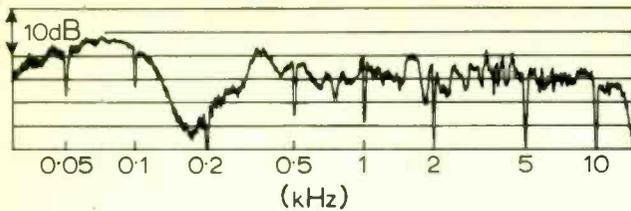
Fig. 6. Effect on characteristic of placing loudspeaker in corner touching walls and floor (warble tone).
