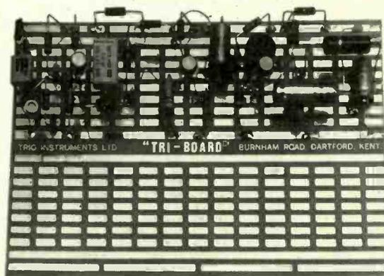
The ideal "Breadboard" material for rapid construction of electronic circuits at the design and prototype stages of development programmes.
