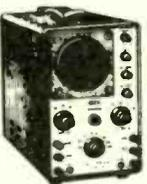
Features 3in. clear view tube, easy to use controls and good stability. Y amp. Sensitivity. 1V p-p/CM. Bandwidth 1.5cps-1.5MHz. Input imp. 2 meg Ω. 25 PF. X amp sensitivity. 9V p-p/CM. Bandwidth 1.5 cps-800 KHz. Input imp. 2 meg Ω. 20 PF. Time base. 5 ranges 10 cps-300 KHz. Synchronization. Internal/external. Illuminated scale.
