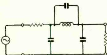
Fig. 6. Schematic for passive realization of 3rd-order Darlington response.
