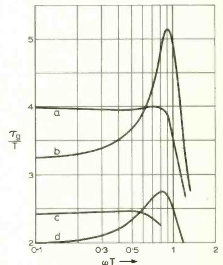
Fig. 18. Normalized group delay of Butterworth and approximately linear-phase filters.
