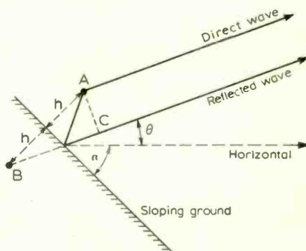
Fig. 2 With the aerial at a height  $h$  above ground sloping at an angle  $\alpha$ , the direct and reflected waves are in phase when  $2h \sin(\alpha + \theta) = \lambda/2$ . For small values of  $\theta$  this becomes  $2h \sin \alpha \approx \lambda/2$ . This diagram is identical with Fig. 1 except for rotation through the angle  $\alpha$ , and the increased ground angle.
