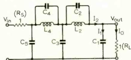
Fig. 2. Standard passive realization of 5th-order Darlington low-pass filter.
