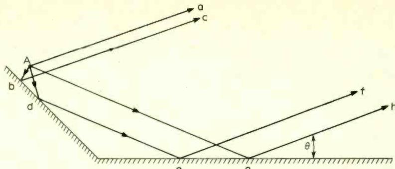
Fig. 3 Ground sloping down into the sea. The direct wave Aa, foreground reflection Abc, distant reflection Agh, and double reflection Adef add in phase if θ is small,  $hg \approx \lambda / (4 \sin \theta)$ ,  $h_s \approx \lambda / (4 \sin \theta)$ , these being the heights of A above ground and sea respectively.
