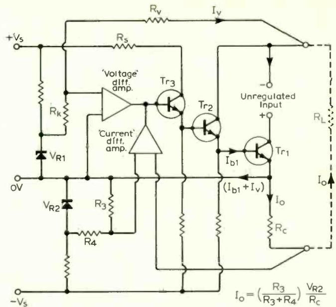
Fig. 4. Using the circuit to supply constant currents.
