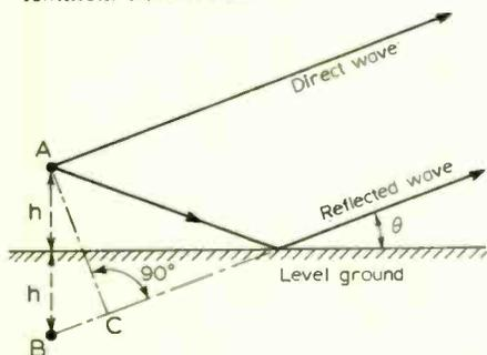
Fig. 1 When a horizontal aerial is erected at a height  $h$  over level ground, its image  $B$  is an antiphase. The direct and reflected waves are in phase at a distant point when  $BC = \lambda/2$ , i.e. when  $2h \sin \theta = \lambda/2$  where  $h$  is the angle of radiation.
