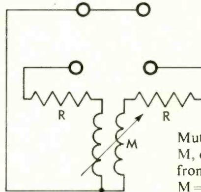
Mutual Inductance,  $M$ , can be derived from bridge C reading:  $M = R^2 \cdot C$ .
