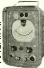
**DISTORTION FACTOR METER TYPE TF 142E.** Frequency range: 100-8,000Hz in four ranges. Distortion range: 0.05 to 50%. Input impedance 600Ω, attenuation 0-60db continuously variable. Sensitivity 1mV. £42.10.0. Carriage 20/-.
