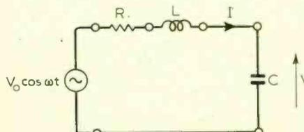
Fig. 2. The driven circuit.
