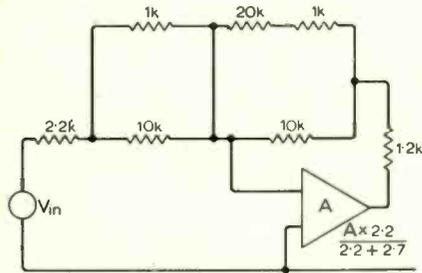
Fig. 2. High-frequency equivalent circuit.
