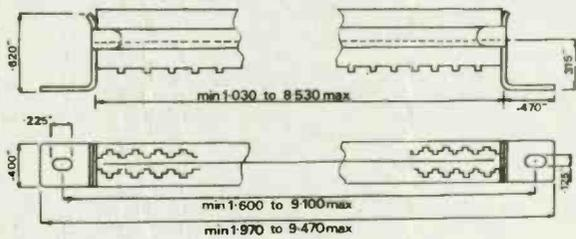
5 to 85 way single sided with solder and printed wiring tails.
