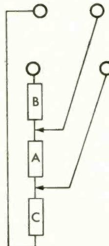
4-terminal connections minimise lead and contact resistance errors. Bridge measures A, ignoring B & C.
