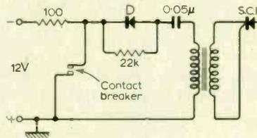
'crowbar' across the inverter output at each spark seems rather brutal and I have always used choke charging with an inductance of 3 to 5 henries between the inverter and  $C_1$ . The circuit can be simplified by using a small differentiating transformer to produce the s.c.r. firing pulse.
