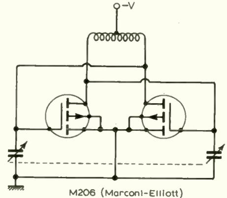
Fig. 1. Oscillator operating up to 300MHz.
