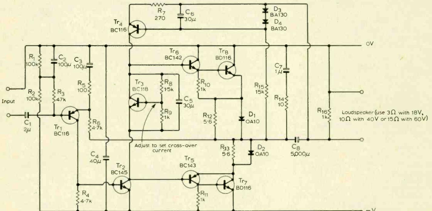
Except for  $Tr_3$  and  $Tr_4$  the transistors are from the Fairchild AF11 kit, as are  $D_3$  and  $D_4$ . All the electrolytic capacitors must carry half the supply voltage except for  $C_4$ , which carries the full voltage, and  $C_5$  and  $C_6$  which carry a couple of volts at the most.
