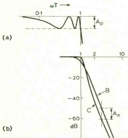
Fig. 15. Illustrating 5th-order Chebyshev response: (a) pass-band ripple, (b) increased attenuation compared with Butterworth 5th-order response, B.
