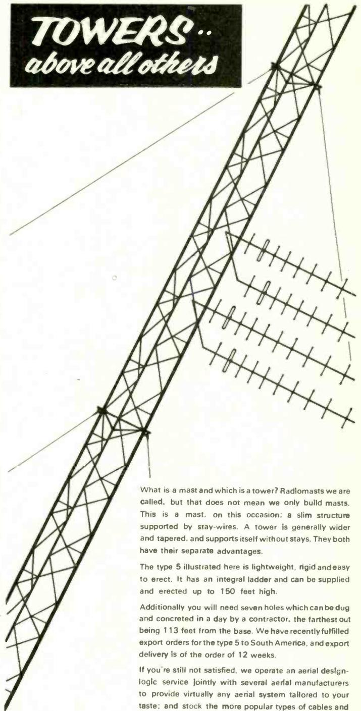
What is a mast and which is a tower? Radiomasts we are called, but that does not mean we only build masts. This is a mast, on this occasion: a slim structure supported by stay-wires. A tower is generally wider and tapered, and supports itself without stays. They both have their separate advantages.
