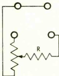
Potentiometer ratios can be related to angular rotation. Bridge reads  $R \times (1/\text{ratio})$ .
