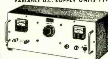
0-48 volt 10 amps, continuous from 240 volts A.C. Silicon full wave bridge rectification, isolated transformer with Variac controlled primary.
