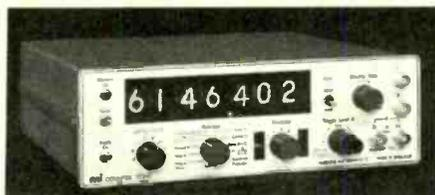
frequency standards at present available for TF2411 are: TM9933—a high-performance crystal and oven with an age rate of  $1 \times 10^{-7}$  per month and a warm-up time of 10 minutes to reach  $1 \times 10^{-7}$  operation; TM9888H—simple crystal oscillator which includes a 10-MHz external standard panel; and TM9890 which accepts external standard frequency signals between 1 and 10MHz. The choice of standard is made at the time of ordering. Marconi Instruments Ltd, Longacres, St. Albans, Herts.
