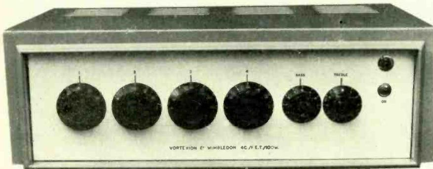
**THE 100 WATT MIXER AMPLIFIER** with specification as above is here combined with a 4 channel F.E.T. mixer, 3 mic. 1 gram with tone controls and mounted in a standard robust stove enamelled steel case. A stabilised voltage supply feeds the tone controls and pre amps, compensating for a mains voltage drop of over 25% and the output transistor biasing compensates for a wide range of voltage and temperature. Also available in rack panel form.
