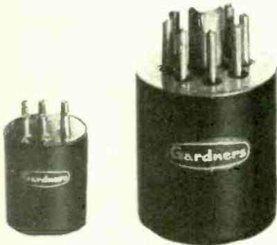
to the existing types, now have a 20,000V capability to meet the Post Office requirement. They are protected mechanically by a new filling of closed-cell epoxide resin foam compound (the smaller types are vacuum-impregnated with a micro-crystalline wax). Advanced technical data sheets AT15, AT16 and AT17 are available from the makers. Gardners Transformers Ltd, Christchurch, Hants., BH23 3PN.
