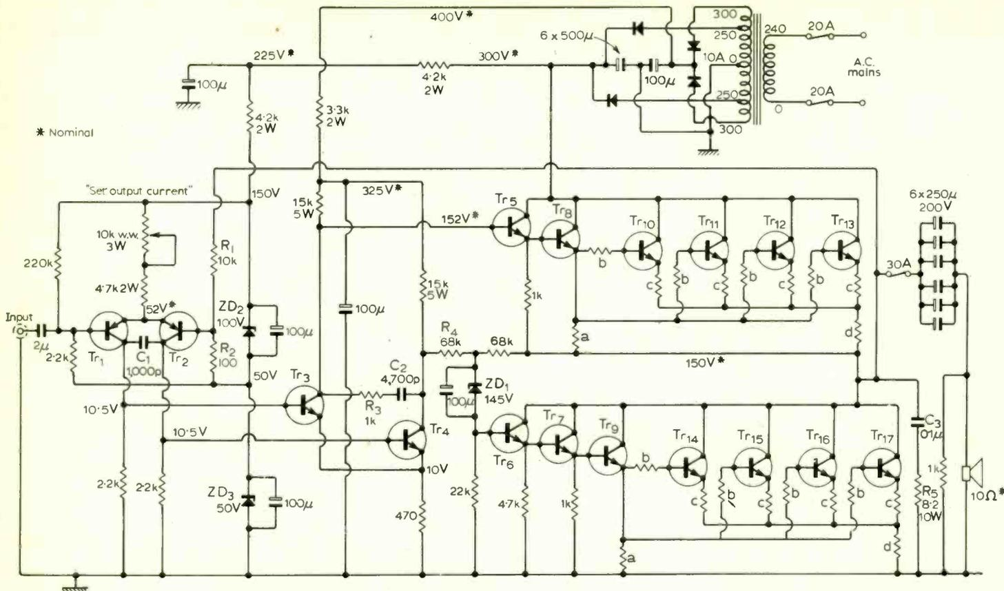
Fig. 2. Expanded version of Fig. 1 employing a Darlington triple as the output device.  $Tr_1, Tr_2$ —R.C.A. 38496;  $Tr_3$  to  $Tr_7$ —MJE340;  $Tr_8$  to  $Tr_{17}$ —MJ413. Lettered resistor values: a = 22Ω, 2W; b = 10Ω, 2W; c = 0.5Ω, 5W; and d = 0.1Ω, 5W.
