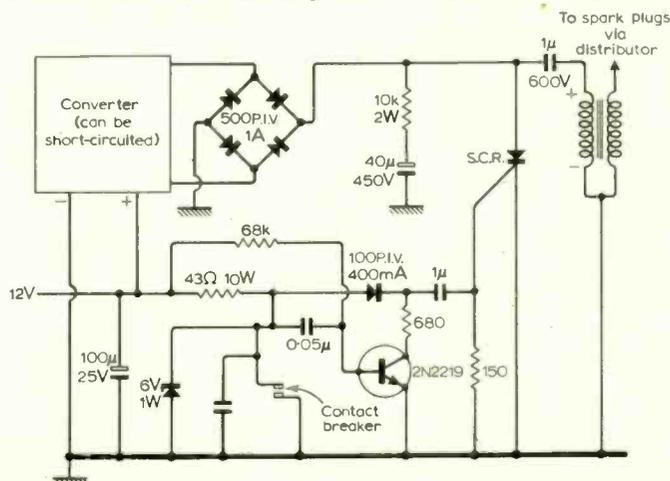
Mr. Vanderkooy's circuit. The converter is an h.f. near-perfect square-wave unit using a nickel-tape-wound toroid.
