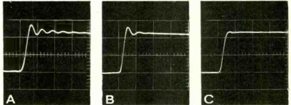
Fig. 16. Step responses of three filters: (a) a 5th-order Darlington, (b) a 5th-order Butterworth, (c) an approximate linear-phase filter.
