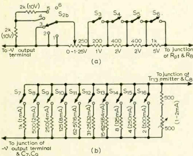
Fig. 9. (a) Construction of  $R_v$ ; (b) Construction of  $R_c$ .
