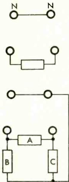
2-terminal connection for normal component measurements.
