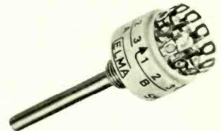
standard torque setting is 200 gm/cm; 400 and 600 gm/cm can be supplied to order. A ceramic wafer and gold-plated stud contacts are used. Contact resistance is better than  $5m\Omega$  and wafer insulation better than  $10^{13}\Omega$ . Switching capacity is up to 1A. Radiation Components Ltd, 76 Crown Road, Twickenham, Middlesex.
