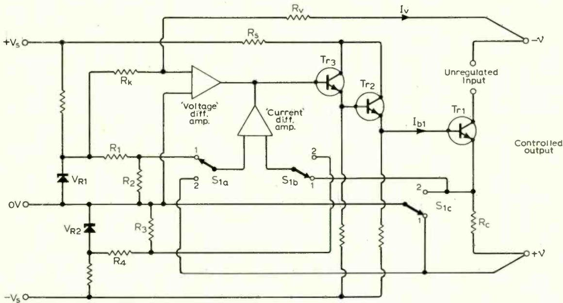
Fig. 5. Combining the circuits of Figs. 3 and 4 to provide a choice between a stabilized voltage output with current limiting or a constant current output with voltage limiting.
