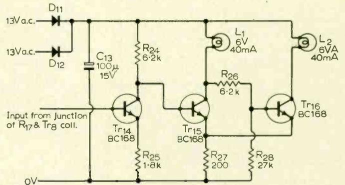
Fig. 7. Overload indicator circuit.
