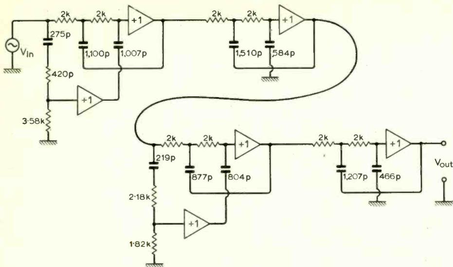
Fig. 19. Realization of the 8th-order Storey-and-Cullyer linear-phase characteristic. Resistors, Ω. Capacitors, pF.
