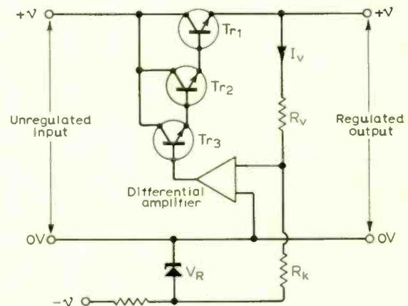
$$\text{Regulated output voltage } V_o = R_v \frac{V_R}{R_k} \quad V_o \propto R_v \text{ if } \frac{V_R}{R_k} \text{ is constant}$$
