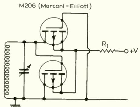
Fig. 2. Arrangement for operation between 50 kHz and 350MHz.
