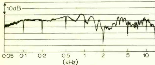
Fig. 7. High quality monitoring speaker placed in upper corner of television sound-control room (warble tone). The microphone had a cardioid characteristic.
