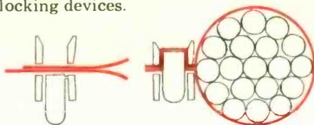
More Hellermann ingenuity . . . an exclusive extrusion system that prevents strapping pulling out even under extreme vibration. The principle is utilised in two Hellermann tying systems.
