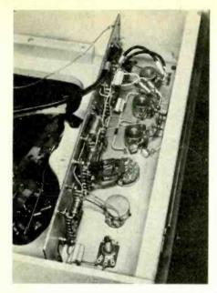
Fig. 7. View from the rear towards the front of the prototype pre-amplifier. The supply regulator is at the far end adjacent to the volume control. The tone control circuit is next, adjacent to its controls. The i.c. is at the centre, with the input stage equalization network nearest the camera.
