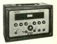
Universal Bridge for 0.1% measurements of any LCR combination from 20 micro-of-ms to 500 gigohms. Source/ detector (1592Hz) operate from a.c. or internal rechargeable battery. Sockets for external 200Hz–50kHz. Display gives units, zeroes and decimal point. Four-terminal connections from Adaptor Q221 for accurate low impecance measurements. B221
