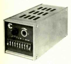
line regulation of 0.01% + 1mV; load regulation of 0.03% + 3mV (0 to full load); 1.5mV ripple voltage; re-entrant protection; input a.c. voltages of 220 or 240V a.c.  $\pm 10\%$ , with a frequency range of 45 to 400Hz; a temperature coefficient of 0.02% + 2mV per °C; and nominal d.c. outputs variable  $\pm 10\%$ .
