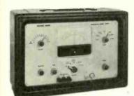
Autobalance Capacitance Bridge gives direct readout frcm 0.1pF to 10µF and w II follow a changing value. Comprehensive facilities for 'zero suppression' and comparative measurements. Analog voltage and current outputs. Accuracy 0.25%. Internal 1kHz source, 'detector. A.C. or battery operation. B541C
