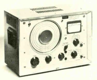
The Marconi TF 1370A gives sinewaves from 10 Hz to 10 MHz, in six decade bands – plus quality squarewave to 100 kHz and four output impedances of 75, 100, 130 and 600 ohms.
