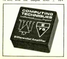
at ± 10mA from ± 15V supplies up to 20kHz. Using silicon devices throughout, the amplifier is encapsulated in epoxy resin and is housed in a plastic case 38mm square and 15mm thick. It is fully protected against short circuits from output to ground and input to supply rails. Computing Techniques Ltd, Westminster Bank Chambers, Bridge Street, Leatherhead, Surrey.
