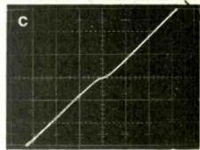
Fig. 2. Transfer characteristics at 200mA bias (a), 20mA (b), and 0mA (c). Vertical scale 500mA/division, horizontal scale 500 mV/division.
