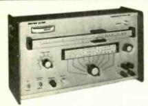
Slide-rule LCR Bridge has ten overlapping ranges for rapid 1% measurements of any component, also tolerance and phase angle. Switch selects 1kHz or 100/120Hz operation. 2, 3 and 4-terminal connections
