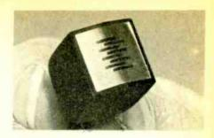
DHM/030, has a track width of 0.5mm and track spacing of 0.81mm. Inductance at 1kHz is  $30\text{mH} \pm 20\%$ . Playback full level is  $85 \mu \text{ V} \pm 1.5 \text{dB}$ . Crosstalk from a tape recorded to saturation level on seven tracks, measured on the unrecorded track, is better than -20dB. Signal current is  $300\mu\text{A}$  r.m.s. and peak bias 1.7mA at 50kHz. Phi Magnetronics (Sales) Ltd, Penwerris Lane, Falmouth, Cornwall.
