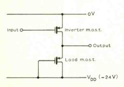
Fig. 1. The circuit of an m.o.s. inverter.
