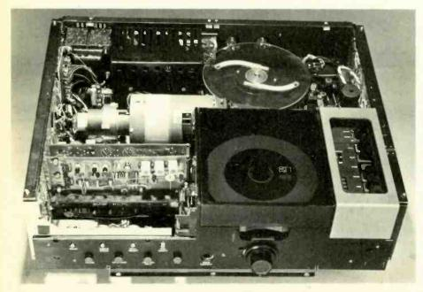
Fig. 9. The prototype player with cover removed and a cartridge inserted.
