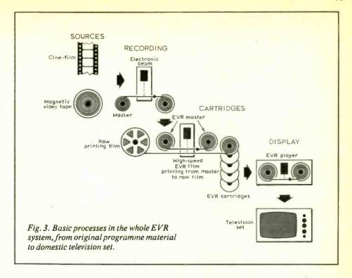
provided for loss of resolution and divergence from the desired scale characteristic. The original programme material is converted into a colour television signal which is separated into its luminance and chrominance components. Both signals are enhanced by vertical and horizontal aperture equalization and both are gamma corrected to ensure that the entire system approaches unity gamma.
