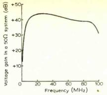
Fig. 4. Wideband amplifier gain plotted against frequency.
