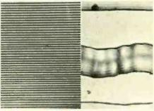
A single groove of a normal stereo gramophone record (right) compared in size with the closely packed grooves of the video disc (left) which register information by a frequency modulated carrier, hill-and-dale, recording technique. The carrier wavelength on the video disc varies with the video signal amplitude.
