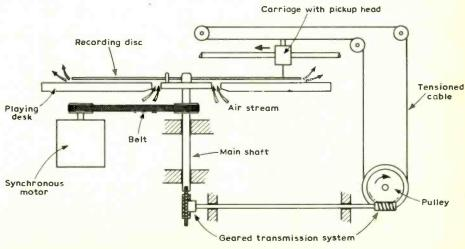
Fig. 1. Principle of the video disc reproducer mechanism.
