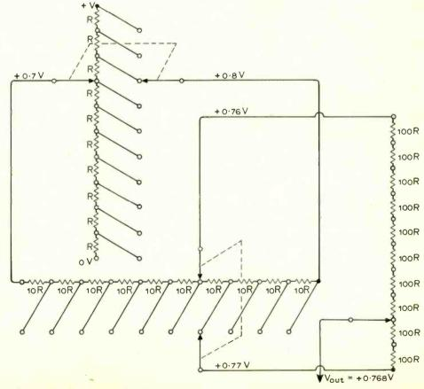
Thumb-wheel switch attenuator.
