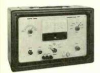
Autobalance Capacitance Bridge gives direct readout from 0.1pF to 10µF and will follow a changing value. Comprehensive facilities for 'zero suppression' and comparative measurements. Analog voltage and current outputs. Accuracy 0.25%. Internal 1kHz source/detector. A.C. or battery operation.
