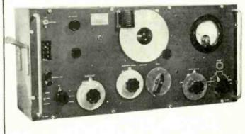
MARCONI SIGNAL GENERATOR TYPE TF-144G: Freq. 85 Kc/s-25Mc/s in 8 ranges. Incremental: ± 1% at 1Mc/s. Output: continuously variable 1 microvolt to 1 volt. Output Impedance: 1 microvolt to 100 millivolts, 10 ohms 100mV - 1 volt - 52.5 ohms. Internal Modulation: 400c/s sinewave 75% depth. External Modulation: Direct or via internal amplifier. A.C. mains 200/250V. 40-100c/s. Consumption approx. 40 watts. Measurements 191 × 121×10 in. Secondhand condition. £25 each, carr. 30/-.
