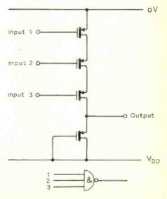
Fig. 4. A three-input NAND gate.
