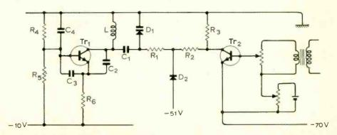
Fig. 1. The heart of the wobbulator is shown here.  $Tr_1$  is a Colpitt's oscillator tuned by the varactor diode  $D_1$ . The control voltage for this is applied through  $R_1$  from the collector of  $Tr_2$ ; this produces an output which is the exponential of its input, its base-emitter path acting as the diode of Fig. 3 (b).
