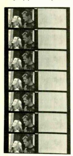
Fig. 2. Section of EVR film, showing luminance information in left-hand track, chrominance information in right-hand track, and small synchronizing windows (white rectangles) running down the middle.
