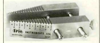
An easily adjusted hand tool for the accurate bending of resistor, capacitor, diode leads, etc., for printed circuits. Will bend leads to within  $\frac{1}{16}$  of ends of components and up to  $3\frac{1}{4}$  centres.
