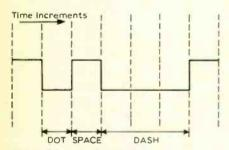
Fig. 6. Morse code waveforms corresponding to dot dash.
