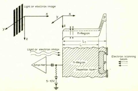
Fig. 1. Target cross-section through one diode of the RCA silicon intensifier tube.
