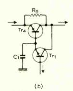
Fig. 10. (a) power supply basic circuit, (b) modification to increase current output.
