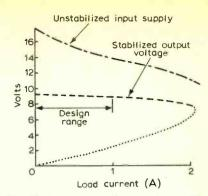
Fig. 12. Input output characteristics of 1 A output version.
