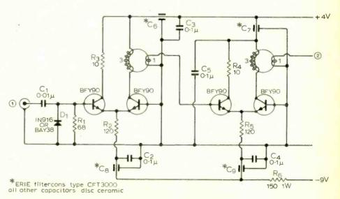
Fig. 2. Wideband amplifier circuit. The transformers are wound with 24 s.w.g. enamelled wire, primary three turns, secondary one turn.
