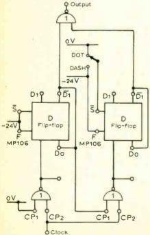
Fig. 7. Dot dash waveform generation.
