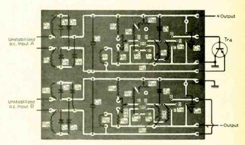
Fig. 14. Layout of power supply on standard board, frequency divider unit version.
