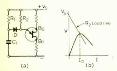
Fig. 11. (a) Heart of long period timer, and (b) steady state unijunction characteristic.
