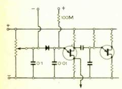
Fig. 12. Very sensitive current detector.
