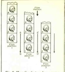
Fig. 8. How the electron beam scans the film in the electron beam recorder.
