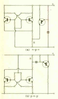
Fig. 7. Triggering a simple bistable pair from a unijunction transistor. Small "memory" capacitors are needed across the two collector-base feedback resistors. The emitter current pulse in R must knock the "on" transistor off.
