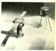
type package. All three devices are epitaxial silicon n-p-n planar transistors with an overlay emitter electrode construction. Typical ratings of the 2N5913 device at 12.5V is 2W at 250MHz (9dB gain) and at 8V is 1.5W at 250MHz (7dB gain). These devices are available from Electronic Components Division, RCA Ltd, Sunbury-on-Thames, Middlesex, and from RCA's distributors in the UK: Semicomps Northern Ltd, ECS Ltd and REL Equipment and Components Ltd.
