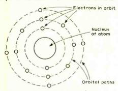
Fig. 1. Simplified diagram of an atom of silicon, an element used to make transistors. (The orbits of the electrons round the nucleus are not actually in the same plane and concentric as shown.)
