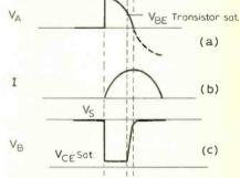
Fig. 3. The leading edge of the pulse at B (c) depends mainly on the speed with which the unijunction switches into the conducting state, and on the speed of the transistor. The trailing edge is determined by the transition of the LC "ring" across the base characteristic of the transistor. For a supply voltage of 10 V we should have  $V_{Amax} \approx 5 V$  and  $V_{BE} \approx 0.25 V$ . This would make the ratio of on-time to fall time about  $90^{\circ}/3^{\circ} \approx 30$ .
