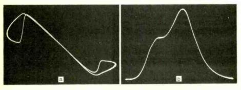
These photographs were taken with outputs from the sound channel. At (a) the output was taken from the a.f. output point; at (b) it was taken via a rectifier probe from the collector of the last i.f. stage. The circuit was not returned to correct for the probe capacitance.
