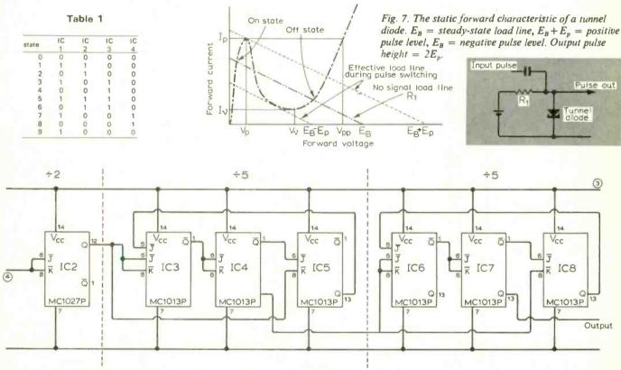
Fig. 8. The logic circuit diagram. The first divide-by-two stage is on the pulse shaper circuit.
