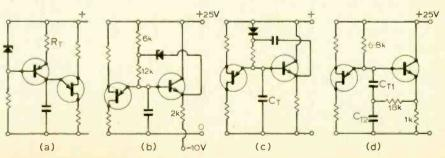
Fig. 6. Linearization circuits for sawtooth generator: (a) constant current; (b) zener bootstrap; (c) capacitor bootstrap; (d) integrator feedback.
