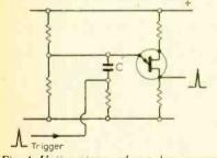
Fig. 4. Unijunction used as pulse repeater.
