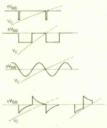
Fig. 9. Triggering details for pulse, squarewave, and sine-wave locking. If the square wave is roughly differentiated we can even (as shown on the right) get an improvement over pulse behaviour.
