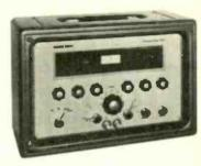
Universal Bridge for 0.1% measurements of any LCR combination from 20 micro-plims to 500 gigohms. Source/detector (1592Hz) operate from a.c. or internal rechargeable battery. Sockets for external 200Hz-50kHz. Display gives units, zeroes and decimal point. Four-terminal connections from Adaptor Q221 for accurate low impedance measurements.
