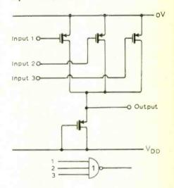
Fig. 3. A three-input NOR gate.
