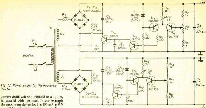
current drain will be attributed to  $RV_1 + R_3$ in parallel with the load. In our example the maximum design load is 100 mA at 9 V i.e. 90 Ω. Therefore assuming a linear related load at 1 V output:
