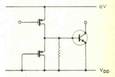
Fig. 2. Connecting a m.o.s. inverter to an n-p-n transistor.
