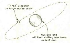
Fig. 2. Atom with "free" electron travelling in large, outer orbit. (For simplicity the inner electrons and nucleus are shown as a solid sphere.)
