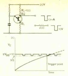
Fig. 8. Triggering a divider
