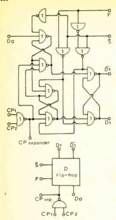
Fig. 5. Counter-register-bistable circuit type MP106.
