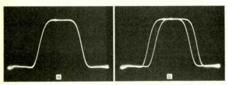
Here the marker is at 36.5MHz (a) and in (b) the phase control has been deliberately misadjusted to illustrate the effect.
