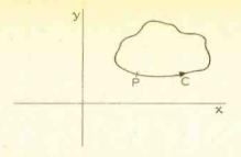
Fig. 4. At every point f(z) = f(x+jy) is analytic and single-valued. Then f(z) dz = 0 as you go round from P back to P.
