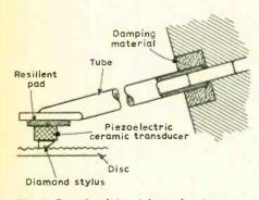
Fig. 2. Details of the pickup, showing stylus and transducer at the end of the fine support tube. The arrangement provides elastic suspension.
