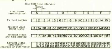
Fig. 5. Intercalation method for making an EVR film from a television (or cine film) programme source.
