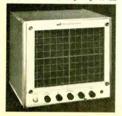
company's sweep generators. Vertical sensitivities are calibrated 5mV/cm and 50mV/cm positions with continuously variable control. The vertical bandwidth is from d.c. to 10kHz. Horizontal sensitivity is 100mV/cm (approx.) with continuously variable control. The horizontal bandwidth is d.c. to 1kHz. Price about £180 in U.K. Marconi Instruments Ltd, St. Albans, Herts.
