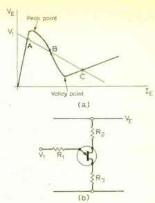
Fig. 13. (a) Bistable load line. (b) Bistable circuit.
