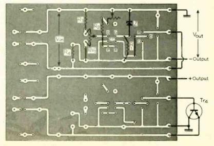
Fig. 15. Layout of power supply for other purposes.
