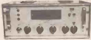
**DM2004.** For DC measurement from 1mV to 1 kV. Scale 1999 in two manually selected states of 0-999 and 100-1999. Input impedance Range 1: 1M ohms; Ranges 2, 3 and 4: 10M ohms. Accuracy 0.1% of reading. Price £95
