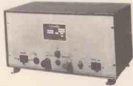
For operating and servicing battery equipment from AC Mains.
