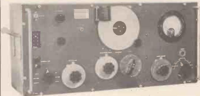
**MARCONI SIGNAL GENERATOR TYPE TF-144G:** Freq. 85 Kc/s–25Mc/s in 8 ranges. Incremental: ± 1% at 1Mc/s. Output: continuously variable 1 microvolt to 1 volt. Output Impedance: 1 microvolt to 100 millivolts, 10 ohms 100mV - 1 volt - 52.5 ohms. Internal Modulation: 400c/s sinewave 75% depth. External Modulation: Direct or via internal amplifier. A.C. mains 200/250V, 40-100c/s. Consumption approx. 40 watts. Measurements 19¼ × 12¼ × 10 in. Secondhand condition. £25 each, carr. 30/-.
