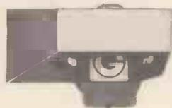
**800/E** Designed for transcription arms, a micro-elliptical diamond is fitted to a fine cantilever, end-damped against natural tube resonances, accurately terminated in a special conical hinge to give pin-point pivoting.
