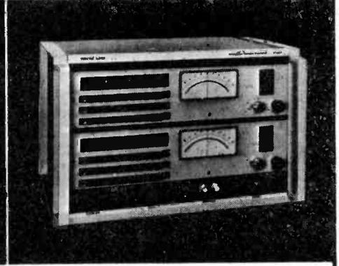
**Autobalance Precision Bridge** accurate of 0.01% though simple to operate. It measures virtually any meaningful immittance in any quadrant. Automatic compensation for measurement lead impedance. Six-figures discrimination. Analog outputs.
