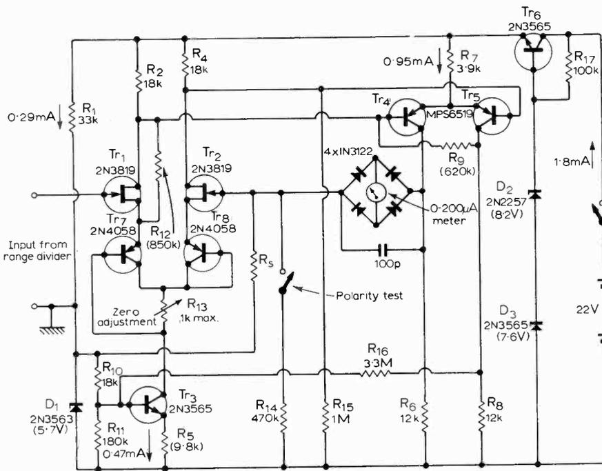
Fig. 3. Circuit of follower voltmeter. Input range divider and function switch omitted. Leaving bridge rectifier in circuit for direct voltage measurement simplifies switching.  $R_s$  determines sensitivity. Values in parentheses depend on semiconductor devices used.
