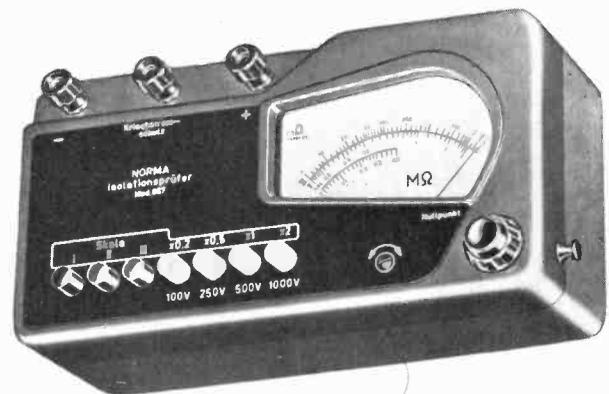
A portable lightweight insulation test set suitable for measuring the insulation resistance of all components, installations, etc. Cranking is obviated by the utilisation of a transistor converter; the power supply being two 4½-volt dry batteries. The test voltage and range are selected by push buttons which facilitate quick and easy reading of the resistance value.
