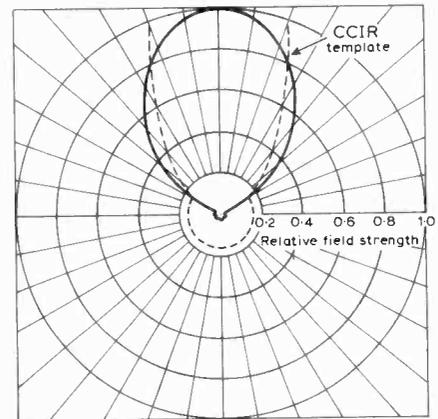
Fig. 5. Radiation pattern at 650MHz for vertical polarization.
