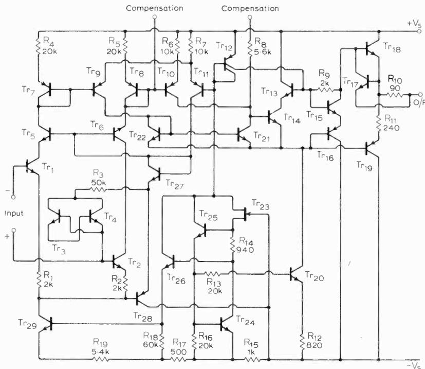
Fig. 6. Third generation example, the LM108.  $Tr_1$  and  $Tr_2$  are 'super-gain' or 'punch-through' transistors which operate at very low voltages.
