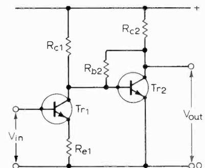
Fig. 10. Skeleton form of two-stage voltage amplifier.
