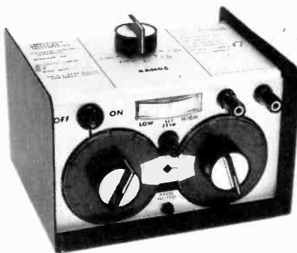
when the bridge is out of balance. Accuracy is  $\pm 0.2\%$   $\pm 1$  scale division. Resistance range is from 0.1 ohm to 1.1 megohms. J. J. Lloyd Instruments Ltd, Brook Avenue, Warsash, Southampton, Hants.
