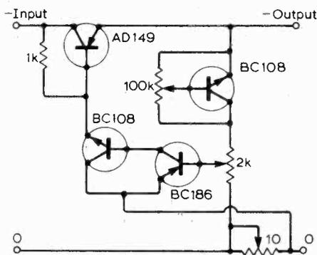
Fig. 2. Regulator with zero or negative output resistance.
