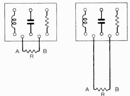
Fig. 2. We can move R away from the system on the end of a line of characteristic impedance R.
