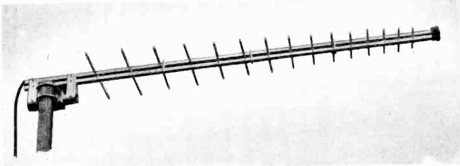
Fig. 3. Aerial and mount adjustable for either horizontal or vertical polarization.
