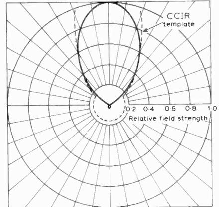
Fig. 4. Radiation pattern at 650MHz for horizontal polarization
