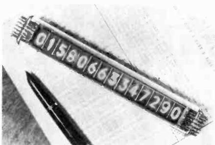
claimed to be more reliable than separate tubes. It uses a mixture of gases to give a luminance of  $600\text{cd/m}^2$ . Coincident pulses of greater than  $150\mu\text{s}$  are used to illuminate digits. Separate cathodes are provided for decimal points. Flicker can be eliminated by using an alternating supply of over 70Hz. Mullard Ltd, Torrington Place, London WC1E 7HD.
