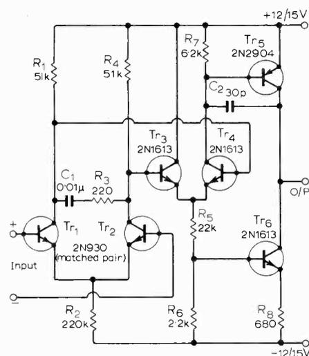
Fig. 1. Discrete component operational amplifier.
