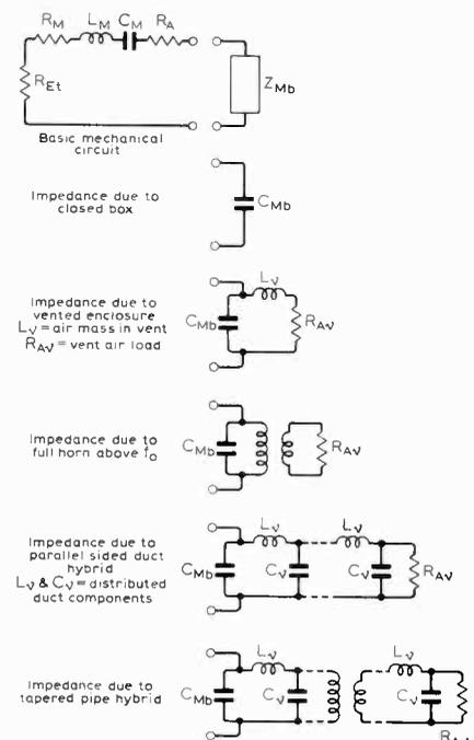
Fig. 2. Mechanical impedances applied to rear of cone by different enclosures. The impedance appears in series with the analogous circuit.
