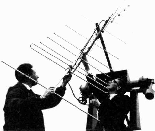
*The mutli-element crossed Yagi designed by Marconi for the ship-to-shore link. It has the fairly wide beamwidth of  $30^\circ$  to allow for rolling of the ship. The frequencies used were 135.6 and 149.22 MHz, the shore station power was 250W.*
