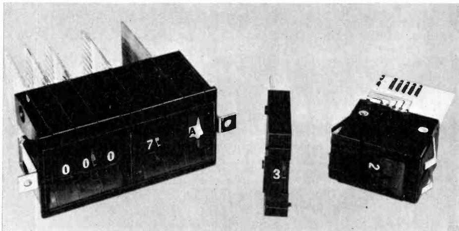
binary, and binary with complement. Multi-pole switching is achieved by coupling together a switch and up to four slave modules. Terminations are for direct wiring or for edge connectors and are numbered. Contact rating is 100mA at 50V d.c. Life is specified as being not less than  $10^6$  operations. Dimensions of the switches are height 33mm, width 8mm. Professional Component Division, Plessey Components Group, Abbey Works, Titchfield, Fareham, Hants.
