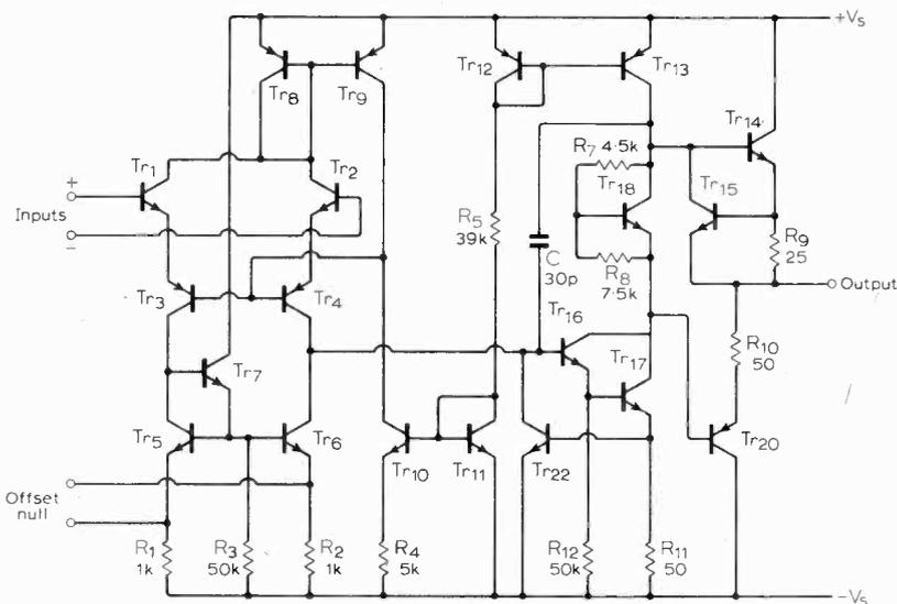
Fig. 4. The μA741. Note the diffused compensation capacitor.
