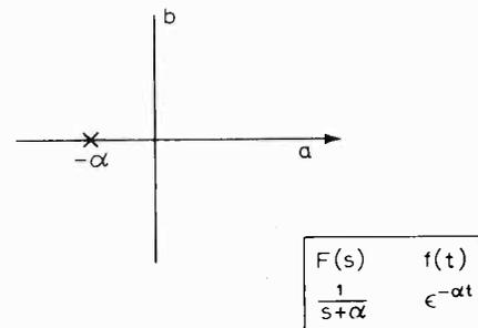
Fig. 7. The  $s$ -plane, ( $s = a + jb$ ), showing the pole of  $s$  at  $s = -\alpha$ .
