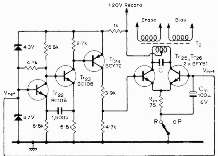
Fig. 30. Circuit diagram for an erase-bias oscillator.
