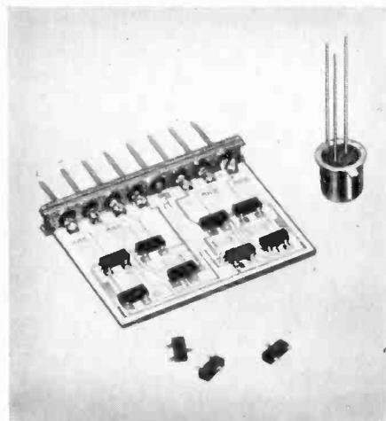
$V_{CEO}$  maximum ratings of 45V. Transistors measure  $2.9 \times 1.3 \times 0.85$ mm excluding contacts. Types BCW69/70 are p-n-p types and BCW71/2 are n-p-n types. In the illustration they are compared with
