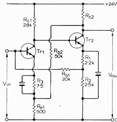
Fig. 11. More detailed version of the circuit in Fig. 10, designed for a voltage gain of 100.
