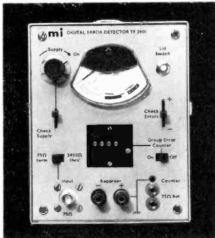
errors in 24- and 32-channel equipment at bit rates of 1.536 and 2.048 Mbits/sec. A meter indicates presence of a signal and errors. A totalizer displays total errors over any period of time. It has an internal 9V battery. Marconi Instruments Ltd, St. Albans, Herts.
