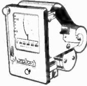
by RUSTRAK of America. This recorder indicates the magnitude of applied currents or voltages by a continuous distortion-free line on pressure sensitive paper. Chart width 2 1/2 in. Chart speed 1/4 in. per min. Moving coil movement, scale calibrated 0-100 microamps. Int. resistance 4,600 ohms. Chart drive motor 12V. D.C. Supplied less case. C/W handbook. Price £40. P. & P. 10/-.
