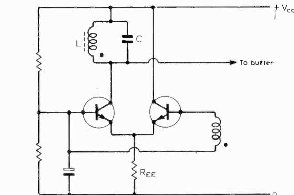
Fig. 25. A current-switching oscillator.
