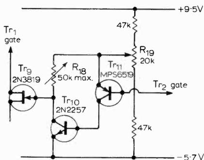
Fig. 6. Feedback circuit for raising input impedance. With this circuit voltmeter reading changed by only 1% of full scale in 30 min with a  $0.01\mu F$  input capacitor (self time constant 400 days).
