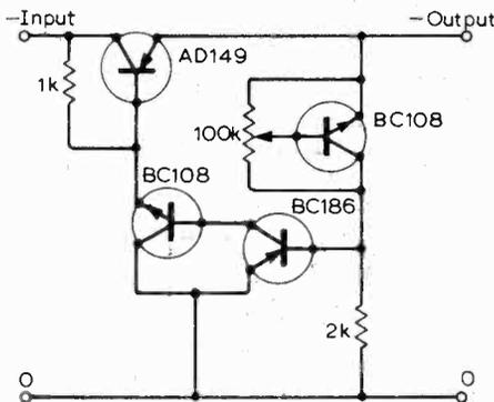
Fig. 1. Power supply giving 9V output from 12V input.
