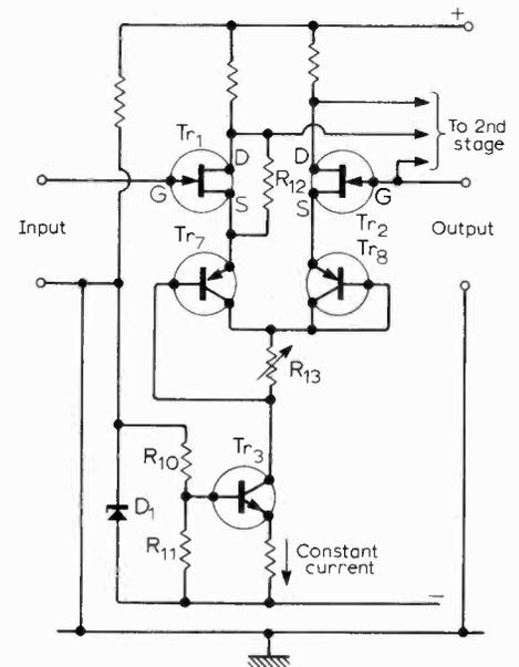
Fig. 2. Circuit compensates for bias differences by using diodes ( $Tr_7$  &  $Tr_8$ ) to approximate constant voltage devices.
