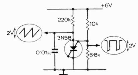
The s.c.s. has been in use for many years, why give it a new name? The circuit shown above, using a General Electric 3N58, produces much the same result as Fig. 14 in Mr. Greiter's article.
