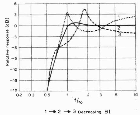
Fig. 6. Effect of  $Bl$  on response of vented enclosure.
