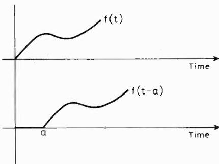
Fig. 6. A function, and the corresponding delayed function.
