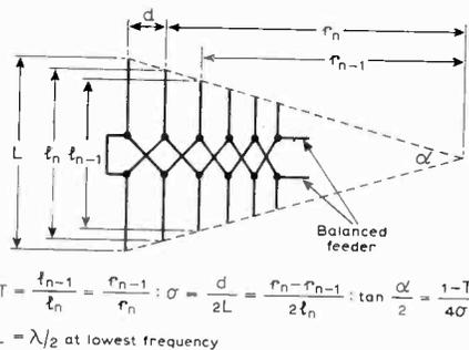
Fig. 1. Schematic representation of log-periodic aerial with dipole elements connected to balanced feeder. Longest and shortest elements are made approximately  $\lambda/2$  at lowest and highest frequencies.
