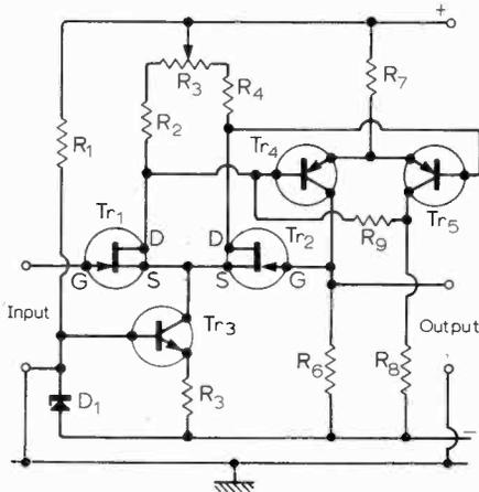
Fig. 1. Basic voltage follower circuit. Field-effect-transistor differential amplifier gives high input impedance with low offset voltage. Low output impedance is achieved by both negative feedback from  $Tr_4$  collector and positive feedback from  $Tr_3$  collector.
