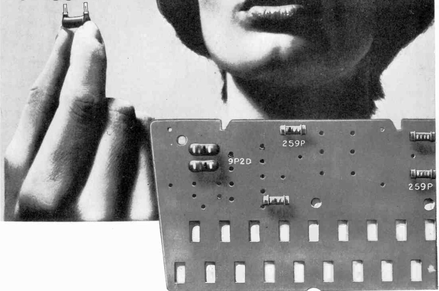
Erie's range of high stability tin oxide resistors has a new feature that makes them unique — PLUGGABILITY. They are the 259P and 259P2 Series and are, of course, close tolerance types.
