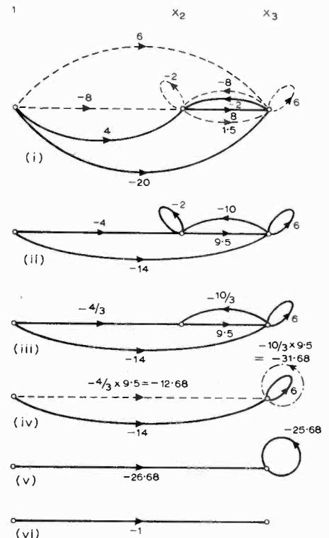
Fig. 7. Solution of the signal-flow graph of Fig. 1 by successive node elimination.
