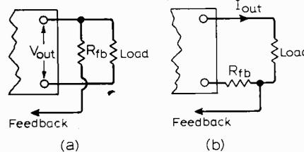
Fig. 2. General circuits for (a) parallel-derived and (b) series-derived feedback.
