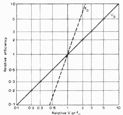
Fig. 4. Variation of efficiency with cabinet volume  $V_b$  and low-frequency limit  $f_0$ .
