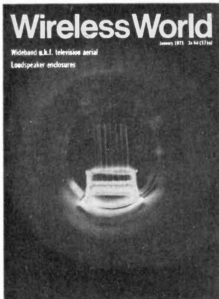
This month's cover picture depicts the high temperatures needed for semiconductor diffusion. It illustrates one of the 26 diffusion furnaces, which normally operate in the 900 to 1200°C range, at the Toulouse manufacturing plant of Motorola Semiconductors. Primarily used for the diffusion of integrated circuits each furnace has an output of at least 10,000 wafers per week.
