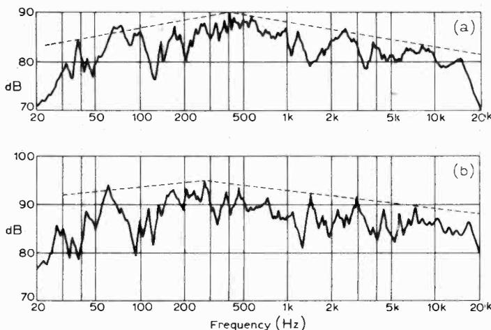
Response curves for a loudspeaker placed against a wall (a) and in a corner (b).
