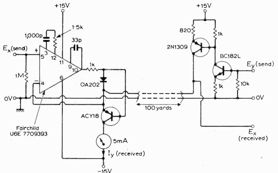
than 20mV throughout the entire range of  $E_x$  from 0 to 5V. (2) With a change of  $E_x$  from 0 to 5V the change in  $I_y$  was less than  $30\mu A$  throughout the entire range of  $I_y$  from 0 to 5mA.
