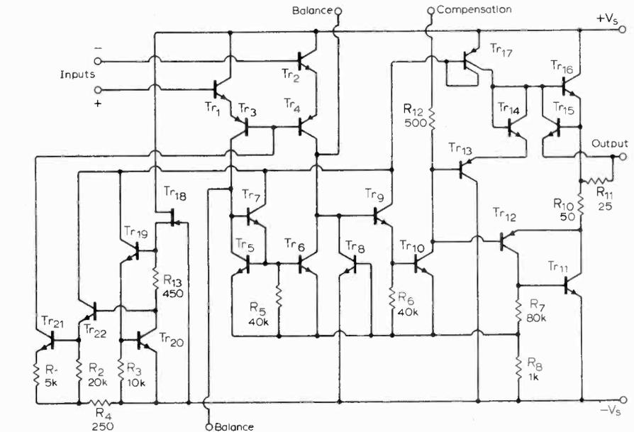
Fig. 5. Second generation example, the LM101A. Both bipolar and field effect transistors are used.
