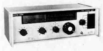
Direct reading frequency scale is accurate to 1% and a secondary output is provided for connection of a frequency meter. Frequency is unaffected by the load impedance and affected by only 0.5% by the attenuator. The generator works from 110 or 240V mains and weighs 6kg. Wayne Kerr Ltd, Roebuck Road, Chessington, Surrey.
