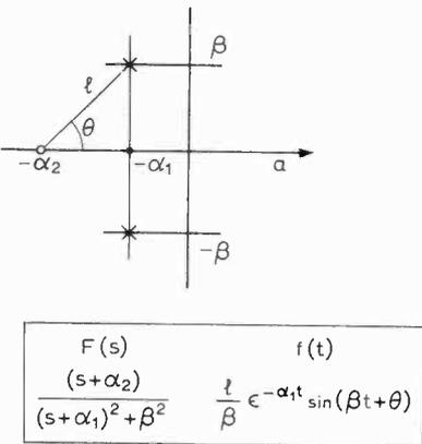
Fig. 10. Two poles and a zero in the s-plane.
