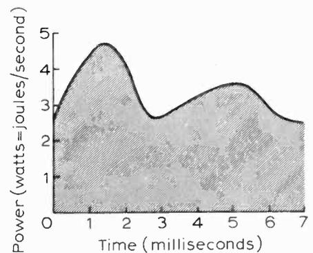
Fig. 3. Graph of a signal in which information is represented by a variation of power with time.
