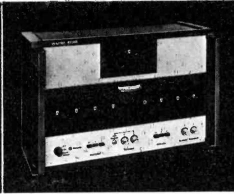
**Universal Bridge** for 0.1% measurements of any LCR combination from 2 micro-ohms to 500 gigohms. Source/detector (1592Hz) operate from a.c. or internal rechargeable battery. Sockets for external 200Hz - 20kHz. Display gives units, zeroes and decimal point. Four-terminal connections for accurate low impedance measurements.
