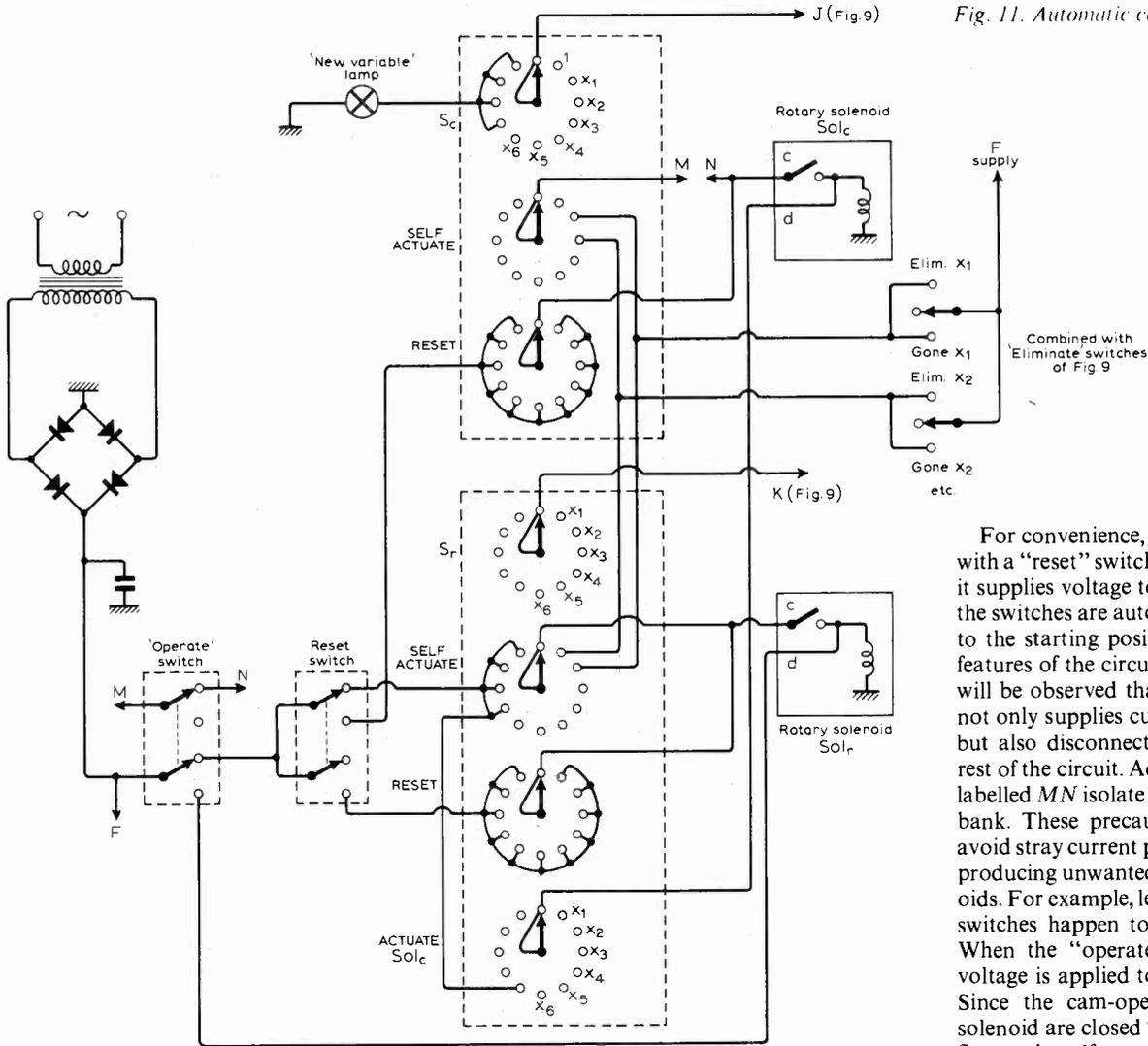
Fig. 11. Automatic control unit.
