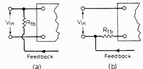
Fig. 3. General circuits for (a) parallel-injected and (b) series-injected feedback.
