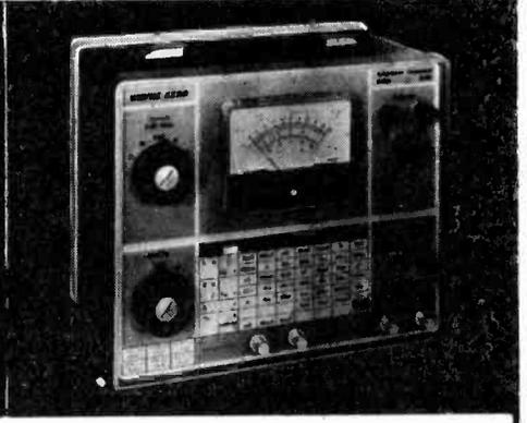
**Autobalance Component Bridge** for immediate readout of resistance, capacitance and shunt loss, inductance and series loss. C and R comparisons from -25% to +25%. Electrolytics tested with d.c. Accuracy 0.25% (R & C), 2% (L). Internal 1kHz source/detector.
