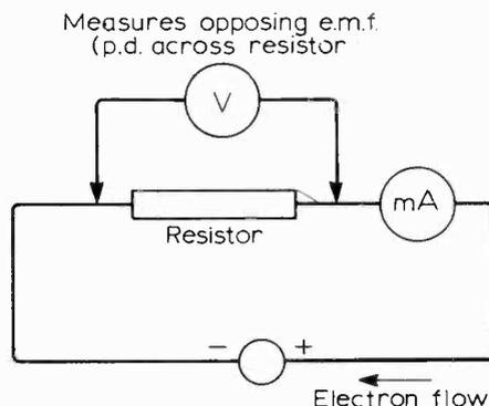
Fig. 2. Simple circuit illustrating work done by an e.m.f. source in moving electrons against resistance. The e.m.f. could be varied to form a signal.
