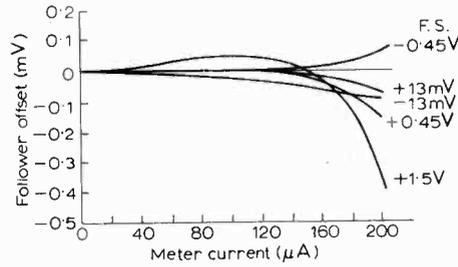
Fig. 4. Plot of offset voltage vs meter current for five scales ( $\pm 15mV$ ,  $\pm 0.5V$  and  $+ 1.5V$ ) by changing  $R_s$  shows total variation in offset is within  $0.1mV$  on  $\pm 15mV$  scales. This shows feasibility of  $\pm 5mV$  scale at  $\pm 1\%$  error.
