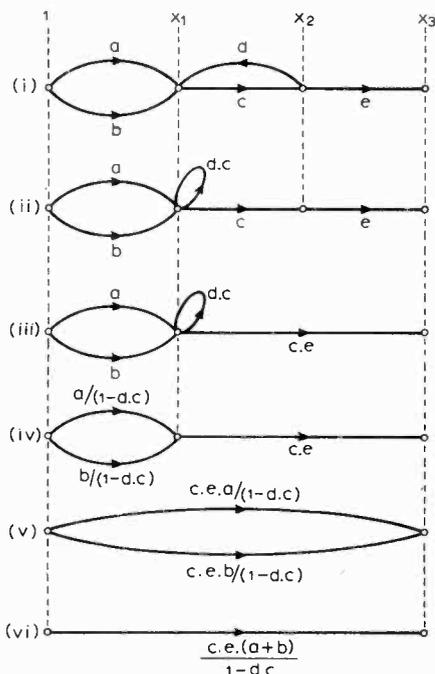
Fig. 6. Rules for feedback loops, self-loops and node elimination.
