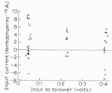
Fig. 7. Measurements of follower input current over two-week periods show input current is within  $\pm 10^{-14} A$  and that compensation reduces input current by 200.
