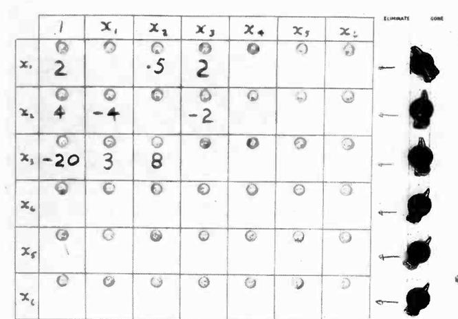
Fig. 10. Detailed view of display board set ready for solution of equations (2).
