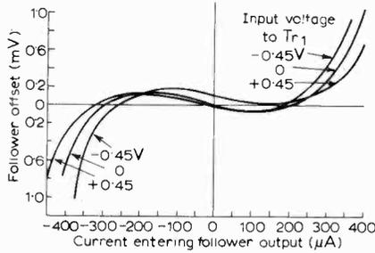
Fig. 5. Follower output characteristics for three values of input voltage. Slope of central part is altered by adjusting  $R_9$ . Curves for  $\pm 0.45V$  are moved vertically by adjusting  $Tr_1$  shunt and breadth altered by changing  $R_6, R_7$  &  $R_8$ .
