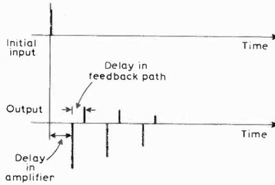
Fig. 5. Circulating pulse in feedback amplifier.
