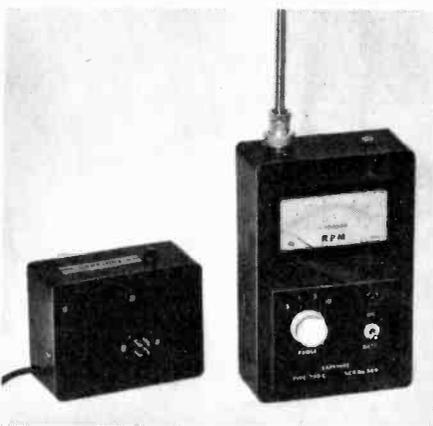
pressed zero meter for better resolution, automatic gain control and a chart recorder output. A charger unit is supplied with the tachometer, and because output voltage is low the terminals can be exposed on the charger—avoiding terminals on the hand-held unit. Price is £59. Sapphire Research & Electronics Ltd, Sapphire Works, Ferndale, Glam.
