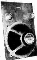
30-14,500 c.p.s., 12in. double cone, woofer and tweeter cone together with a DAKER ceramic magnet assembly having a flux density of 14,000 gauss and a total flux of 145,000 Maxwells. Bass resonance 40 c.p.s. Rated 20 watts. Voice coils available 3 or 8 or 15 ohms. Post Free.
