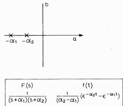
Fig. 8.  $S$ -plane with two poles on the  $-a$  axis.
