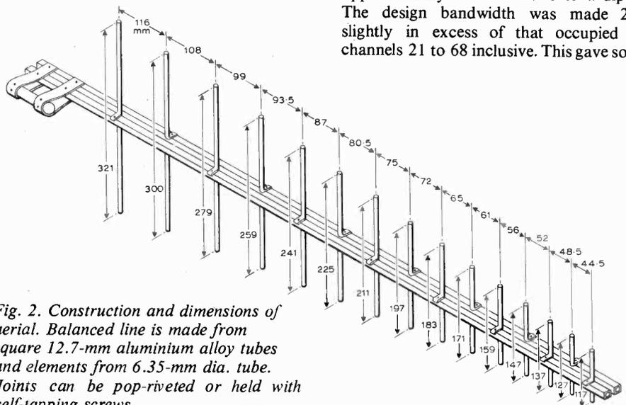
Fig. 2. Construction and dimensions of aerial. Balanced line is made from square 12.7-mm aluminium alloy tubes and elements from 6.35-mm dia. tube. Joints can be pop-riveted or held with self-tapping screws.
