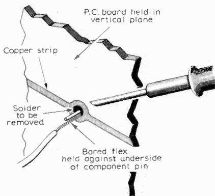
The wire "brush" used should be of reasonably new and clean multi-strand flex, such as 23 x No. 36 s.w.g. A 1 to 1½ in. end should be stripped, gently twisted, and liberally treated with flux. The tip of the iron should be clean with, obviously, a minimum of solder on its surface. More than one application, using a fresh brush each time, may be needed if there is much
