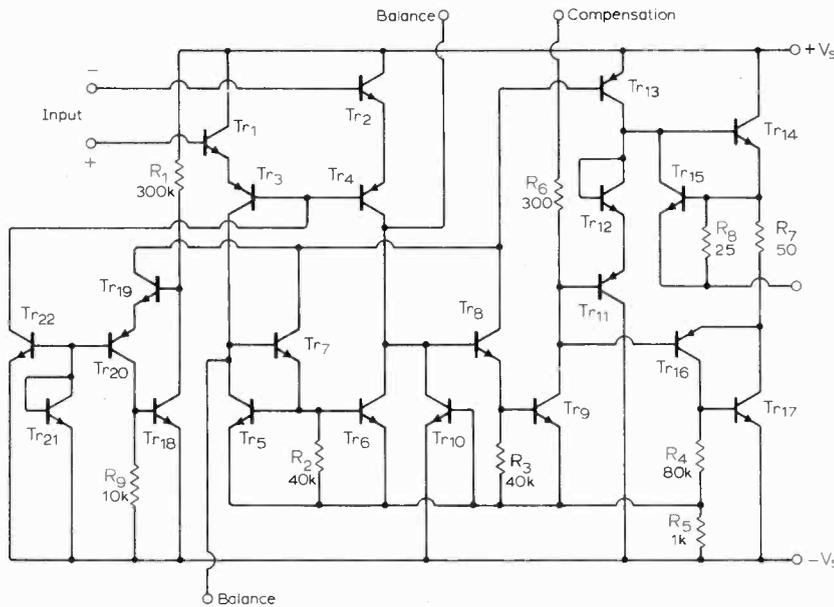
Fig. 3. An example of an improved first generation op-amp, the LM101.
