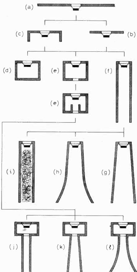
Fig. 1. The lineage of loudspeaker baffles.
