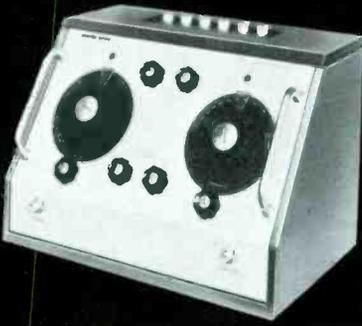
**Radio Frequency Bridge** with its Low Impedance Adaptor reads a wide range of L, C and R values at frequencies from 15kHz to 5MHz, generally to 1%. Special Adaptors, Q601 series, for measuring transistor parameters. Two or three-terminal connections, balanced or unbalanced.
