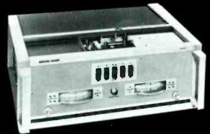
**Universal RF Bridge** measures real and quadrature terms of any immittance to 1%, without frequency dependence, from 100kHz to 10MHz. Includes standards of R, C and L. Unique magnetic potentiometers give exceptional linearity and stability.
