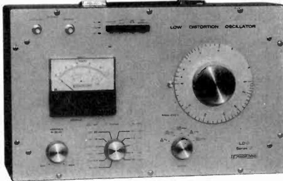
An instrument of high stability providing very pure sine waves, and square waves, in the range of 5 Hz to 500 kHz. Hybrid design using valves and semiconductors.
