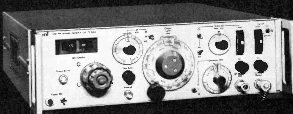
The TF 2012 is the first of 'the quiet ones' - a series of signal generators designed to embody all the features needed for the accurate evaluation of narrow band mobile FM receivers. It is a signal generator with sufficiently low sideband noise to permit - with ease - the exacting two and three signal generator tests required by the licensing authorities on advanced mobile equipment. It has extremely low microphony and its frequency
