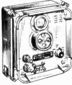
Small portable crystal controlled wavemeter. Size 7in. x 7 1/2in. x 4in. Frequency range 500 Kc/s-10 Mc/s (up to 30 Mc/s on harmonics). Calibrated dial. Power requirements 300 V.D.C. 15mA and 12 V.D.C. 0.5A. Excellent condition. £4 47 1/2. Carr. 37 1/2p.
