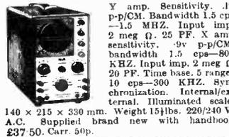
Y amp. Sensitivity. 1v p-p/CM. Bandwidth 1.5 cps-1.5 MHz. Input imp. 2 meg Ω. 25 PF. X amp sensitivity. 9v p-p/CM. bandwidth 1.5 cps-800 KHz. Input imp. 2 meg Ω. 20 PF. Time base. 5 ranges 10 cps-300 KHz. Synchronization. Internal/external. Illuminated scale. 230 x 240 v. A.C. Supplied brand new with handbook. £37 50. Carr. 50p.
