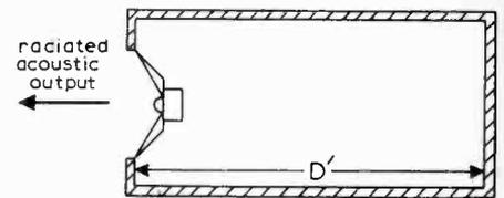
Fig. 2. Unlagged totally enclosed cabinet.
