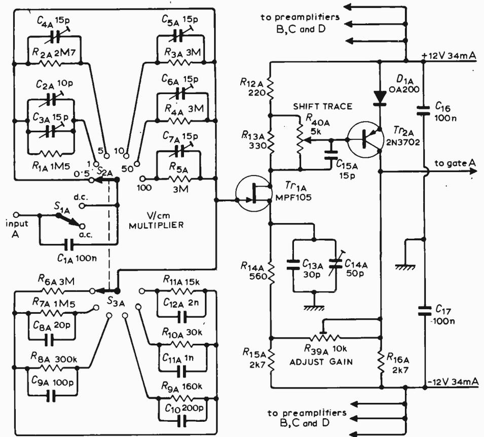
Fig. 6. One of the four input pre-amplifiers.
