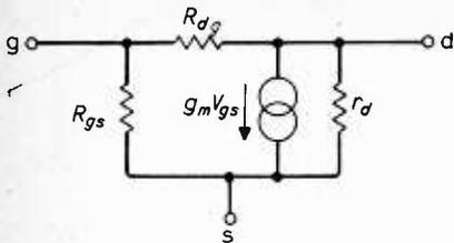
Fig. 5. For low-frequencies this equivalent circuit suffices (when junction capacitance can be ignored).
