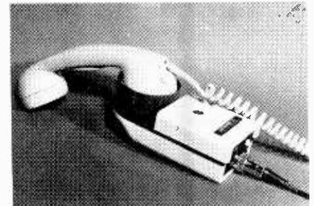
handset. The input signal frequency modulates a 1.7kHz oscillator which drives a transducer held in close proximity to the handset's microphone. At the receiving end the signal is demodulated and used to drive a chart recorder in the receiving unit.
