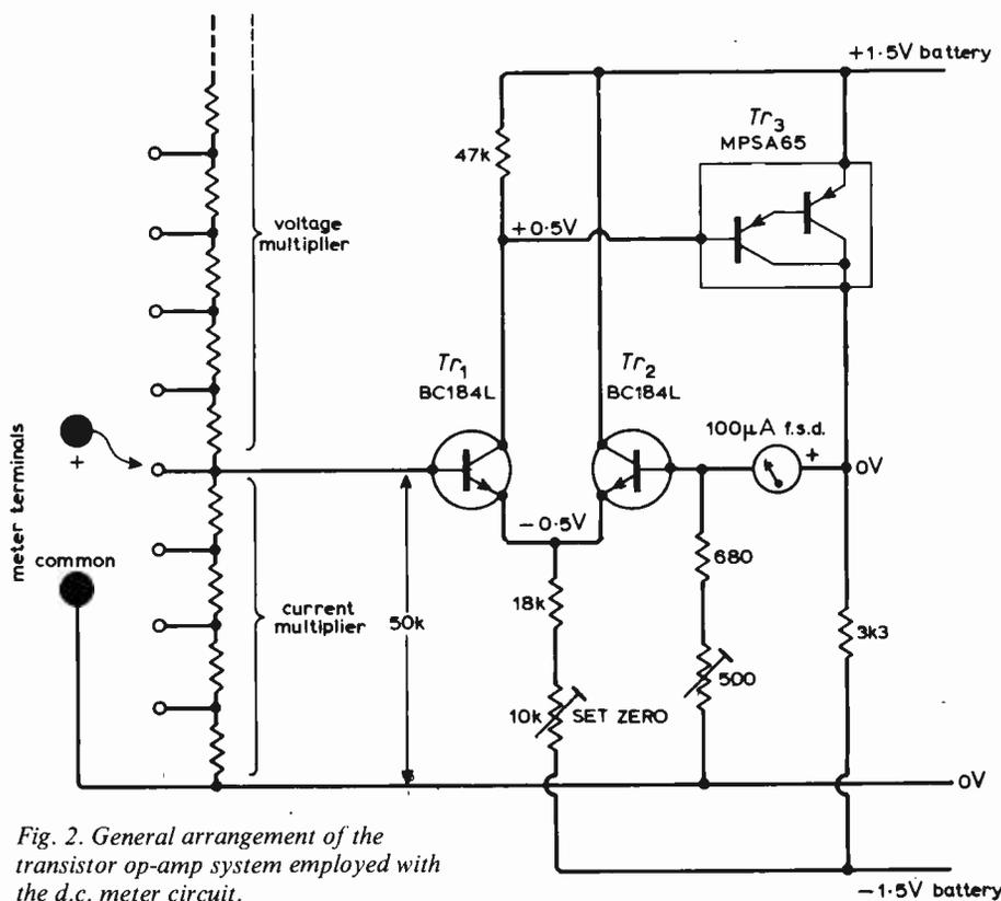
Fig. 2. General arrangement of the transistor op-amp system employed with the d.c. meter circuit.
