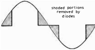
110V equipment which is not critical of waveform shape may be operated from 240V. For practical purposes, heat dissipation is nil and the diodes may be fitted inside the equipment.
