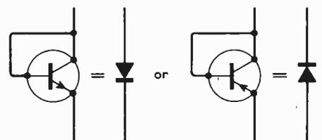
Fig. 5. The 'super diode' configuration. Typical forward voltage drop is approximately 0.52V at 100μA using any small signal silicon transistor.
