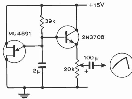
Fig. 1.2. Unijunction transistor circuit for generating test signal.
