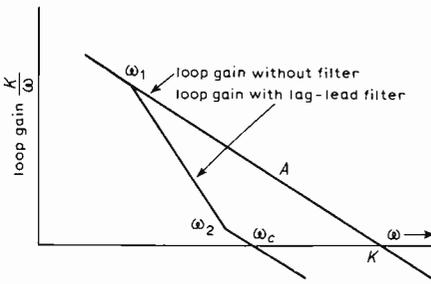
Fig. 4. Bode diagram of phase-locked loop.
