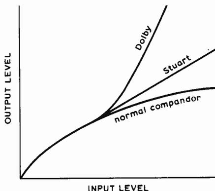
Put another way, the conventional compandor would yield the full noise reduction at a signal level  $20\text{dB}$  larger than in the author's design.
