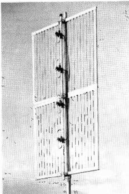
*(left) On-channel repeater aerial from J Beam Engineering for 450 to 470MHz. The aerial is for a repeater "booster" station receiving and transmitting simultaneously on the same frequency. Isolation between the two sections is better than 65dB.*
