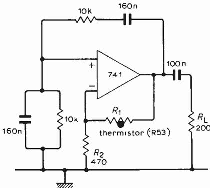
mode with the gain stabilized by a thermistor in the feedback loop. The gain of the amplifier is -
