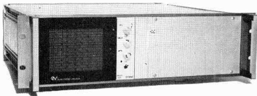
Electronic Visuals' EV8060 is a self-contained display unit providing bright, high resolution displays and is suitable for viewing high density alphanumeric or other low occupancy signals. The rectangular cathode-ray tube has a usable screen area of 10 × 8cm and is available with P31 or P7 phosphors. The d.c. coupled, X, Y and Z amplifiers with balanced inputs, are compatible with t.t.l. and d.t.l. logic levels and to obtain maximum stability, power
