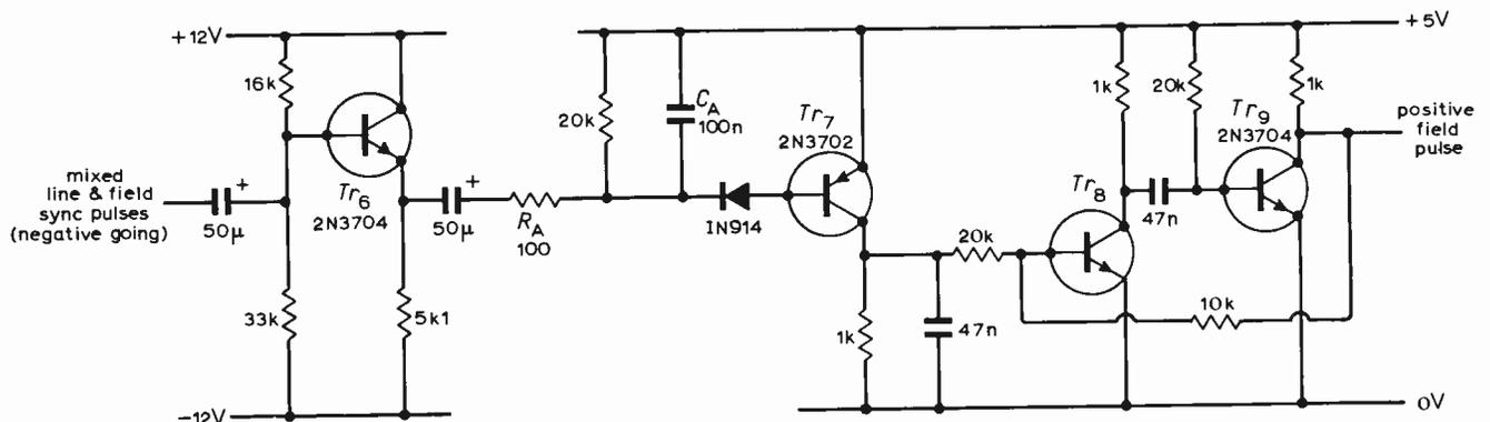
Fig. 6. Circuit for providing positive field sync pulses.
