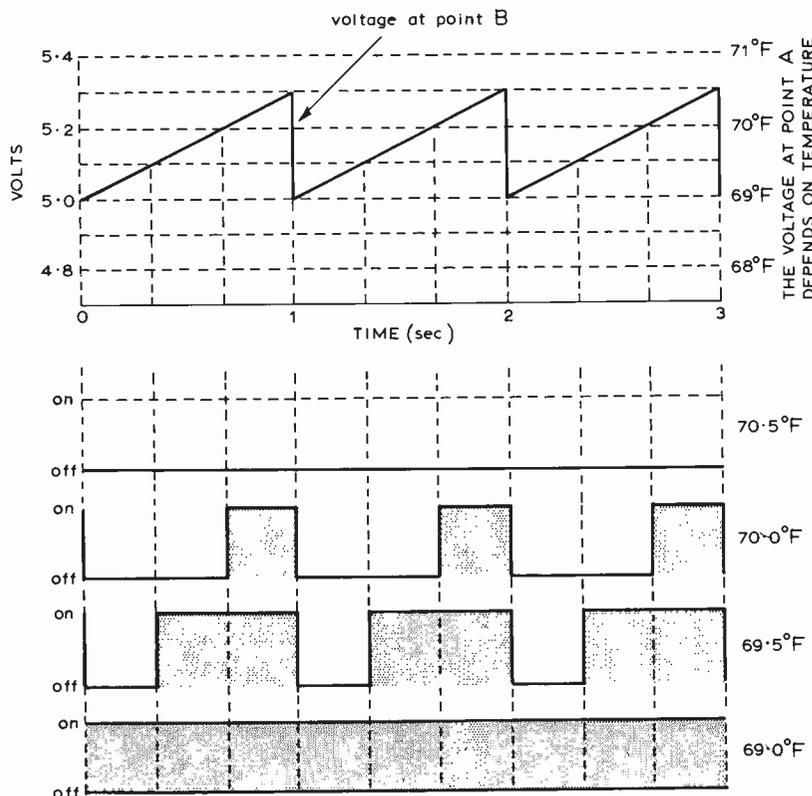
Fig. 4. Showing how a sawtooth waveform impressed on the base voltage of  $Tr_6$  allows proportional control of the heater to be obtained.
