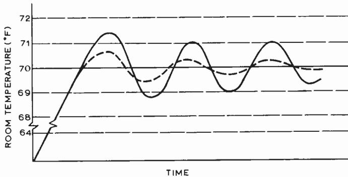
Fig. 3. A comparison of the performance of the thermostat and thermistor controlled circuits of Figs 1 and 2.
