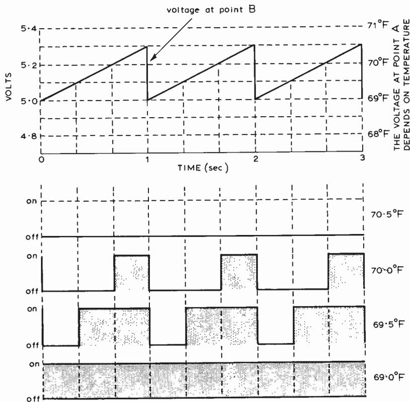
Fig. 4. Showing how a sawtooth waveform impressed on the base voltage of Tr<sub>6</sub> allows proportional control of the heater to be obtained.
