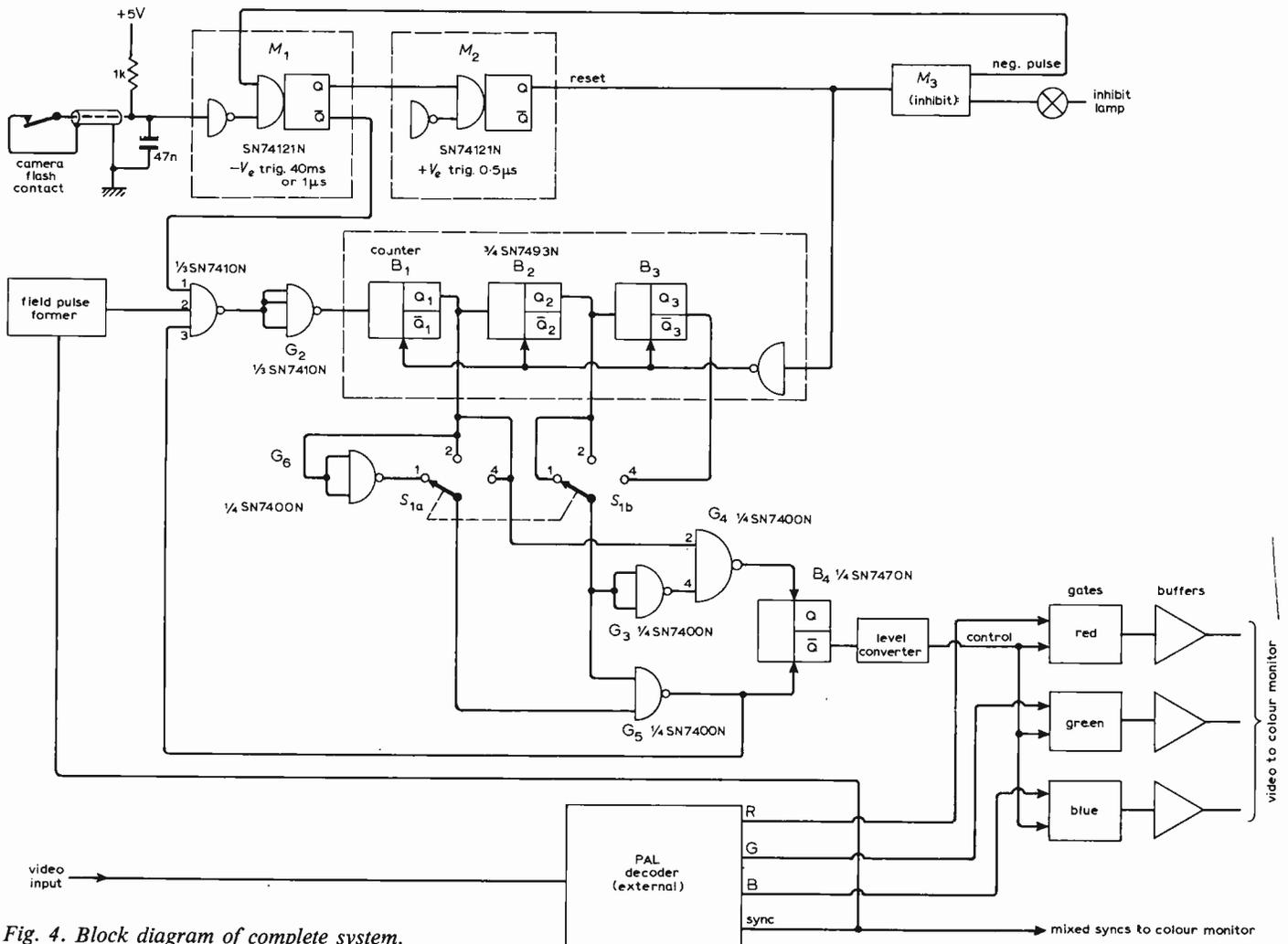
Fig. 4. Block diagram of complete system.
