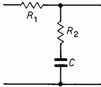
Fig. 5. Lag-lead filter.
