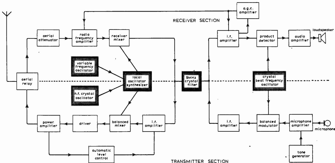
Fig. 1. Transceiver block diagram. The shaded areas are common to transmit and receive.
