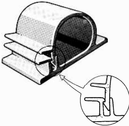
cable runs. Six sizes are available with internal diameters of 4.8, 6.5, 9.5, 12.5, 16 and 19mm.
