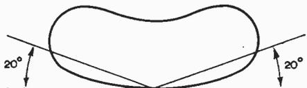
Fig. 1. Polar diagram of the aerial.
