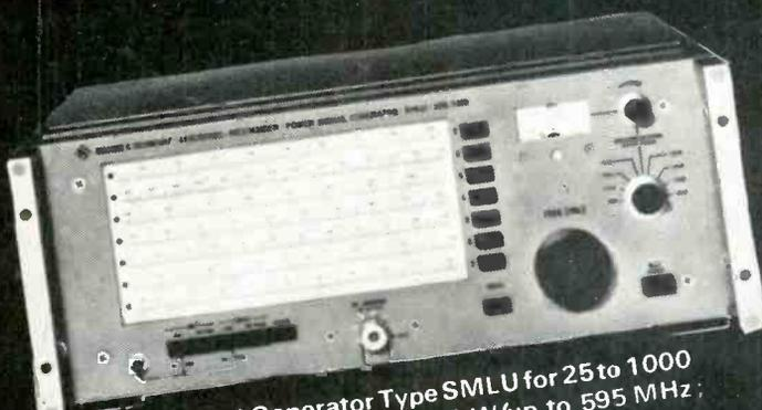
Power Signal Generator Type SMLU for 25 to 1000 MHz. Output level with ALC 2 W (up to 595 MHz; from 565-MHz range) 1 W.
