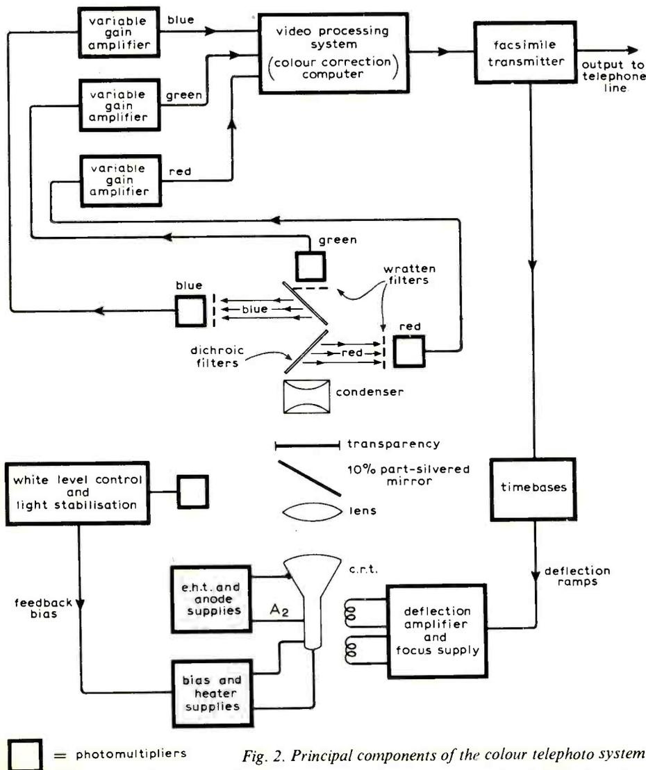
Fig. 2. Principal components of the colour telephoto system.
