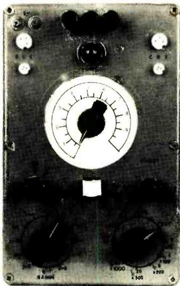
A general view of the prototype tester. In the centre is the  $h_{FE}$  dial. The range switch is bottom left and emitter current selector, bottom right.
