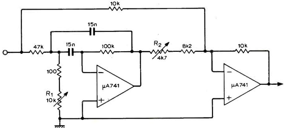
the filter tunes from 170Hz to 3kHz, a bandwidth between 3dB points of 230Hz and a notch rejection of better than 40dB over the complete range. A voltage-tuned notch filter may be realised by replacing
