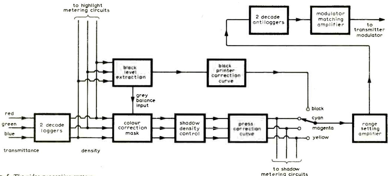
Fig. 5. The video processing system.
