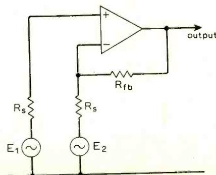
resistors ( $R_S$ ) of the appropriate value to optimize the input noise characteristics, the output noise of the amplifier will be the same whichever of the two generators we assume to be providing the zero input.
