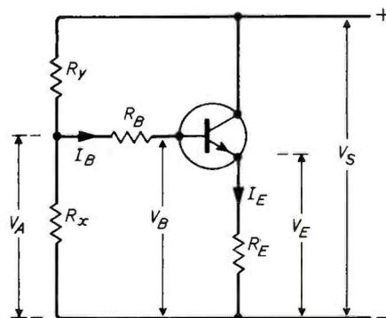
Fig. 2. The common collector configuration.
