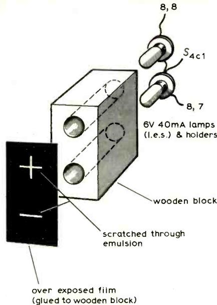
Fig 2. Polarity indicator construction.
