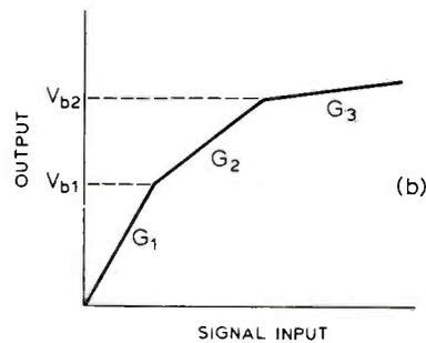
Fig. 7. (a) Circuit for producing a convex transfer function; (b) output/input characteristic of the circuit.
