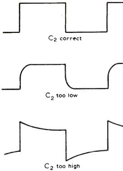
Fig 6. Setting frequency response using a square wave.
