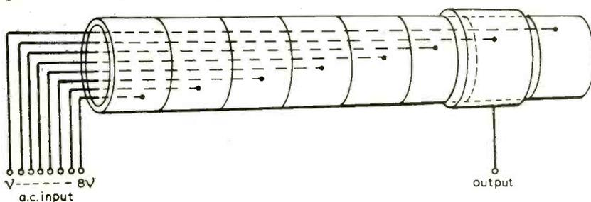
Fig. 7 Rank Precision capacitive displacement transducer.
