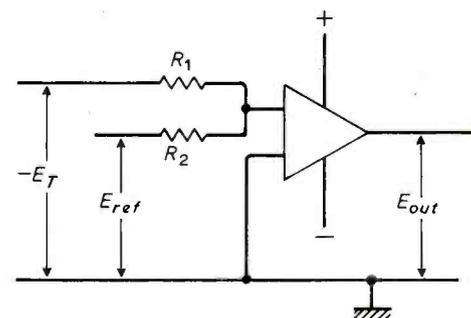
Fig. 3. Voltage comparator.
