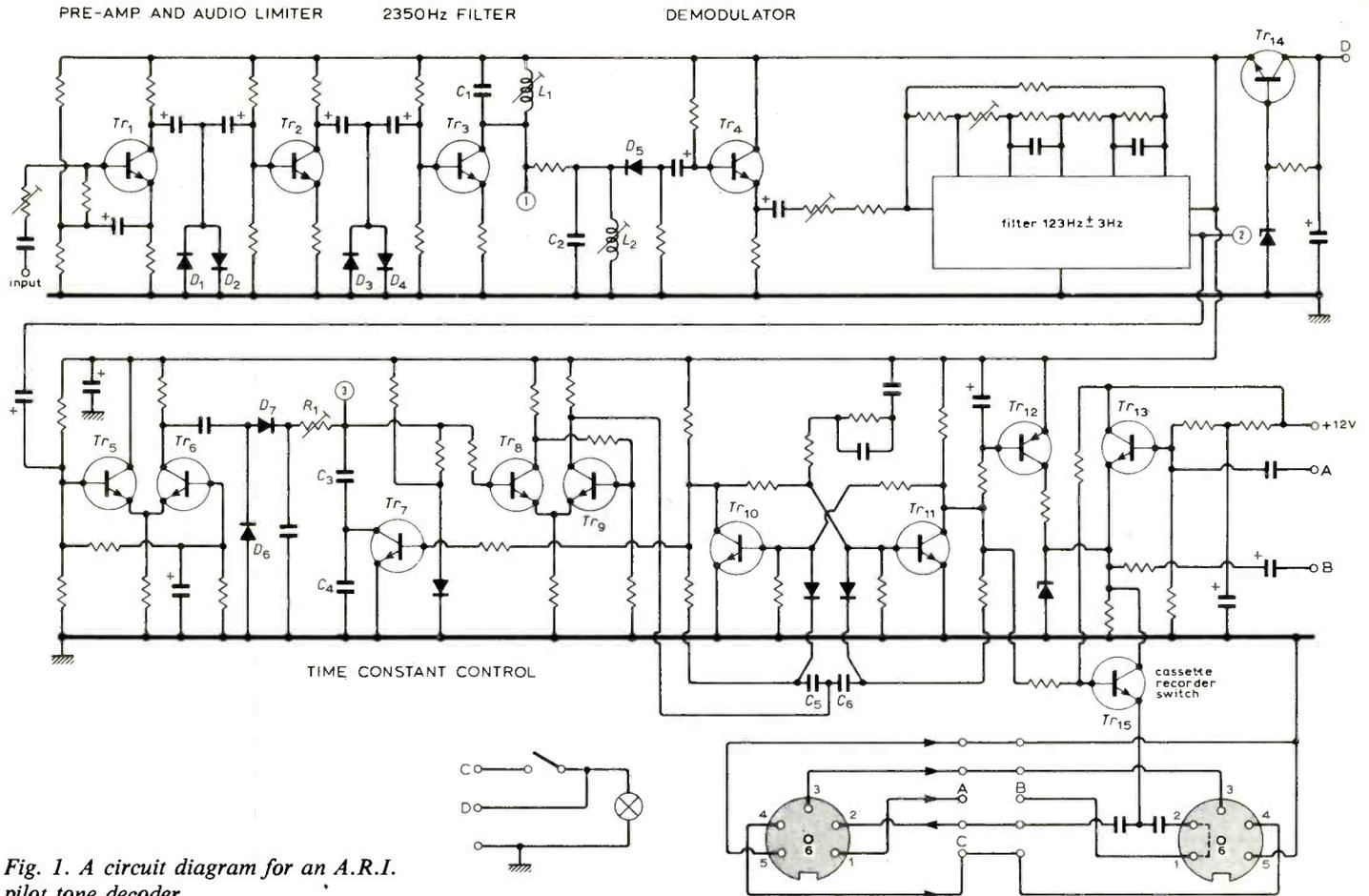
Fig. 1. A circuit diagram for an A.R.I. pilot tone decoder.
