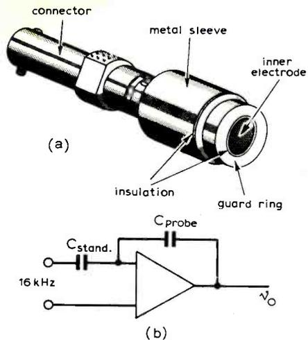
Fig. 8 Wayne Kerr capacitive probe system.
