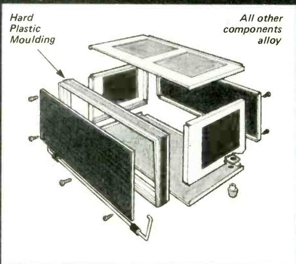
CODE NO: 300900 Height 120mm Length 284mm Depth 138mm
