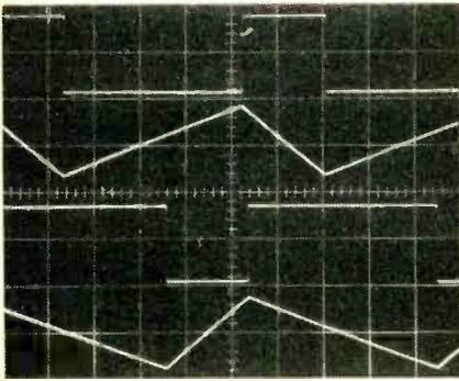
Fig. 9.4. Waveforms for free-running multivibrator (Fig. 9.3) with pulse width control. Traces show output voltage (10V/div.) and voltage at pin 2 (0.2V/div.) for  $V_{in}$  of +5V and -5V respectively. Horizontal scale, 2ms/div.
