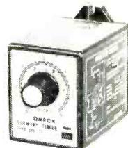
Only OMRON could provide a timer of such unrivalled superiority over all its competitors, anywhere in the world. The STPNH is a synchronous motor driven timer with automatic reset function. Both instantaneous and time limit contacts are fitted and the timer is mounted on an international 8 pin octal base. Time ranges start 0.6 secs and finish 0-28hrs with operating voltage at 110VAC or 240VAC.
