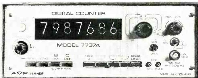
*Digital counter model 7737A manufactured by AMF Venner. This is a seven-digit counter/timer suitable for frequency measurements up to 100MHz.*
