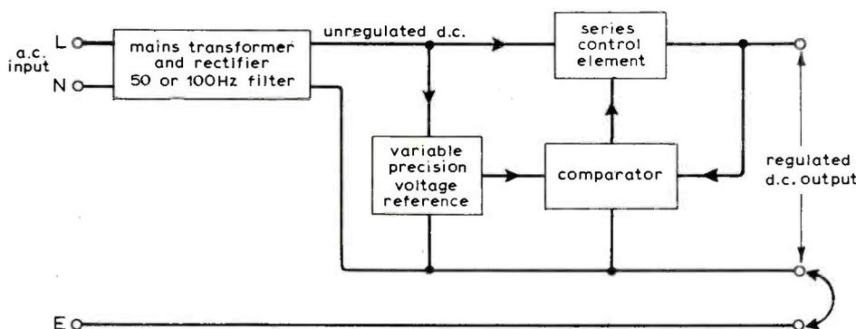
Fig. 1. Series regulator block diagram.
