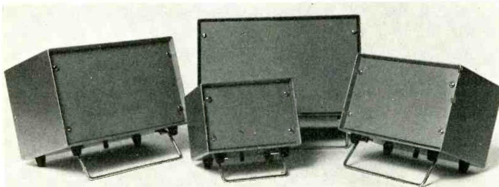
Cases made from 20swg. zinc coated m/s. Front & rear panels 16swg. aluminium. Cases finished in Olive green hamertone with front panels in light straw shade 384. All cases fitted with ventilated rear panels and a very attractive chrome plated retractable leg can be fitted as an optional extra.
