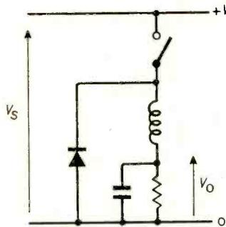
Fig. 1. In trying to achieve a current constant against variations in supply voltage, load resistance, ambient temperature, and component parameters an intermediate step is sometimes used where power is switched before reconversion to d.c.
