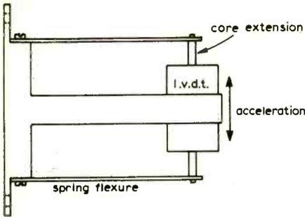
Fig. 3 The l.v.d.t. in an accelerometer application.
