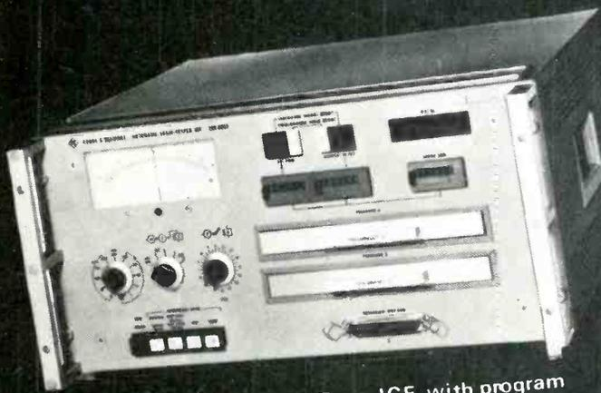
Automatic Logic Tester Type ICF with program input via punched cards and tapes.
