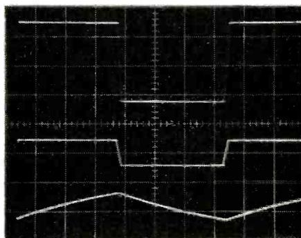
Fig. 9.2. Free-running multivibrator waveforms: upper trace, pin 6; middle trace, pin 3; lower trace, pin 2. Vertical scale, 10V/div.; horizontal scale, 0.2ms/div.
