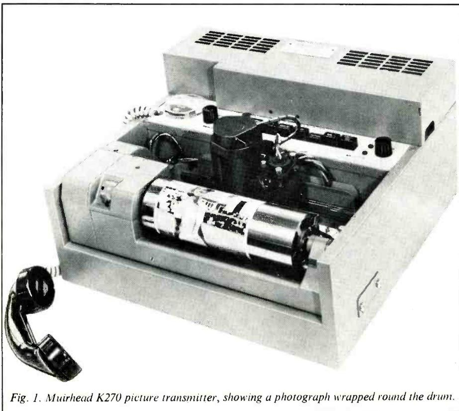
Fig. 1. Muirhead K270 picture transmitter, showing a photograph wrapped round the drum.
