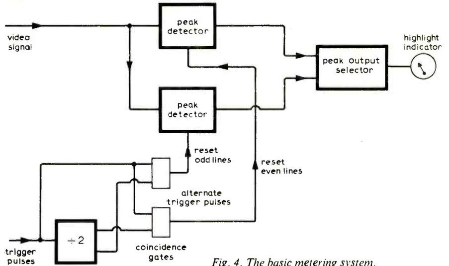
Fig. 4. The basic metering system.
