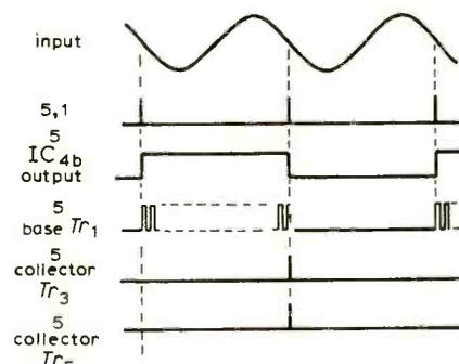
Fig 5. Period meter waveforms.
