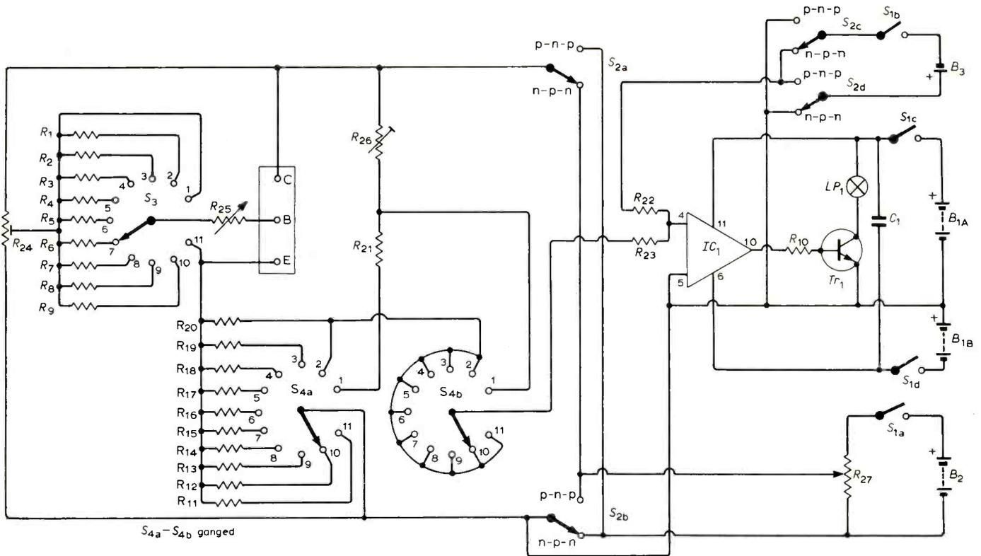
Fig. 4. Circuit diagram of tester.
