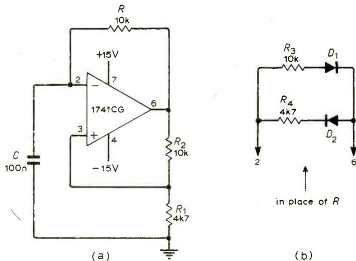
Fig. 9.1(a). Free-running multivibrator; (b) alternative timing resistors.
