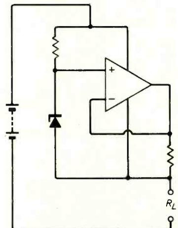
Fig. 4. Current control can also be achieved by using Fig. 3 as a two-terminal circuit between source and load.
