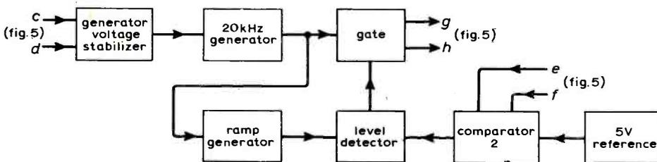
Fig. 6. Block diagram of the inverter control module.
