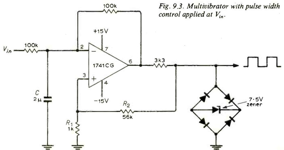
Fig. 9.3. Multivibrator with pulse width control applied at  $V_{in}$ .
