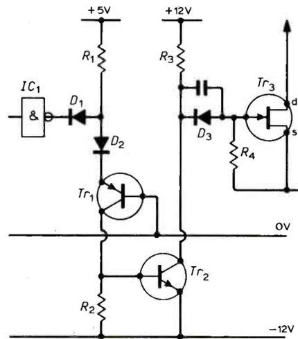
Fig. 11. Method of driving f.e.t. switches from 5V lines.
