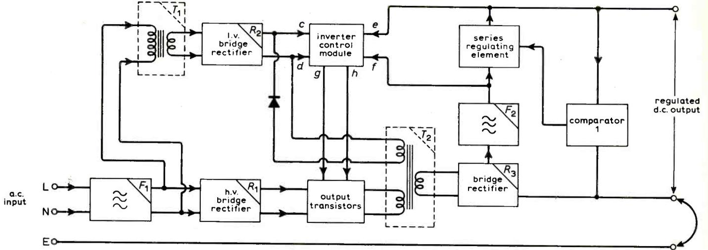
Fig. 5. Block diagram of the combined switching and series regulator.
