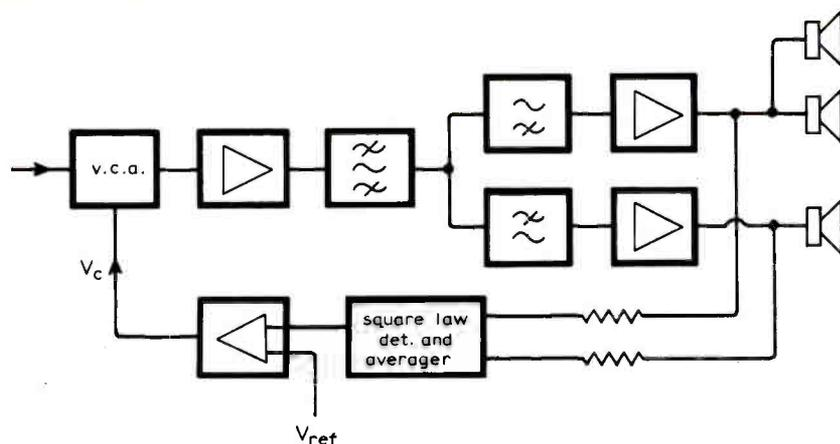
Voice-coil protection circuit in KEF speaker, model 5/1AC, uses voltage-controlled attenuator that is actuated when the mean power over 5 seconds reaches an unsafe level, as set by  $V_{ref}$ .
