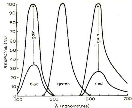
Fig. 3. Spectral distributions of the three channels.
