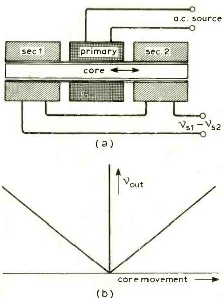
Fig. 1(a) Sectional drawing of l.v.d.t.
