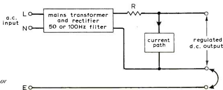
Fig. 2. Shunt regulator block diagram.
