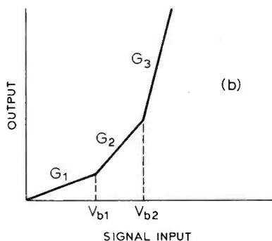
Fig. 6. (a) Circuit for producing a concave transfer function; (b) output/input characteristic of the circuit.
