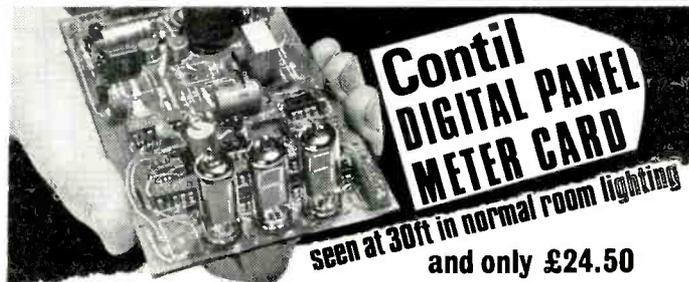
The Contil DPM is a complete instrument built on a single board with the DEM in mind. Believed to be the lowest cost 2½ digit DPM available, it requires only a 5V supply to operate.
