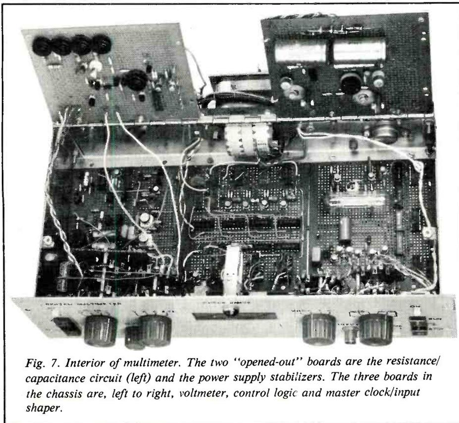
Fig. 7. Interior of multimeter. The two "opened-out" boards are the resistance/capacitance circuit (left) and the power supply stabilizers. The three boards in the chassis are, left to right, voltmeter, control logic and master clock/input shaper.
