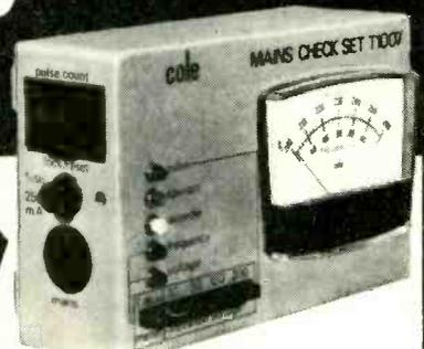
Ideal for installation, maintenance, and the laboratory, the T1007 measures supply voltages from 200 volts to 260 volts A.C., and frequencies from 35Hz to 65Hz. An electromechanical counter records the incidence of interference pulses occurring above threshold levels selectable from 10v to 200v. Provision is made for the connection of a recorder for external monitoring. A 100 volt to 130 volt A.C. range model is also available.
