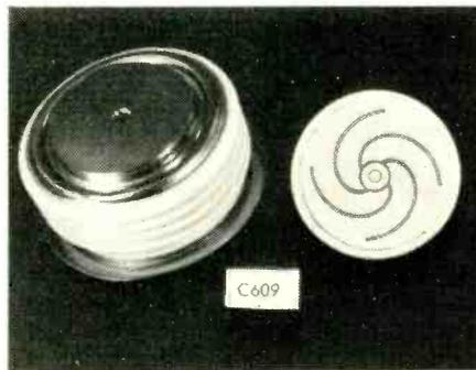
*The C609 inverter thyristor from General Electric, rated at 1kHz and 1200A. The involuted cathode structure permits a rating of 850A at 5kHz, long-term di/dt of 500A/microsecond and minimum dv/dt of 400V/microsecond.*
