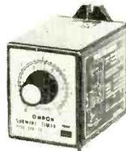
Only OMRON could provide a timer of such unrivalled superiority over all its competitors, anywhere in the world. The STPNH is a synchronous motor driven timer with automatic reset function. Both instantaneous and time limit contacts are fitted and the timer is mounted on an international 8 pin octal base. Time ranges start 0.6 secs and finish 0-28hrs with operating voltage at 110VAC or 240VAC.
