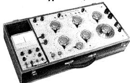
With **Electronic Null Detector Five Dials and Slidewire High Resolution Low Wattage Dissipation** Accuracy ± 0.01%
