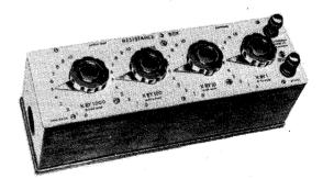
A range of robust resistance decades for use in AC or DC networks and measuring systems. They all incorporate the "CROPICO" type SP1 low contact resistance switch and the coils are wound in "Manganin". Standard models are available from stock with 1, 4, 5 or 6 dials.
