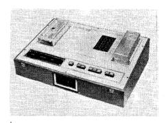
up to 64 ways on the edge connector. Programming is by patch-panel for experimental testing or short production runs. A pre-wired matrix plug is used for longer test runs. Wayne Kerr Co Ltd, Durban Road, Bognor Regis, Sussex PO22 9RL.
