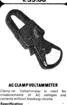
Measurement ranges:—Current 10-25-100-250-500 Amps. Voltage 300, 600 V. Accuracy 4%. Scale length 60mm. Overall dimensions 283x94x36mm. Weight 1.5 lbs.
