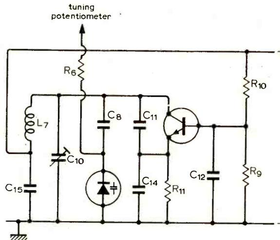
Fig. 8 From this redraw of Fig. 7 it is clear that the circuit is that of a Colpitts oscillator.
