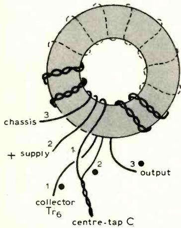
Fig. 3. Construction of the broadband output transformer for Tr<sub>6</sub>.
