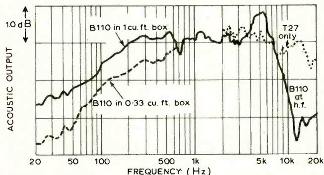
Fig. 1. For the common-bass system the mid and upper-ranges use B110 and T27 drive units, as in the original design. Graph shows axial response of B110 in a 1-cu.ft sealed box (upper solid line). T27 curve (broken line) shows an upper crossover of about 4kHz is suitable. Lower B110 curve shows axial response for a small, 0.33-cu.ft sealed box, for which slope correction is needed (see Fig. 5). Acoustic response curves taken with a writing speed of 80mm/s and a paper speed of 3mm/s.
