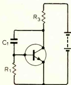
Fig. 13 The Miller integrator circuit.
