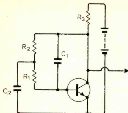
Fig. 12 A redraw of Fig. 10 with  $R_3$  in the collector circuit.
