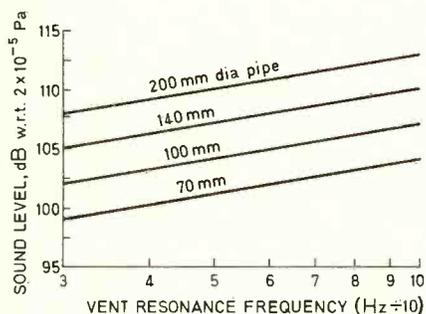
Fig. 7. Minimum programme sound levels in room of 2000ft<sup>3</sup> (60m<sup>3</sup>) for various diameter long pipes and vent resonance frequencies before distortion is appreciable.
