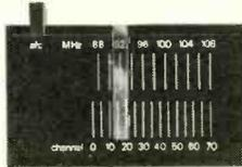
Size 85×50×20mm (3½×2×¾ ins.). Tunes 87.5 to 108MHz. DETECTOR – I.C balanced coincidence (I.C equivalent to 26 transistors) Distortion – 0.2% at 1KHz for 30% modulation. SENSITIVITY – 5 microvolts for 30dB quieting. Output – 300mV for 30% modulation. Aerial imp. – 75 Ω or 240-300 Ω. Dual Varicap tuning. 4 pole ceramic filter. Switchable A.F.C. Operating power 23-30 volts.
