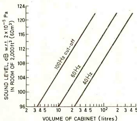
**Fig. 1. Relation between Sound Pressure Level for 3% of second harmonic distortion in room of 2000ft<sup>3</sup> (60m<sup>3</sup>) and volume of closed cabinet, assuming various lower cut off frequencies and isothermal conditions.**
