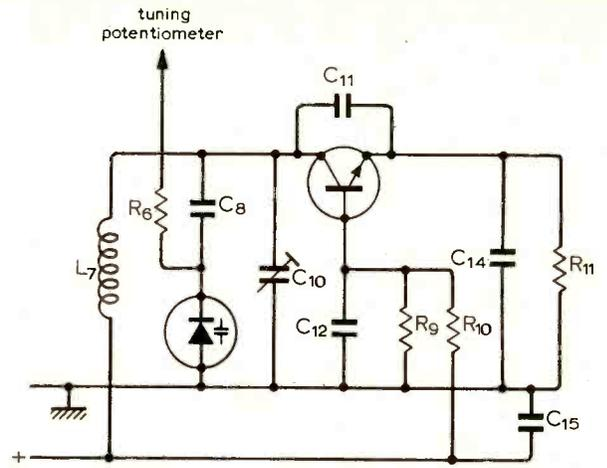
Fig. 7 Circuit diagram of a stage in an f.m. receiver.
