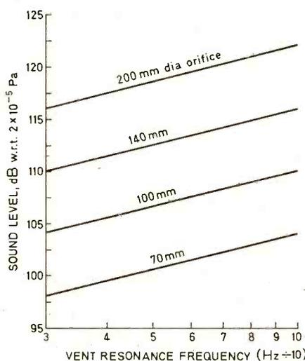
Fig. 3. Minimum programme sound level in room of 2000ft<sup>3</sup> (60m<sup>3</sup>) for various size orifices and vent resonance frequencies before nonlinearity is appreciable from orifice.
