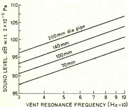
Fig. 6. Minimum pure-tone sound levels at vent resonance frequency in room of 2000ft<sup>3</sup> (60m<sup>3</sup>) for various diameter long pipes and vent resonance frequencies before distortion is appreciable.
