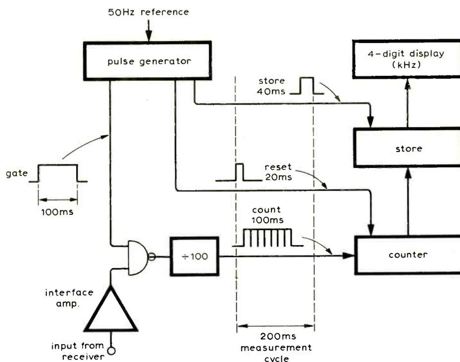
Fig. 1. Basic diagram of frequency meter operation.
