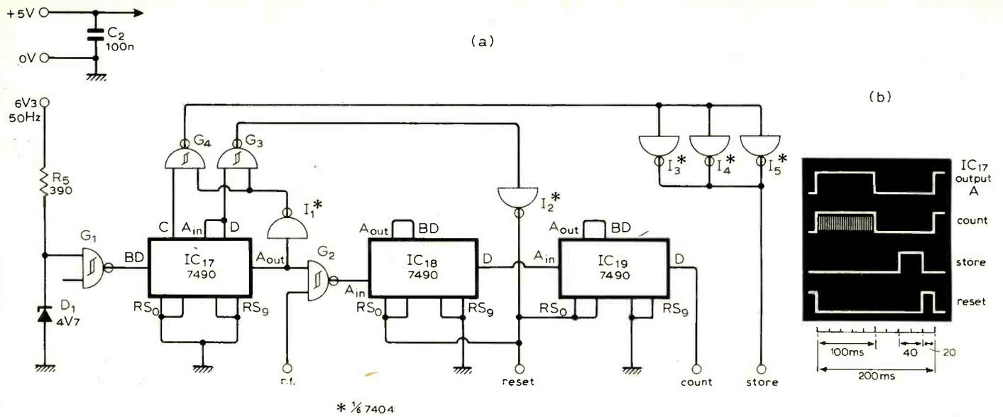
Fig. 4(a). Pulse generator circuit. The four Schmitt gates were 7414 in the prototype, but as they are rather difficult to obtain it is suggested that 7413 + 7440 be used in its place (7413 in  $G_1$  and  $G_2$  positions). A timing diagram for the unit is shown at (b).
