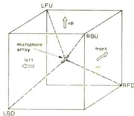
Fig. 4. Microphone aiming directions for four-channel, three-dimensional surround-sound pickup.
