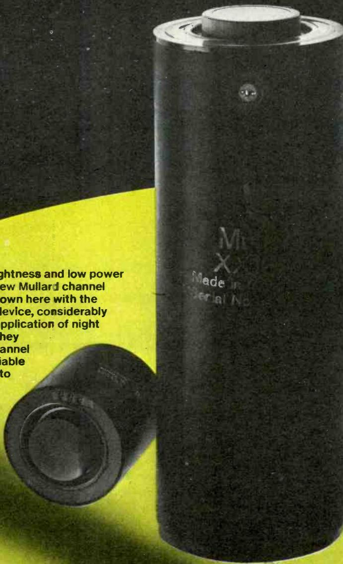
Resistance to highlight overload and ease of gain control give them particular application in low light level television systems as well as direct view equipment.
