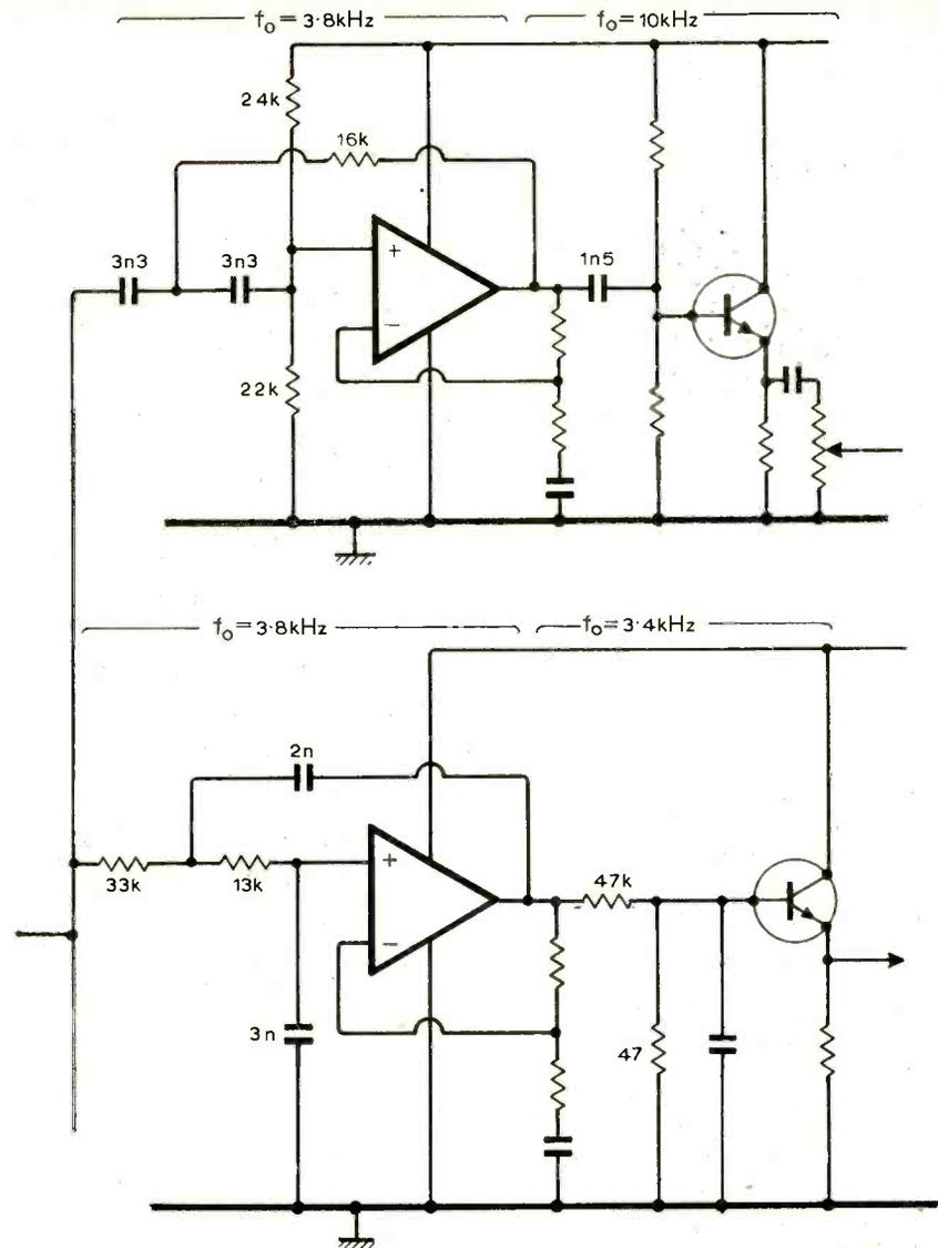
Fig. 9. Original active crossover design (December) can be improved by lowering upper crossover frequency to 4kHz. New component values shown above.
