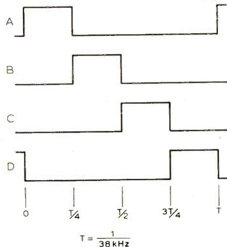
Fig. 7. Switching functions used to sample the four audio signals.
