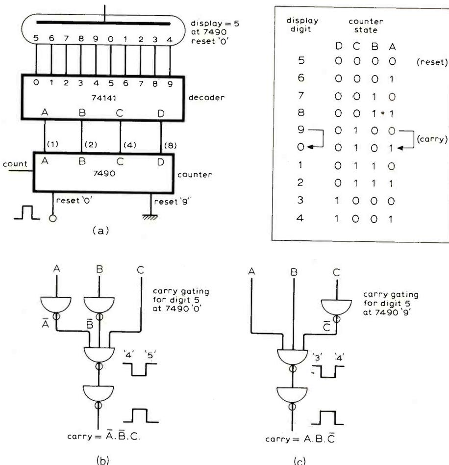
Fig. 2(a). A typical counter, decoder and display, showing the "crossed" connexions between decoder and display. "Carry" to the next decade is enabled by the circuits of (b) and (c) for resets to "0" or "9".
