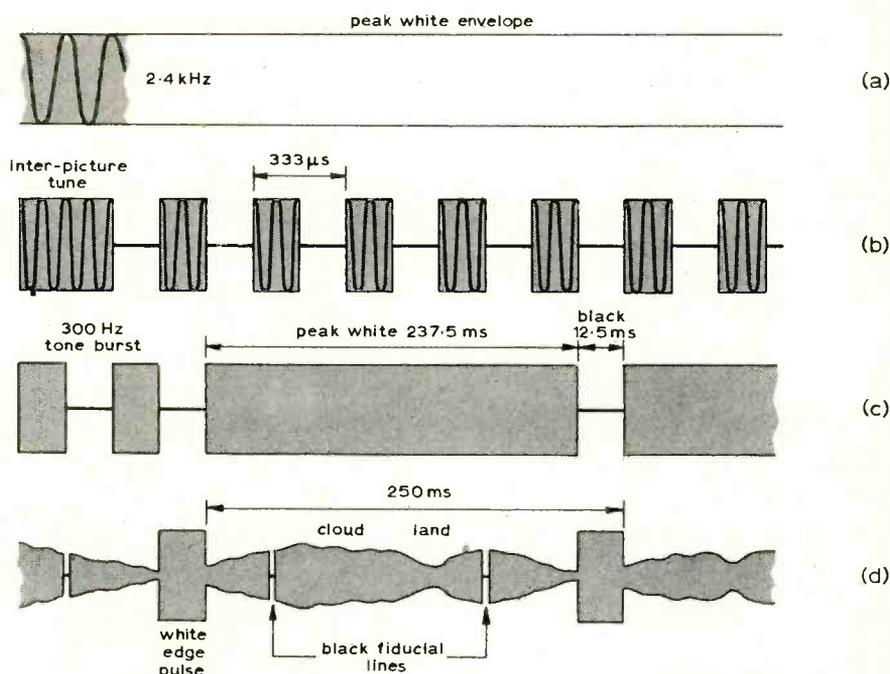
Fig. 1. ESSA-8 telemetry waveform sequence (APT), (a) peak white inter-picture tone, (b) three-second 300Hz tone burst, (c) five-second white/black phasing signal, (d) typical picture line.
