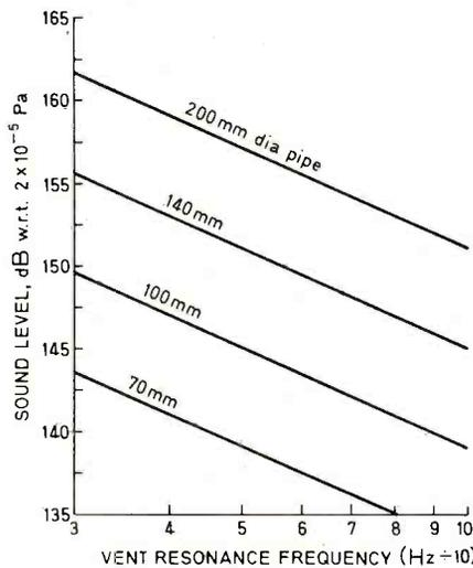
Fig. 5. Minimum pure-tone sound levels at vent resonance frequency in room of 2000ft<sup>3</sup> (60m<sup>3</sup>) from vent pipes of 100mm length and various diameters for 3% second harmonic distortion.
