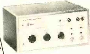
9Kc/s to 100Mc/s continuously variable. Accuracy ± 4%. ± 1% F.S. MAIN OUTPUT 20mV-1V into 50 ohm external termination continuously variable. Accuracy ± 5%. Maximum output on open circuit 2V. RISE TIME less than 1ns up to 500mV. TRIGGER OUTPUT 0.2 0.4 1.0 2.0V into 50 ohm external termination maximum output on open circuit 4V. Rise time nominally 1.5ns. Fall time nominally 3.5ns. Size: 11 in W, 5 1/2 in H, 9 in D. Wt: 7.1 lb. **LAST LISTED PRICE £95**
