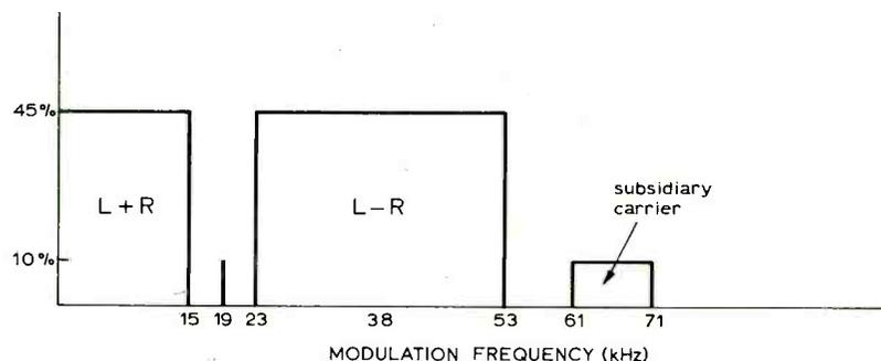
Fig. 1. Present allocation of the modulation spectrum showing the positions of the monophonic signal, difference signal and "storecast" channel.
