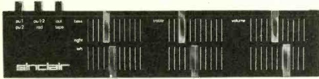
260×50×20mm (10½×2×¾ ins.) separate slider controls on each channel for treble, bass and volume. INPUTS – Mag. P.U 3mV (RIAA corrected) ceramic – 300mV, Radio 100mV, Tape 30mV. S/N ratio 60dB. Frequency range – 20Hz to 15KHz ±1dB. OUTPUTS – 2.5V rms max (30V. supply) and tape plus AB monitoring. PRESS BUTTONS for P.U., Radio and Tape. Operating power – 20 to 35V. Black case with white indications.
