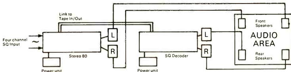
The output from any good stereo cartridge feeds into Stereo 80 and passes via the tape outlet to the 805SQ decoder. Here the signal is separated into its constituent 4 channels, those for the front being accepted by the Stereo 80, those for the rear going from the decoder to the two additional power amplifiers and speakers.
