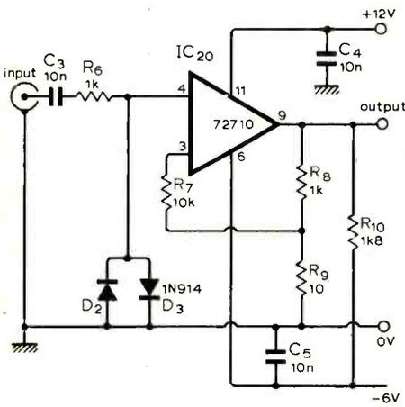
Fig. 5. Circuit diagram of the interface amplifier.
