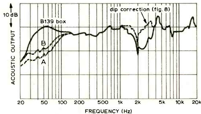
Fig. 6. Filter response for small enclosure, using values of Fig. 5 (a). Curves A and B are obtained with high-pass part of band-pass filter removed (by taking output from  $Tr_4$  emitter) and apply for an inexpensive system using only the 0.33-cu.ft enclosures (see Fig. 7).
