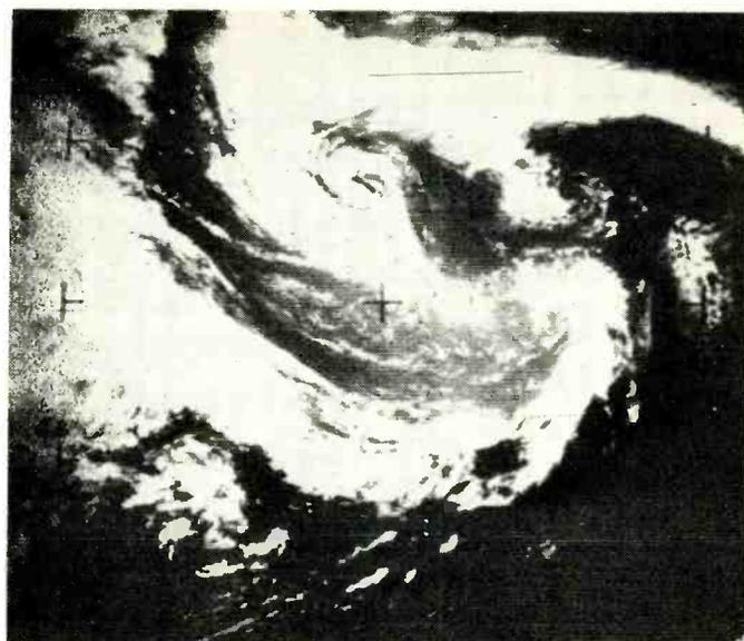
*ESSA-8 (1968-114-A): Orbit 25294 22 June 12.08Z. Weather system to west of Spain: N.W. coast of Spain is on right-hand border. Portion of complete satellite picture, produced on first run of prototype facsimile machine by G. R. Kennedy on 25.6.74. Paper Kodak WSG bromide, single weight, no. 2 (normal). Crater tube white current 7mA, black current 30mA. Brightness pot 9.00. Traverse jitter and drum vibration evident on print No. 6.*
