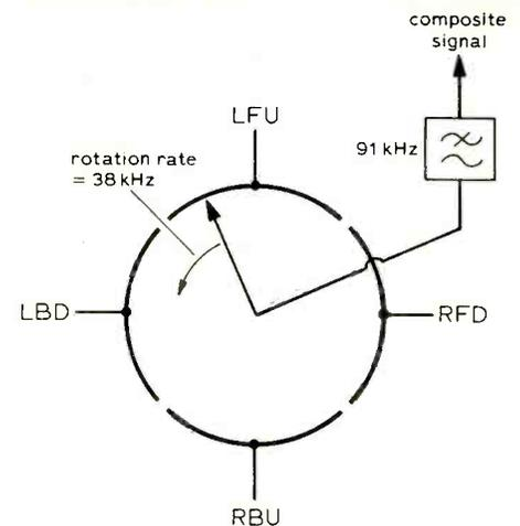
Fig. 5. Schematic showing principle of sampling four signals sequentially to produce a composite signal.
