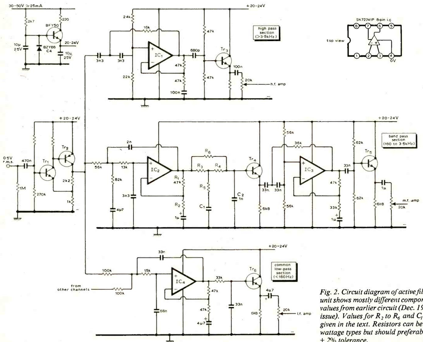
Fig. 2. Circuit diagram of active filter unit shows mostly different component values from earlier circuit (Dec. 1973 issue). Values for  $R_2$  to  $R_6$  and  $C_1$  are given in the text. Resistors can be low-wattage types but should preferably be  $\pm 2\%$  tolerance.
