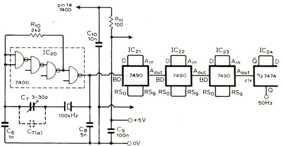
Fig. 6. Crystal reference oscillator circuit. The value of  $C_{7(a)}$  will depend on the crystal used.
