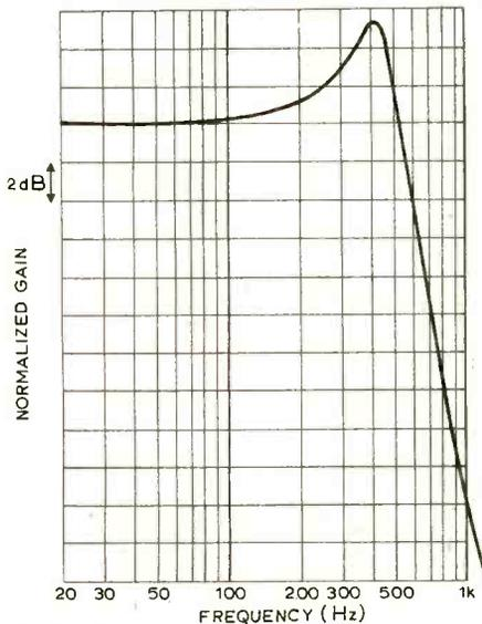
Fig. 8. Peak of appropriate height to compensate dip in Fig. 7 obtains for  $R_2=27k\Omega$ , with  $R_1=47k\Omega$  in  $IC_2$  circuit.
