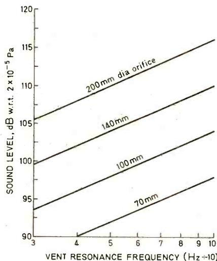
Fig. 2. Minimum pure-tone sound levels at vent resonance frequency in room of 2000ft<sup>3</sup> (60m<sup>3</sup>) for various size orifices and vent resonance frequencies before nonlinearity is appreciable from orifice.
