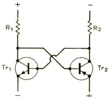
Fig. 6 A redraw of the circuit diagram of Fig. 5: in this form it is clearly a multivibrator.
