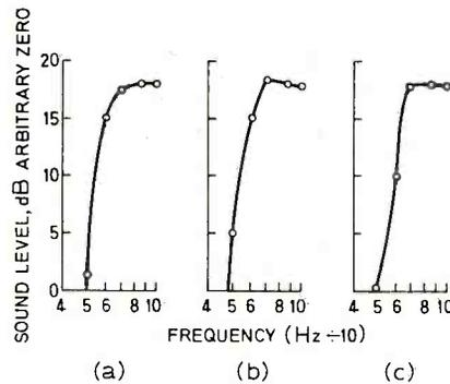
Fig. 4. Level of fundamental tone for 3% third harmonic distortion from miniature loudspeaker fitted with various vents. (a) pipe diameter 18mm, (b) pipe diameter 25mm, (c) orifice 18mm, pipe diameter 25mm.
