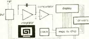
This state-of-the-art MOS LSI chip contains all the logic necessary for a 3 1/2 decade, dual slope integrating, automatic polarity detecting DVM. Supplied with free data and circuit booklet. AY-5-3507
