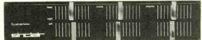
Size 260×50×20mm, matching Stereo 80 in style. Connects with tape socket on stereo 80 or similar facility on any stereo amplifier. Frequency response 15Hz to 25KHz ±3dB. Distortion 0.1%. S/N ratio 58dB. Rated Output – 100mV. Separate bass and treble slider controls on each channel, also volume. Phase shift network 90° ±10°, 100Hz to 10KHz. Operating power – 22-35V.
