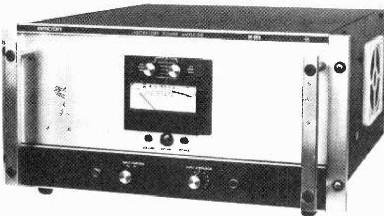
Coupling two M600s together through a socket provided at the back of each amplifier produces a 140 Volt balanced output. This configuration is called an M2000, and produces 2 kilowatts into an 8 ohm load. A peak catching meter, and threshold lights provide convenient front panel output monitoring.
