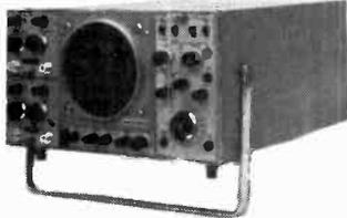
Portable Double Beam Oscilloscope Solartron Type CD 1400. DC-15MHz. Sensitivity 100 uV/cm with the following Plug-ins available CX 1441 Wide Band Amp. CX 1442 High Gain D.C. Diff. Amp. CX 1443 General Purpose Time Base Unit. CX 1444 Sweep Delay Time Base **£160-£180**
