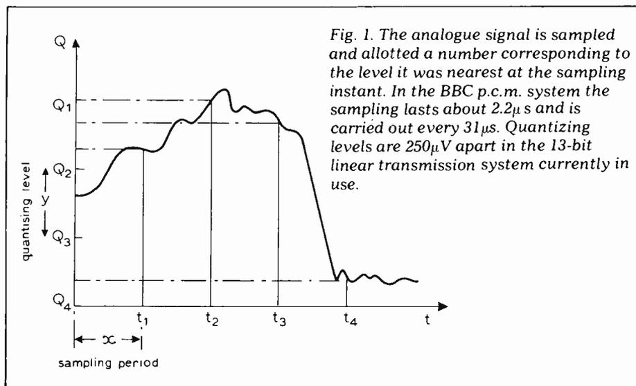
Fig. 1. The analogue signal is sampled and allotted a number corresponding to the level it was nearest at the sampling instant. In the BBC p.c.m. system the sampling lasts about  $2.2\mu\text{s}$  and is carried out every  $31\mu\text{s}$ . Quantizing levels are  $250\mu\text{V}$  apart in the 13-bit linear transmission system currently in use.
