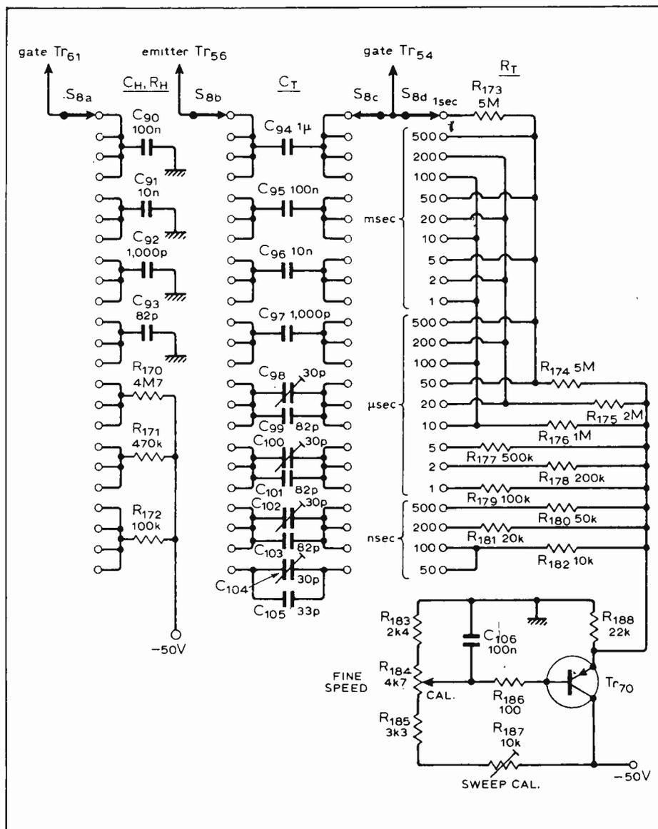
Fig. 8. Sweep-time selector switch and fine sweep-time control.  $C_H$  and  $R_H$  are hold-off components to allow  $C_T$  time to discharge.
