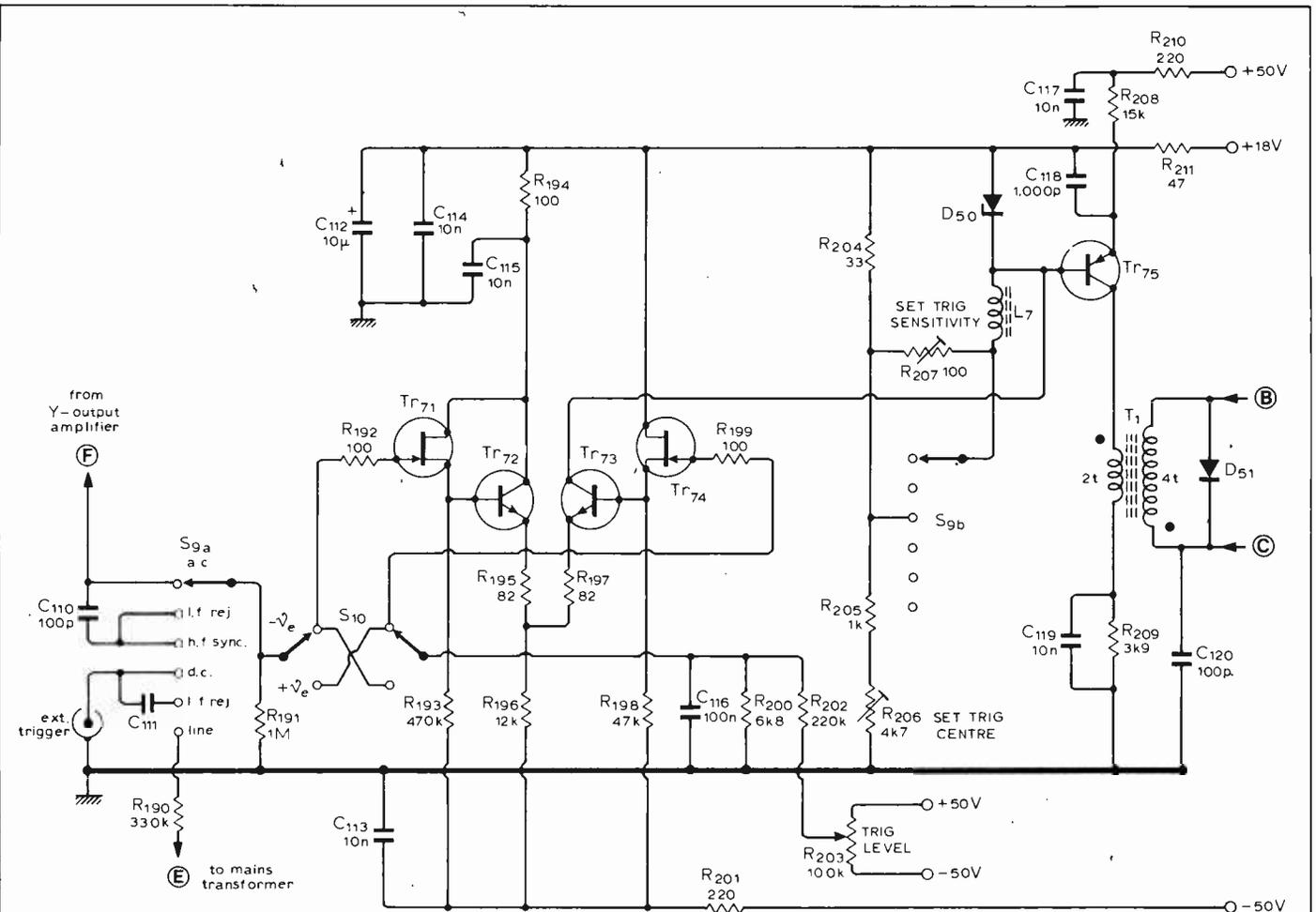
Fig. 9. The trigger generator.  $T_1$  is wound on a ferrite bead.
