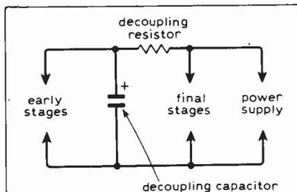
Fig. 1. A decoupling resistor.
