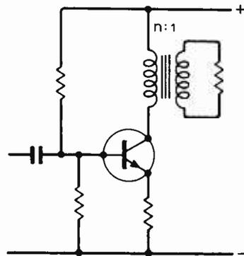
Fig. 7. A load resistor connected to the collector circuit of a bipolar transistor by a transformer.
