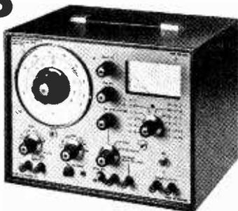
**DM344A Distortion Factor Meter.** Designed to make accurate and rapid measurements of total harmonic distortion generated within high quality audio amplifiers, recording and transmission equipment. **Selling Price: c/w Bench Case £175.00 + VAT.**
