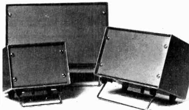
Standard minicases are made from 20g. mild steel sheets zinc-coated and finished in silver grey hammer-tone stove enamel. Front panels made from 18g. steel, finished in light grey high gloss enamel.
