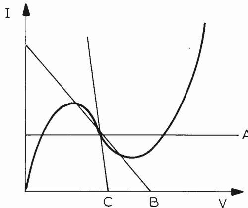
Fig. 10. The effect of varying the load line of the tunnel diode by  $R_{207}$ . A and B show Schmitt operation, with varying degrees of hysteresis, while C is the slope for oscillation.
