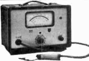
H.F. Multivoltmeter Philips Type GM 6014 Ranges 1mV-300mV in 6 Ranges. Facility also for 100mV-30V. Meter equipped with dB scale. Accuracy at 30kHz less than 3% F.S.D. Amplitude characteristic flat within  $\pm 5\%$  **£55**
