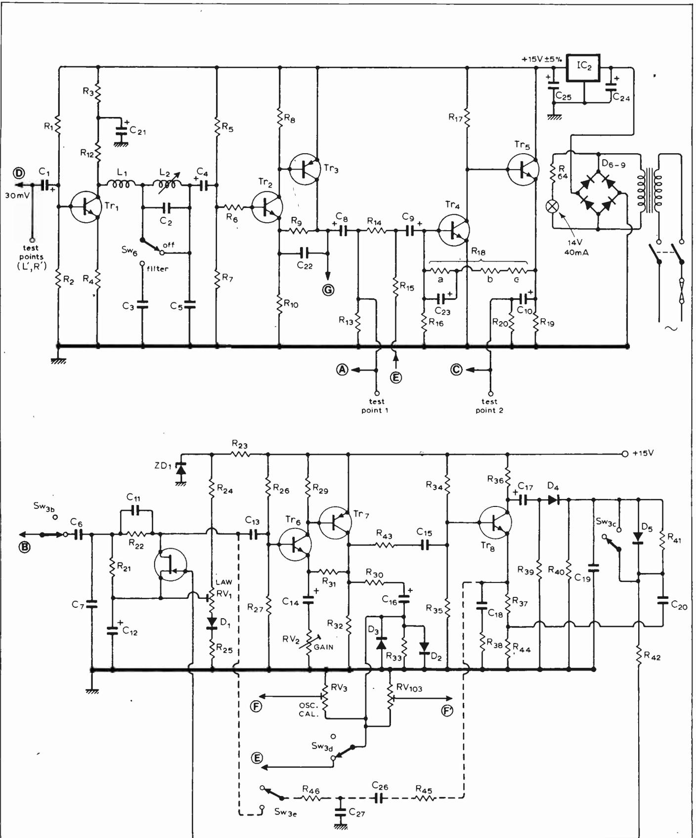
Fig. 12. Circuit of one channel of the stereo Dolby B noise reduction unit. Upper circuit is of main signal path, input at D, output at C. Point G serves meter circuits of Fig. 15, while point A or point C feeds the side-path input B (bottom), according to whether encode
