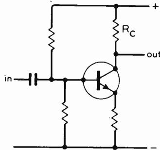
Fig. 5. A load resistor  $R_c$  connected directly into the collector circuit of a bipolar transistor.
