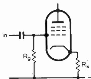
Fig. 2. Essential features of the automatic cathode biasing circuit.
