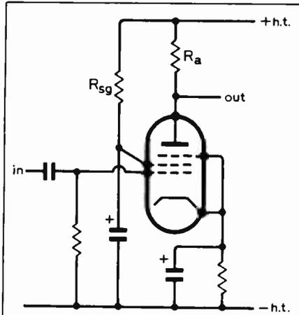
Fig. 4. Method of applying positive bias to the screen-grid of a pentode.
