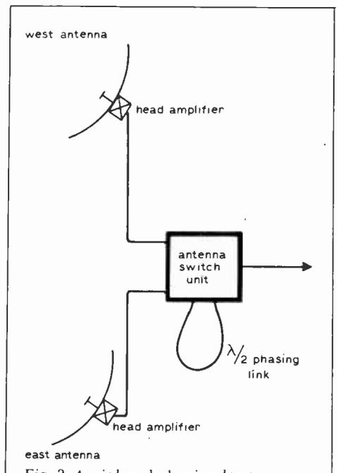
Fig. 2. Aerial and phasing loop connections.
