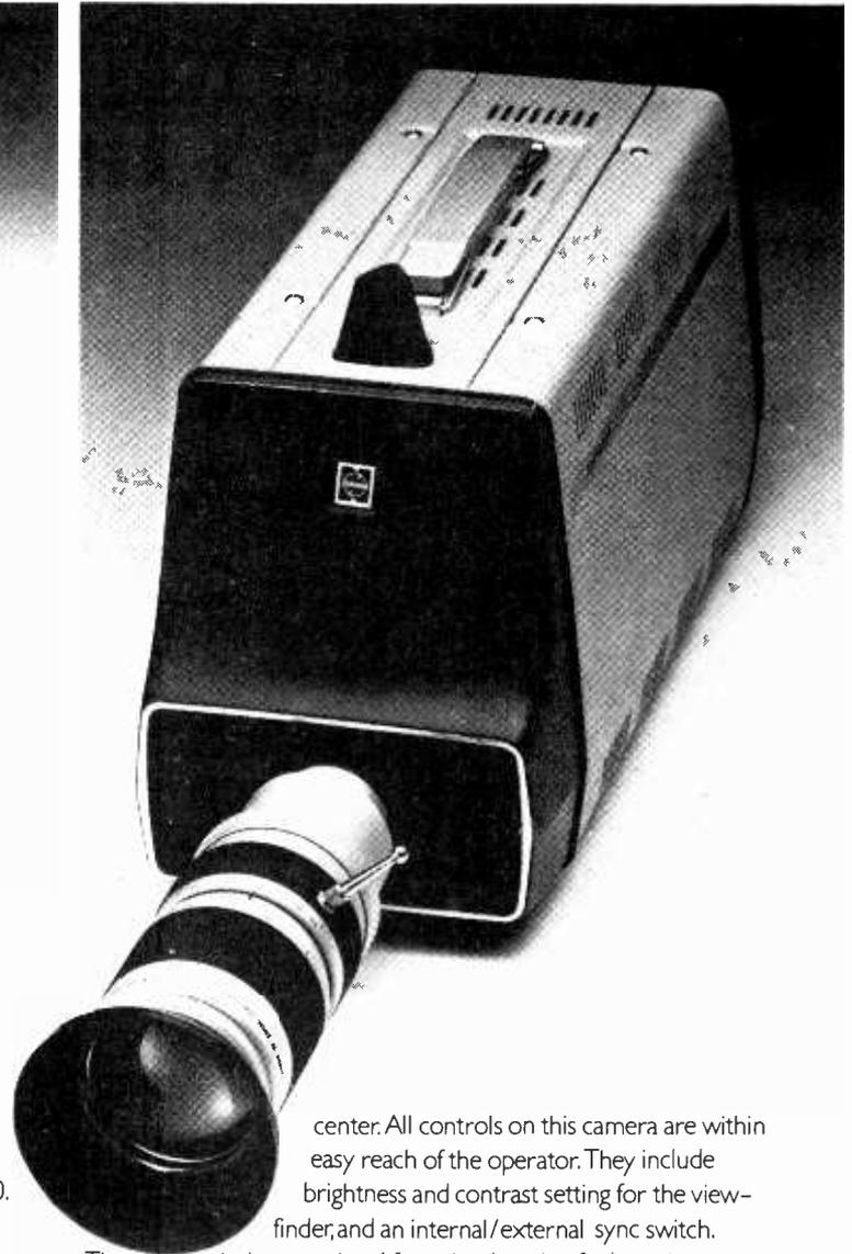
center. All controls on this camera are within easy reach of the operator. They include brightness and contrast setting for the viewfinder, and an internal/external sync switch. They also include an optional focus knob, a viewfinder selection switch, an intercom connection, and an on/off switch with pilot light. All are located at the back of the camera. Beam focus and target controls are on the side of the camera where they are unlikely to be misadjusted. At £220 this camera is quite a buy.
