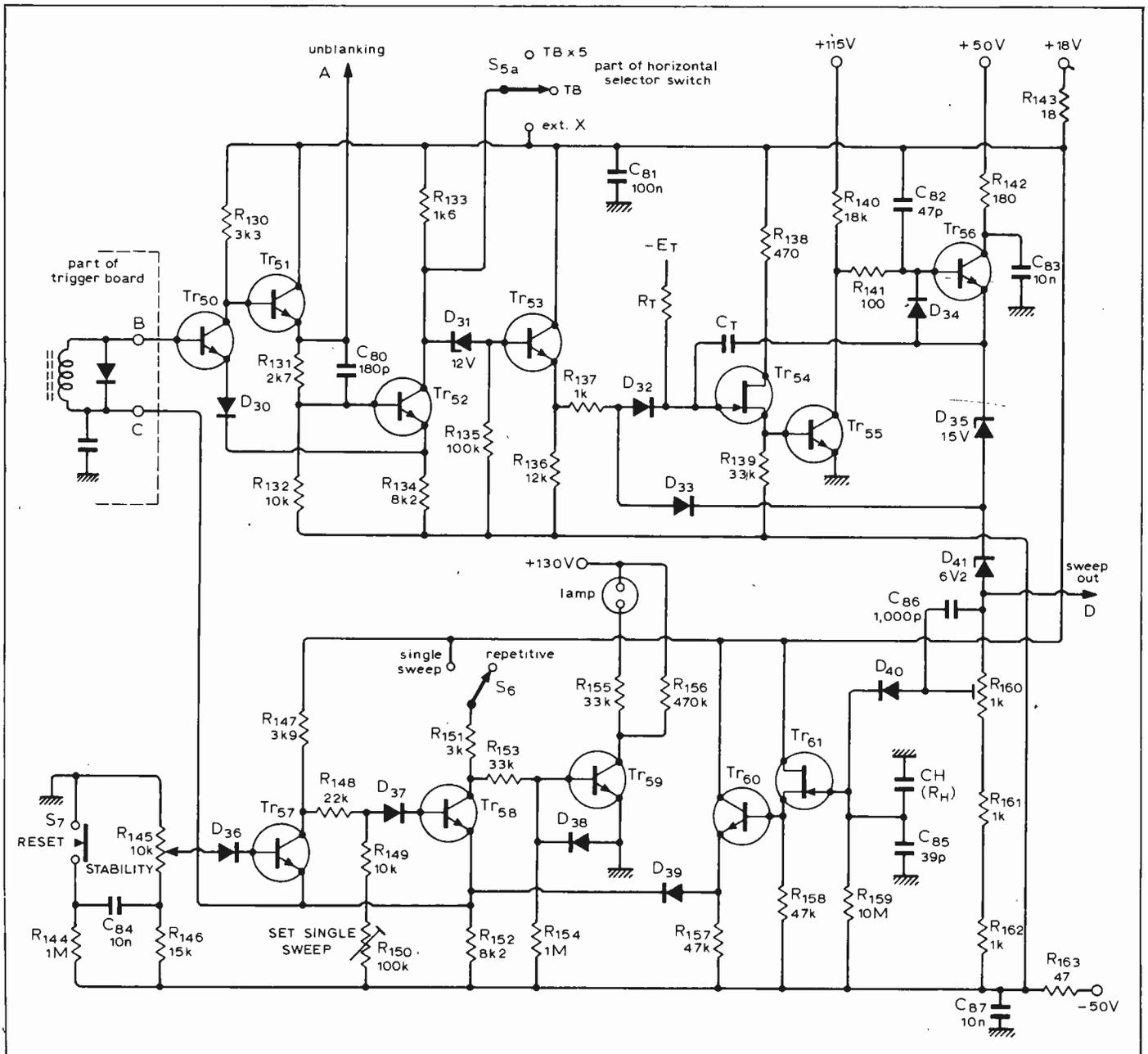
triggering signal may be selected from the Y amplifier, with a choice of a.c. coupling or low frequency rejection (high pass filter), from the 50Hz mains, or from an external socket. A facility is provided for single-shot operation — either triggered or free running, depending on the position of the stability control. A push-button and neon indicator resets the sweep and provides an indication that the circuit is ready to be triggered.
