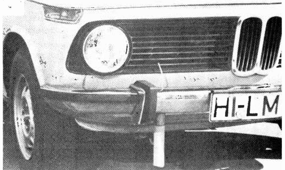
Fig. 3. Ferrite rod "aerial" for inductive transmission and reception on the chassis of a car.
