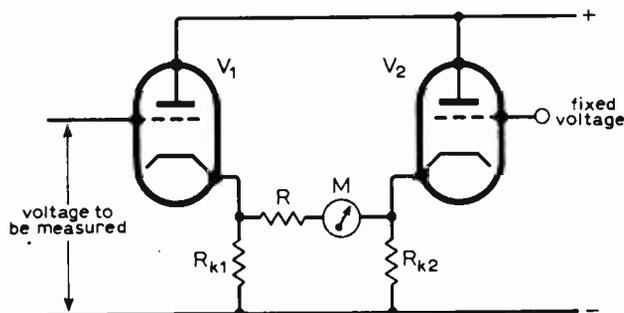
Fig. 10. Basic form of an electronic voltmeter circuit.
