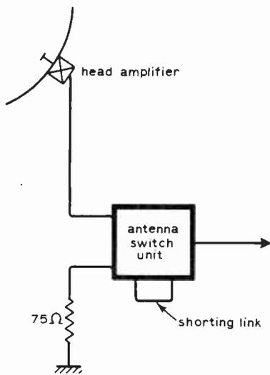
Fig. 3. Dicke mode connection.
