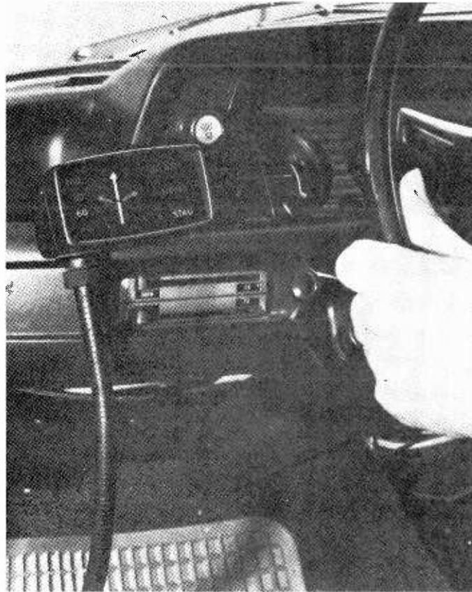
Fig. 2. Announcement display in the vehicle. This has arrows to give directions, warnings of road conditions and recommended speeds.
