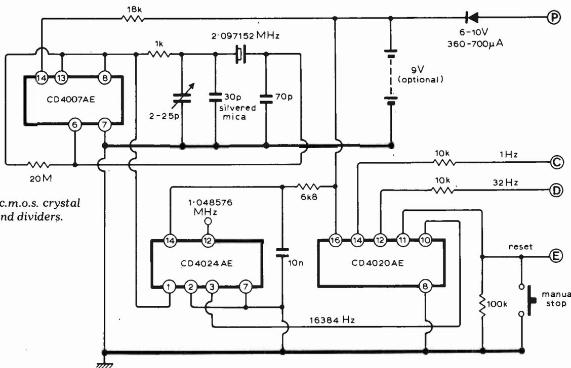
Fig. 7. The c.m.o.s. crystal oscillator and dividers.
