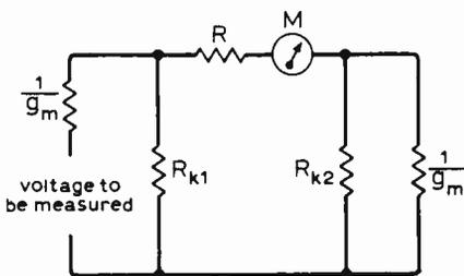
Fig. 11. First step simplifying the circuit of Fig. 10.
