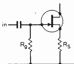
Fig. 3. One method of biasing a depletion-type f.e.t. using a resistor in the source circuit.
