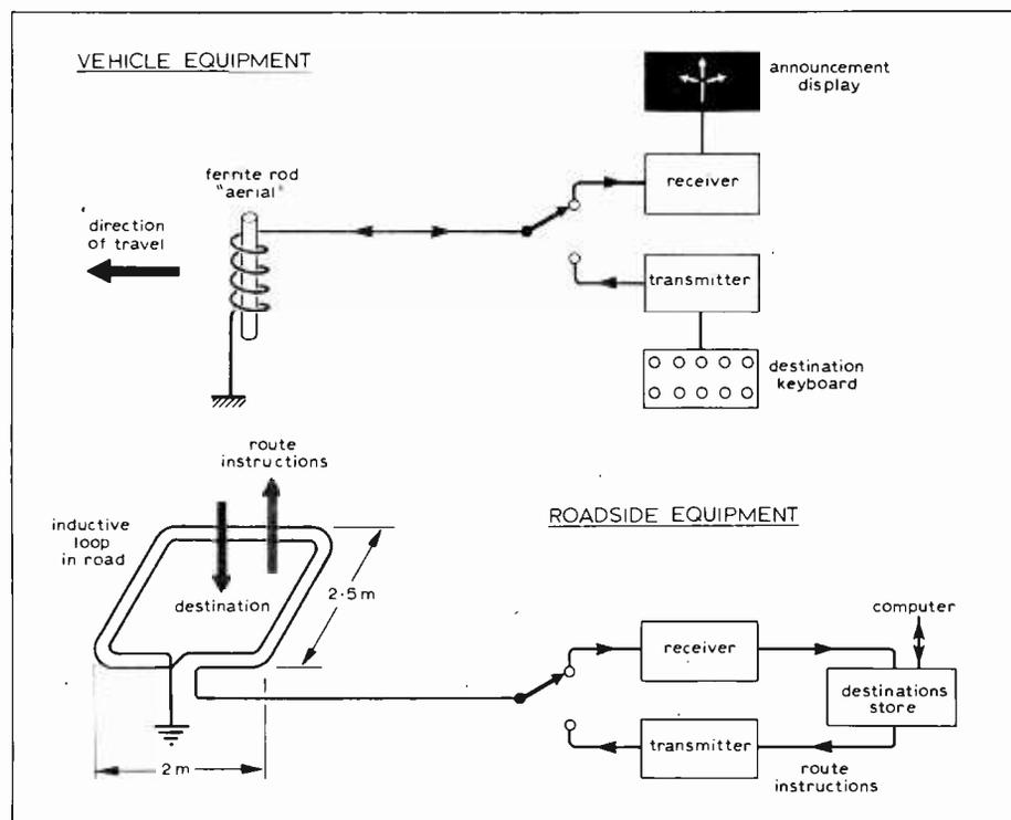
Fig.1. Simplified schematic of the drivers' guidance and information system, showing a vehicle equipment and roadside equipment communicating with each other by magnetic induction.
