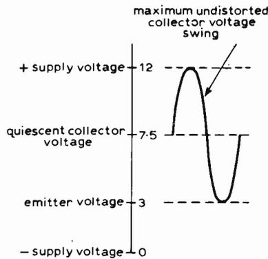
Fig. 6. Representing operating conditions in the collector circuit of a bipolar transistor with a directly-connected load.
