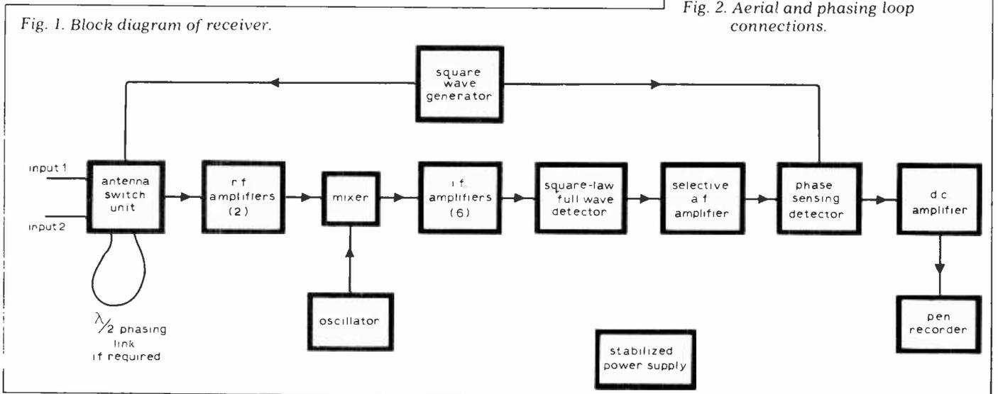
Fig. 1. Block diagram of receiver.
