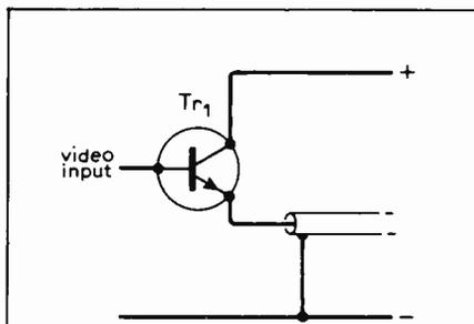
Fig. 13. An emitter follower used to feed video signals into a coaxial cable.
