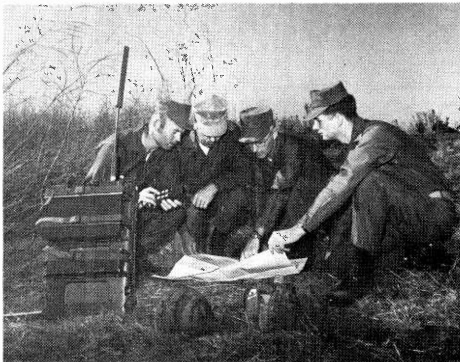
*Position Location Reporting System seen in use here was developed for the US Marine Corps by Hughes Aircraft Company's ground systems group at Fullerton, California. The set, which weighs 15 pounds, continuously and automatically exchanges information with a master unit back at the command post.*
