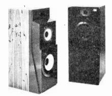
Stepped mounting of drive units in this Leak 3080, largest of the new 3000 range, is to provide time-delay compensation, which is said to provide an improved stereo image and a greater impression of depth in a single speaker.
