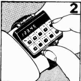
2. Hold the switch to the left to use the functions to the left above the keys...
