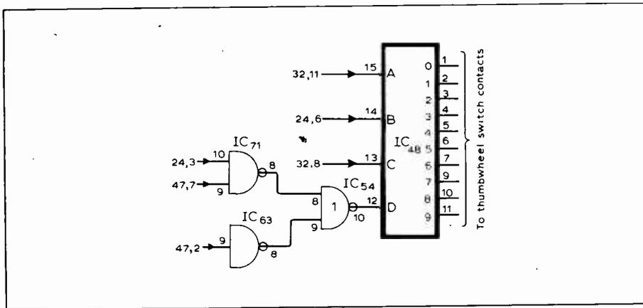
Fig. 1. Modification to cope with transmission of interleaved magazines.
