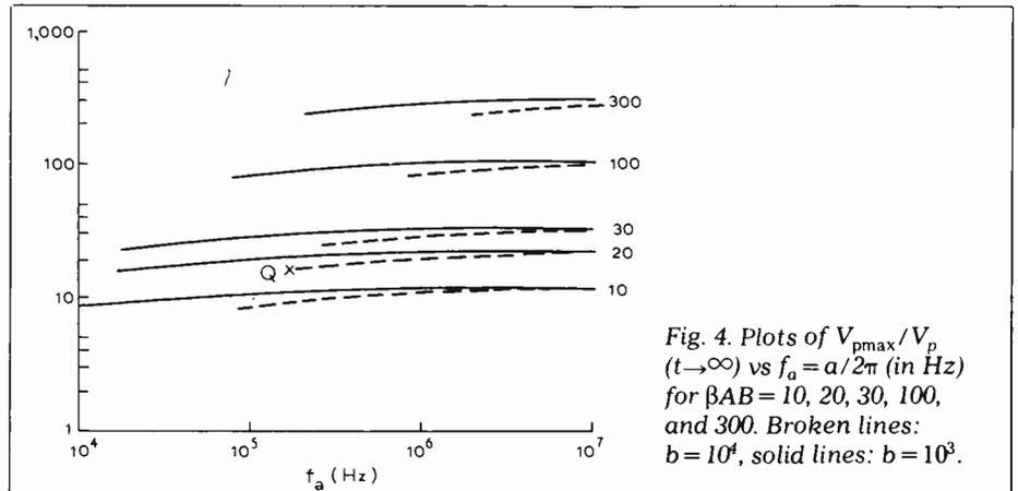
Fig. 4. Plots of  $V_{pmax}/V_p(t \rightarrow \infty)$  vs  $f_a = a/2\pi$  (in Hz) for  $\beta AB = 10, 20, 30, 100,$  and  $300$ . Broken lines:  $b = 10^4$ , solid lines:  $b = 10^3$ .
