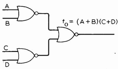
Fig. 5. Dualizing  $f = AB + CD$  with NOR gates.
