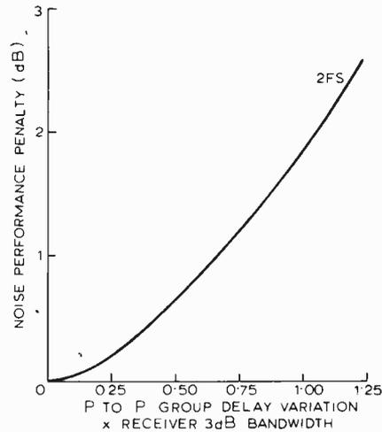
Fig. 5. Effect of group delay distortion on noise performance.
