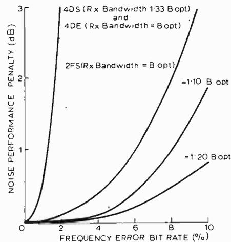
Fig. 6. Effect of system frequency stability on noise performance.
