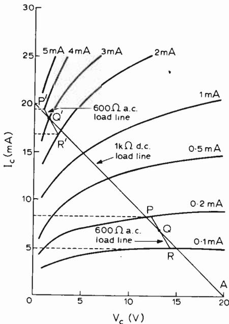
Fig. 19.  $I_c-V_c$  characteristics and typical a.c. and d.c. load lines for forward a.g.c.
