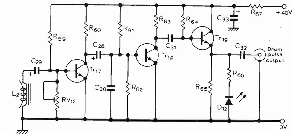
Fig 13. Drum-pulse amplifier
