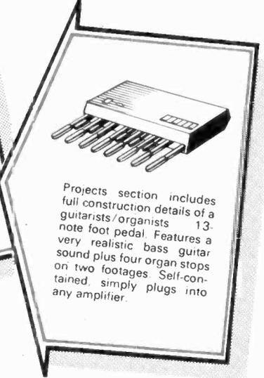
Projects section includes full construction details of a guitarists/organists 13-note foot pedal. Features a very realistic bass guitar sound plus four organ stops on two footages. Self-contained, simply plugs into any amplifier.
