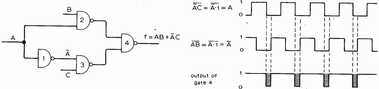
Fig. 7. Mechanism of "spike" generation.
