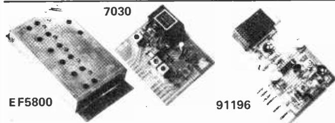
From left to right, the EF5800 6 circuit varicap FM tunerhead. Two MOS RF stages, both with AGC control, and an ultra stable oscillator. Next the 7030 Linear Phase 10.7MHz IF. Distortion 0.08%, muting, AGC, meter, auto stereo switch outputs. Finally the new 91196 mpx decoder and combined birdy filter. Mono THD 0.05%, stereo sep. 55dB at 1kHz, 42dB at 10kHz - the best decoder module yet. EF5800.....£14.50 7030.....£10.95 91196.....£12.99 (Built).
