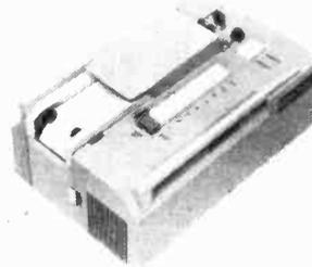
Polarized moving iron movements with syphon pens directly attached. Built-in solid state amplifier (one per channel) provides 8 calibrated sensitivity steps. Two marker pens are provided. Basic error 4% Frequency response from DC to 100Hz 2dB.
