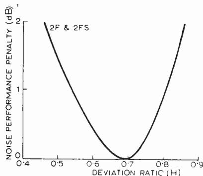
Fig. 8. Effect of f.s.k. deviation ratio on noise performance.
