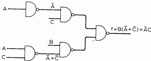
Fig. 12. Two-input NANDS used to realise  $f = B(\bar{A} + \bar{C}) + \bar{A}C$ , which is hazard-free form of  $f = AC + B\bar{C}$ .
