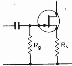
Fig. 21. A depletion-type f.e.t. biased by a resistor in the source circuit
