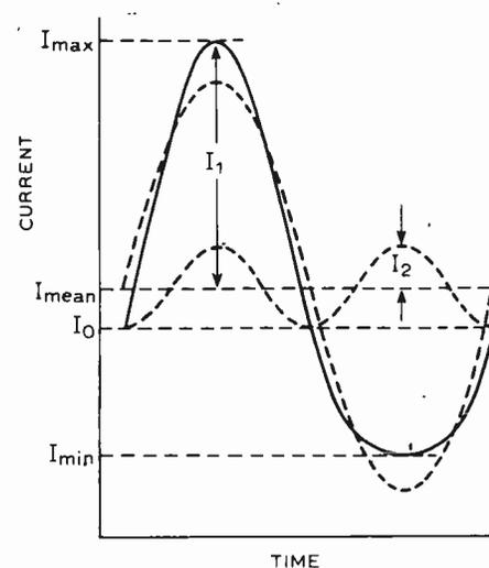
Fig. 16. Fundamental and second-harmonic components of the waveform of Fig. 15
