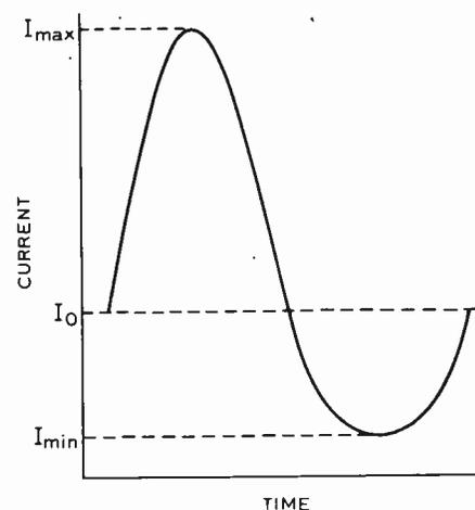
Fig. 15. Type of waveform distortion given by a device with a parabolic characteristic
