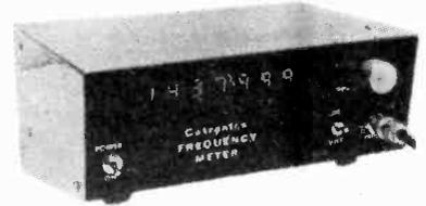
**200MHz D.F.M. for direct readings up to the mobile radio VHF 'High Band'**
