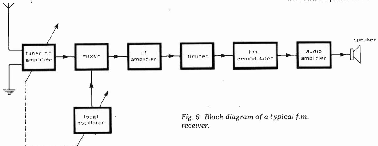
Fig. 6. Block diagram of a typical f.m. receiver.
