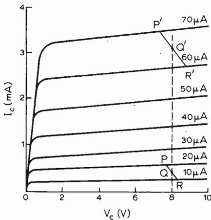
Fig. 18.  $I_c-V_c$  characteristics and load lines showing the action of reverse a.g.c.
