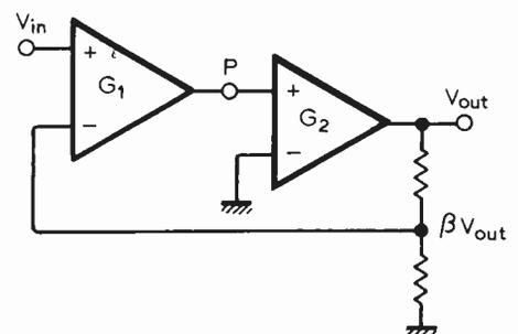
Fig.2. Two-stage amplifier with overall negative feedback.
