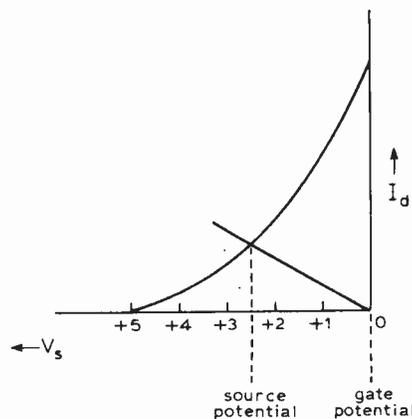
Fig. 23. The  $I_d-V_s$  characteristic is the same as the  $I_d-V_g$  with the voltages reversed in sign
