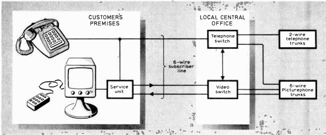
Fig. 2. (above). Basic local arrangement used in the Picturephone system developed by Bell Telephone; (right) Picturephone computer access system
