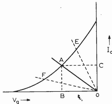
Fig. 22. Load lines on  $I_d-V_g$  characteristics showing bias value achieved
