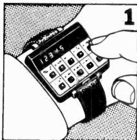
1. The switch in its normal, central position. With the switch centred, numbers – which make up the vast majority of key-strokes – are tapped in the normal way
