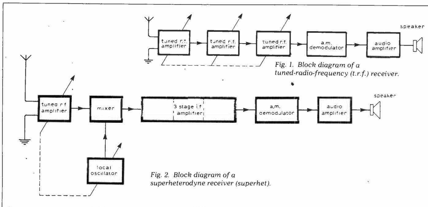
Fig. 1. Block diagram of a tuned-radio-frequency (t.r.f.) receiver.
