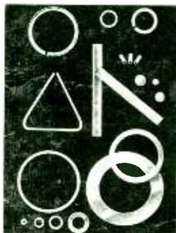
Whether cream or preforms are used, just raise the temperature of the metal surfaces to around 50°C above the melting temperature of the solder. The solder cream or preform does the rest. Heating techniques can include gas flame, hot plate, oven conveyor, induction coils, resistance/electrode soldering, hot gas and infra-red.
