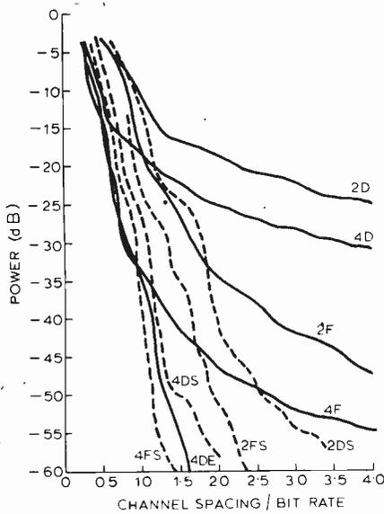
Fig. 2. Adjacent channel rejection factor.
