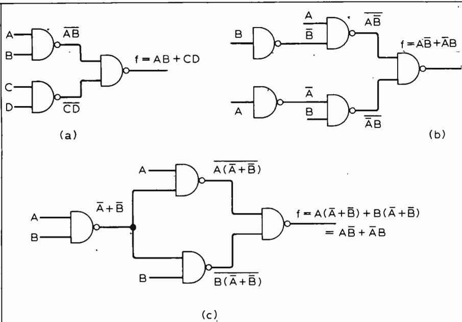
Fig. 3. The use of NAND gates to obtain a sum-of-products function (a). The minimal form of expression need not give a minimal circuit; minimal expression  $f = \bar{A}\bar{B} + \bar{A}B$  in (b) needs one more gate than non-minimal expression  $f = A(\bar{A} + \bar{B}) + B(\bar{A} + \bar{B})$  at (c).
