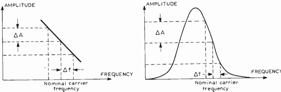
Fig. 5. The f.m. demodulator characteristic, shown in Fig. 4, can be approximated by operating on the flank of a tuned circuit's response curve, as shown. Demodulator is tuned so that the nominal frequency is halfway down the response curve
