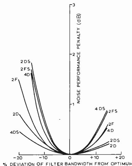
Fig. 4. Effect of filter bandwidth on noise performance.
