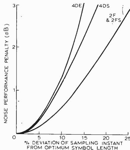
Fig. 7. Effect of demodulator sampling instant errors on noise performance.
