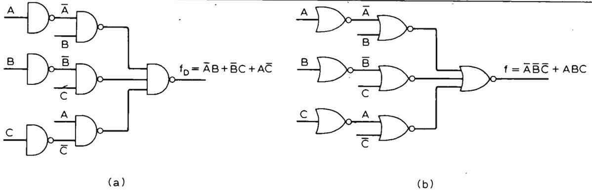
Fig. 6. Generating a function using NOR gates. Function  $f = \bar{A} \bar{B} \bar{C} + A B C$  is first dualized, minimized and implemented in NAND logic, as at (a). This circuit is then converted to NOR gates to provide the required output.
