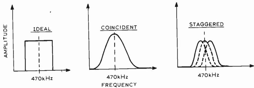
Fig. 4. Ideal response curve for an f.m. demodulator.
