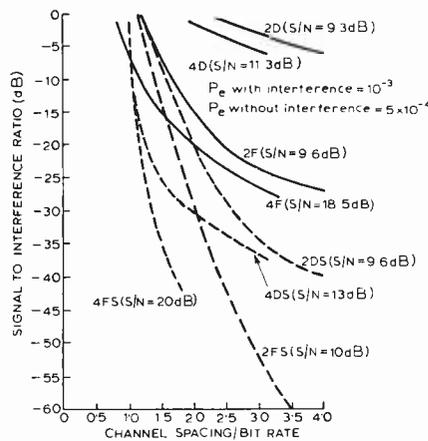
Fig. 3. Minimum channel spacing versus  $s/i$  ratio.
