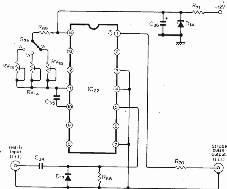
Fig 14. SR strobe-pulse generator
