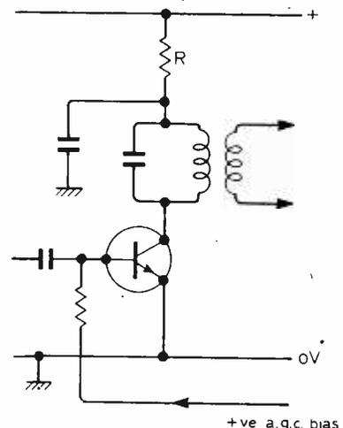
Fig. 20. Essential features of circuit for forward a.g.c.
