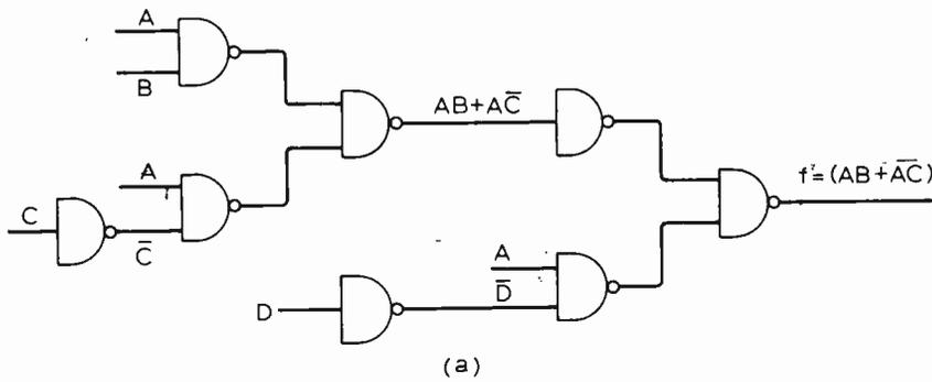
Fig. 9. Bracketing two products in  $f = AB + AC + AD$  enables use of 2-input gates but requires eight instead of six, as in (a). Removing a common factor again meets fan-in restriction to 2 inputs, with varying savings in number of gates, as seen in (b) and (c).
