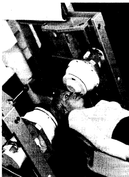
J & P Engineering's Tomoscanner. The two detectors are shown tilted at about 45°. They are each capable of detecting two different activity-level isotopes. The movements of the detectors, either around the patient, along her body or in two parallel planes at either side, can be controlled by a small hand-held device connected to the scanner.
