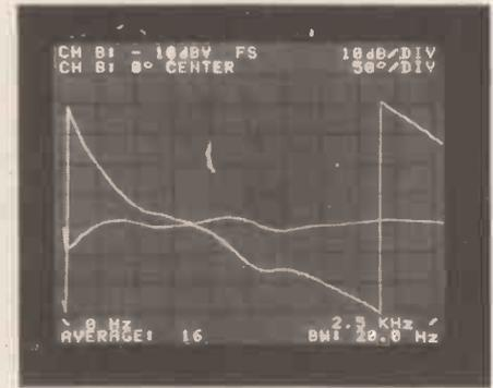
Fig. 12. Frequency and phase response of a Chartwell LS3/5A loudspeaker measured with an impulse. a) 0-25kHz, b) 0-2.5kHz.
