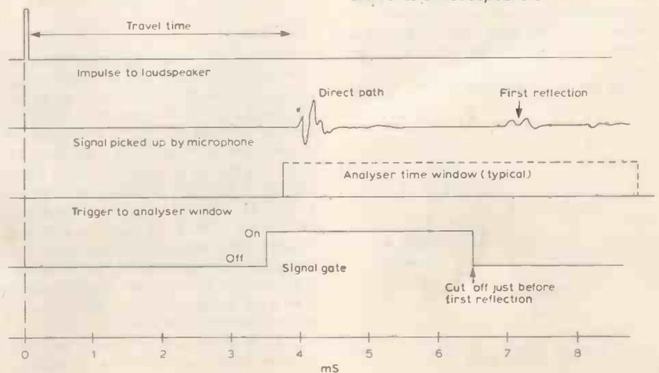
low frequency response is to be examined in detail), an electronic signal gate is needed so that the first direct-path signal can be isolated. To do this, and to be able to adjust all the delays correctly and generate the test impulse required some auxilliary equipment in addition to the analyser itself. This is unfortunate because it seems that it would have been quite simple to build all the required functions into the analyser in the first instance.\*
