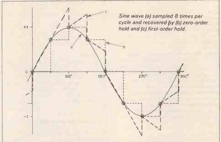
generate a slope which will, one hopes, lead towards the point where the next sample will arrive as shown here. This method effects a significant reduction in the delay terms. A second order hold is also possible and this will generate sections or parabolae. I do not know of any applications in real time where this technique is used, but it is not uncommon for curve generation in the computer numerical control of milling machines, for example.
