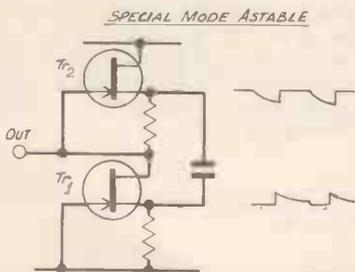
Current-operated circuits extend the range of possibilities as compared to the restriction of voltage operation. A halfway house is provided where active devices are operated in series from a voltage supply. These are again a specialized sub-group of astables, but can be simple and effective. The version shown is a serial form of the emitter-coupled astable though implemented with junction f.e.t.s as this eliminates a number of bias components.
