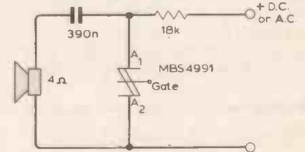
A<sub>2</sub> reduces this to around 3V. An 8 $\Omega$  speaker can also be used with a small reduction in output power.
