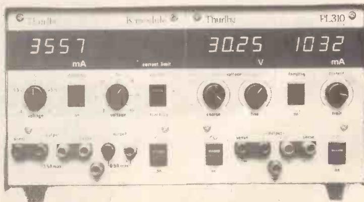
PL310K, 0 to 30V at 0 to 1A, 0 to 30V at ½A, 5 ± 1V at 3½A, £199.50
