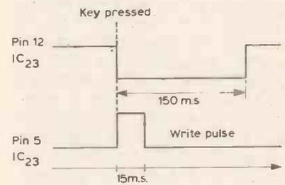
Fig. 9. Single write pulse.
