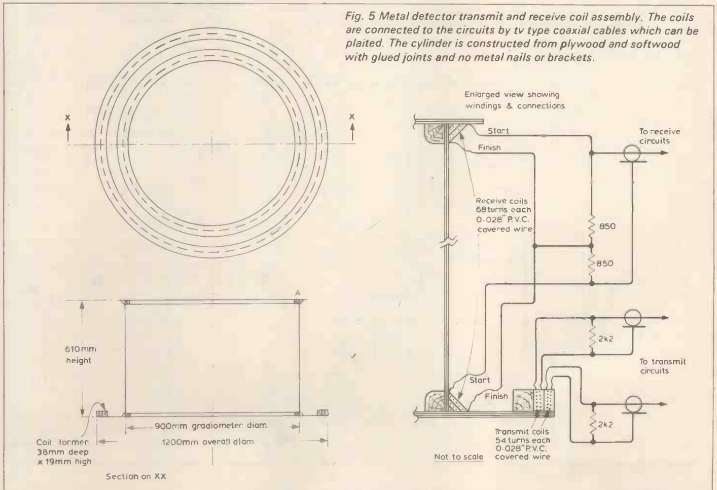
Fig. 5 Metal detector transmit and receive coil assembly. The coils are connected to the circuits by tv type coaxial cables which can be plaited. The cylinder is constructed from plywood and softwood with glued joints and no metal nails or brackets.
