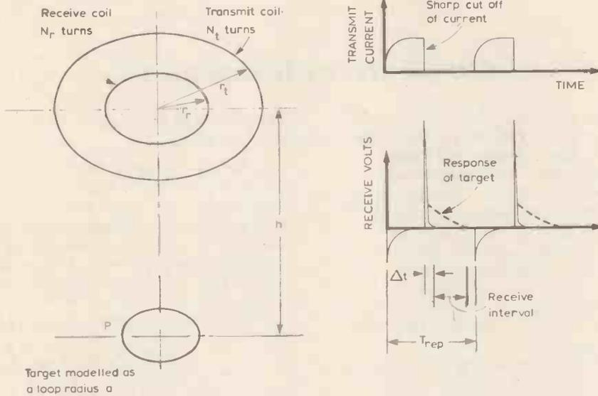
Fig. 1 Elements of a pulse induction system.
