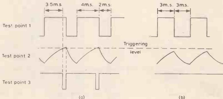
Fig. 13. Circuit waveforms.
