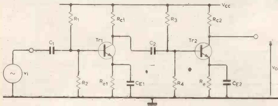
frequently encountered circuits behave as true Thevenin or Norton circuits; for example, the common emitter amplifier shown in Fig. 5. Neglecting the bias-resistance loading effects and assuming that all capacitors are short circuits, the mid-band voltage gain is given approximately by
