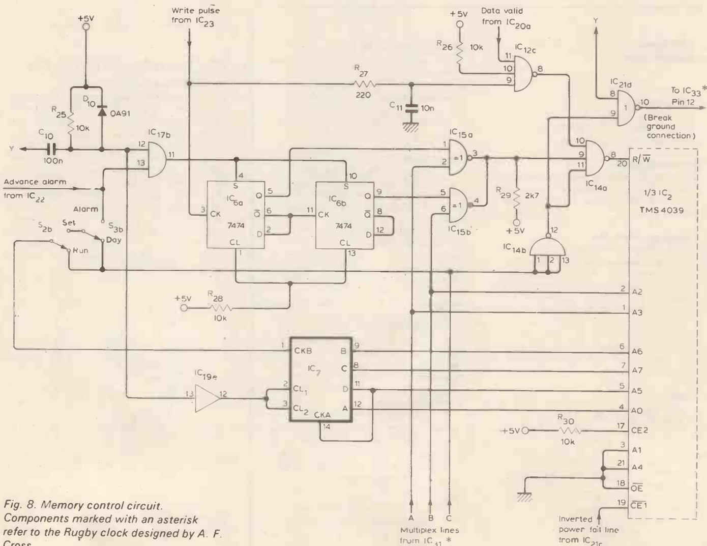
Fig. 8. Memory control circuit. Components marked with an asterisk refer to the Rugby clock designed by A. F. Cross.
