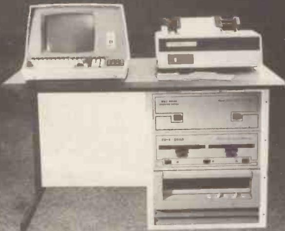
The MSI System 12 computer system combines the popular MSI 6800 processor ... complete with 56K of memory ... the MSI FD-8 QUAD floppy disk system, and the new MSI HD-8/R 10 megabyte fixed/removable hard disk system in one compact desk unit.
