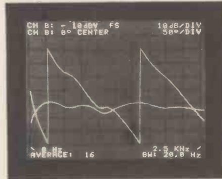
Fig. 11. Frequency and phase response of a Spendor BC1 loudspeaker measured with an impulse, a) 0-25kHz, b) 0-2.5kHz.
