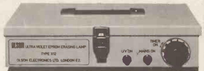
Low cost ultra violet eeprom erasing lamp will erase up to 12 chips at one time.
