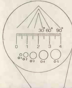
The graticule is calibrated to 4mm overall in increments of 0.1mm, with angles shown from 30° to 90° and hole sizes of 0.2, 0.3, 0.4 and 0.5mm diameter.
