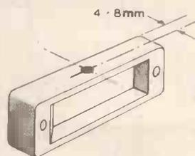
Fig. 10. Mixer power can be adjusted by fitting a  $2\text{mm}$  screw in shroud.
