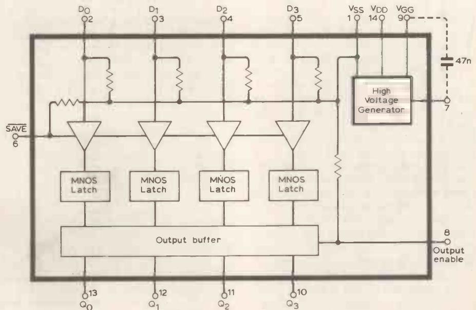
Fig. 1. Internal block diagram of MN9102 quad latch.
