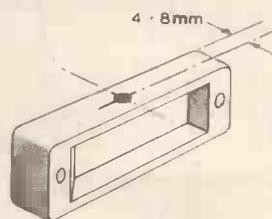
Fig. 10. Mixer power can be adjusted by fitting a 2mm screw in shroud.
