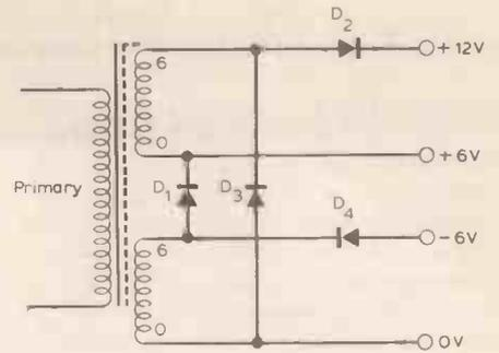
windings alternately and both low current rails are fed on alternate half-cycles. The voltages shown increase when capacitors are connected to provide an adequate margin for the regulators.
