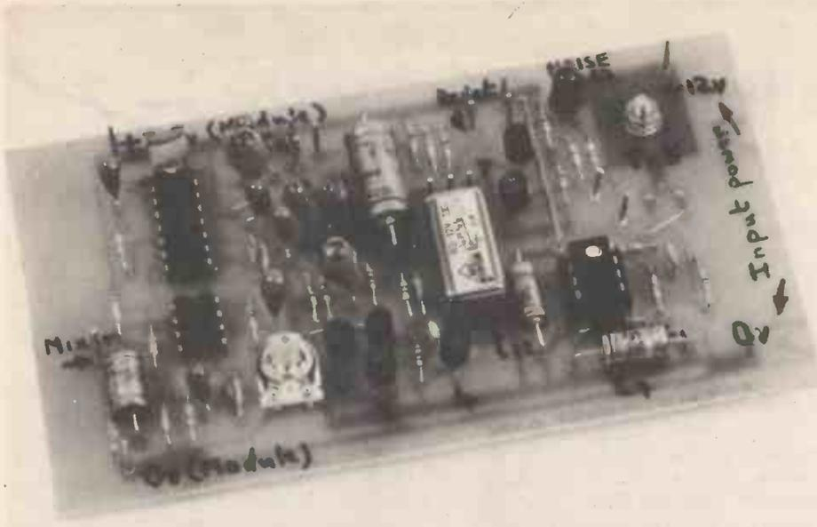
◀ Circuit board for combined alarm and monitor circuits of Figs. 9 & 11 includes noise indicator on board for demonstration use. Board pattern appears on page 81 with location diagram on page 84.
