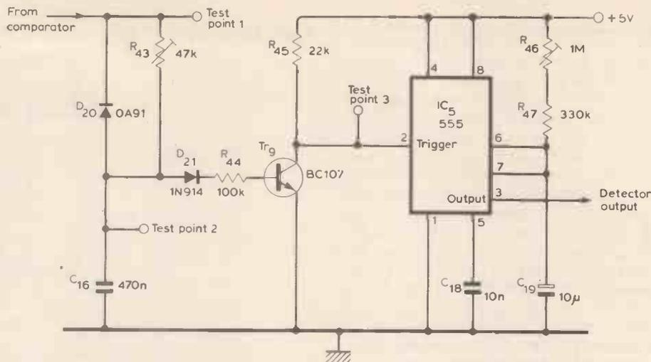
Fig. 11. Comparison detector. Resistor R<sub>43</sub> is adjusted so that pulses shorter than 4ms are rejected.
