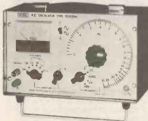
**FREQUENCY** 3Hz to 300kHz in 5 decade ranges.
