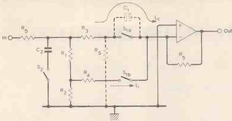
Fig. 7 Internal capacitance effect and compensation low-pass filter.
