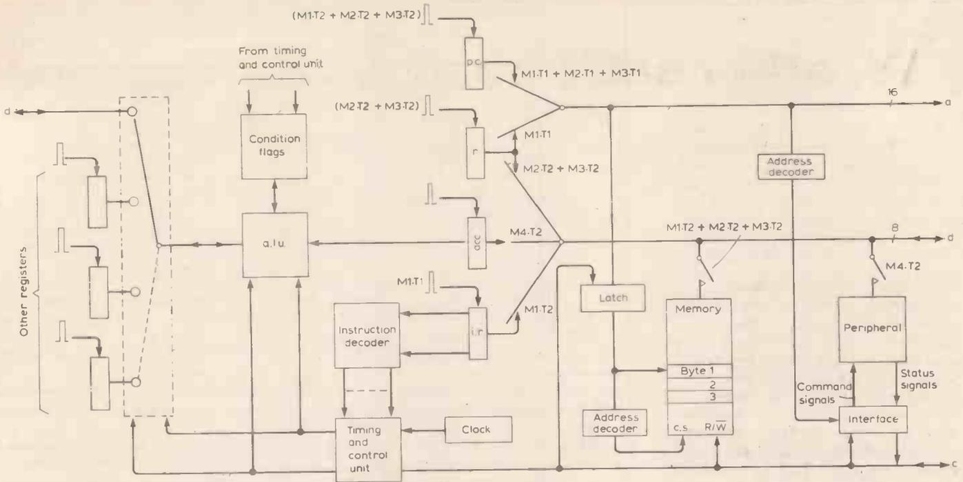
Fig. 7. Components and internal organization of an eight-bit microprocessor chip.
