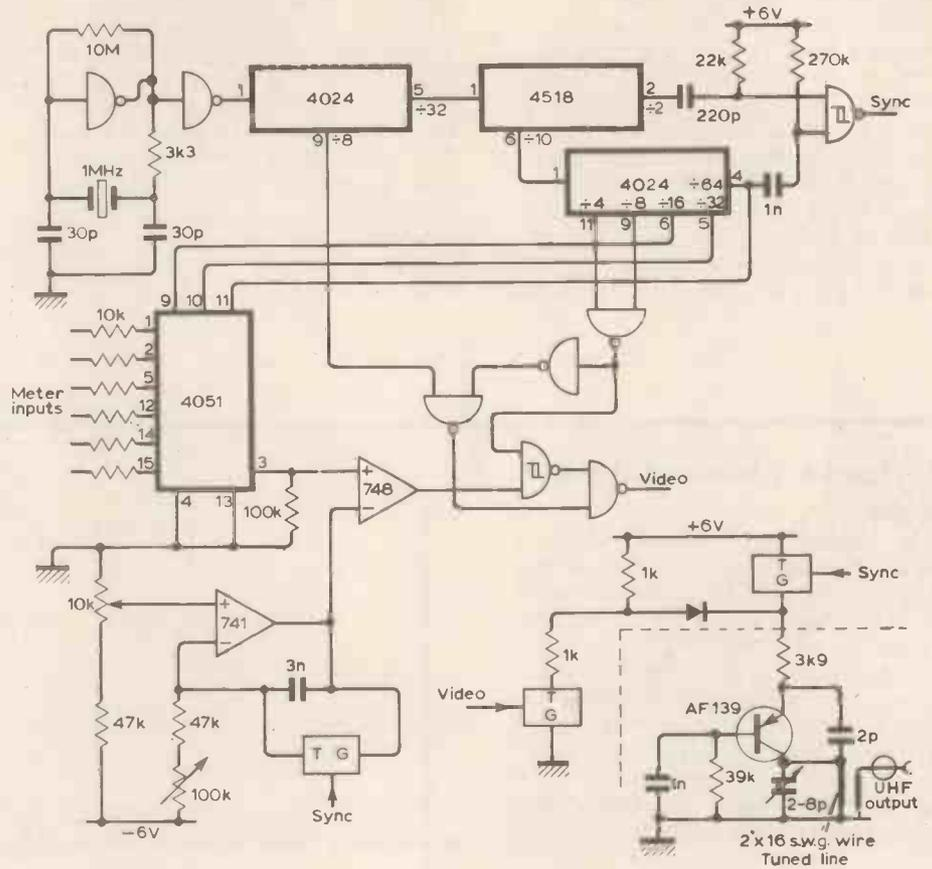
pulse. For 25 channels, four 4051 i.cs are enabled in turn by a 1-of-4 decoder driven by a divide-by-32 and 64 on the second 4024. All of the 4024 outputs, except frame sync., are increased in frequency four times.
