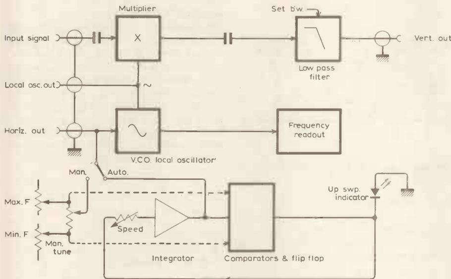
Fig. 8. Detailed block diagram of the instrument. Horizontal and vertical outputs are taken to the oscilloscope, and the local oscillator output is for use with an external counter or other test gear.
