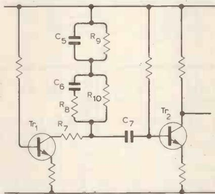
The resistor  $R_7$  is used only for "equalizing" the loading of  $Tr_1$ .
