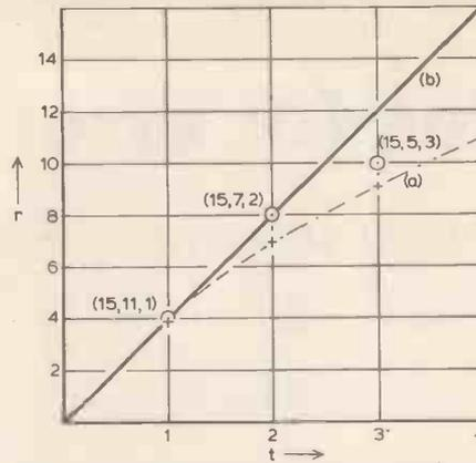
Fig. 1. Numbers of check digits for error-correcting codes of length 15. (a) Theoretical (non-integral) values. (b) The  $mt$  rule for BCH codes. Circled points indicate the values for actual BCH codes.
