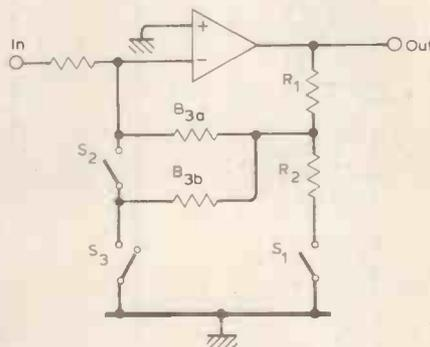
Fig. 4 Extended circuit with two independent switches.
