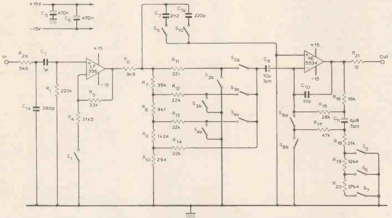
Fig. 8 Complete attenuator circuit for one channel. The switches are grouped in five i.c.s as follows; S<sub>5</sub> + S<sub>6</sub>, S<sub>7</sub> + S<sub>8a/b</sub>; S<sub>2a/b</sub> + S<sub>3a/b</sub>, S<sub>4a/b</sub> + S<sub>1</sub>, and S<sub>9</sub> + S<sub>10</sub>. All resistors should be 1%.
