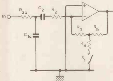
Fig. 10 Inverting input buffer.
