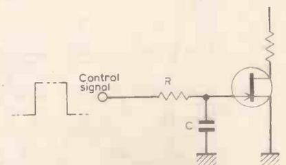
Fig. 6 Soft switching to overcome spikes.
