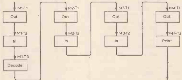
Fig. 8. Internal operation of a microprocessor chip.
