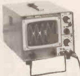
ELMAC 4810 CRT 5MHz scope £120 + VAT. As recommended by ETI. The best selling 5MHz 4" CRT scope in the UK. Timebase include sweep range — 100 msec/div to 1  $\mu$  sec/div in 5 steps. 3" also available. £96 + VAT.
