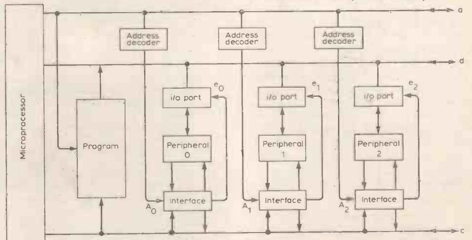
Fig. 6. Basic configuration for single-processor systems.
