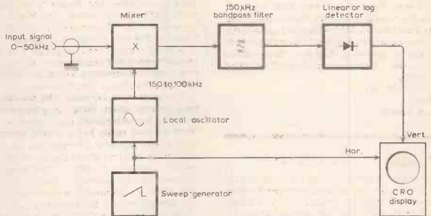
Fig. 3. Block diagram of a conventional spectrum analyser. The 150kHz bandpass filter must be very narrow: one commercial design uses five crystal resonators to achieve the required performance.
