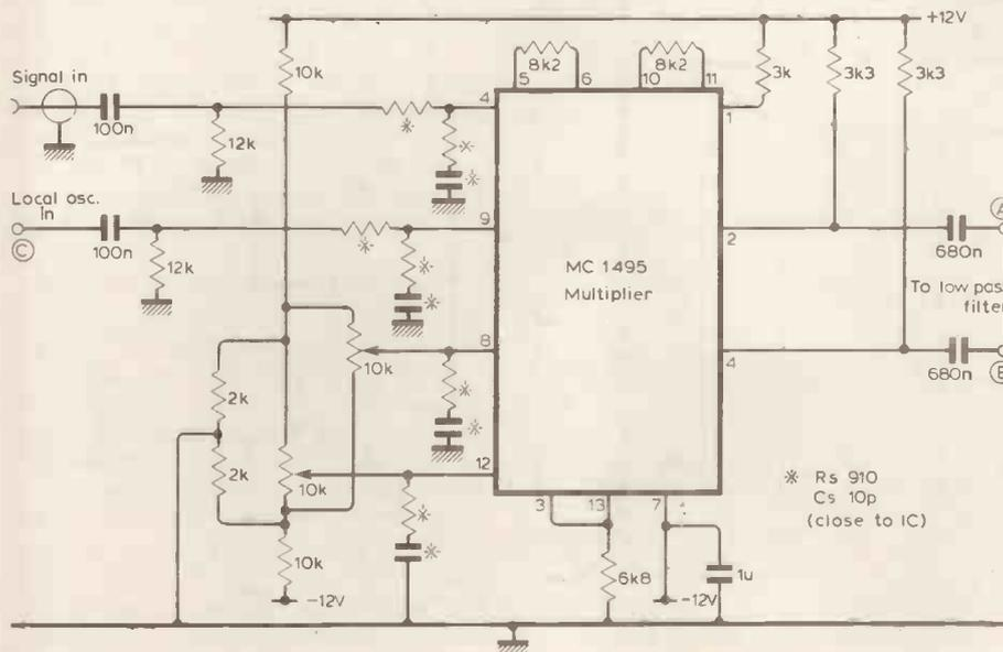
Fig. 9. Multiplier circuit.
