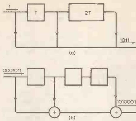
Fig. 2. (a) Encoding a single digit by means of delays  $T$  and  $2T$ . (b) Encoding a group of digits by means of a tapped shift register and adders.
