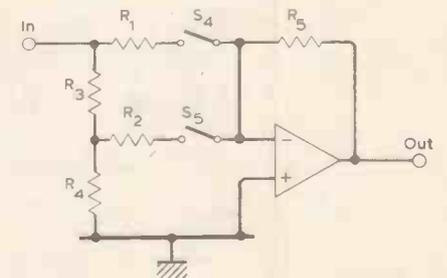
Fig. 5 Alternative two-switch circuit.
