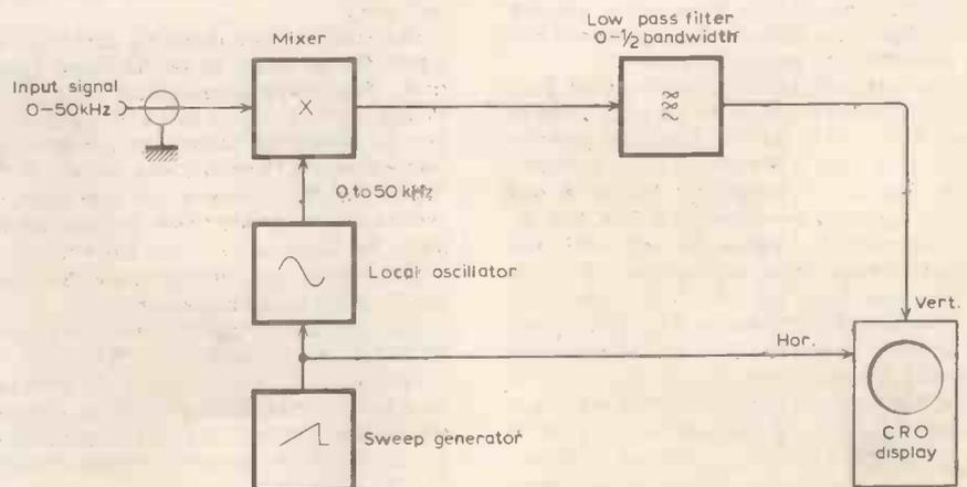
Fig. 4. Method used in this design, in which the filter takes the form of a low-pass circuit in the audio range.
