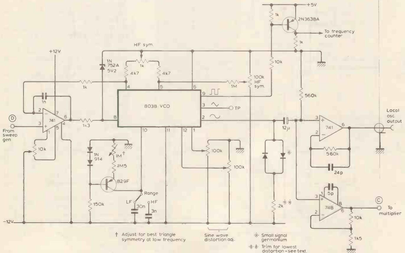
Fig. 11. Local oscillator circuit diagram.
