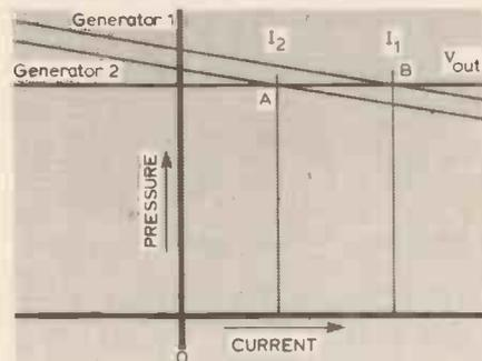
here. If the internal resistance is too low the output characteristics of the two generators are almost horizontal and the distance between points A and B can become large. Indeed it is quite possible for one of the points to be to the left of the vertical axis, which means that one generator is supplying current not only to the load but also into the other generator. Clearly there is magnification of inequalities.
