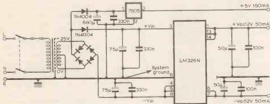
Fig. 15. Power supply circuit.
