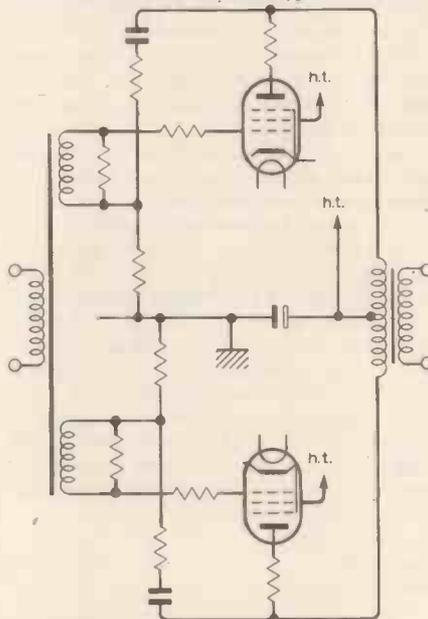
of a well-designed transformer. So there would not in this amplifier be a serious load-sharing problem. The arrangement of the output stage was, as far as I can remember, as shown above: unfortunately my pre-war *Wireless Worlds* are not to hand.
