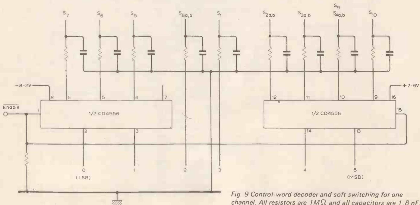
Fig. 9 Control-word decoder and soft switching for one channel. All resistors are 1MΩ and all capacitors are 1.8 nF.
