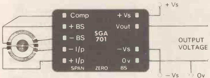
The series SGA 700 (based on our well-proven SGA 300\*) provides the complete solution to Strain Gauge Amplification. Simply connect the bridge, connect the power supplies ( $\pm 11\text{v}$  to  $\pm 15\text{v}$ ) and the SGA 700 does the rest. It also offers high stability (up to  $1\mu\text{V}/^\circ\text{C}$ ). Miniature size (above is actual size), good supply rejection — in fact a specification as good as many instruments many times the price and size.
