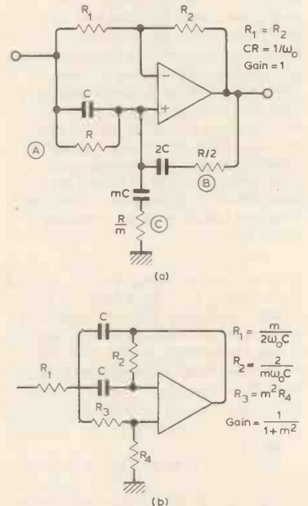
Fig. 5 Two active, all-pass circuits which can be made to give any value of damping factor. The Holt and Gray circuit (a) looks more complex but is easier to implement, since circuit (b) requires special R-values and an extra amplifier to recover unity gain.
