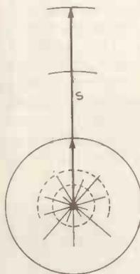
Fig. 1. Illustrating coherence. The vector  $S$  represents the signal whilst the noise is a number of random vectors in the centre. The area of the circles represents the power in the signal and the noise. Addition of  $N$  signal vectors in phase increases the signal power  $N^2$  times. The noise can only be added as power, so  $N$  samples gives only  $N$  times noise power, a signal/noise power gain of  $N$ .
