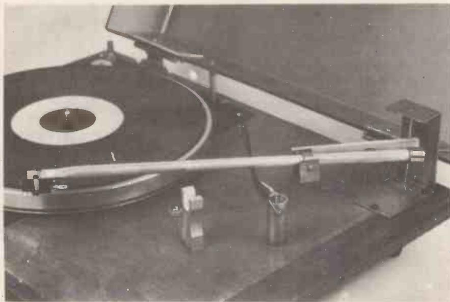
tightened, care being taken that the weight has its longer axis exactly parallel to the vertical pivot shaft so that it does not touch either this or the carrier bar.
