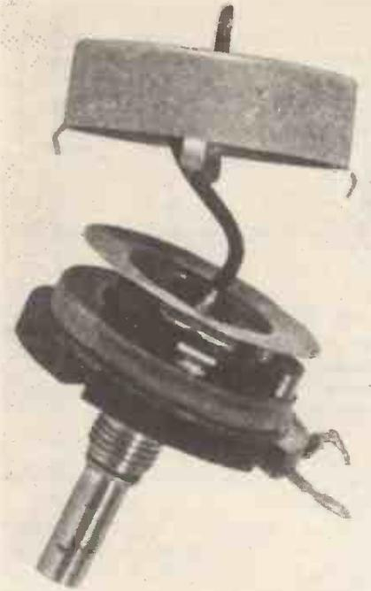
Fig. 31. Attenuator whose principle is shown in Fig. 30. Note screen round output. Photograph by courtesy of Electronic Engineering
