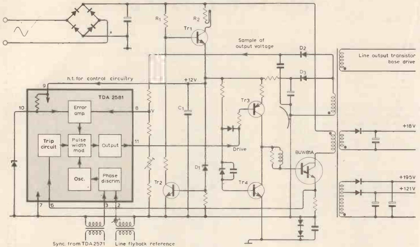
Fig. 18. Simplified version of complete power supply circuit.
