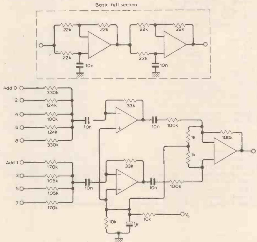
ever, more sections are then needed to retain the 200 Hz bandwidth, which increases cost but gives extra coherent gain. A good arrangement would be six stages with  $m$  about 1.7, but the cosine-on-pedestal with its low sidelobes was attractive and this model was made.
