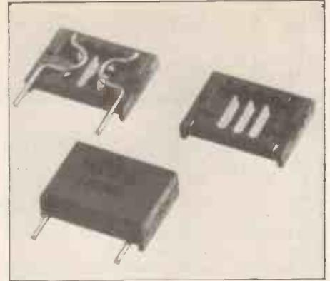
Fig. 8. Internal construction of a sealed spark-gap.
