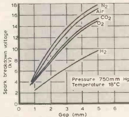
Fig. 6. Breakdown voltage between two 2.5mm dia. spheres in various atmospheres<sup>1</sup>.
