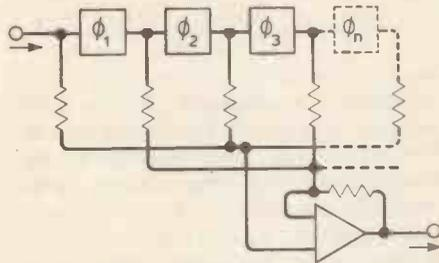
Fig. 2 Transversal filter. The tapped outputs along the delay line are added in alternate phases. At the section mid-frequency where  $\phi = 180^\circ$  all samples are fully coherent. Away from this phase position coherence declines, and a bandpass filter results.
