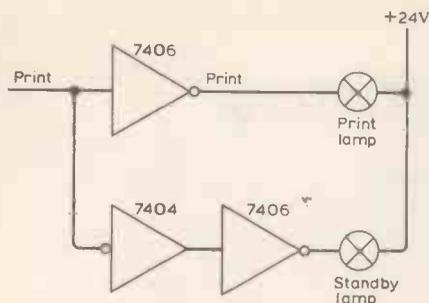
Fig. 5. Printer circuit, showing that ambiguities can appear.
