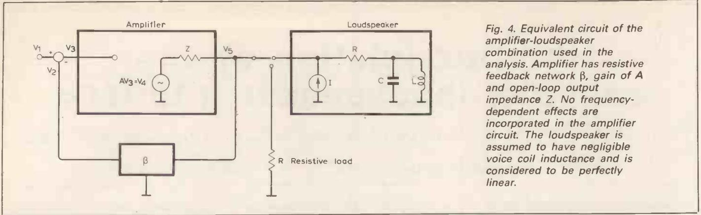
Fig. 4. Equivalent circuit of the amplifier-loudspeaker combination used in the analysis. Amplifier has resistive feedback network  $\beta$ , gain of  $A$  and open-loop output impedance  $Z$ . No frequency-dependent effects are incorporated in the amplifier circuit. The loudspeaker is assumed to have negligible voice coil inductance and is considered to be perfectly linear.
