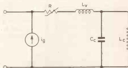
Fig. 3. Simplified loudspeaker equivalent circuit.  $L_C$  and  $C_C$  are cone dynamic mass and suspension compliance, respectively,  $L_v$  the voice coil inductance,  $R$  the voice coil resistance, including the radiation resistance, and  $i_g$  the generator effect current source.
