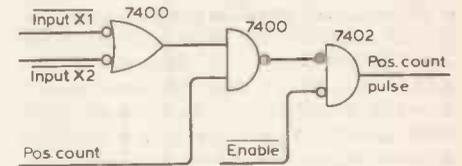
Fig. 3. Circuit of Fig. 1 drawn in 'intentional' symbols.
