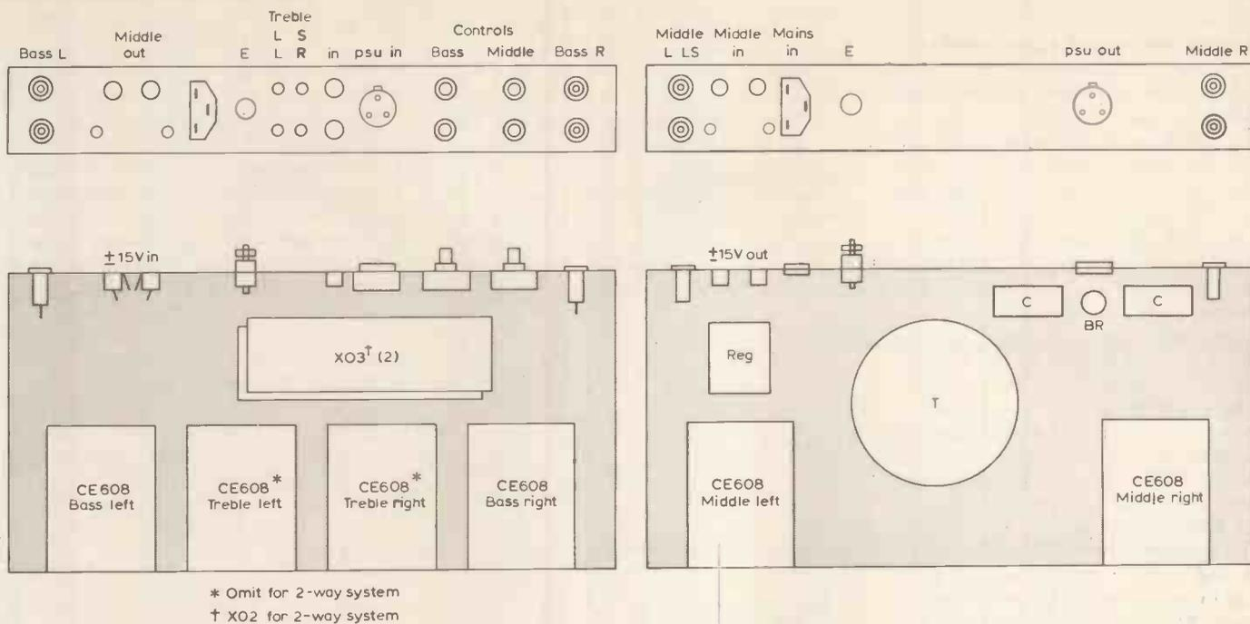
Fig. 9. Suggested layout of amplifiers and filters.
