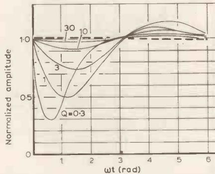
Fig. 5. Typical waveforms from equation 7 as functions of normalized time, with the resonant quality factor  $Q$  as parameter. The loudspeaker-generated oscillation is very large, especially for low values of  $Q$ . Corresponding waveform for resistive load is shown with a dashed line.
