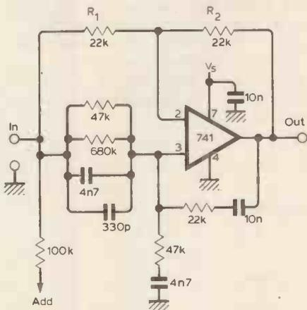
Fig. 6 All-pass section with  $f_o = 725\text{Hz}$  and  $m0.94$ . All resistors except the 680k are of 2% tolerance and all capacitors except the bypass and the 330pF are  $2\frac{1}{2}\%$  polystyrene. The actual value of  $R_1$  and  $R_2$  is not important but they should be a well matched pair.
