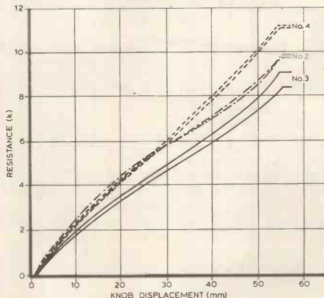
Fig. 21. Samples of characteristics of dual linear pots.
