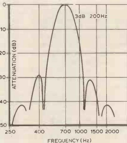
Fig. 10 Frequency response of the eight-stage cosine-on-pedestal model.
