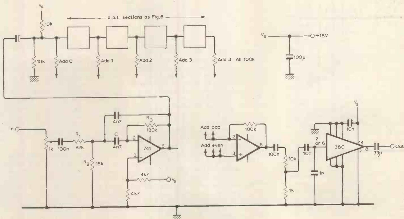
necessary to check that the output terminals (pin 6) are at about  $\frac{1}{2}V_s$ , and that the phase shift per section is  $180^\circ$  at 725 Hz. The latter test can be made by connecting both input and output taps of one section to the inverting input of the adder; the output of the adder should zero at the  $180^\circ$  frequency. If these tests are satisfied then all is probably well, though it is advisable to use an oscilloscope to test for self oscillation.
