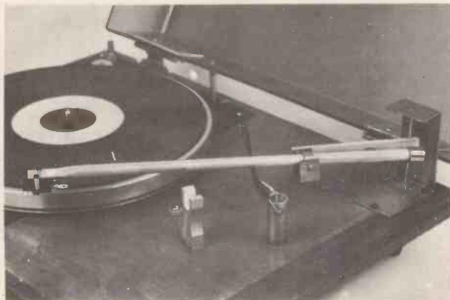
with tapered ends to form pivot points, are threaded into these holes, one from each vertical side face of the pivot block.
