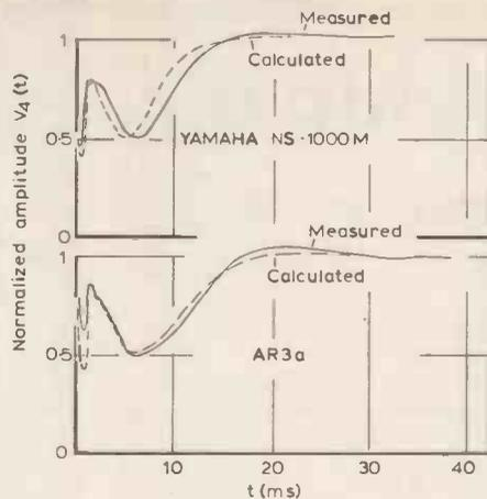
Fig. 7. Measured responses  $V_4(t)$  and calculated responses for the AR3a and NS-1000M loudspeaker systems. Only the two first resonances around 35Hz and 400Hz were taken into account in the calculated values. The good match of the responses show that the theoretical model used is satisfactory.
