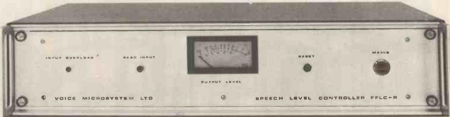
Precision control of speech amplitude, signal to noise ratio and waveform characteristics using a feedforward control process developed at University College, Swansea with NRDC backing (British Patent Application No. 12050/77). High speed digital processing techniques are employed using a Zilog Z80A microprocessor to sample and process the speech waveform.
