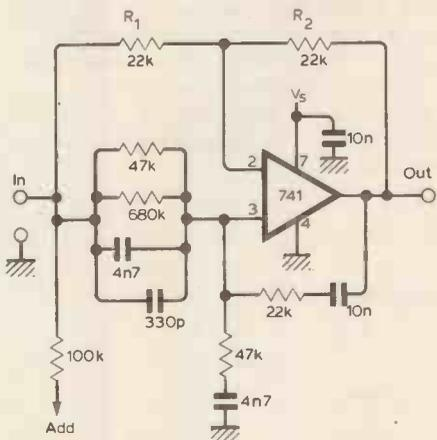
Fig. 6 All-pass section with  $f_o = 725\text{Hz}$  and  $m0.94$ . All resistors except the 680k are of 2% tolerance and all capacitors except the bypass and the 330pF are 2½% polystyrene. The actual value of  $R_1$  and  $R_2$  is not important but they should be a well matched pair.
