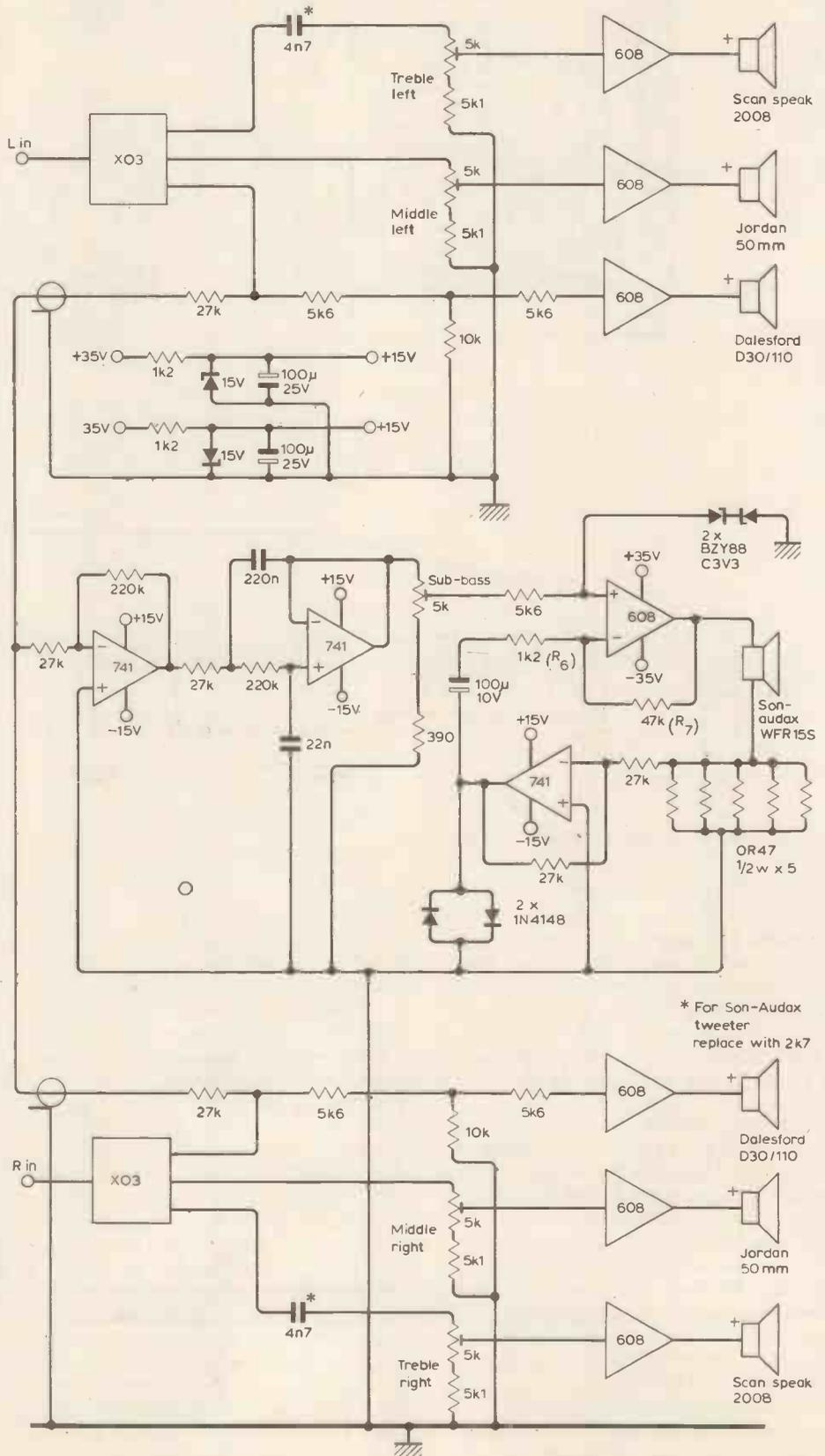
Fig. 8. Summing amplifier and filters for sub-woofer drive.
