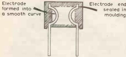
Fig. 4. Electrode arrangement.
