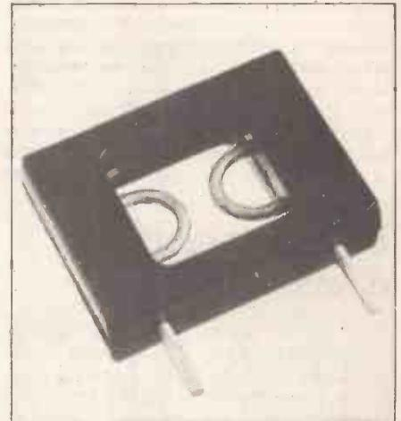
Fig. 1. Open construction spark-gap.
