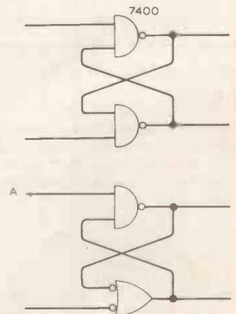
Fig. 4. Flip-flop circuit drawn in the conventional way (top) and in 'intentional' symbols.
