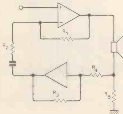
We know that with  $R_g = 0$ ,  $Q_{es} = 0.46$  and that  $R_e = 7.3$ , so from eqn. 2,  $\omega_s C_{mec} = 0.063$  and the required  $R_g$  is  $-3.7\Omega$ .
