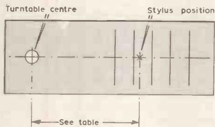
As the figures in the Table show, the magnitude of the tracking error becomes less as the effective length of the pick-arm increases. The vertical pivot in this design is located at a distance from the turntable which is the maximum for a given plinth size, so the effective length of the arm is virtually equal to its overall length.
