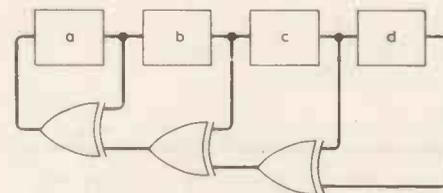
The problem of finding the appropriate connections is the subject of an extensive literature. A convenient starting point is "Shift Register Sequences" by S. W. Golomb (Holden-Day, 1967). Most of us find in this book a convenient finishing point, too. It contains a table of values of Mr Wood's  $a$  and  $b$  for values of  $a+b$  up to 36.
