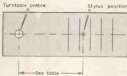
As the figures in the Table show, the magnitude of the tracking error becomes less as the effective length of the pick-arm increases. The vertical pivot in this design is located at a distance from the turntable which is the maximum for a given plinth size, so the effective length of the arm is virtually equal to its overall length.
