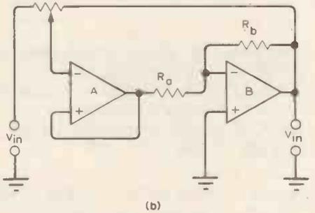
Fig. 23. Two circuits embodying the Fig. 22(b) idea. Circuit (b) uses voltage follower to avoid need for high-value resistors  $R_a$  and  $R_b$ .
