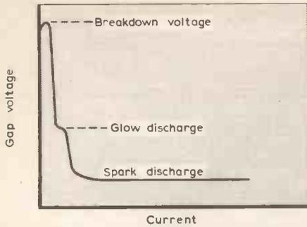
Fig. 3. Voltage - current characteristic of a two-electrode spark-gap.
