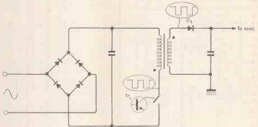
Fig. 16. Principle of the switched-mode power supply.
