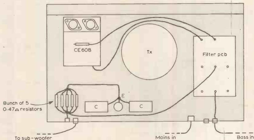
Fig. 10. Layout of sub-woofer amplifier and filter.
