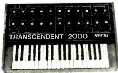
Designed by consultant Tim Orr (formerly synthesizer designer for EMS Ltd.) and featured as a constructional article in ETI, this live performance synthesizer is a 3-octave instrument transposable 2 octaves up or down giving sweep control, a noise generator and an ADSR envelope shaper. There is also a slow oscillator, a new pitch detector, ADSR repeat, sampe and hold, and special circuitry with precision components to ensure tuning stability amongst its many features.
