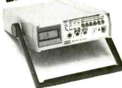
8050A 4 1/2 Digit LCD DMM with true RMS on AC volts and current DC volts 200mV-1KV, 10µV resolution AC volts. 200mV-750V, 10µV resolution. DC/AC current 200µA-2A, 0.01µA resolution resistance 200Ω-20MΩ, 0.01Ω resolution. Also reads dB direct referenced to 16 stored impedances. Conductance ranges 2mS and 200nS.
