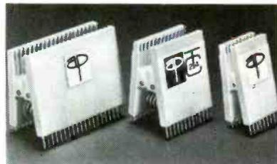
Clip an AP TEST-CLIP over an IC and you immediately bring up all the leads from the crowded board into an easy working level.
