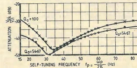
Fig. 4. Attenuation of the band-elimination filter with self-tuning frequency. V<sub>04</sub> = output of filter; V<sub>i1</sub> = interference signal.
