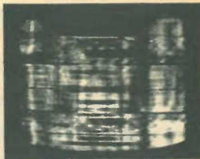
(b) Ionized F2 layer conditions caused reception of this picture in the UK from the USSR's TSS service close to the Chinese border on channel R1 (49.75MHz vision). The image shown features distortions typical of pictures received by F2 propagation.
