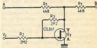
Fig. 2. Voltage-dependent resistor using a f.e.t., to be used for R in Fig. 1. Its value  $R' = (2R_1 + R_f^2/R_f) = \text{effective resistance between the terminals A and B. } R_f = \text{f.e.t. resistance, determined by the control voltage, } V_c. R_2 = \text{resistors for equalising the f.e.t. characteristics.}$
