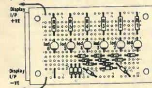
You will need: One EXP 300 or EXP 350 breadboard 15 silicon diodes 6 resistors 6 Light Emitting Diodes
