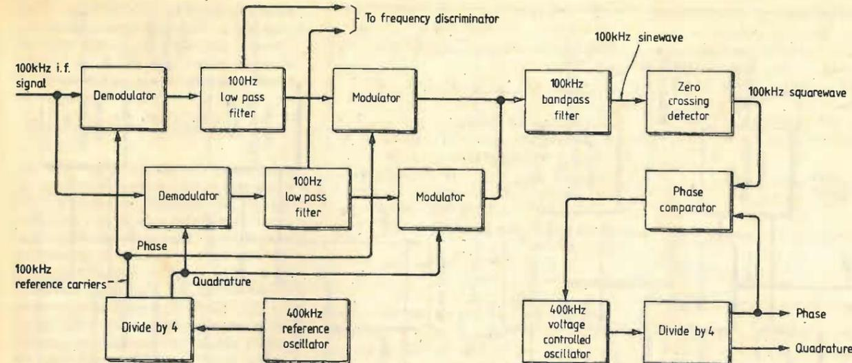
Fig. 2. Carrier filter for synchronous receiver
