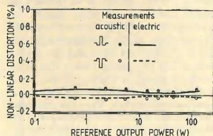
Fig. 11. Non-linear distortion of a Kenwood L-07 MII power amplifier. Broken lines represent electric measurement and solid lines acoustic measurement.
