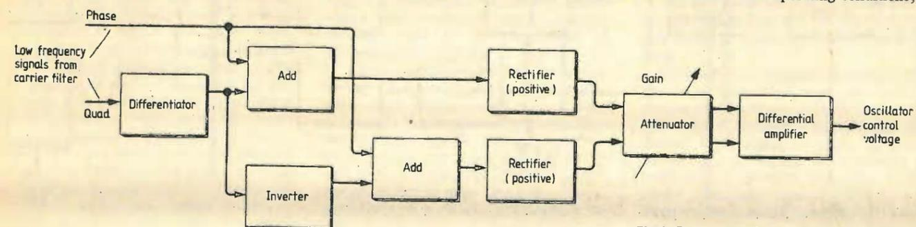
Fig. 3. Frequency discriminator for synchronous receiver
