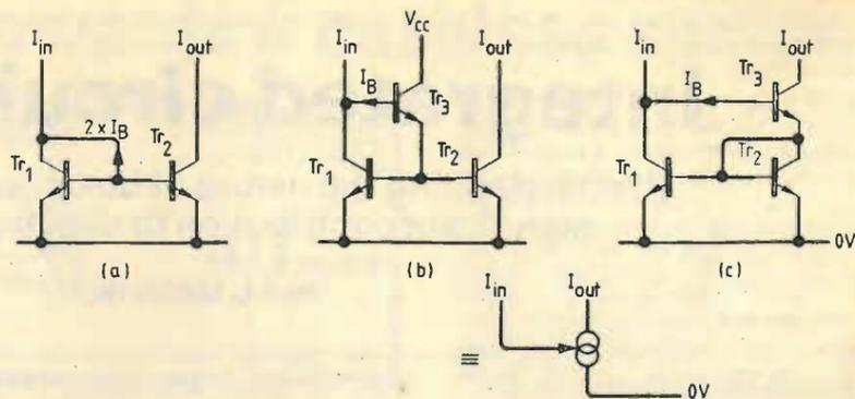
Fig.4. Output current mimics input current in these current mirror variations, all much more easily integrated than resistors and capacitors.
