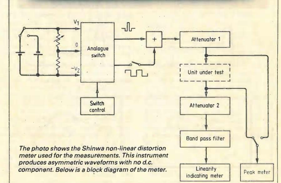
The photo shows the Shinwa non-linear distortion meter used for the measurements. This instrument produces asymmetric waveforms with no d.c. component. Below is a block diagram of the meter.
