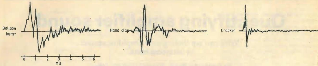
Fig. 1. Typical waveforms of transient sounds are asymmetric, with no d.c. component.
