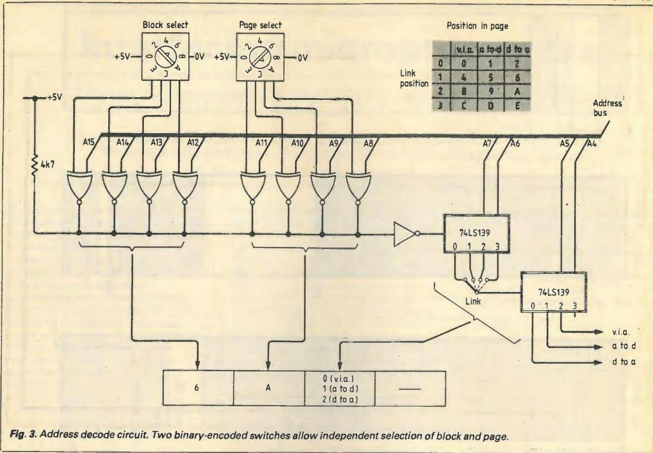
Fig. 3. Address decode circuit. Two binary-encoded switches allow independent selection of block and page.
