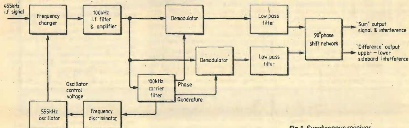
Fig. 1. Synchronous receiver
