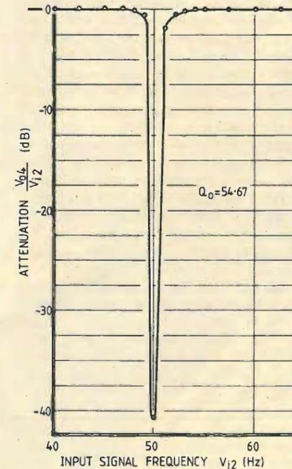
Fig. 5. Attenuation of the filter with frequency of input signal, V<sub>i2</sub>, the filter being self-tuned to the 50Hz power-line interference signal, V<sub>i1</sub>. V<sub>04</sub> = output of filter; V<sub>i2</sub> = physiological data signal with the interference signal present.
