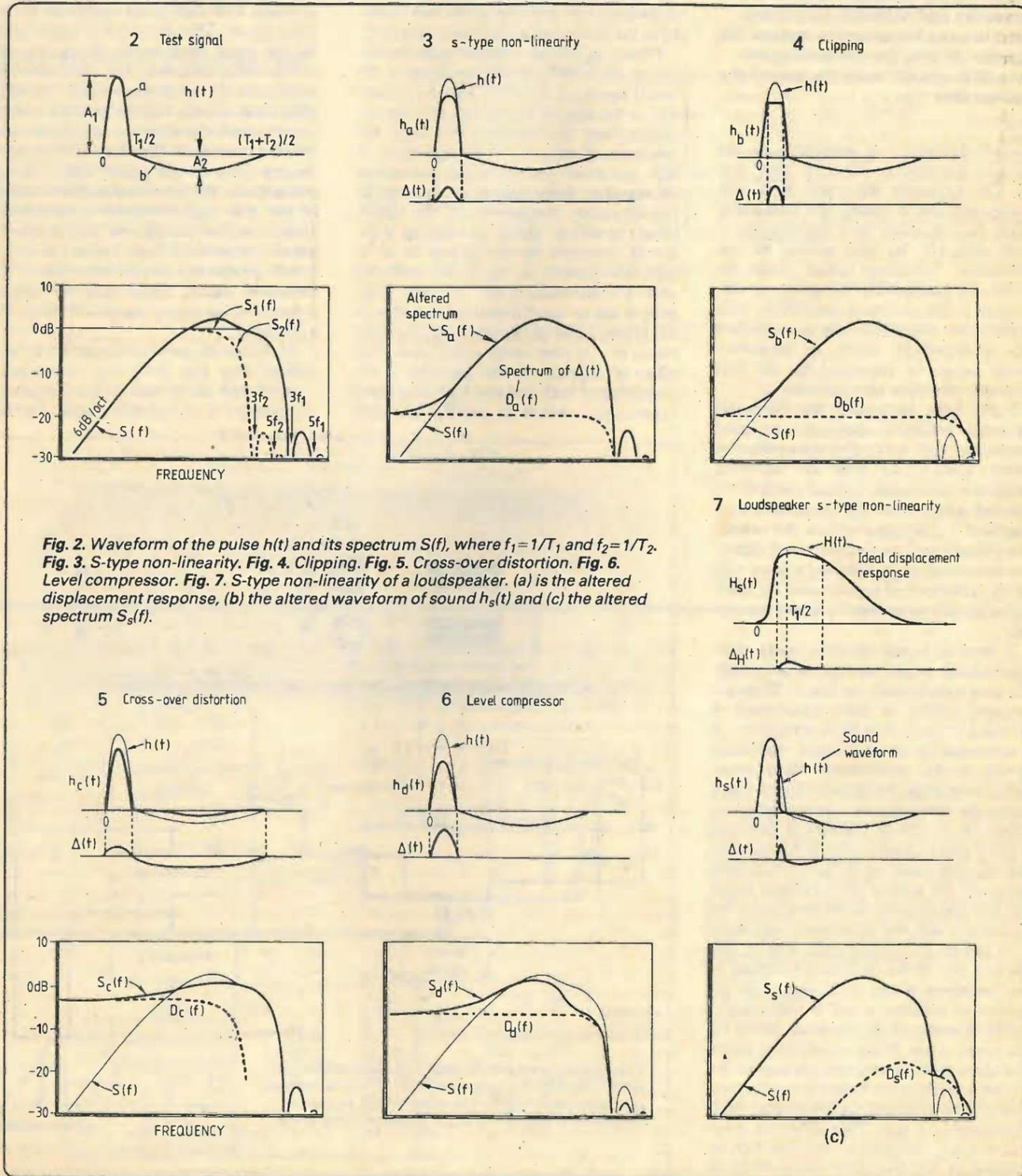
Fig. 2. Waveform of the pulse  $h(t)$  and its spectrum  $S(f)$ , where  $f_1=1/T_1$  and  $f_2=1/T_2$ . Fig. 3. S-type non-linearity. Fig. 4. Clipping. Fig. 5. Cross-over distortion. Fig. 6. Level compressor. Fig. 7. S-type non-linearity of a loudspeaker. (a) is the altered displacement response, (b) the altered waveform of sound  $h_s(t)$  and (c) the altered spectrum  $S_s(f)$ .
