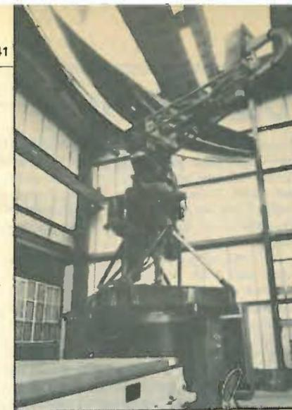
Plessey's AWS-5 radar being vibration tested.
